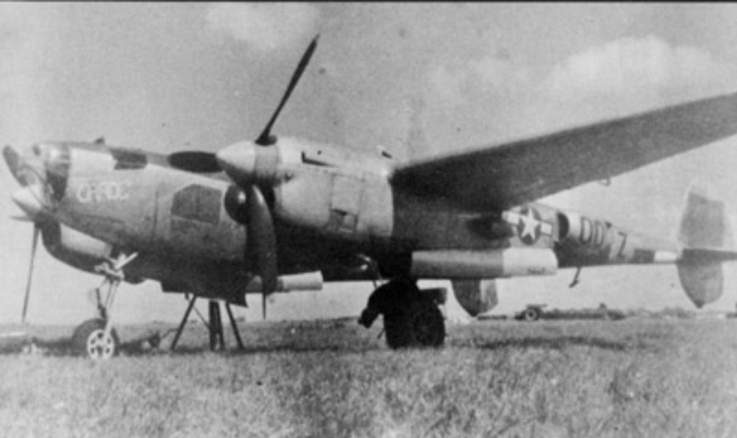
CAROL was a P-38J Droop Snoot of the 82nd Fighter Group. The Droop Snoot conversions were kits built by Lockheed's Modification Center and shipped to combat units for installation in the field. (SGT James Crow)
