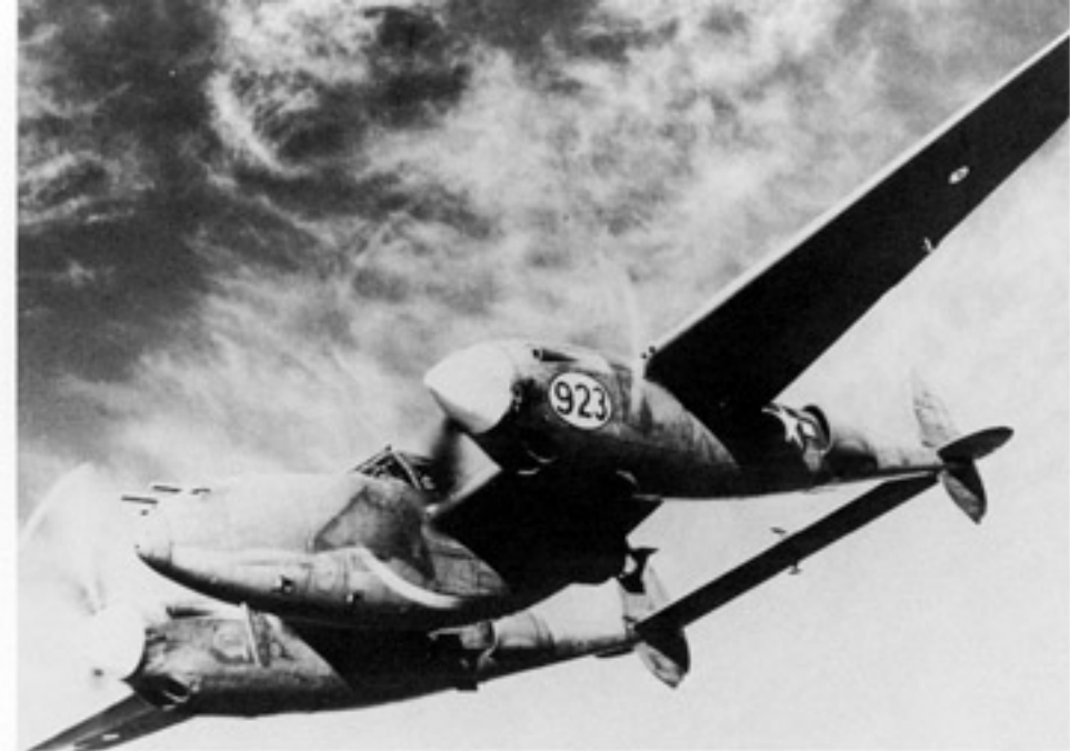
This P-38H is armed with a pair of 500 pound bombs under the wing center section. The aircraft was assigned to Orlando, Florida and used to develop tactics for the P-38. With its strengthened wing and additional power, the P-38H could carry a bomb load equal to a B-17 bomber. (USAF)
