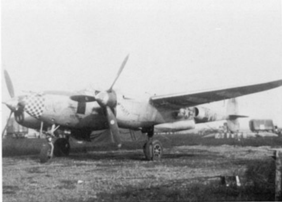
My California Cutie/Mary was a P-38J from the 485th FS/370th FG at Florennes, Belgium. The Black cross on the aircraft data block on the nose indicates that this P-38J had fuel tanks installed in the wing leading edges. (AFM)
