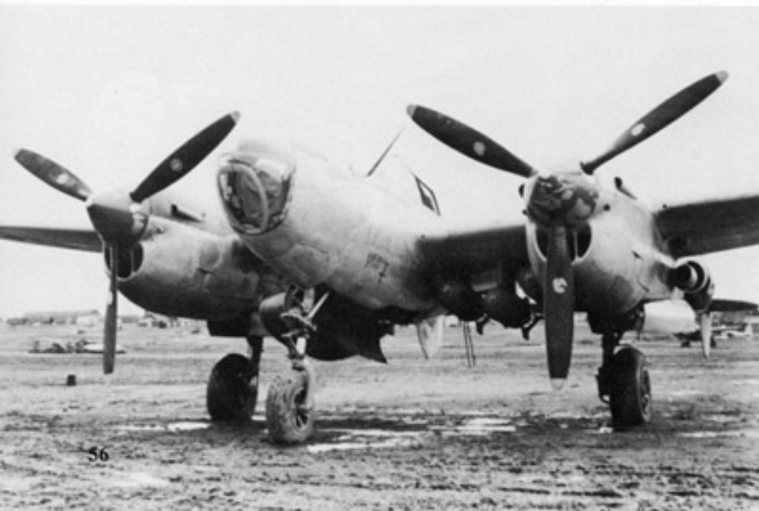
This P-38J Droop Snoot was assigned to the 96th FS/82nd FG at Vincenzo Airfield, Italy. The aircraft is armed with three 500 pound bombs and a 165 gallon drop tank. The radio antenna mast was installed at an angle on all Droop Snoot aircraft. (Lockheed)
