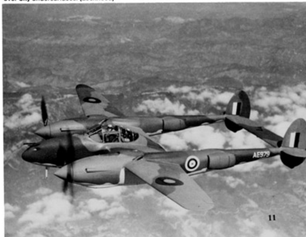
A Lightning I (AE 979) on a test flight over California. The carburetor intake scoop is visible on the boom above the wing. The two pipes exiting above the wing are the engine exhausts, unique to the Lightning I. The RAF camouflage was Dark Earth and Dark Green uppersurfaces over Sky undersurfaces. (Lockheed)
