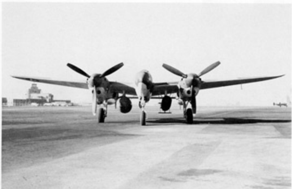
A P-322 Lightning Mk II equipped with one 300 gallon drop tank and a 2,000 pound torpedo. The Lightning II was equipped with standard supercharged Allison F-series engines and were designated as P-38F-13, F-15, and G-15 by the USAAF and were assigned AAF serials. (Lockheed)
