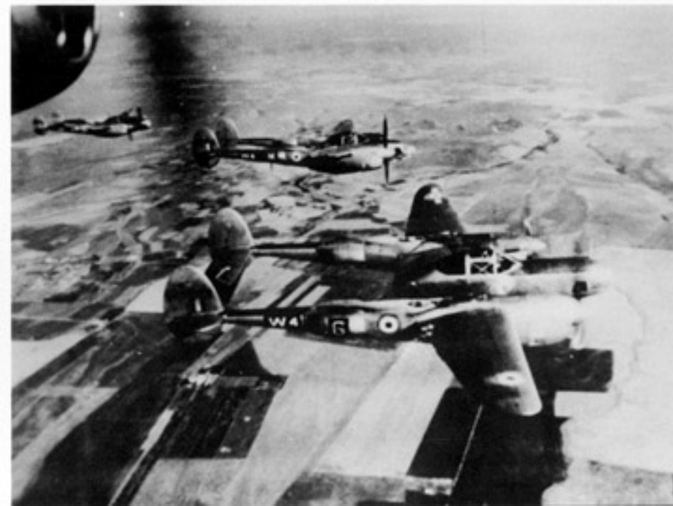
Three French Air Force F-5G-6s of GR 2/33 fly over Europe during 1945. The Free French obtained F-4 and F-5 aircraft under the Lend Lease Act. The aircraft in the foreground has had the French roundel simply painted over the U.S. star and bar insignia on top of the port wing. (Hans-Heiri Stapfer)
