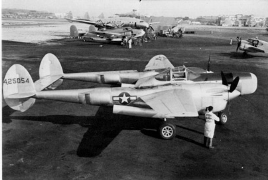
The P-38 Pathfinder was based on the P-38J and L airframes. The P-38J Droop Snoot was a conversion kit that a combat unit could assemble in the field, while the Pathfinder conversions were all modified at Lockheed's Dallas Modification Center. (Lockheed)
