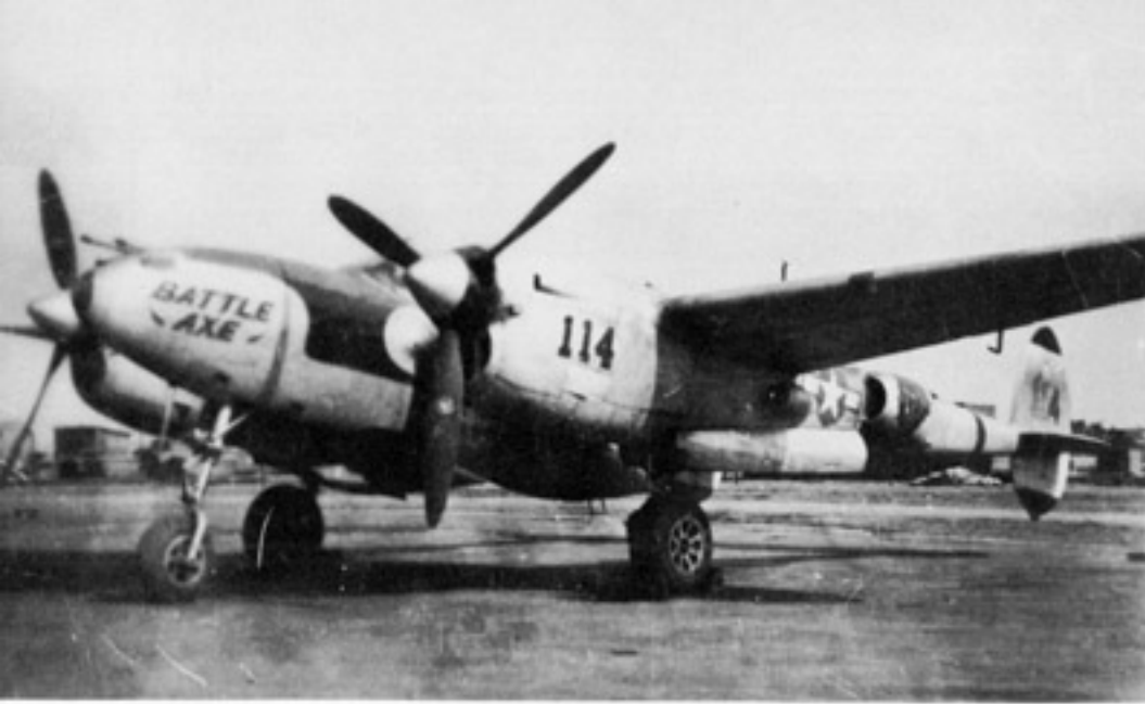
BATTLE AXE was a P-38J-25 from the 431st FS/475th FG based at Biak Island during 1944. Without knowing the aircraft serial number, it is virtually impossible to distinguish a P-38J-25 from a P-38L, since all external features between the two are identical. (Don Garrett, Jr.)
