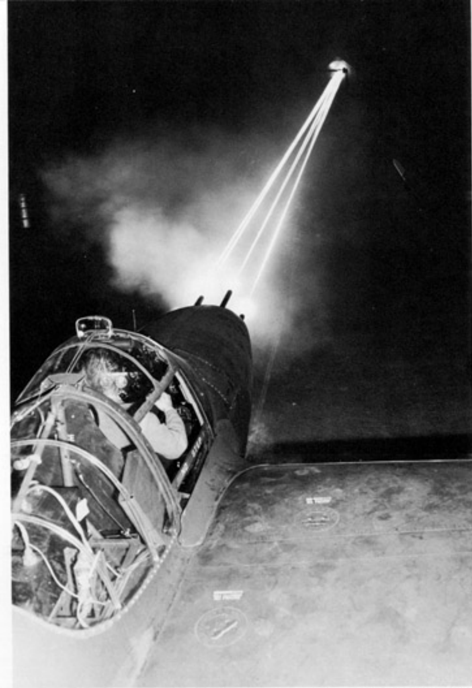
The concentrated firepower of the P-38s four .50 caliber machine guns is demonstrated during a night bore-sighting test. All four machine guns and the 20mm cannon were bore-sighted to fire straight ahead. This is a late P-38F with the rearward opening canopy. (Lockheed)
