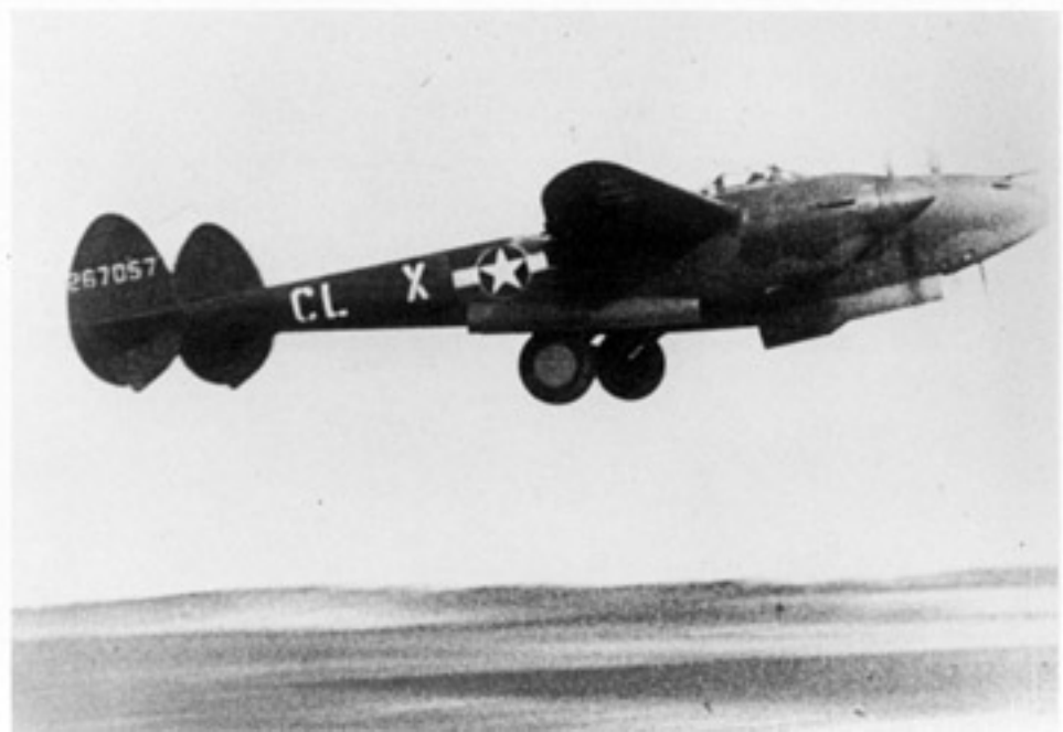
A P-38H of the 338th FS/55th FG takes off from Nuthampstead, England during 1943. The P-38 was the first operational fighter aircraft in the history of the USAAF to be equipped with a tricycle landing gear. (Lockheed)
