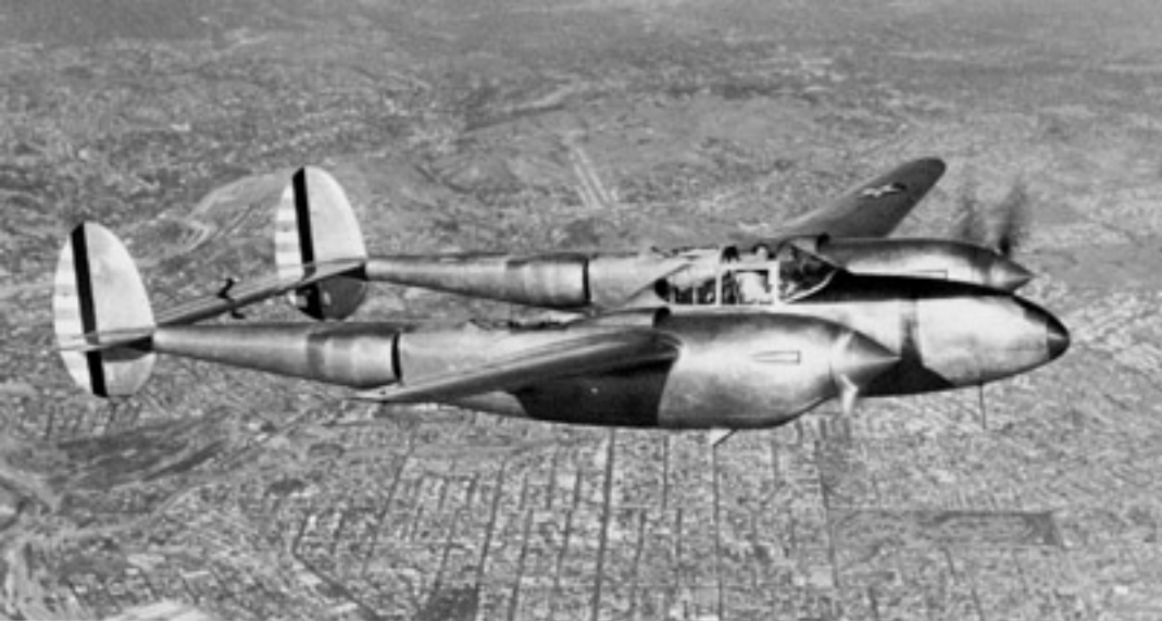
Lockheed Test Pilot Milo Burcham flies a YP-38 (39-689) over Los Angeles during late 1940. The YP-38 had an air scoop mounted ahead of the turbo-supercharger and external mass balances on the elevator. The open scoops under the engine nacelle are for the oil cooler exhaust. (Lockheed)
