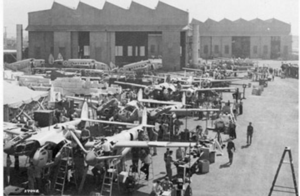
P-322 Lightnings undergo final assembly on the outdoor production line at Lockheed (the aircraft in the background are Hudson bombers). With the normally superb weather in Southern California, many aircraft were completed in outdoor assembly areas such as this one. (Lockheed)
