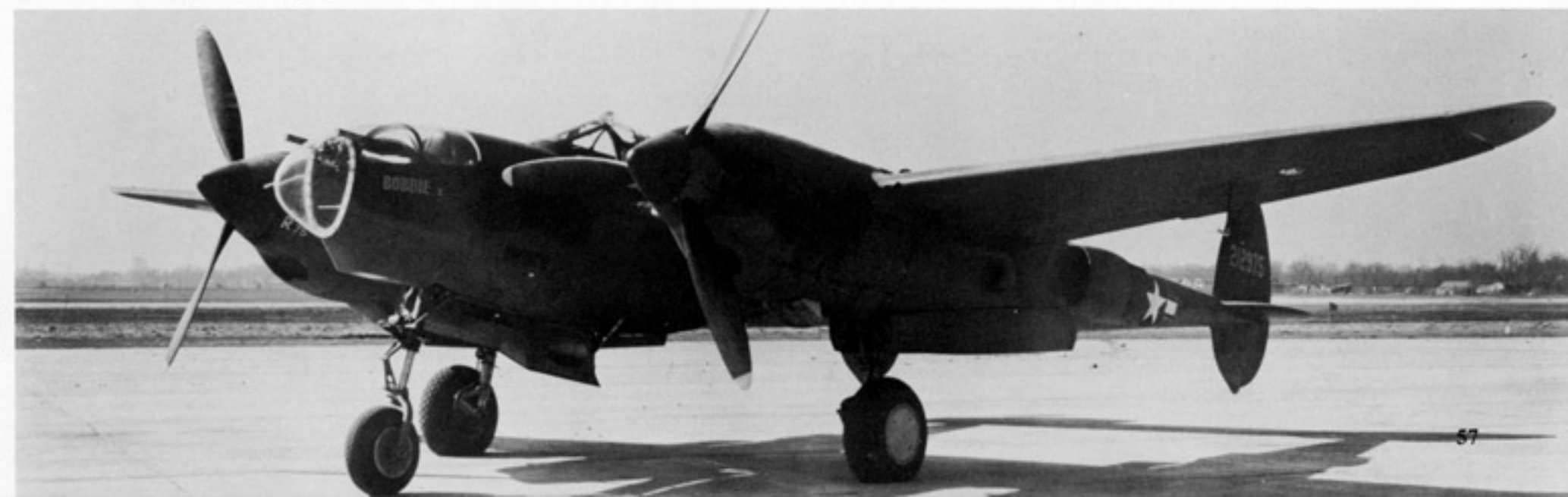
Although this aircraft appears to be a Droop Snoot P-38, it is actually the XF-5D Photo Lighting, which was an F-5A modified with a short camera bay, a navigator's station, and a pair of .50 caliber machine guns. (Art Krieger)
