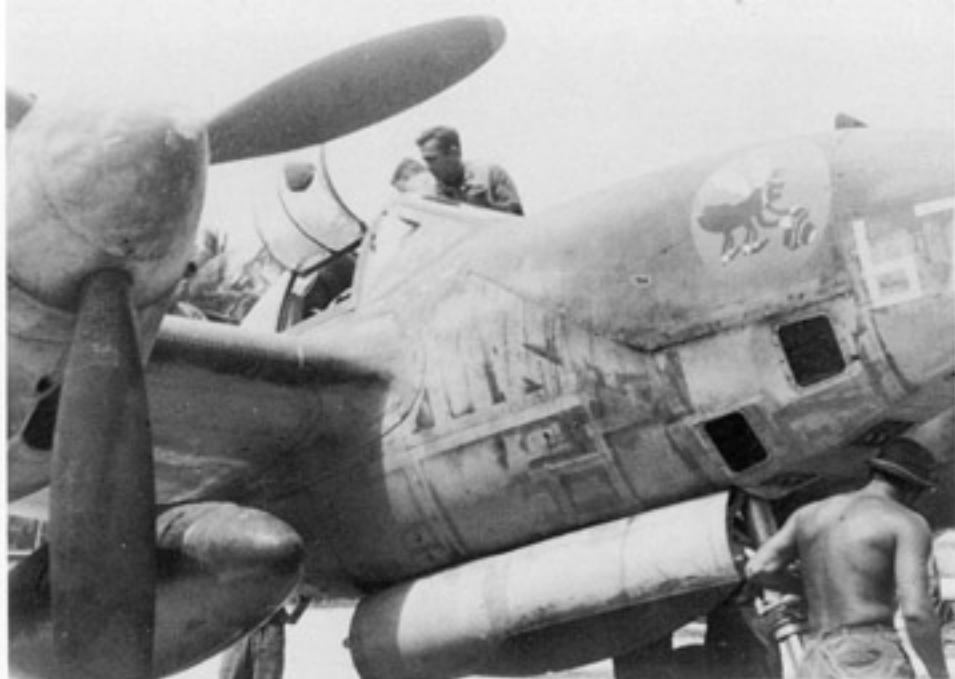
An F-4-1-LO of the 17th Photo Reconnaissance Squadron at Fighter Strip 2 on Guadalacanal during 1943. This F-4-1-LO has been modified with the addition of a pair of K-17 oblique cameras in addition to the normal vertical cameras. (Canning)
