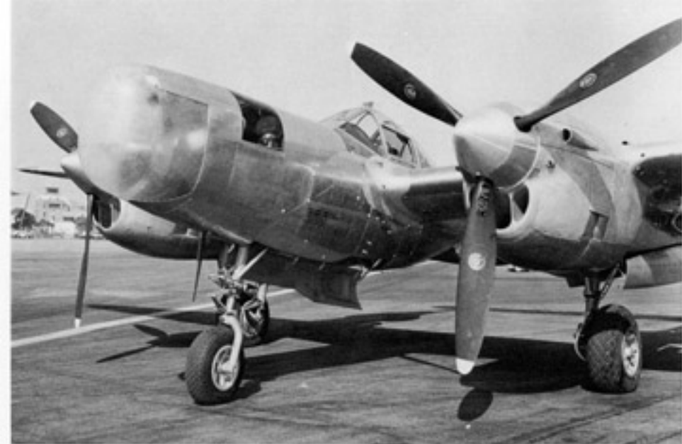
A variant of the Droop Snoot was the P-38 Pathfinder aircraft. The Pathfinder was fitted with AN/APS-15 Bombing Through Overcast (BTO) radar housed in an oblique plastic nose cap in place of the usual Norden visual bombsight. (Lockheed)
