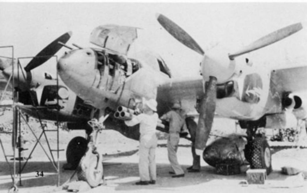
Armorsmen mount 4.5 inch bazooka rocket tubes to the fuselage sides of this P-38J of the 459th FS/80th FG in India. Known as the "Twin-Tailed Dragons," the 459th FS flew both air-to-air and air-to-ground missions against Japanese positions in Burma and China. (Ernie McDowell)
