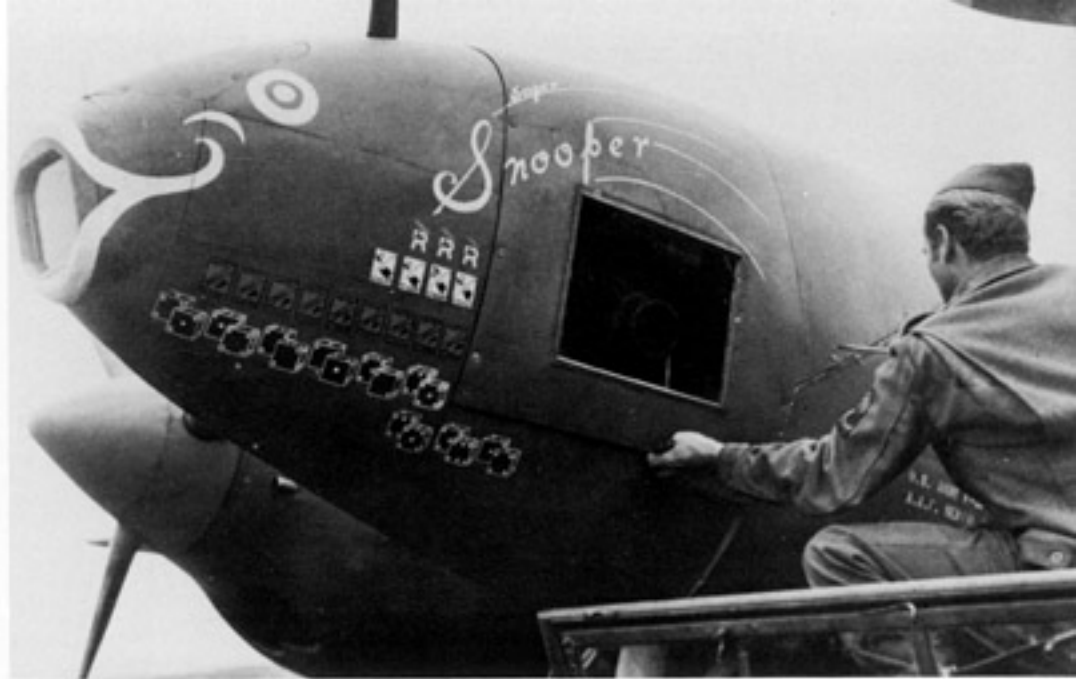
Super Snooper was an F-4A-1 of the 33rd PRS/10th PRG at Exchwege, Germany, during 1945. The Photo Lightning was equipped with a forward oblique (or dicing) camera in the nose and carried "dice" as mission markings. (AFM)
