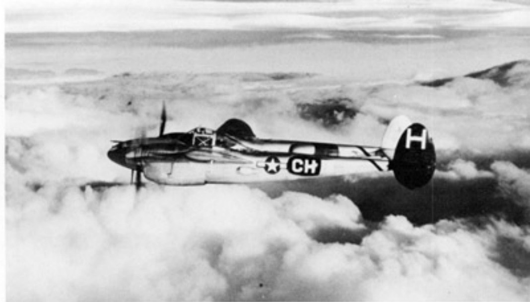
A P-38L of the 82nd Fighter Group on patrol over Italy during 1944. The P-38L was externally virtually identical to the P-38J-25 differing primarily in the power plants installed. The P-38L was powered by the Allison V-1710-F30R and L engines rated at 1,600 hp in the War Emergency setting. (Lockheed)
