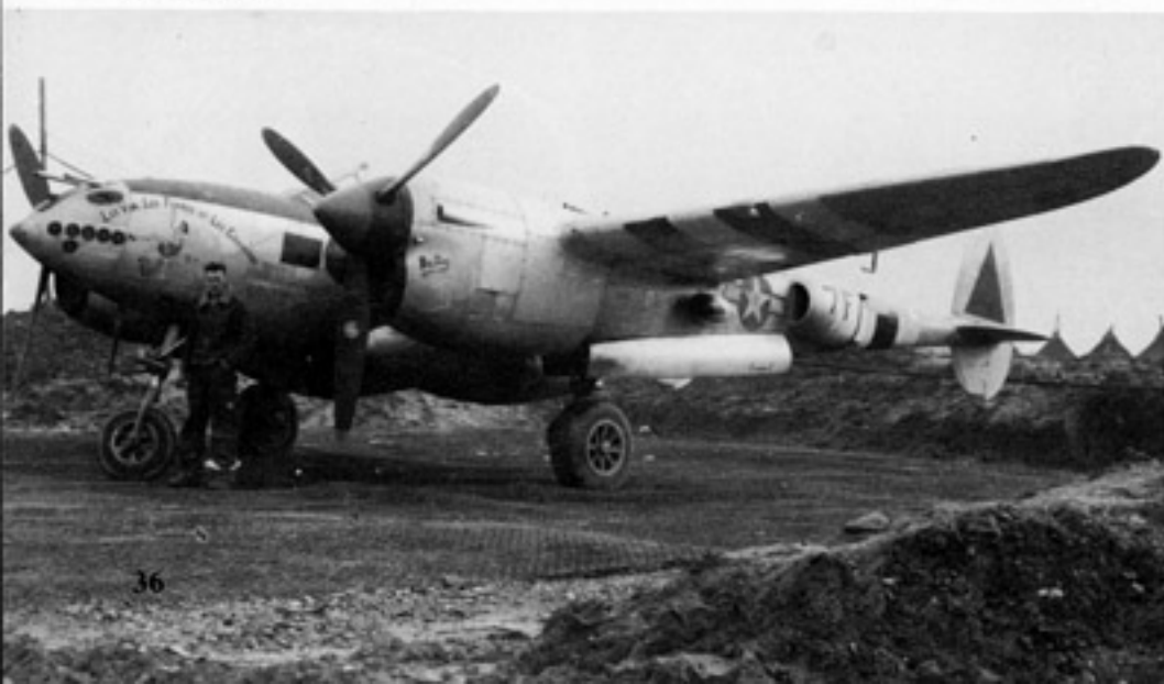
Les Vin, Les Femmes, et Les Chansons , French for "Wine, Women, and Song," was flown by MAJ Sabo, CO of the 485th FS at Florennes during the Fall of 1944. The aircraft is a P-38J-25 (44-23675) with the landing light in the wing leading edge and dive recovery flaps. (Lockheed)
