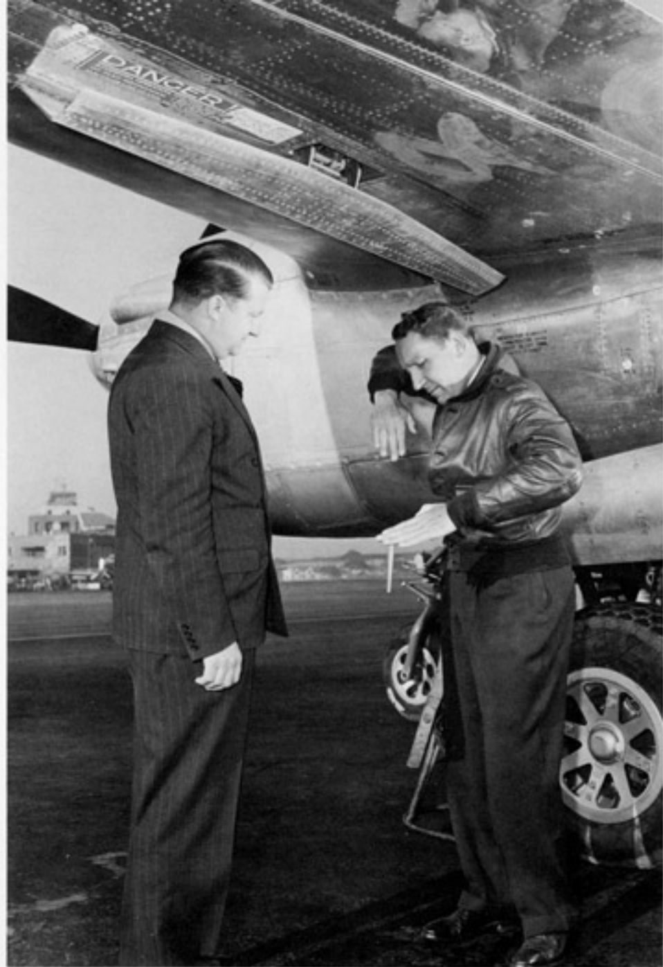
Kelly Johnson and Milo Burcham discuss the flying characteristics of the P-38J-25 equipped with the "dive recovery flaps" (which are visible above their heads). These flaps effectively eliminated the compressibility problem with the P-38. (Lockheed)
