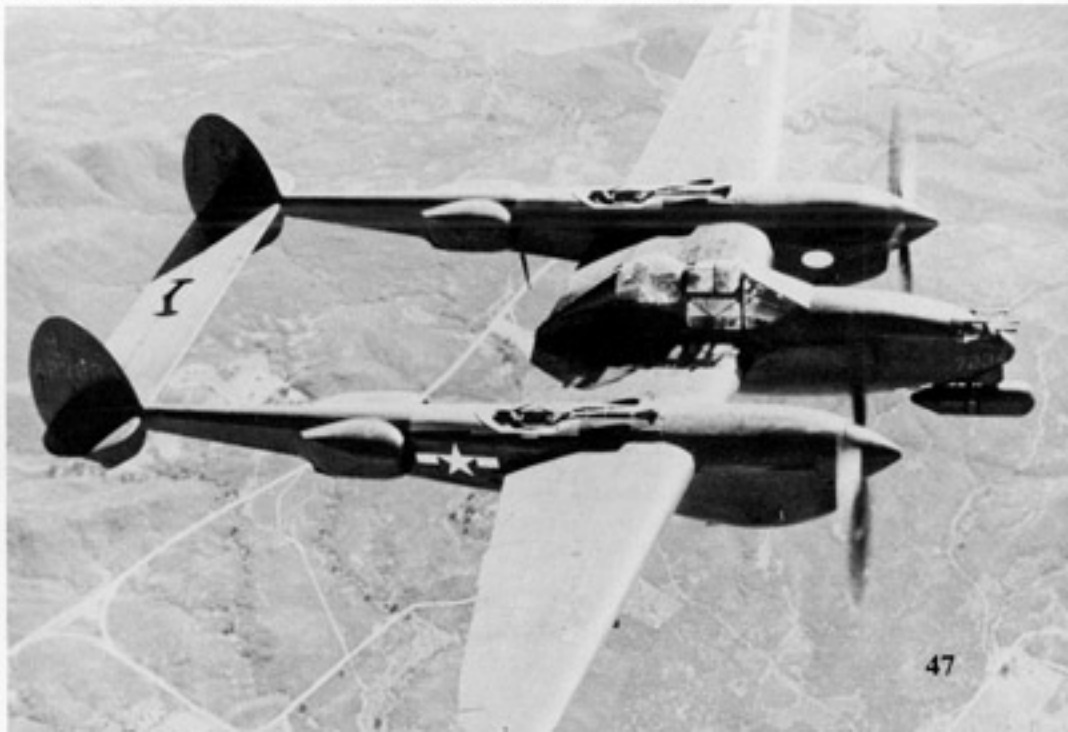
The P-38M Night Lightning had the radio antenna mast moved from under the nose to a position under the port boom near the radiator housings. (Lockheed)
