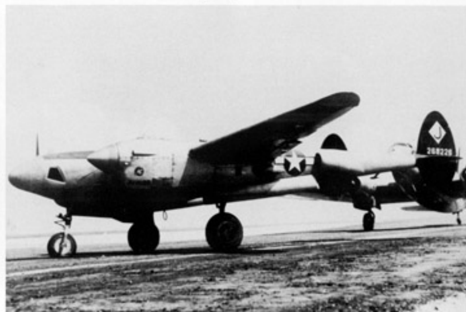
JUNIOR , an F-5E-2, taxis out at Yontan Airfield on Okinawa during July of 1945 ahead of a C-46 transport. The aircraft carried the late Black tail markings of the 28th PRS. Lockheed modified 100 P-38Js to F-5E-2 standards. (AFM)
