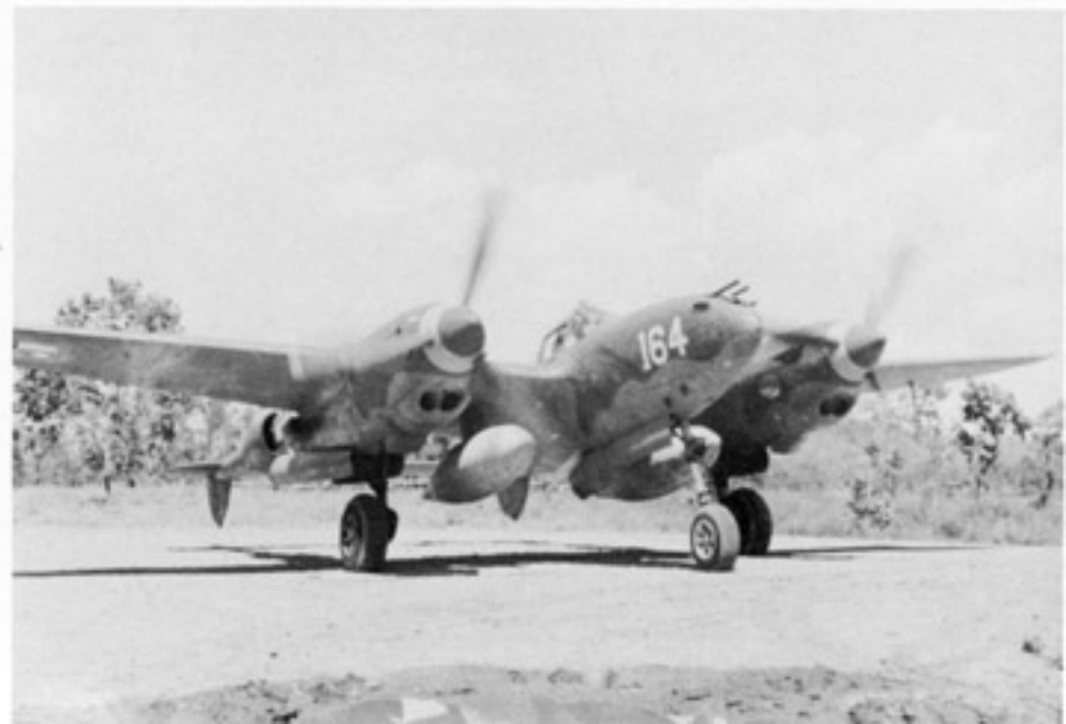
LT George Prentice flew this P-38G when he was assigned to the 432nd FS/475th FG at Dobodura, New Guinea, during 1943. The spinners and tail tips are Yellow with White trim, while the numbers on the nose and tail are in White with a Yellow border. (Jeff Ethell)
