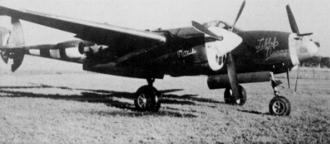
Libb Nanny/Roxie , a P-38J of the 77th FS/20th FG parked on the grass at Kings Cliffe. The aircraft has suffered some battle damage to the right rudder. The nose was polished metal with a White band in the hope that Luftwaffe pilots could mistake it for one of the unarmed "Droop Snoot" P-38s. (AFM)
