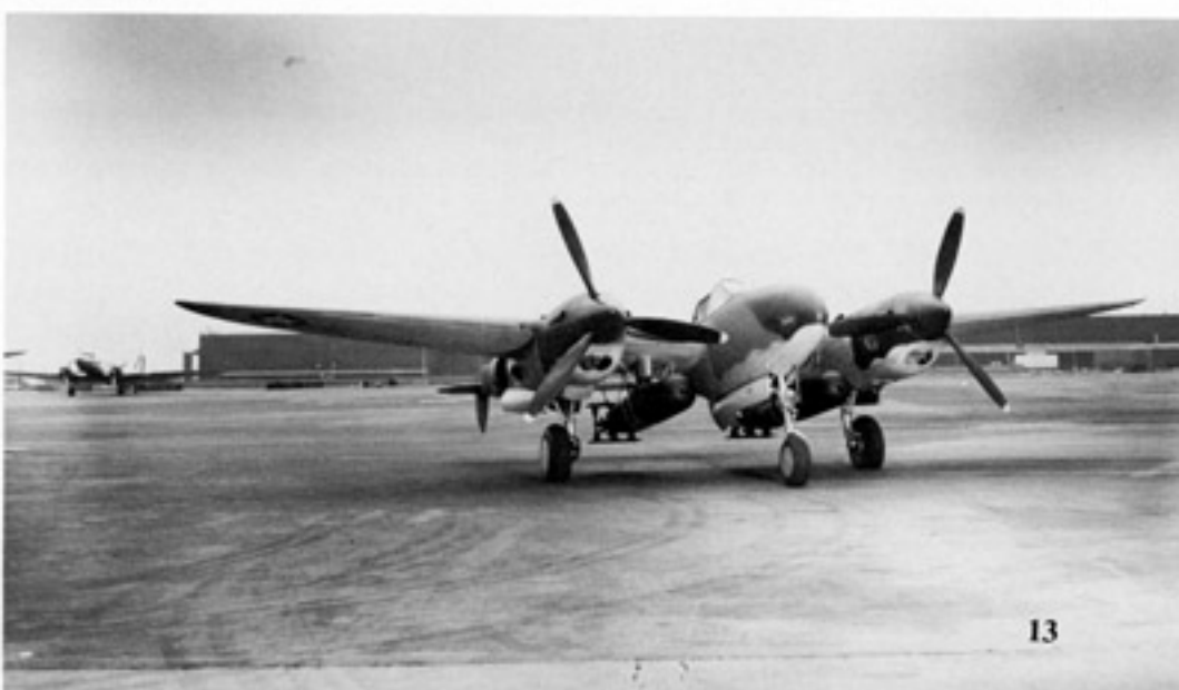
The first Lightning II, AF221 (serial 43-2035), reveals the great load-carrying capability of the P-38 wing. The aircraft is configured with a pair of 2,000 pound Navy torpedos under each wing. For the test flights the torpedos were secured in place with steel cables. (Lockheed)
