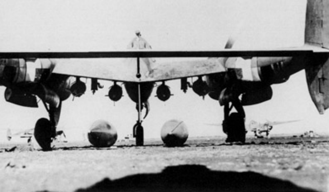
This Lightning of the 82nd Fighter Group in Italy is armed with four 500 pound bombs and will also be loaded with the two 165 gallon drop tanks on the ground under the aircraft. This was a field installation, since no factory P-38 had over one pylon under each wing center section. (Lockheed)
