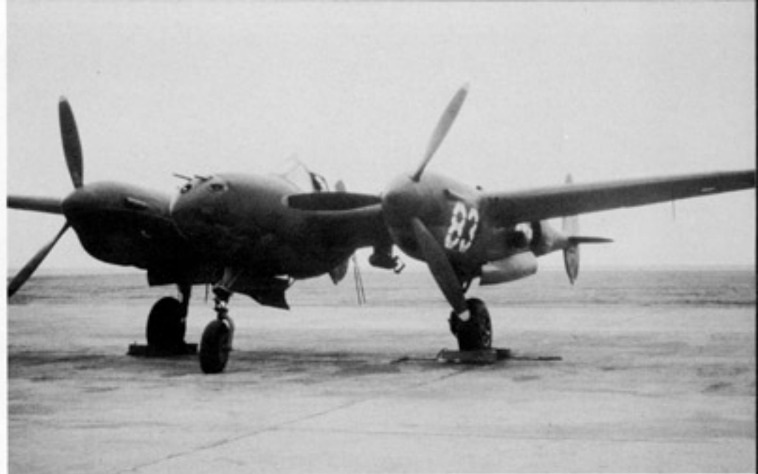
This P-38G is armed with 100 pound practice bombs at a training base in Florida during late 1943. The P-38G was externally identical to the P-38F differing only in the power plants with improved engine controls. (USAF)
