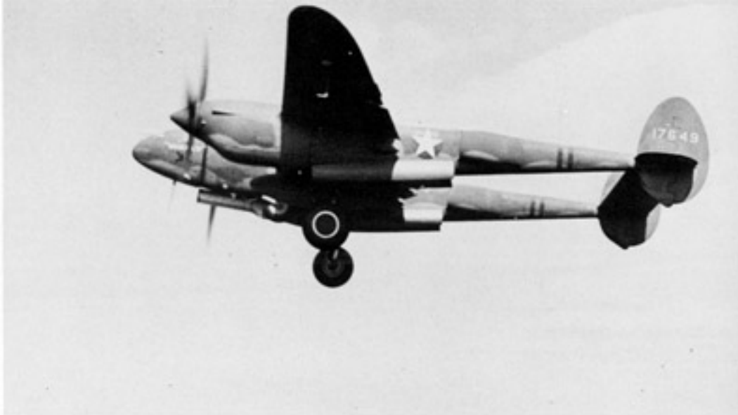
WALLY , a P-38F of the 48th FS, was flown by the unit's Commanding Officer during late 1942. At the time, the unit was attached to the 14th FG, based at Youks-Les-Bains, Algeria. The P-38F differed from the P-38E in having the pitot tube moved from under the nose to under the port wing. The propeller spinners and bands on the boom are in Red. (AFM)
