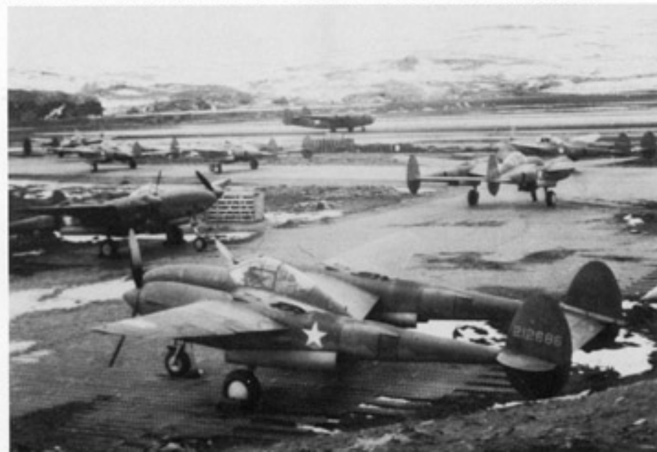
A pair of F-5A-1s share the Marston matting ramp at Adak with fighter P-38s during the Summer of 1942. Lockheed built twenty F-5As using modified P-38G airframes. (AFM)
