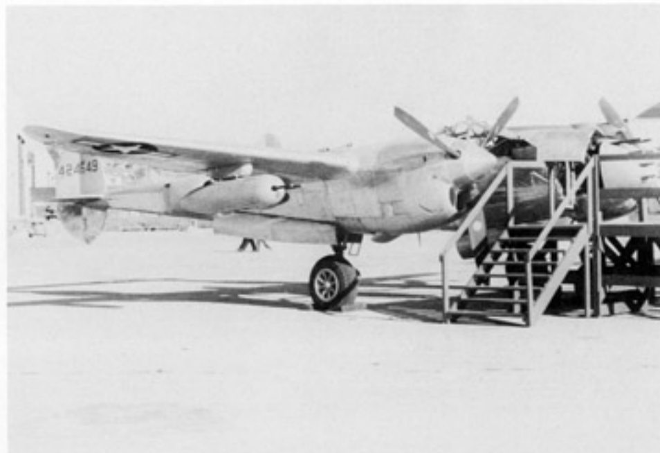
Armament testing with the P-38 went on constantly throughout the war. This P-38L has eight .50 caliber machine guns in the nose and four additional guns housed in pods under the wings. Another P-38 was tested with .60 caliber machine guns. (Fred Dickey via Ernie McDowell)
