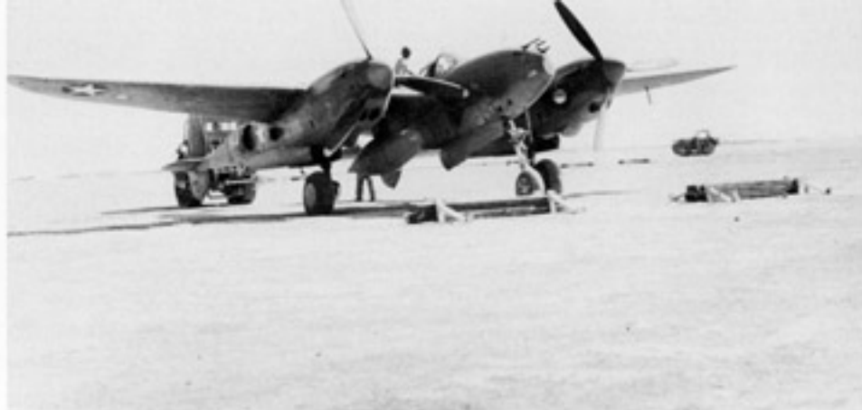
A Cietrac tow tractor pulls a P-38F of the 82nd FG/12th AF away from the wooden wheel stops on the compass check stand at Telergma Air Field, Algeria. The Lightning is carrying a single drop tank. The small bright area on the nacelle is a patch of polished metal used like a mirror to check the nose wheel position. (USAF via Jeff Ethell)
