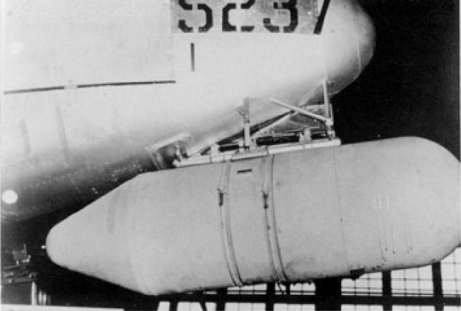
This AN/APS-4 AI radar pod was mounted on a modified drop tank pylon on the P-38J that served as the prototype for the P-38M. The aircraft was built at Wright Field in the Summer of 1944. (AFM)
