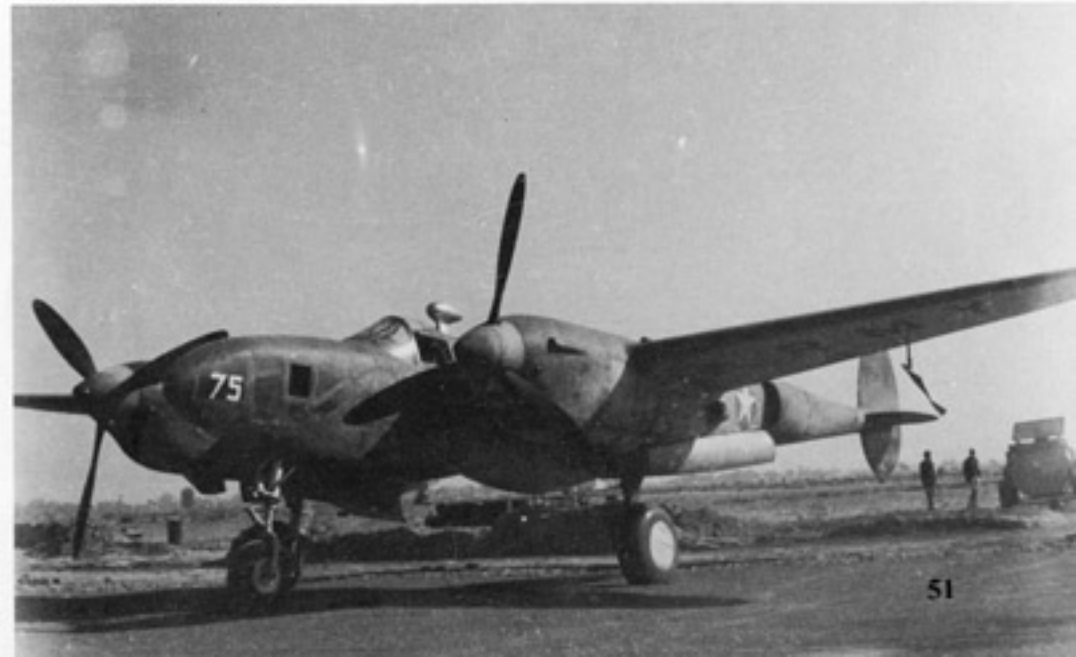
This F-4A-1 of the 8th PRG in India carried a football-shaped ADF loop antenna over the canopy. Haze camouflage involved painting the entire aircraft Black, then over-spraying it with White in varying degrees. The large square camera oblique window was a feature of the F-4A-1. (Vaclav Simecek)
