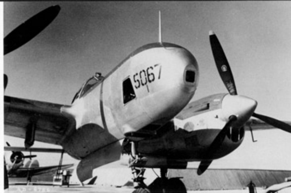
The F-5G Photo Lightning used a P-38L-5 airframe with a camera nose employing a forward looking oblique, or "dicing" camera in addition to the K-17 oblique and K-18 vertical cameras. (Lockheed)
