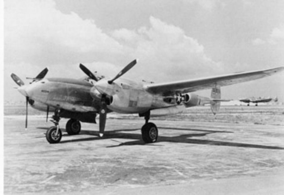
A new production P-38J-10 on the Lockheed ramp at Burbank, California during 1944. The P-38J-10 first introduced the flat-panel armored windscreen. The radiator housings on the rear portion of the boom were also redesigned being larger and more streamlined. The aircraft in the background is a TWA Lockheed 049 Constellation undergoing taxi trials. (Lockheed)
