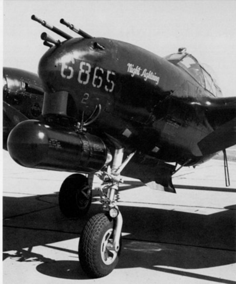
Night Lightning , a new production P-38M on the ramp at Lockheed's Dallas, Texas, facility. The AN/APS-4 AI radar pod was mounted under the nose with a modified P-38 drop tank pylon. The guns were all fitted with flash hiders to keep from blinding the pilot when they were fired at night. (Lockheed)
