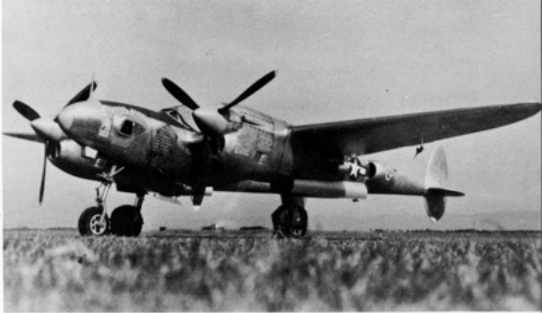
TURBO ANNY was a highly decorated F-5E-2 of the 34th PRS/69th TRG based at Haguenau, France during the Spring of 1945. She carried at least 111 small Swastikas on the nose indicating photo missions over Germany. The unusual shroud ahead of the forward K-17 camera was designed to keep debris off the camera window. (Chris Goodman via Art Krieger)
