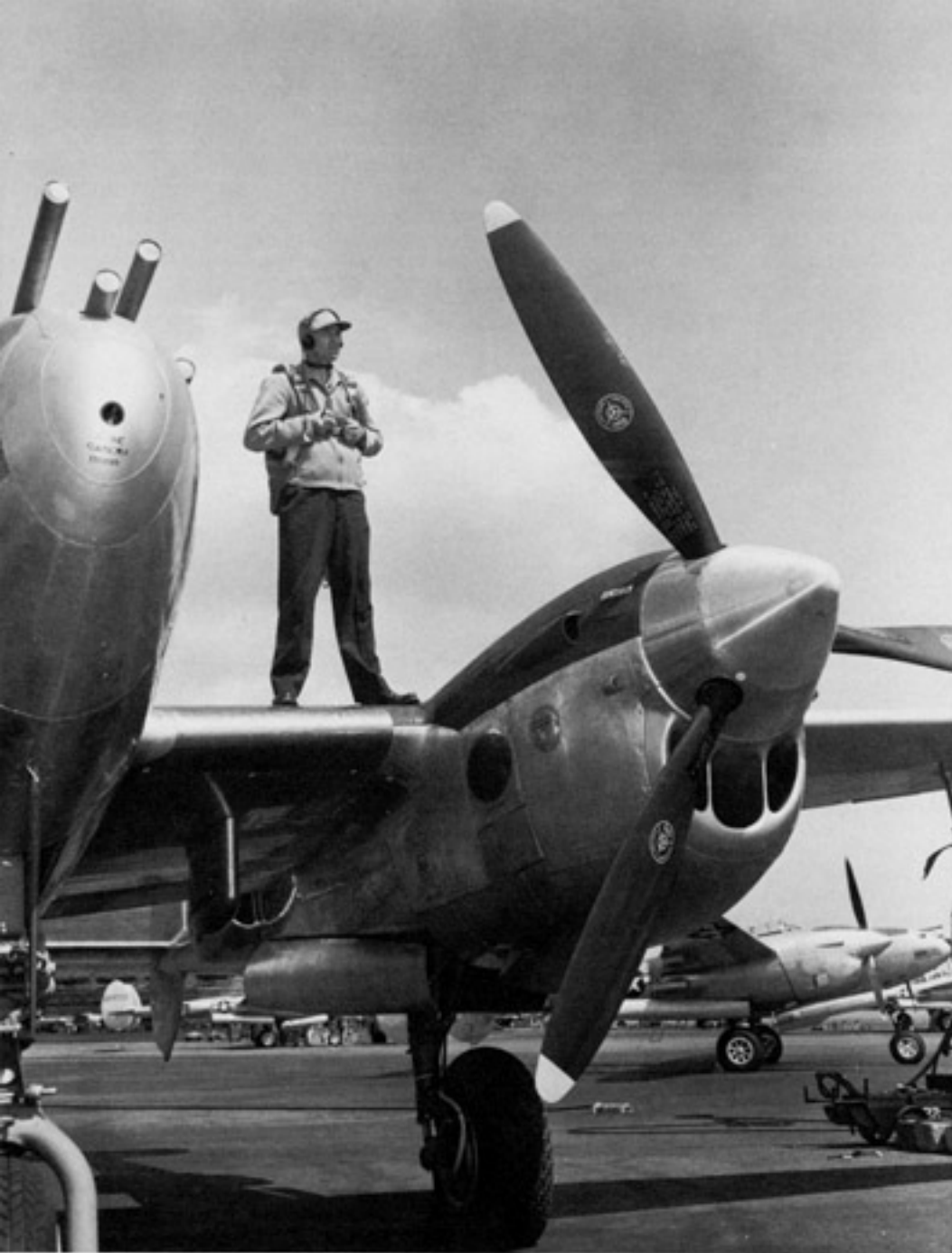
Lockheed Test Pilot Milo Burcham on the wing center section of a new production P-38J. The installation of the oil intercooler in the chin fairing allowed the space within the wing leading edge to be used for fuel. The polished oval panel on the inside of the engine nacelle allowed the pilot to visually check the nose gear position. (Lockheed)
