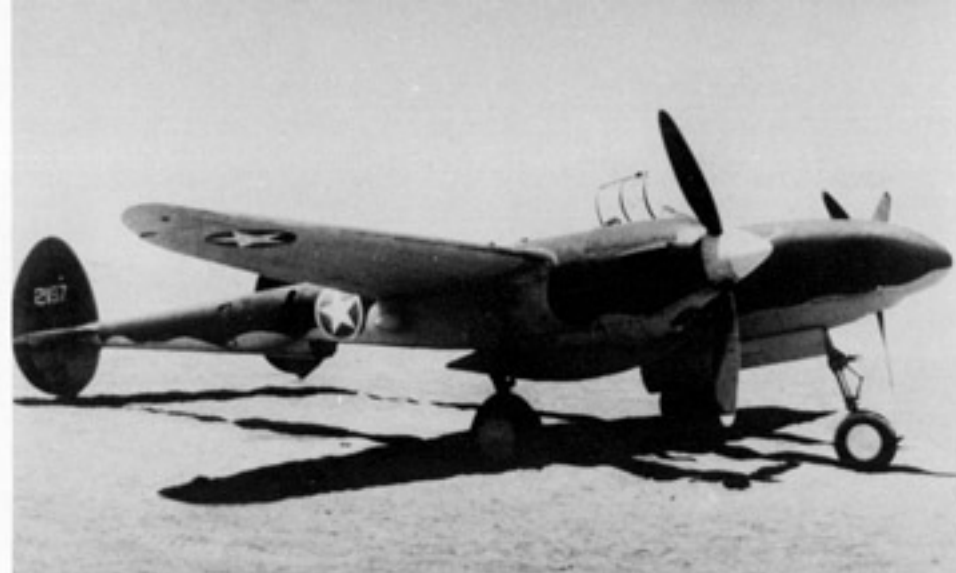
This F-4-1-LO Photo Lightning served in North Africa during January of 1943. The F-4-1-LO was a P-38E airframe with the guns replaced by a pair of K-17 vertical cameras in the gunbay. (AFM)
