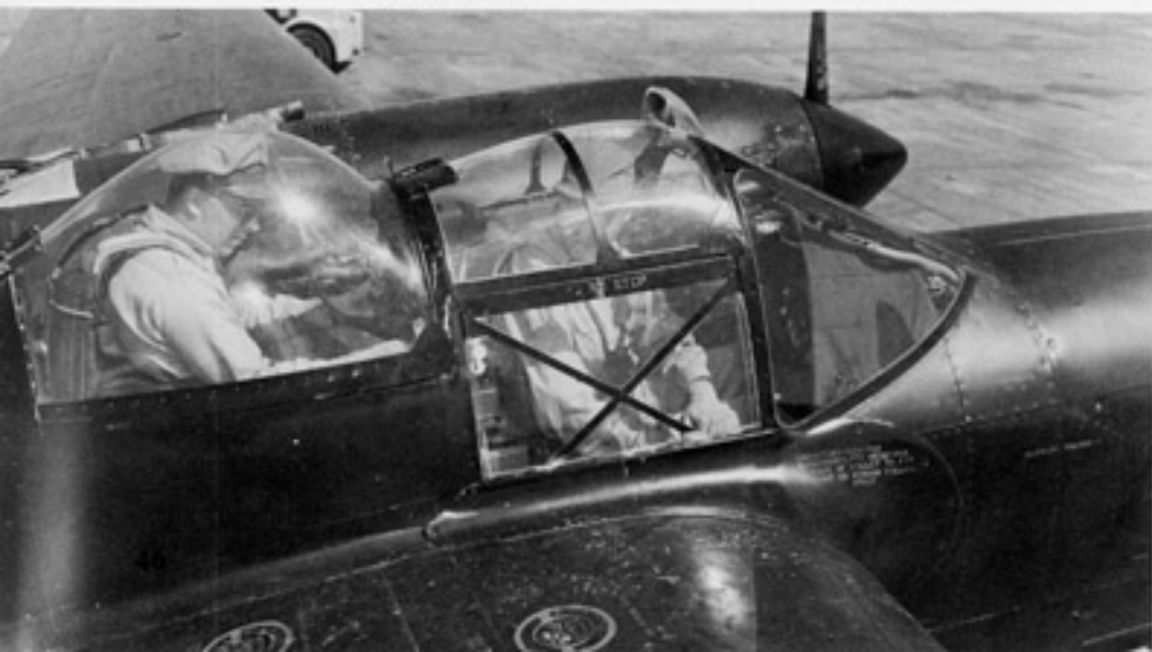
Night Lightning , a new production P-38M on the ramp at Lockheed's Dallas, Texas, facility. The AN/APS-4 AI radar pod was mounted under the nose with a modified P-38 drop tank pylon. The guns were all fitted with flash hiders to keep from blinding the pilot when they were fired at night. (Lockheed)
