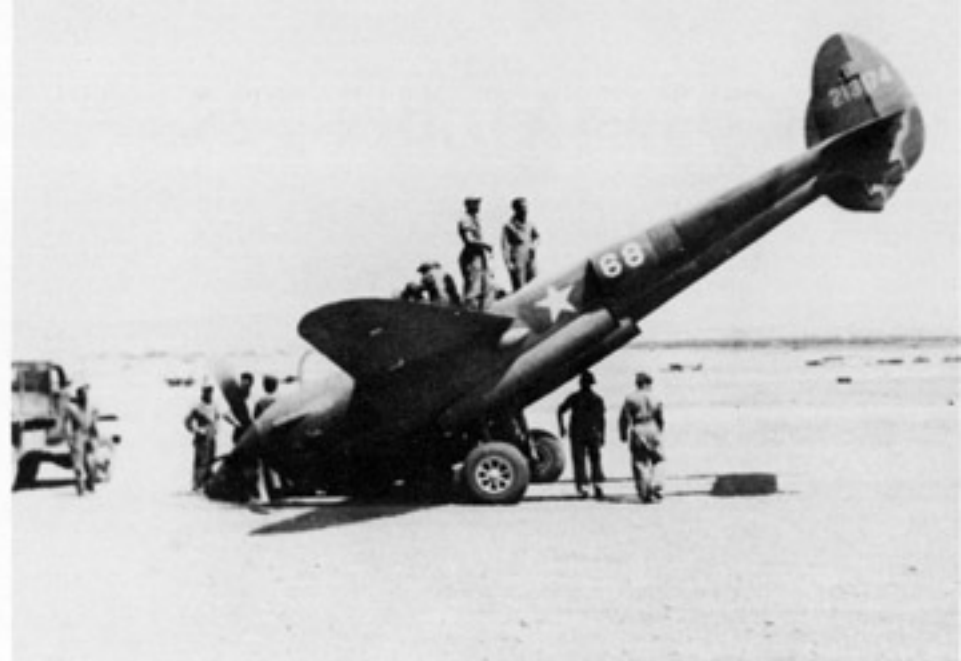
Nose wheel strut collapse was a common accident among P-38 units. This P-38G of the 82nd FG was based at Pelergma, Algeria. Although most North Africa based aircraft carried the Yellow surround insignia, this P-38 had an unbordered insignia.
