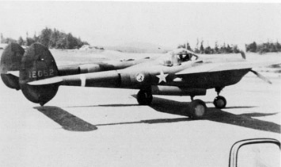
A P-38E of the 54th FS on the ramp at Vancouver, British Columbia while enroute to the Aleutian Islands during the Summer of 1942. The P-38Ds and Es of the 54th FS were the first Lightning fighters to see combat. The White band around the boom identifies this Lightning as a Flight Leader's aircraft. (SGT James Crow)
