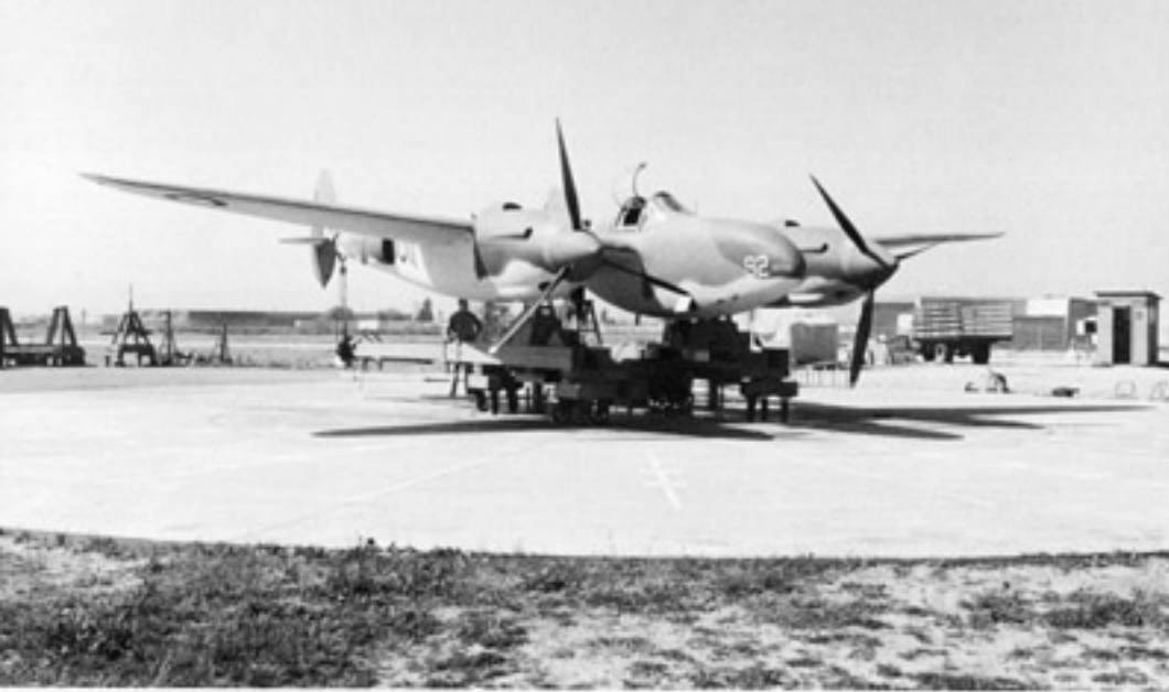
A P-322 Lightning sits on the compass test stand at the Lockheed Air Terminal, Burbank, to check for compass error. The Royal Air Force named the aircraft the Lightning and the USAAF adopted the name for the P-38. (Lockheed)
