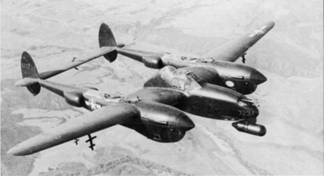
Lockheed built seventy-five P-38M Night Lightnings before the war ended; however, only four saw active service. These aircraft were assigned to the Occupation Force in Japan. The natural metal areas surrounding the superchargers was for heat reflection. (Lockheed)
