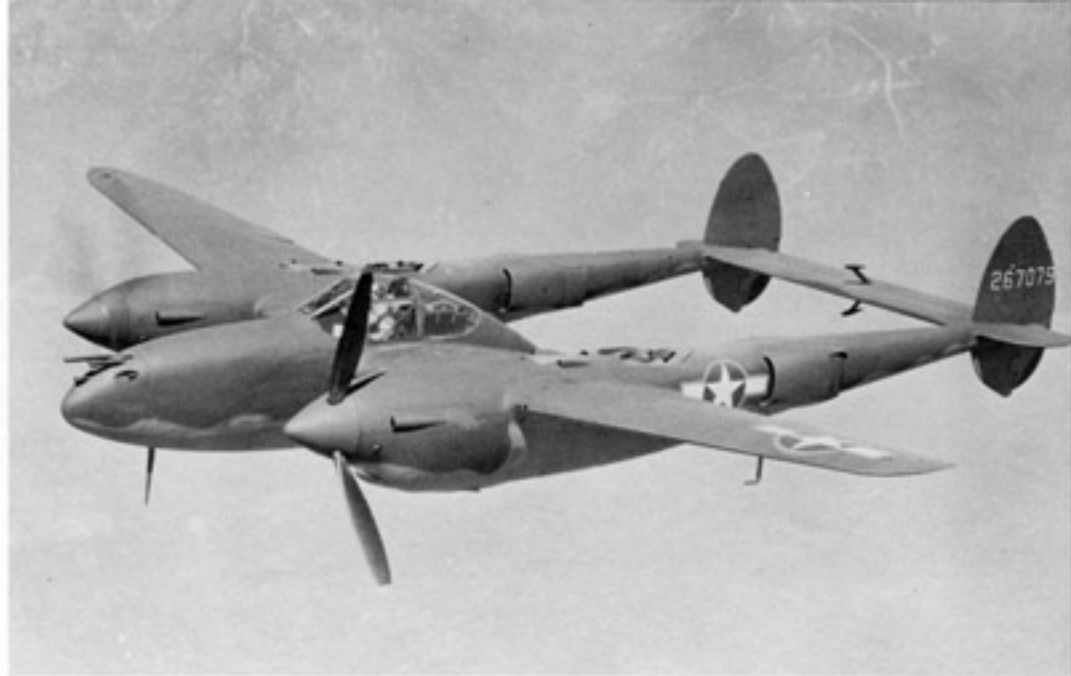
Lockheed pilot Jimmie Mattern conducts a test flight of a new production P-38H with one propeller feathered. The P-38H was powered by a 1,425 hp Allison engine instead of the 1,225 hp Allison used in the P-38G. (Lockheed)
