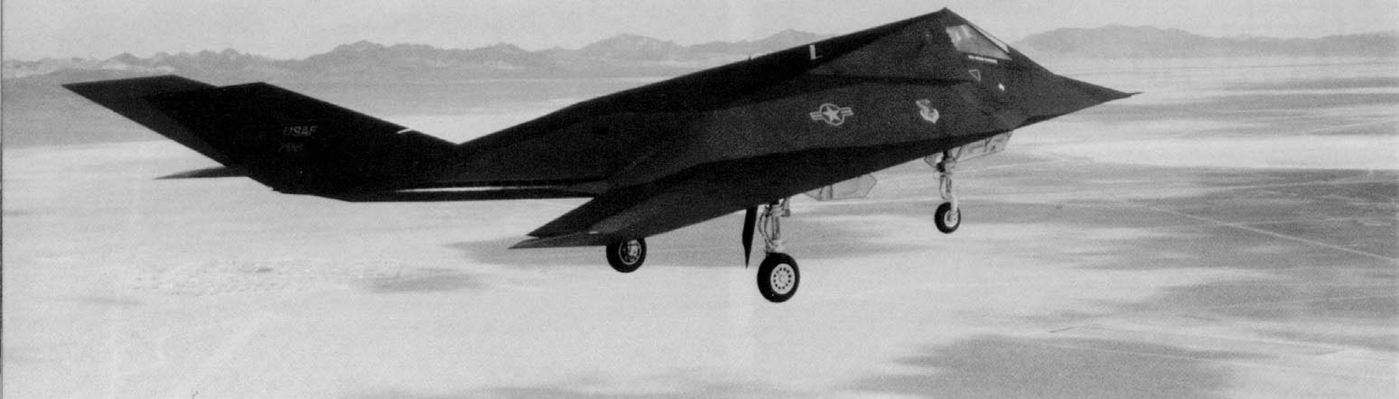
An F-117A (796) on final approach to Tonopah Test Range. For day flights the Stealth fighter normally keeps its retractable communications antennas deployed. (Eric Schulzinger)
