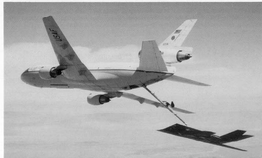
An F-117A takes on fuel from a KC-10 Extender tanker based out of March AFB, California. Only certain KC-10A and KC-135 tanker crews have been trained to work with the F-117A on night missions. (USAF)
