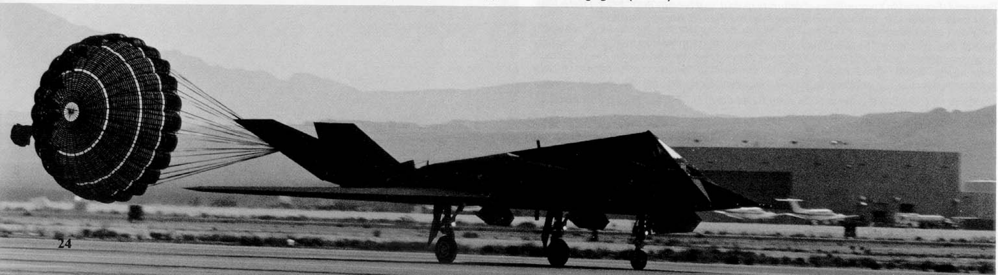
An F-117A (828) lands at Nellis Air Force Base, Nevada, during its first public press conference. The drag chute is normally used on F-117A landings and is Black. The bright spots on the landing gear legs are the approach and landing lights. (Author)
