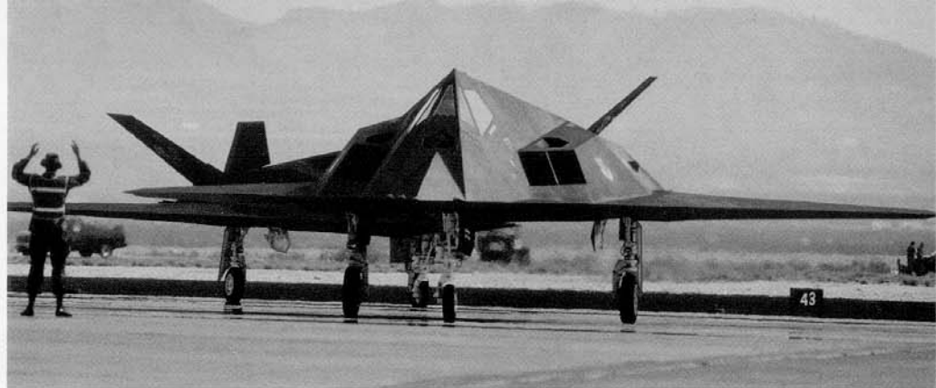
A ground crewman directs an F-117A into its parking spot on the ramp at Nellis Air Force Base during the aircraft's first public display. The small bulges on the fuselage sides are detachable radar reflectors. (Author)
