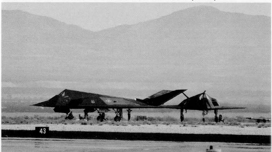
Two F-117As (828 and 790) taxi in to the ramp at Nellis Air Force Base. The aircraft in the foreground has the brake chute container doors at the base of the fin open. The interior of the container well and the insides of the doors are in Gloss White. (Author)
