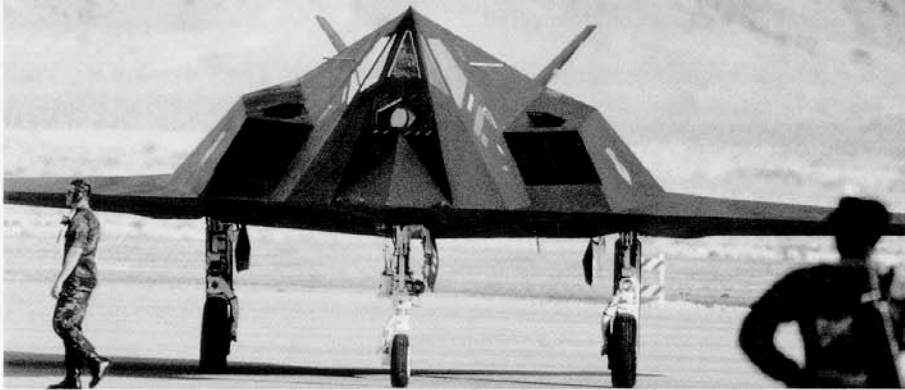
Ground crews perform post flight checks of the landing gear and install the gear locking pins in the Nellis Arm/Disarm area on F-117A 814. Once cleared, the aircraft would then taxi in to the ramp area. Visible are the twin retractable ILS antennas located just behind the cockpit. Additionally, the FLIR is in the view position. (Author)
