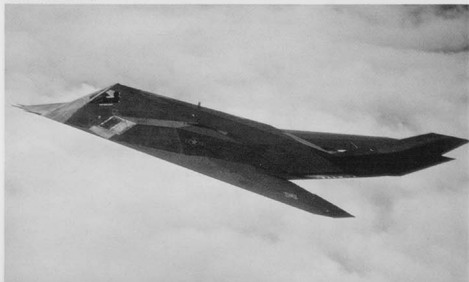
An F-117A of the 415th TFS, 37th TFW over the Atlantic Ocean enroute to Saudi Arabia on 19 August 1990. The aircraft did not carry the 37th TFW markings, TR tail code and TAC badge on the fin. For the ferry flight, all aircraft were equipped with removable rotating beacons. (Mike Dornheim).
