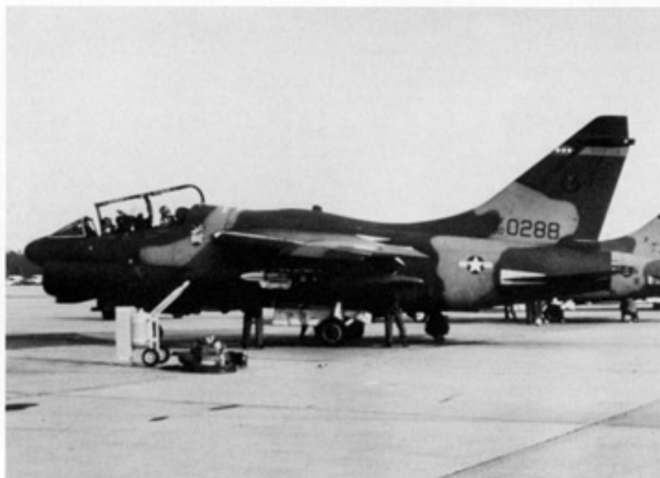
Ground crewmen remove the "Remove before flight" flags from an A-7K of the 149th Tactical Fighter Squadron, Virginia Air National Guard. 80-0288 was one of twelve new A-7Ks delivered during 1981. The A-7K had a built in Auxiliary Power Unit (APU) and did not need an external starter cart. (Paskowski via T.Love)
