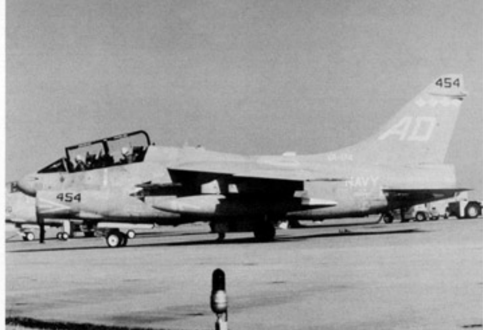
This TA-7C (BuNo 156747) of VA-174 carries the low-vis tactical Gray camouflage scheme. AD454 was attached to VA-174, the Atlantic Fleet RAG. All markings were in Light Gray including the Tomahawk on the underwing fuel tanks. The TA-7C was used as an advanced combat trainer and was fully combat capable. (Navy)
