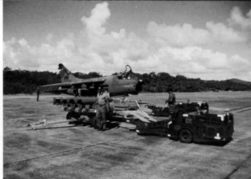
Armors from the 198th TFS use an MJ1 loader to move 500 pound Mk 82 free fall bombs to their A-7Ds, while other armors prepare the fusing wires on the A-7D-10-CV (71-0325) in the background. All Air National Guards units must stay proficient in both air-to-ground and air-to-air tactics. (Eric Cintron)
