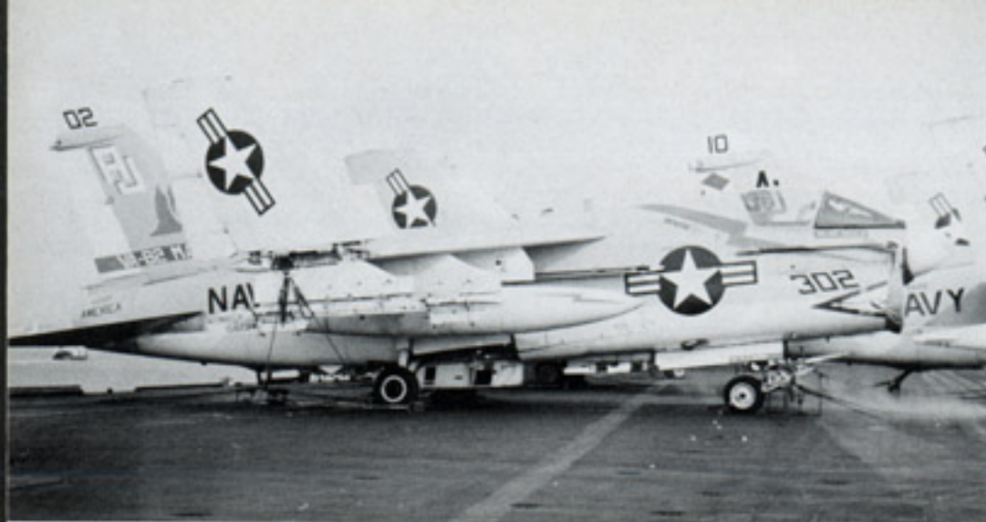
An A-7C (BuNo 156794) of VA-82 Marauders chocked and chained down aboard USS AMERICA (CV-66). VA-82 and VA-86 Sidewinders briefly operated the A-7C when their A-7Es experienced engine problems with the TF41 turbofan. All squadron markings are in Blue, the tail code is in White with a Blue outline. (Bob Sides via J. Sullivan)
