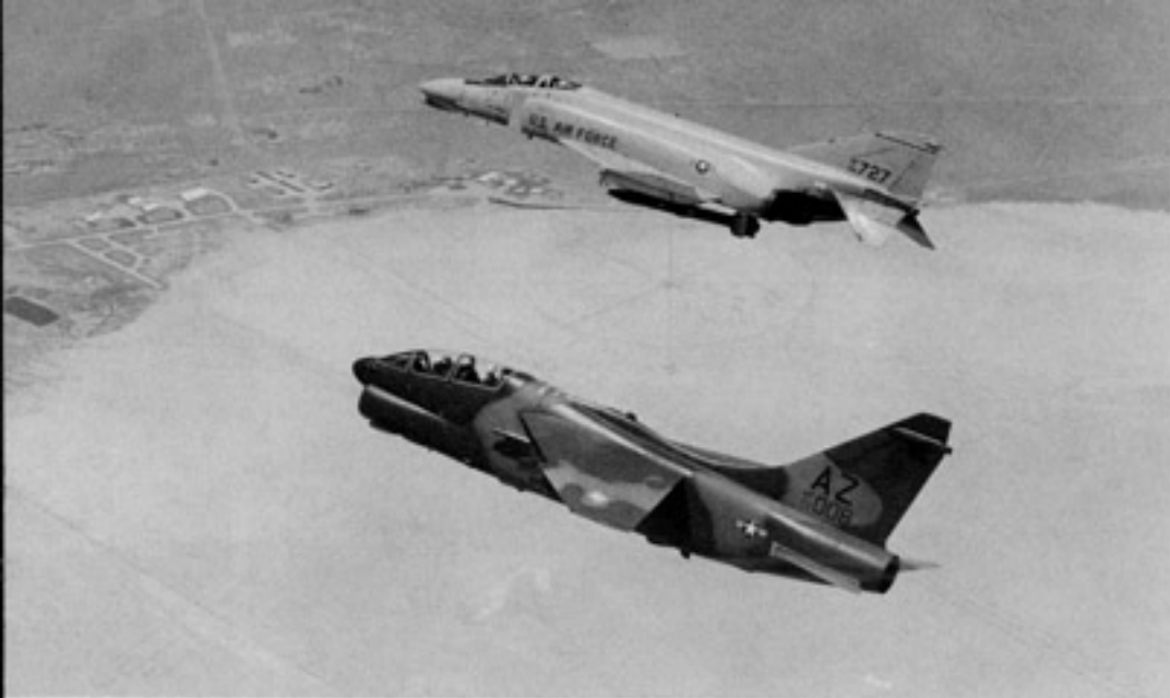
The prototype A-7K (73-1008) flies in formation with a USAF F-4C (64-0727) over Edwards AFB, California. The two aircraft had been conducting AIM-9 Sidewinder missile launches (the F-4 has a missile shaped supersonic target under its left wing). The A-7K was a fully combat capable crew trainer. (USAF)
