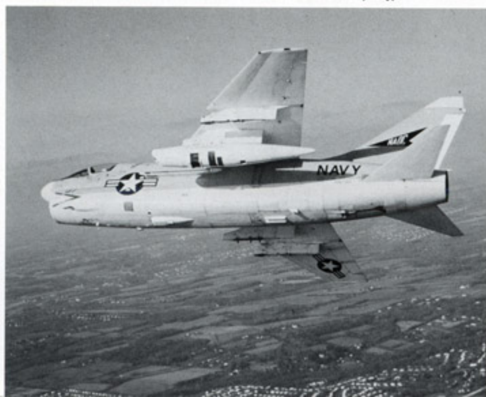
NA-7C (BuNo 156782) carries a Tactical Aerial Reconnaissance Pod (TARPS) during operational testing of the system. This TARPS was the Advanced Development Model (ADM) and contained four cameras and three infrared line scanners. Development work was stopped when it was decided to use the F-14A/TARPS combination instead of the A-7. (Navy)
