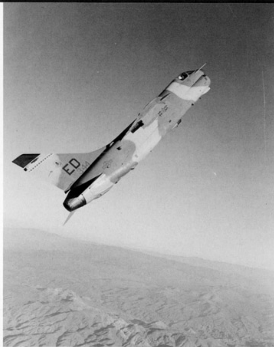
The number 1 YA-7F (71-0344) flies a high angle of attack (AOA) test flight over the El Paso Mountains near Edwards AFB California. The YA-7F has been flown to a top speed of Mach 1.2 the fastest of the A-7 series. (USAF)
