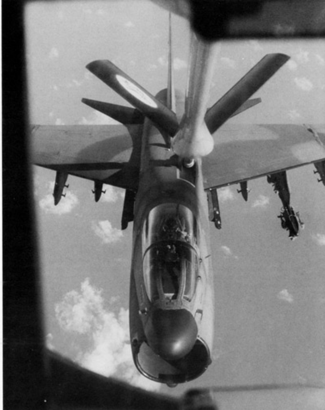
A New Hampshire ANG KC-135 refuels a A-7D of the 198th Tactical Fighter Squadron, Puerto Rico Air National Guard. In this system of aerial refueling the receiver aircraft flies into position behind and below the tanker and the boom operator flies the probe to the fuel receptacle. (Eric Cintron)
