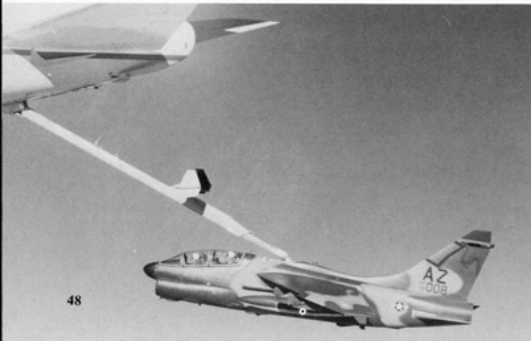
This A-7K (73-1008) takes on fuel from a McDonnell-Douglas KC-10 Extender over Edwards AFB, California. The pilot of the A-7K gets the aircraft into position and the boom operator flies the refueling boom into contact with the A-7K's universal fuel receptacle. (USAF)
