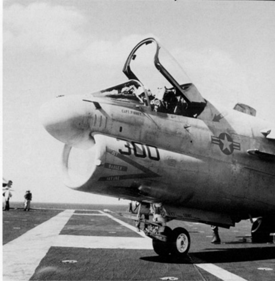
This A-7E of VA-97 aboard USS CARL VINSON (CVN-70) has been modified with ECM button antennas on either side of the air intake. The aircraft side number 300 identifies it as being the squadron's CAG aircraft. (Navy)
