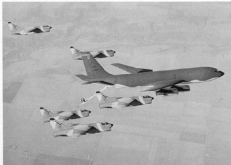
A-7Ds of the Iowa Air National Guard (174th TFS) line up and wait their turn to take on fuel from a Kansas ANG KC-135E (56-3604). The high speed aerial boom refueling technique takes much longer to fuel aircraft than the drogue system since the tanker can only refuel one aircraft at a time. (Iowa Air National Guard)
