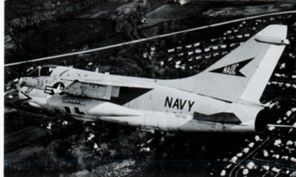
This NA-7C (BuNo 156782) carries a TARPS pod on the outboard wing pylon. The NA-7C served as a test bed for the TARPS program and for a while the A-7 TARPS combination was considered as a possible replacement for the RA-5C. (Navy)
