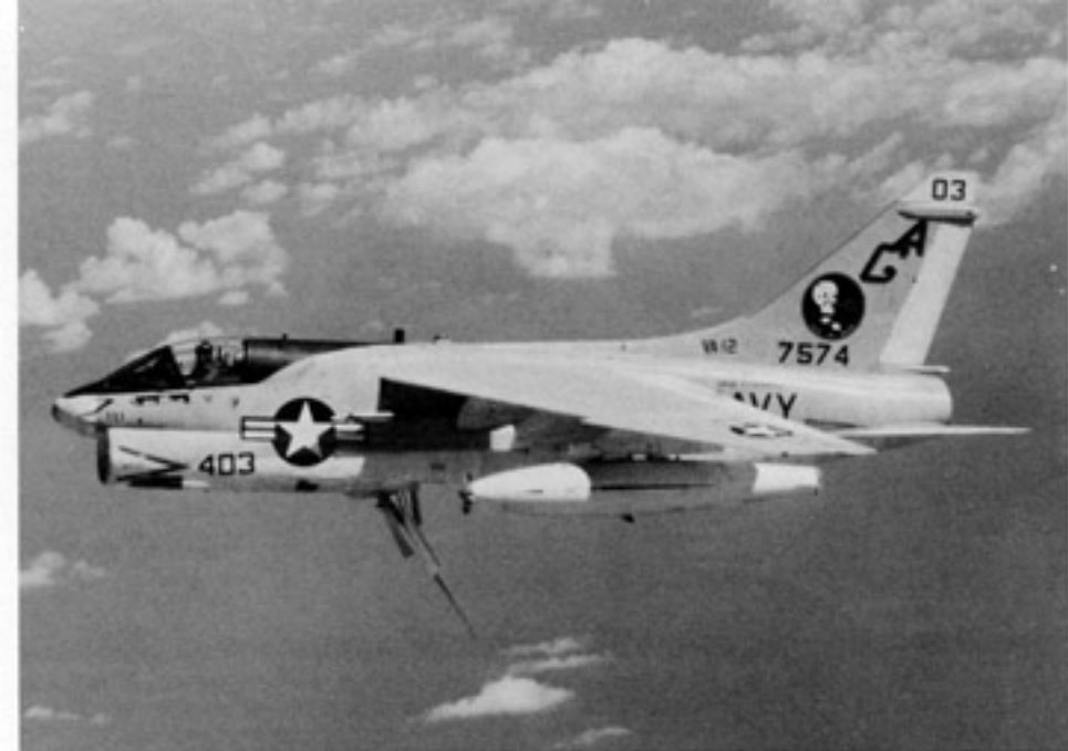
This A-7E (BuNo 157574) of VA-12 Clinchers has the air brake deployed as it pulls into formation during June of 1978. The Corsair has a buddy refueling store on the number one pylon. The tank carries the legend "VA-12 Super Tanker" on the side in Red. (Navy)
