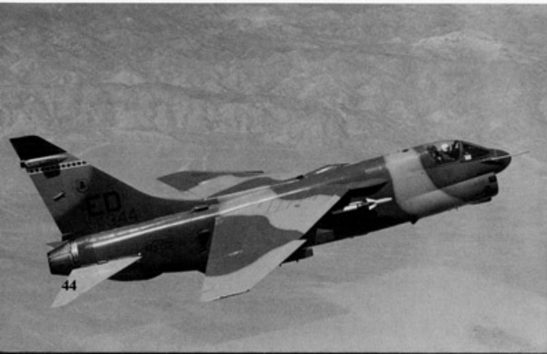
The number 1 YA-7F (71-0344) flies a high angle of attack (AOA) test flight over the El Paso Mountains near Edwards AFB California. The YA-7F has been flown to a top speed of Mach 1.2 the fastest of the A-7 series. (USAF)
