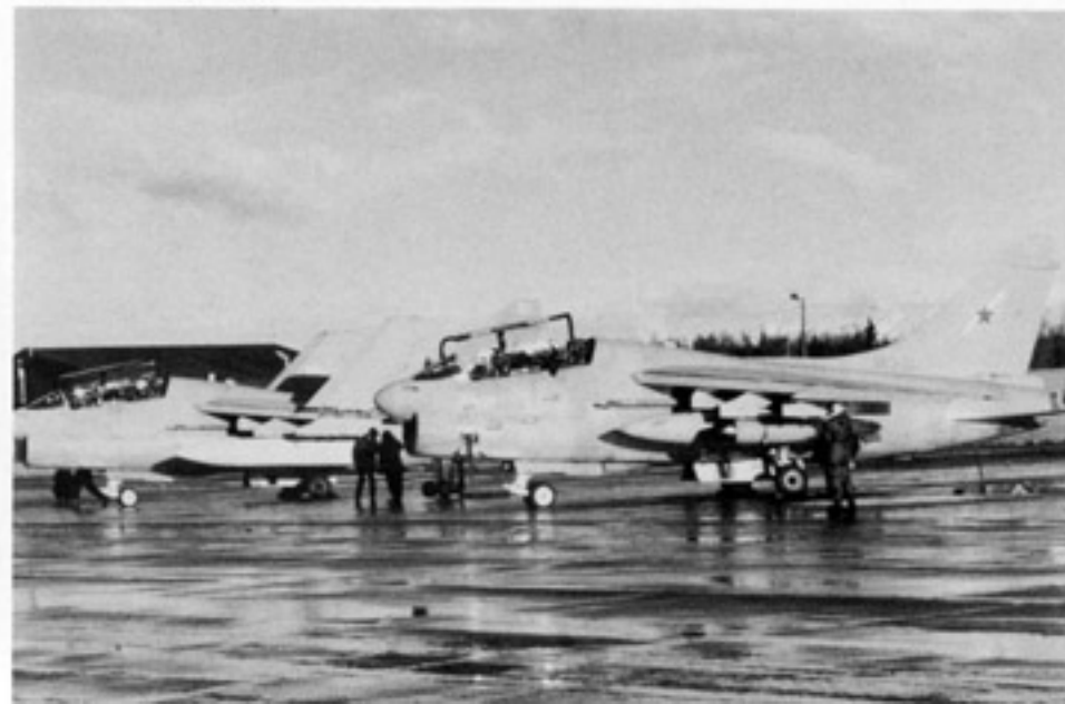
Two EA-7Ls prepare to depart on a training mission during 1987. EA-7Ls are operated by VAQ-34 as simulators for threats to not only aircraft but to ships as well. The emitter pods simulate Soviet aircraft and missile threats. The GD tail code has been replaced by a Soviet style Red star. (Navy)
