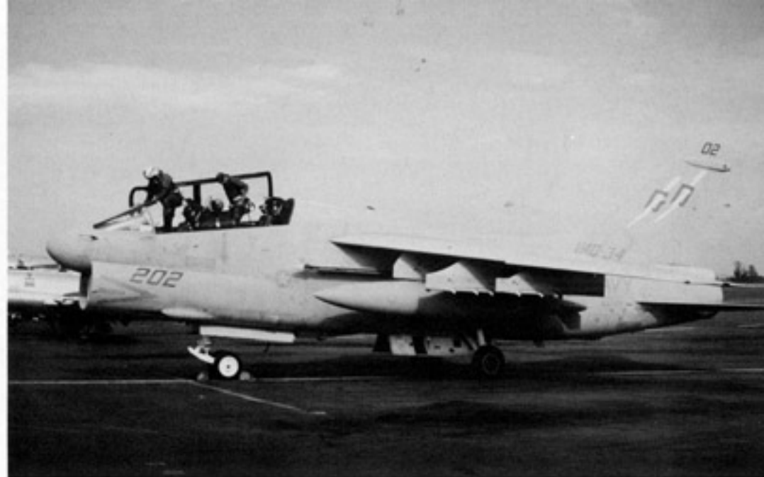
The crew of this EA-7L man their aircraft for another mission. The EA-7L is used by VAQ-34 as an electronics warfare training aircraft. The aircraft is overall Gray with White lighting flashes through the Dark Gray GD tail code. (Kirkup via T. Love)
