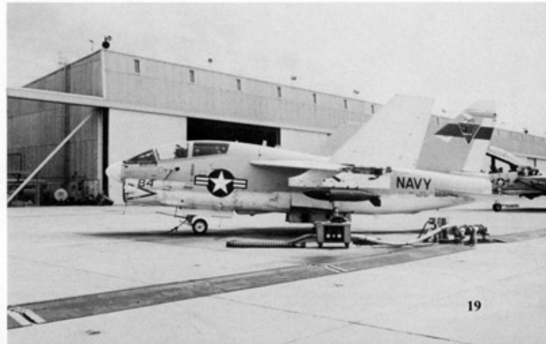
This TA-7C (BuNo 156787) is fitted with a Radar Simulating Set (RSS/JEEP) pod on the number one wing pylon. Aircraft number 84 was attached to the Pacific Missile Test Center, NAS Point Mugu, California. The PMTC emblem is carried over a Blue stripe on the fin. (Navy)
