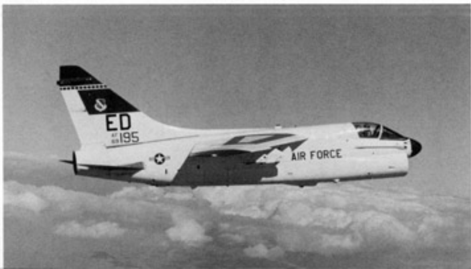
An A-7D-3-CV (69-6195) of the 6512th Test Group flies over Edwards AFB, CA during 1988. This is an early A-7D with the Navy style refueling probe. The aircraft at Edwards are used as test aircraft and chase planes and are painted overall White with Red recognition panels. (USAF)
