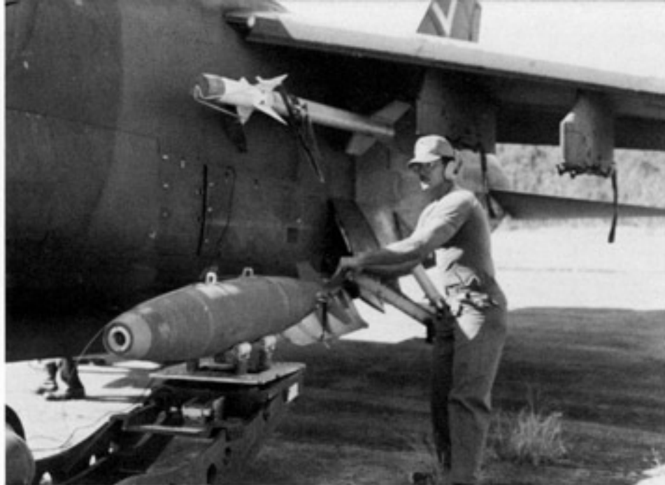
An armorer guides a 500 pound Mk 82 GP low drag fragmentation bomb onto the number 3 wing pylon of this A-7D. The A-7D was capable of carry up to 15,000 pounds of external ordnance on six wing and two fuselage stations. (Eric Clintron)
