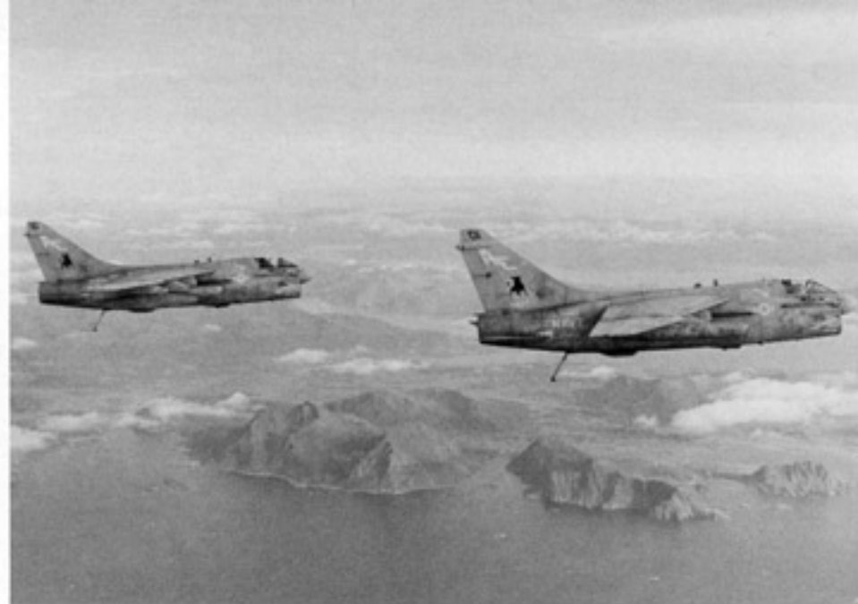
A pair of A-7Es of VA-37 Bulls on patrol off Norway during USS FORRESTAL's (CV-59) North Atlantic deployment in 1990. Both aircraft are carrying Forward Looking Infrared (FLIR) pods on the inboard wing pylons. (Navy)
