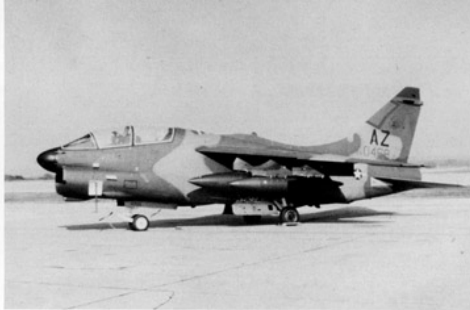
The 162nd Tactical Fighter Training Group (tail code AZ) received the majority of A-7Ks built, including 79-0468. The first A-7K was a rebuilt A-7D, while the other thirty were all new built aircraft. (Terry Love)
