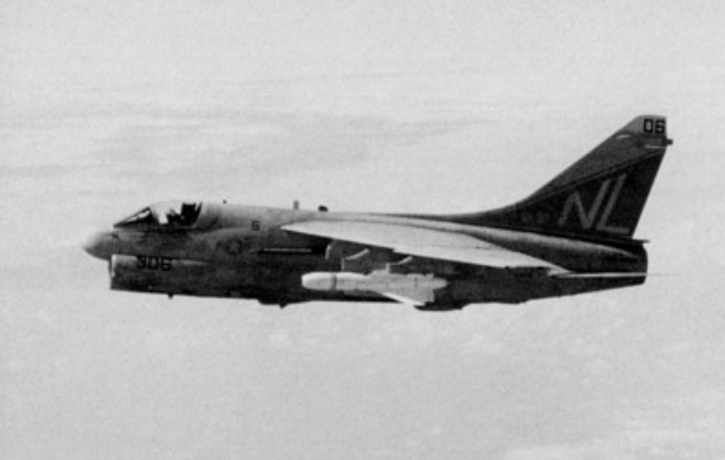
An A-7E Corsair II of VA-97 Warhawks carries an AGM-62 Walleye TV guided glide bomb on the second wing pylon. The Walleye was first used in Vietnam and has proven to be a highly accurate weapon. Walleyes were used in the Persian Gulf to destroy various hardened targets. With data link the Walleye can be launched from one aircraft and then guided by another to its target. (Navy)
