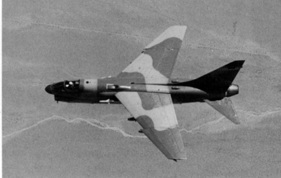
The YA-7F has wing leading edge extensions (LEX) and two upper fuselage air scoops for cooling air. During this test, two AIM-9 Sidewinder air-to-air missiles were carried on the fuselage stations. The fairing over the Pratt and Whitney F100 engine afterburner was removed during flight tests. (USAF)
