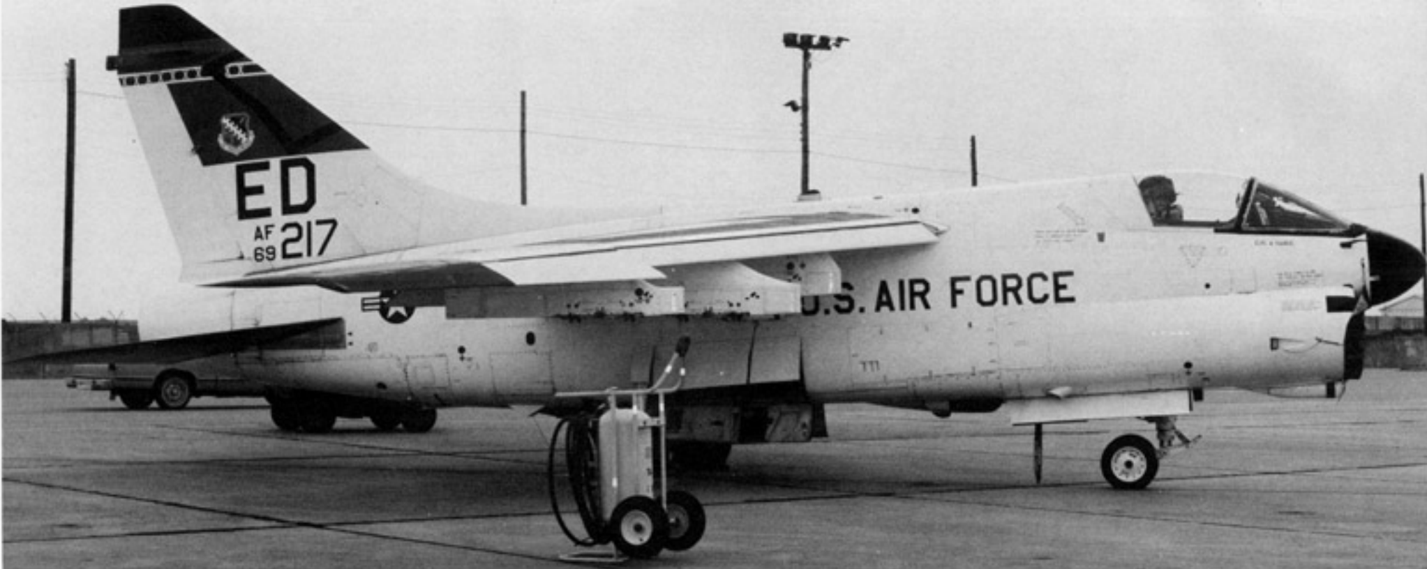
This early production A-7D (69-6217) of the 6512th Test Group on the ramp at Edwards Air Force Base has been modified with the Navy style refueling probe being deleted. (USAF Via Rod Bankston)
