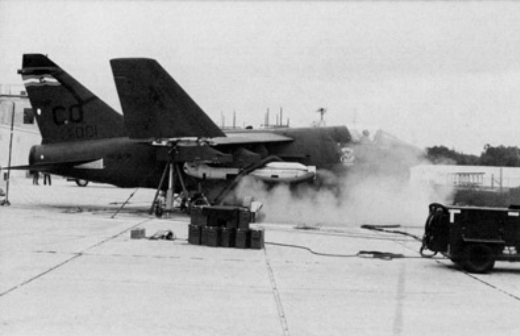
This A-7D-8CV (70-1001) was used at Eglin AFB, FL, to test the GPU-5/A 30MM gun pod. The A-7D was from the 120th TFS Colorado Air National Guard. For the firing test the A-7 was mounted on jacks and securely tied down. The GPU-5/A weighs 1,865 pounds (loaded), is 14 feet 2 inches long and has a muzzle velocity of 3,200 feet per second. (USAF via Rod Bankston)
