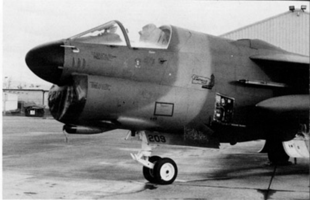
The housing under the nose of this A-7D-5 (69-6209) contains a Pave Penny laser seeker system and the large Black radome houses the AN/APQ-126 forward looking radar. This aircraft was assigned to the 198th TFS Puerto Rico Air National Guard (PRANG) and carried a Green kill marking on the fuselage gained during a deployment to Honduras for exercises. The "kill" was with a simulated Sidewinder AAM. (Eric Cintron)
