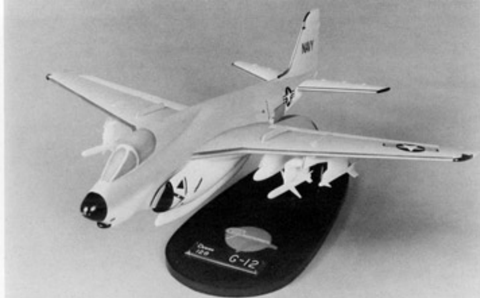
The Grumman G-12 was a competitor to the A-7 for the VA (L) contract. The aircraft was to feature a single seat cockpit and folding horizontal stabilizer. A mock-up was built before the project was cancelled. (Grumman)
