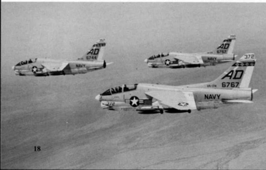
A flight of TA-7Cs on a weapons training mission over the western U.S. The aircraft are armed with Mk 82 bombs on Multiple Ejector Racks (MERs). All are from VA-174, the East Coast Replacement Air Group (RAG). The TA-7C has a braking parachute housing at base of vertical stabilizer. The tail markings are Yellow diamonds on a Black Stripe. (LTV)
