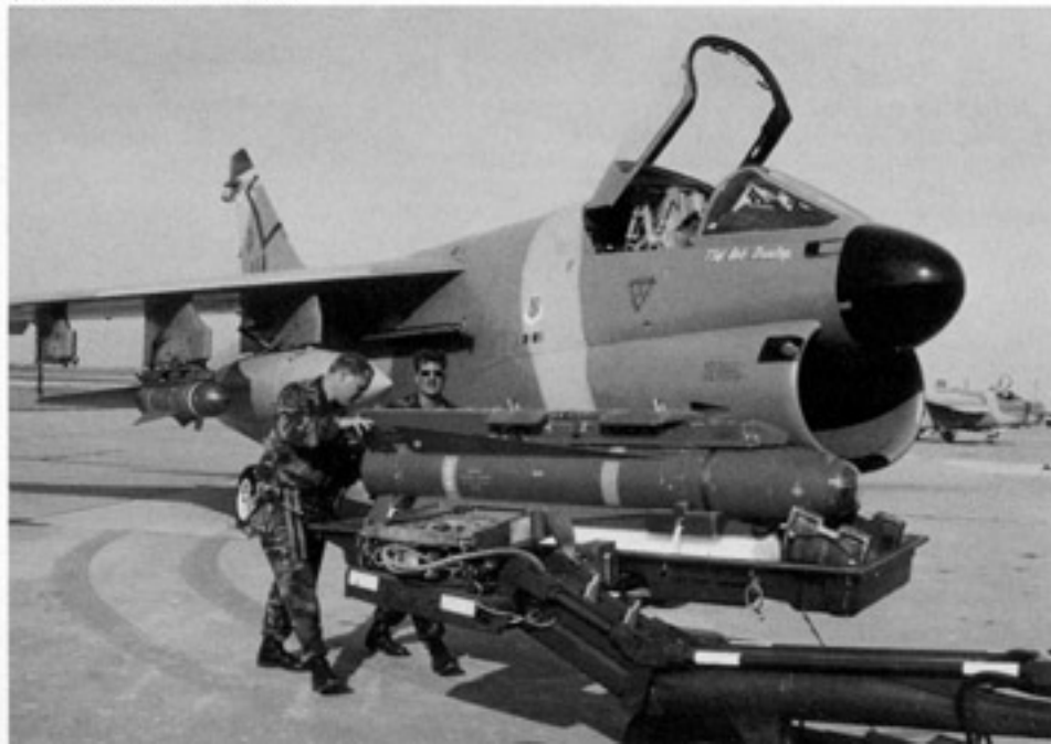
AGM-65 Maverick anti-tank missiles are loaded onto a 174th TFS, A-7D. The AGM-65 is an air-to-ground missile that can be fitted with either a TV or infrared seeker. The Maverick proved itself in the Persian Gulf, knocking out hundreds of Iraqi tanks during the short ground war. (Iowa Air National Guard)
