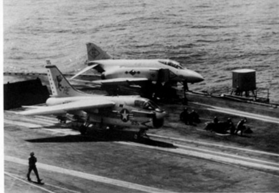
An A-7B of VA-15 Vallions prepares to launch from the number 2 catapult aboard USS INDEPENDENCE (CV-62) while a McDonnell-Douglas F-4J Phantom II of VF-102 Diamondbacks is positioned on the number 1 catapult. AE305 carries a Battle E ribbon award for combat readiness above the fuselage national insignia. (Navy)
