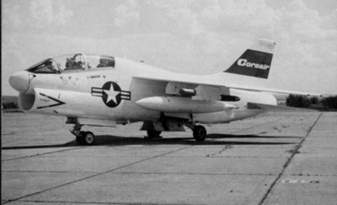
The first production A-7E (BuNo 156801) was converted into a two seat Corsair II. It was initially designated as the YA-7H, then changed to YA-7E then finally to TA-7C. The aircraft was loaned to Martin-Marietta for tests of the Pathfinder navigation system ( installed on the number 2 wing pylon). (Martin-Marietta)
