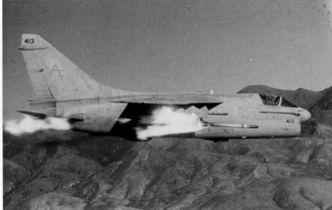
An A-7E Corsair II of VA-204 River Rattlers, flown by LCDR Ed "Boris" Kary, fires a five inch Zuni air-to-ground rocket at a target at NAS Fallon, during May of 1990. The Zuni is normally used against surface targets, however, on at least one occasion during Vietnam, Zunis were used to shoot down a MiG-17. (LT Kimo Moak)
