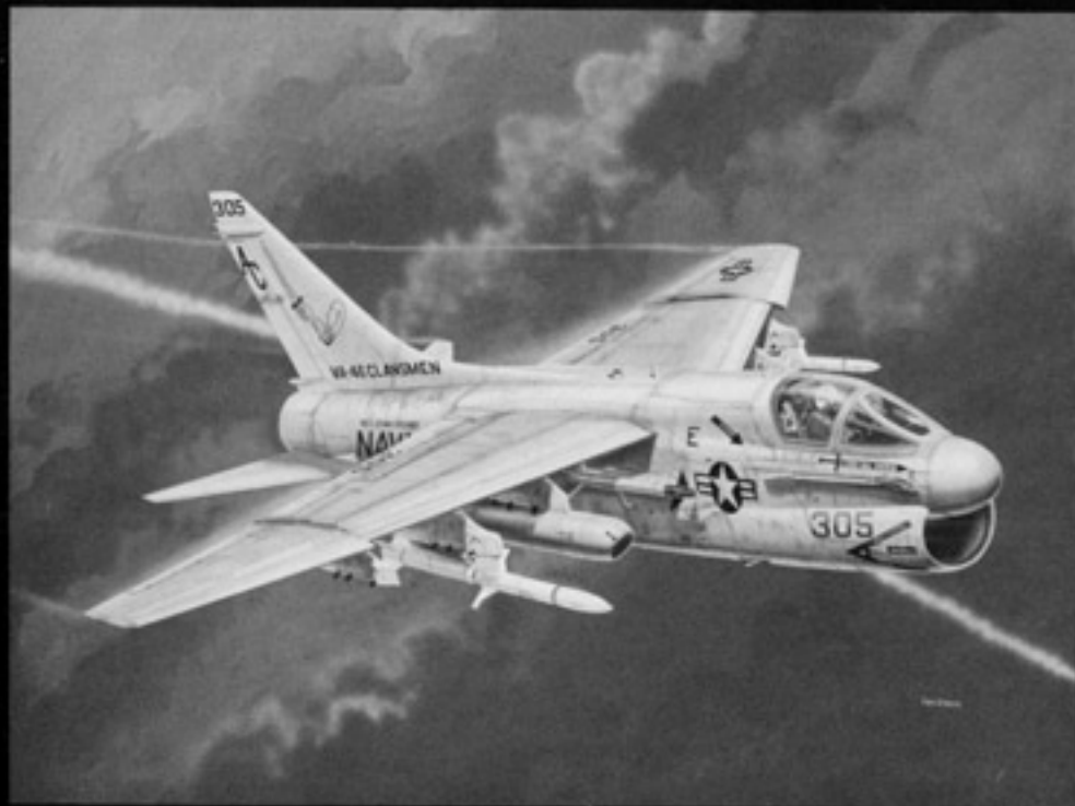
An A-7E Corsair II of VA-46 Clansmen off the USS JOHN F. KENNEDY flies an anti-radar mission over Kuwait. The A-7E was armed with HARM anti-radiation missiles, AIM-9 Sidewinders and carried a FLIR pod on the inboard wing pylon.
