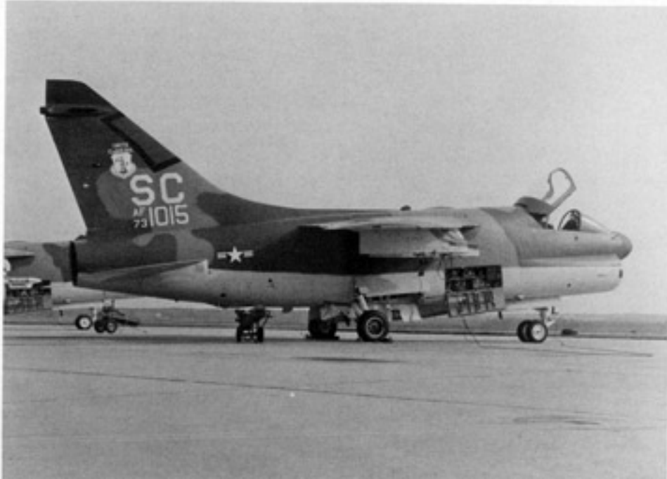
This A-7D-15CV (73-1015) on the ramp at McEntire Air National Guard Base, S.C. carries the ANG badge on the fin and the state name in White. The right avionics bay is open and a radio test was being conducted. All 157th TFS aircraft carried an SC tail code and the aircraft was camouflaged in a two tone Green and Tan over Light Gray scheme. The Black painted outline on the vertical fin is the VHF radio aerial. (Jim Sullivan)
