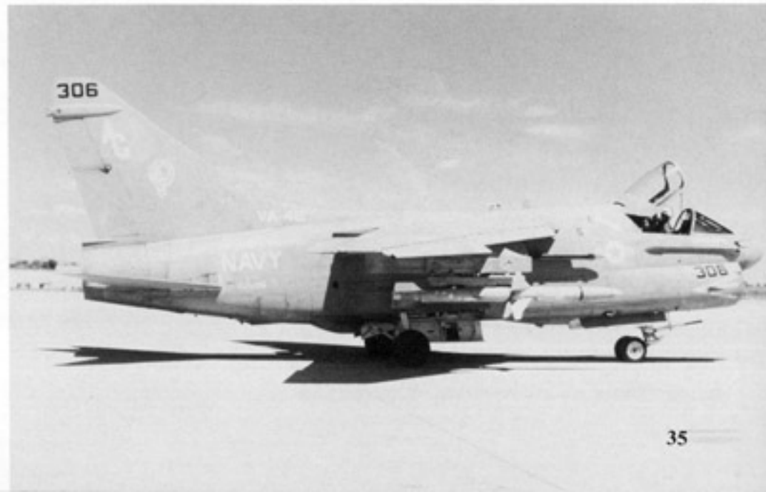
This A-7E Corsair II (BuNo 159285) of VA-46 Clansmen on the flight line at NAS Fallon, Nevada, is armed with an AGM-45A Shrike anti-radiation missile on the outboard wing pylon. The aircraft was camouflaged in overall Dark Gull Gray with Black numbers. (Navy)
