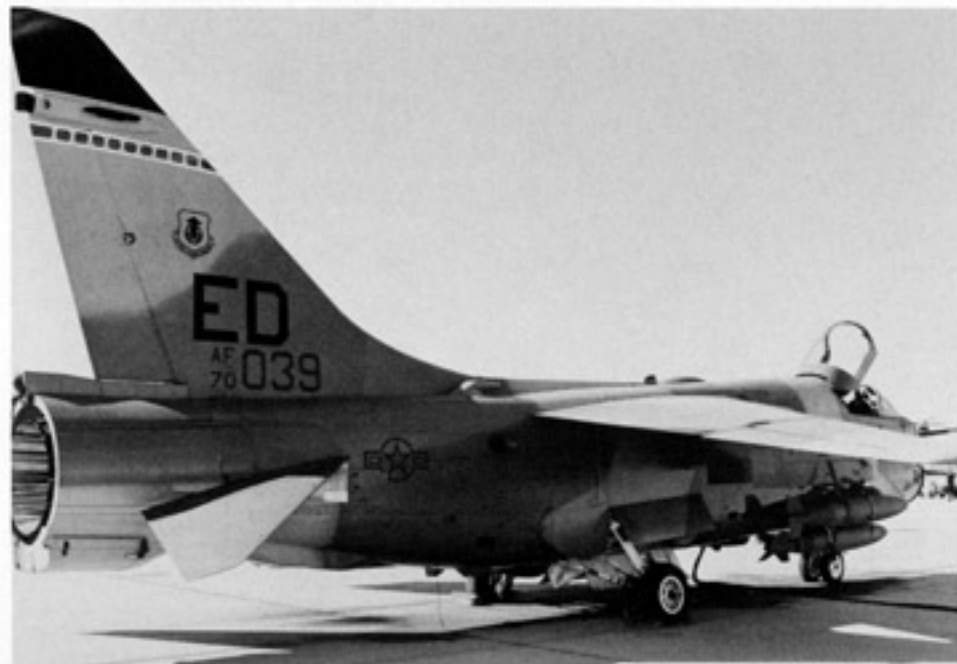
The spin recovery parachute system was housed in the fairing that extended from the base of the rudder back along the tail cone. The parachute was stored in the lower section and was attached by a steel cable to the upper tail section at the base of the vertical fin. The parachute was deployed during a test in July of 1990. (USAF)
