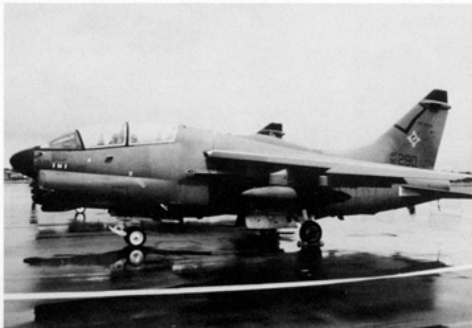
An A-7K (80-0290) of the 188th Tactical Fighter Squadron, New Mexico Air National Guard parked on a rain soaked ramp. A pilot's personal equipment pod is on the number two wing pylon. The A-7K carries no tail code; only the Virginia and New Mexico Air National Guard operate aircraft without tail codes. (Terry Love)
