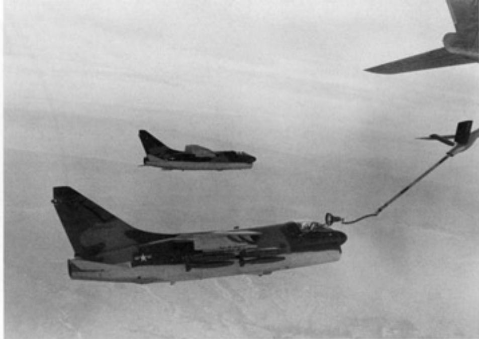
The first twenty-six A-7Ds were produced with the probe and drogue aerial refueling system. For flight tests it was necessary for the tankers to use the drogue system adapter for the flying boom. These two A-7Ds are on a practice bombing mission out of Edwards AFB during 1969. (USAF)
