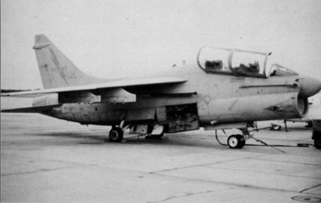
A TA-7C (BuNo 156765) on the ramp with its right avionics bay open. The TA-7C was serving with the Strike Warfare Center at NAS Fallon, Nevada. The TA-7C was a former A-7C and previously served with VA-122 until it was converted to the two seat configuration. (Terry Love)
