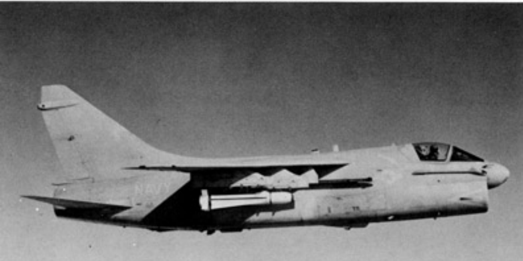
This A-7E (BuNo 156883) is armed with an AGM-65F Maverick infrared guided air-to-surface missile. The A-7E was bailed (loaned) to Hughes Aircraft, developer of the Maverick, for tests of the missile system. The Maverick is a fire and forget type of missile and it can be used day, night and under any weather conditions. (Hughes Aircraft)
