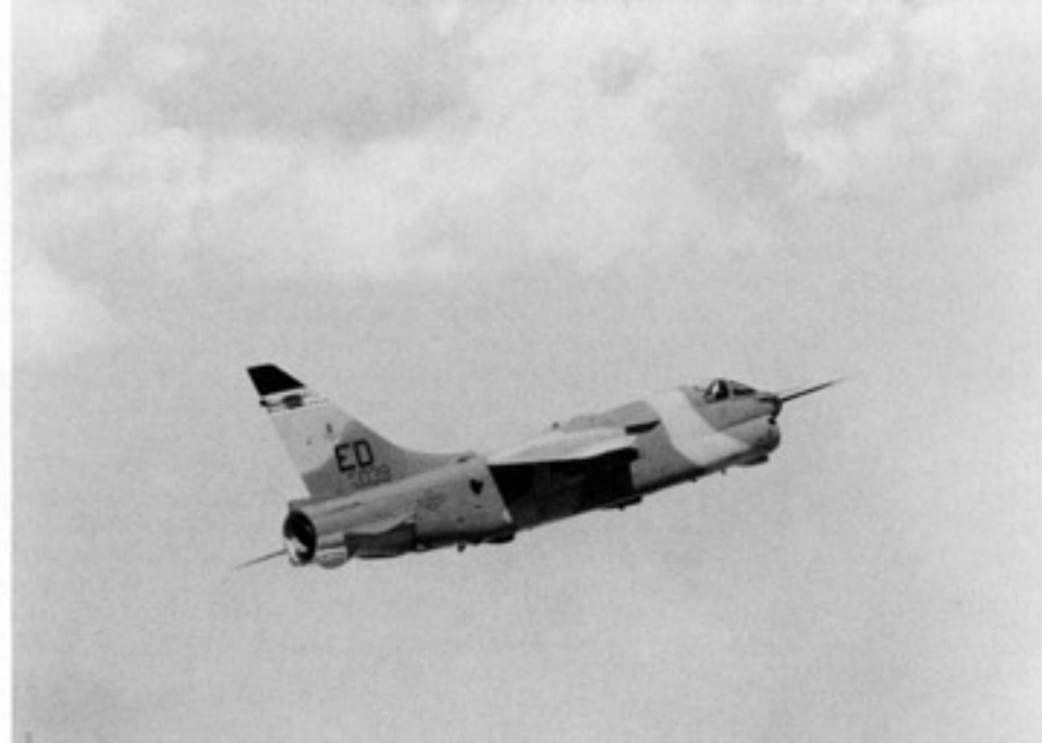
The second YA-7F prototype (70-1039) was fitted with a spin recovery parachute system mounted in a housing below the rudder. The second YA-7F prototype was a rebuilt A-7D that had been previously assigned to the 125th TFS, Oklahoma Air National Guard. After all flight tests were completed the Number 2 YA-7F was given to the Heritage Museum, Hill AFB, Utah. (USAF)
