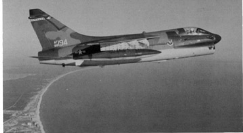
This A-7D (69-6194) flies over the Gulf of Mexico off Eglin AFB Florida. The aircraft was on a test flight to fire a YAQM-127A Supersonic Low Altitude Target (SLAT) missile. The Navy aerial refueling probe identifies this A-7D as one of the first production block. (USAF via Rod Bankston)
