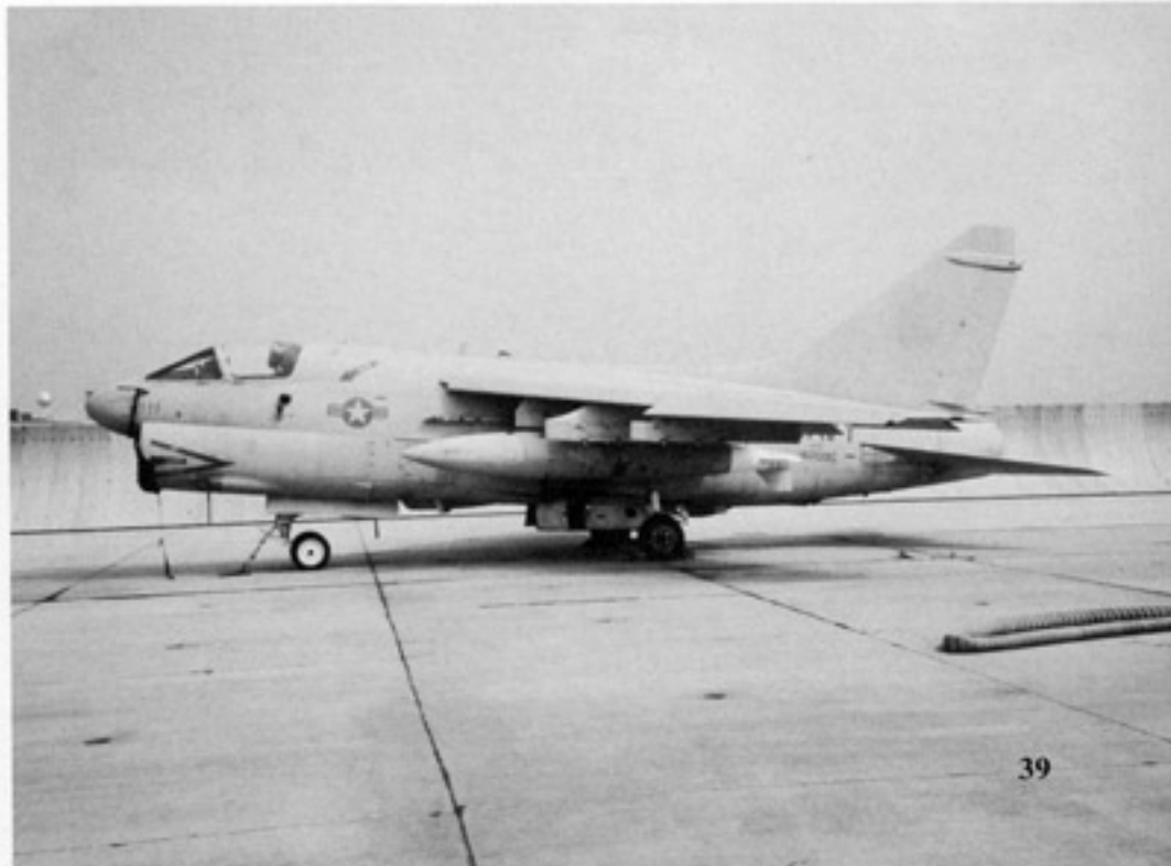
An A-7E on the ramp at the Naval Aviation Depot (NADEP) NAS Jacksonville, Fl., during September of 1991. The former squadron markings (VAQ-34) are completely painted out and all that remains are the service, rescue and warning markings, along with the national insignia. (A. Adcock IV)
