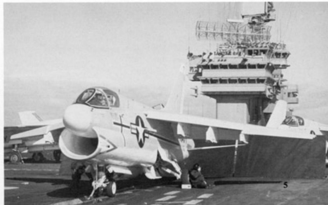
A-7 Number 7 was one of the four preproduction aircraft and was used for carrier suitability trials aboard the USS AMERICA (CV-66). The nose catapult bar is in the catapult shuttle indicating that the aircraft is ready for launch. The stripes on the fuselage are photographic reference markings. (U.S. Navy via Jim Sullivan)
