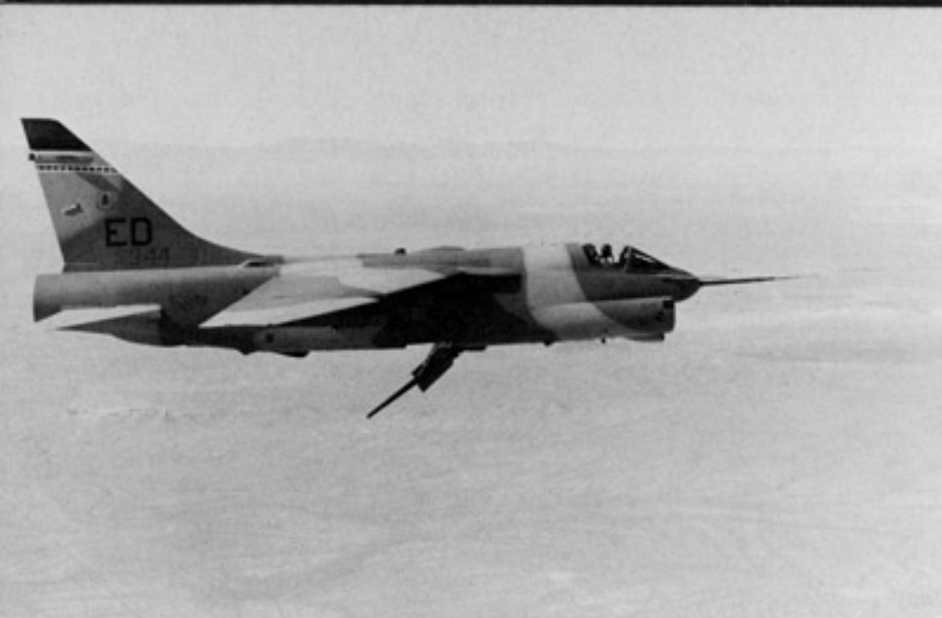
The first prototype YA-7F deploys the under fuselage speed brake during a test flight. The speed brake has an area of 25 square feet and is used to slow the aircraft for tactical maneuvering. During this flight test, YA-7F angle of attack and stall characteristics were investigated. (USAF)
