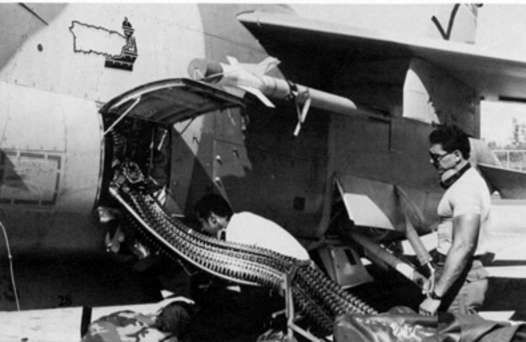
The armament panel on this A-7D indicates that 20mm ammunition was to be loaded. A loader is filling the ammunition drum with High Explosive (HE) cannon rounds. An AIM-9 Sidewinder air-to-air missile is already loaded on the fuselage station. (Eric Cintron)
