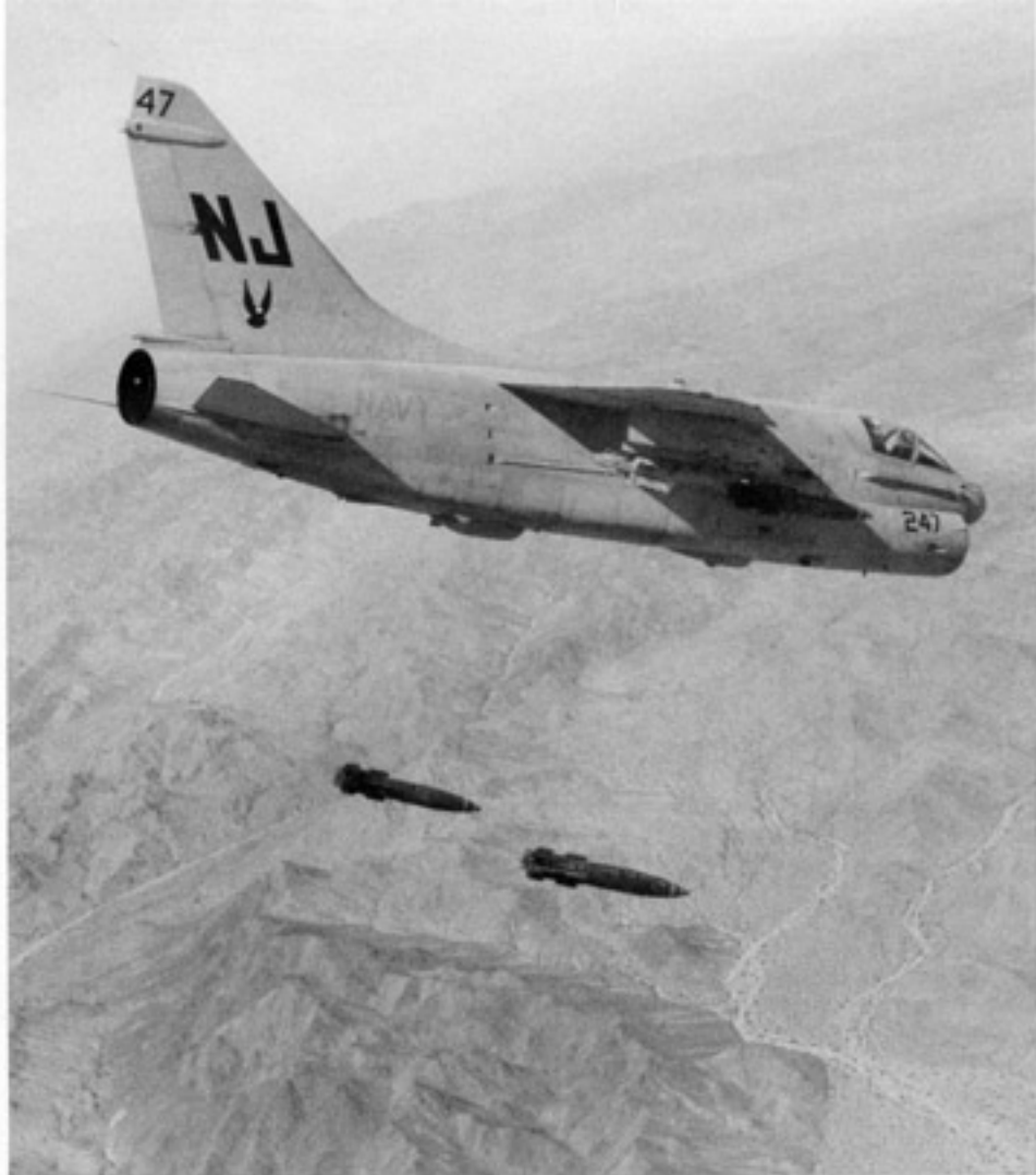
An A-7E of VA-122 Flying Eagles drops two Mk 82 Snakeye 500 pound retarded free fall bombs on the bombing range at the China Lake Naval Weapons Center, California. VA-122 operated as the Pacific Coast Replacement Air Group (RAG) training new A-7 aircrews for operational squadrons. (Navy)
