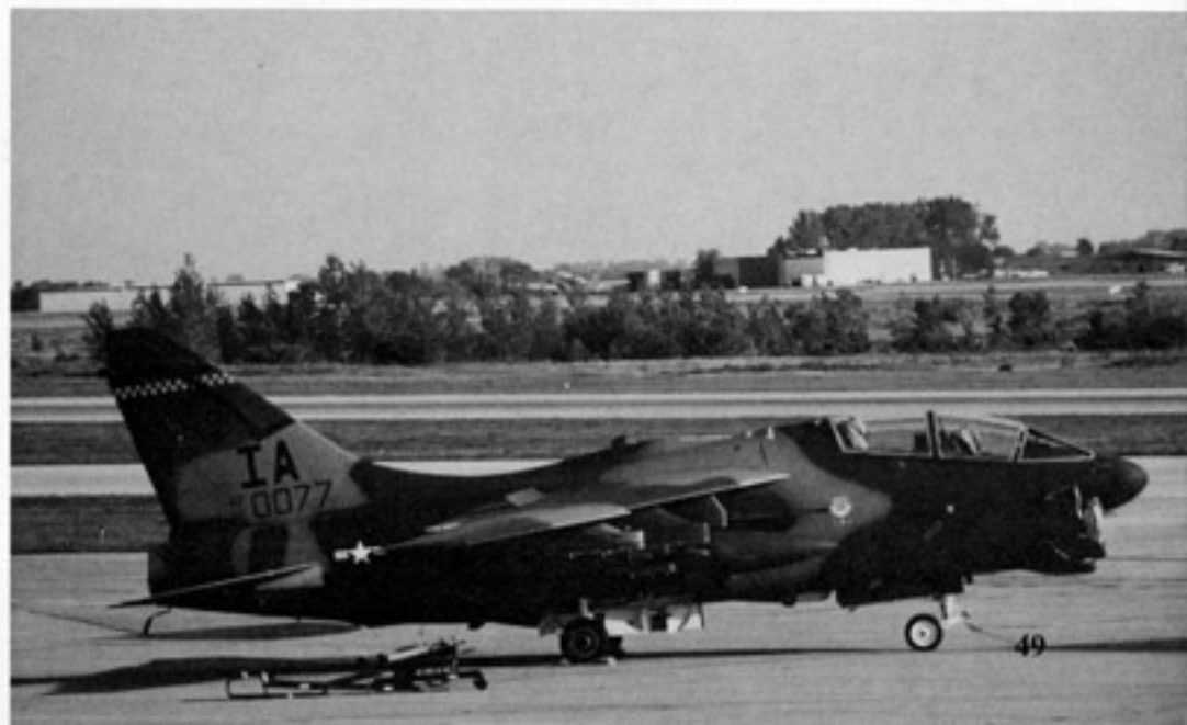
The long side opening canopy is a recognition feature of both the TA-7C and A-7K. This A-7K (81-0077) was assigned to the 124th Tactical Fighter Squadron, Iowa Air National Guard. The aircraft was finished in a two tone Green and Tan wraparound camouflage scheme. (Terry Love)
