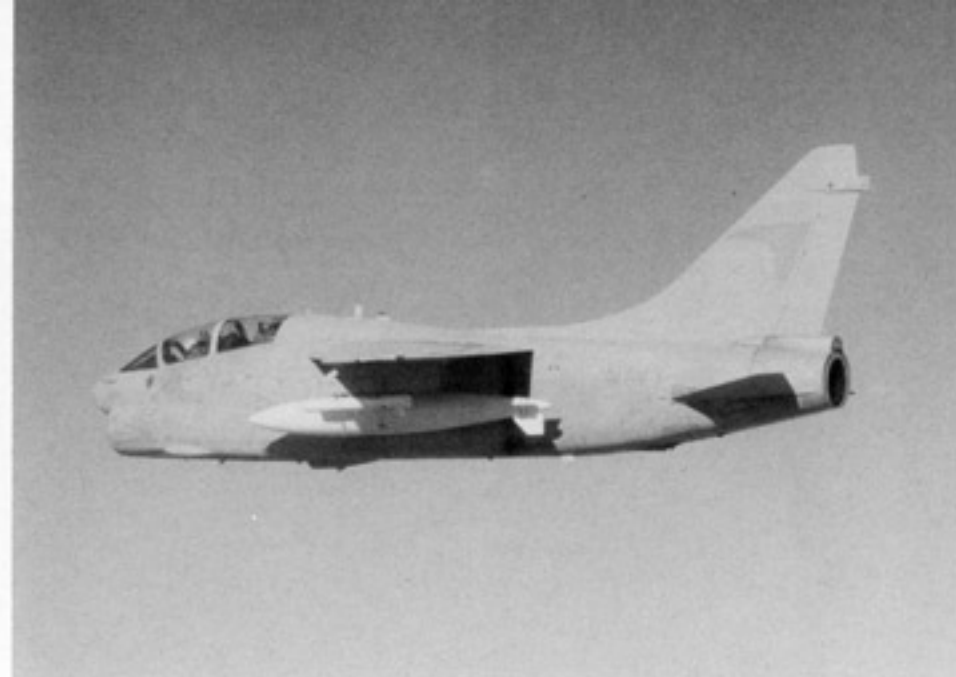
A TA-7C (BuNo 154544) of the Pacific Missile Test Center (PMTC) on a test mission carrying a radar simulator pod on the number one wing station. Aircraft number 82 is finished in overall Medium Gray with a stylized PMTC badge on the tail. (Navy)
