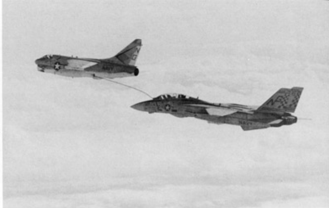
An A-7E of VA-146 Blue Diamonds refuels an F-14A Tomcat of VF-211 over the Pacific Ocean. Both aircraft are assigned to Carrier Air Wing NINE (CVW-9) based aboard the USS CON-STELLATION (CV-64) The A-7E was used as a backup tanker aircraft to the Grumman KA-6D. (Navy)
