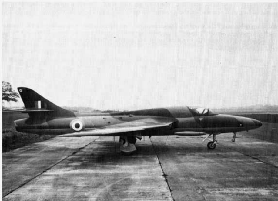
The Indian Air Force operated a number of Hunter trainers under the designation Hunter T.66. This IAF Hunter T.66 (BS361) served with No 17 Squadron at Peana. Like many other export models these aircraft were armed with two Aden cannons. (BAe)
