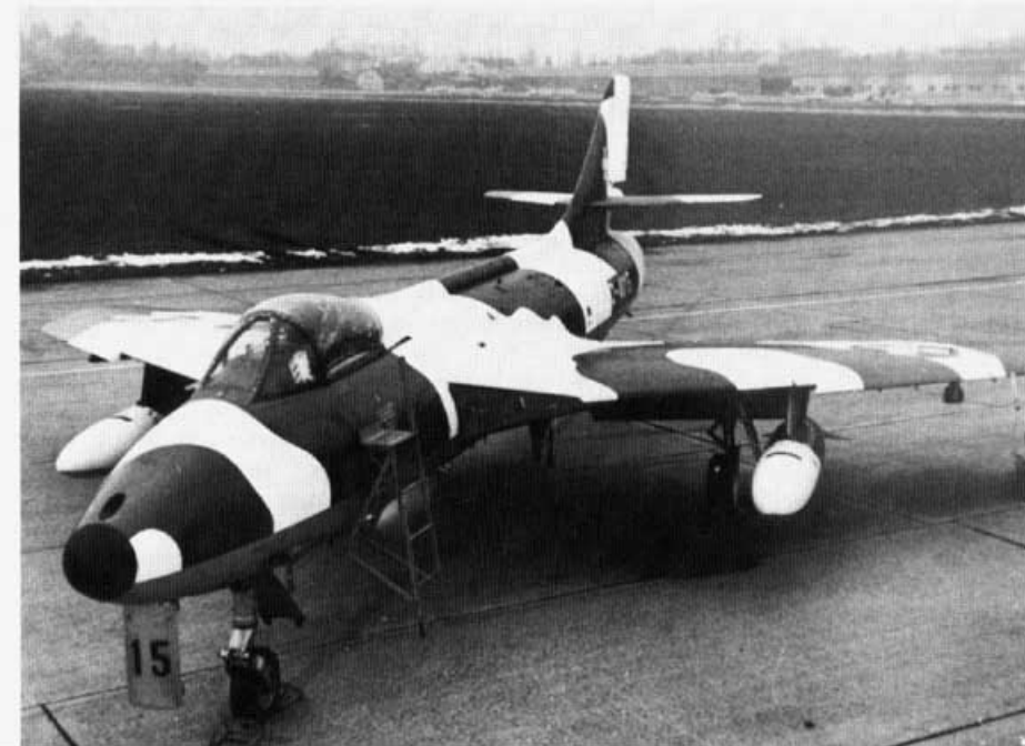
This Swiss Hunter F.58 (J-4015) has had the Gray areas of its two tone camouflage scheme overpainted with a White water-color paint to produce a temporary winter camouflage. (Hans Prisi via Paul Hohn)
