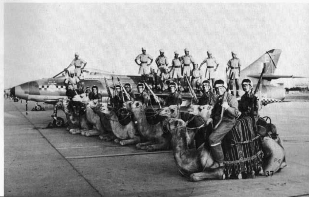
Pilots of No 43 Squadron pose with Gurkha troops in Aden during the late 1960s. XG298/E was a Hunter F.6 that was rebuilt to FGA.9 standard. The bar across the fin is a gust lock, which kept the rudder from being damaged in the windy conditions on airfields in Aden. (BAe)
