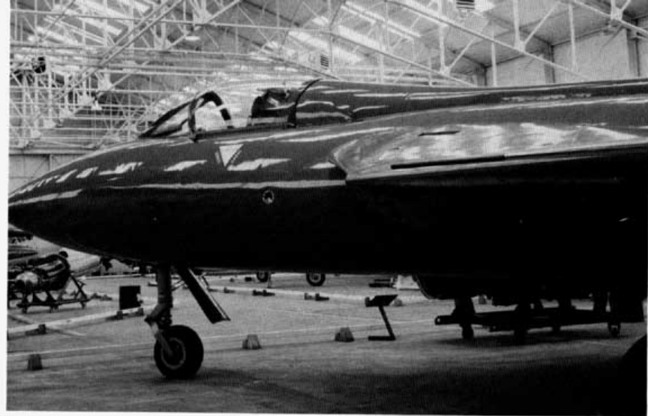
The first prototype Hunter was later modified into the sole Hunter F.3 prototype for an attempt on the World Air Speed Record. The aircraft was modified with a pointed nose and painted with a high gloss finish to reduce drag. (Author)
