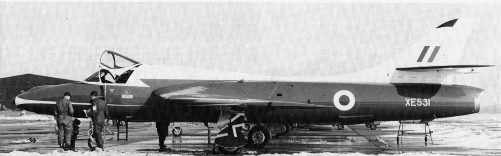
XE531 was the sole Hunter T.12 and was intended to be the trainer for the cancelled TSR.2. It was powered by an Avon and was to have been fitted with the same terrain following equipment as the TSR.2, including a camera in the nose. After the TSR.2 was cancelled the Hunter was operated by the RAE at Farnborough in a special Green and White paint scheme. (BAe)
