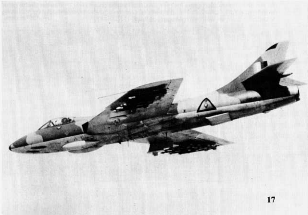
A Hunter F.6 (401) of the Royal Iraqi Air Force carrying the alternate outer wing armament of twelve three inch rockets. The aircraft also carries dual practice bomb carriers on the inboard pylons. The Hunter carries the early type Iraqi fin flash, used prior to the left wing revolt. (BAe)
