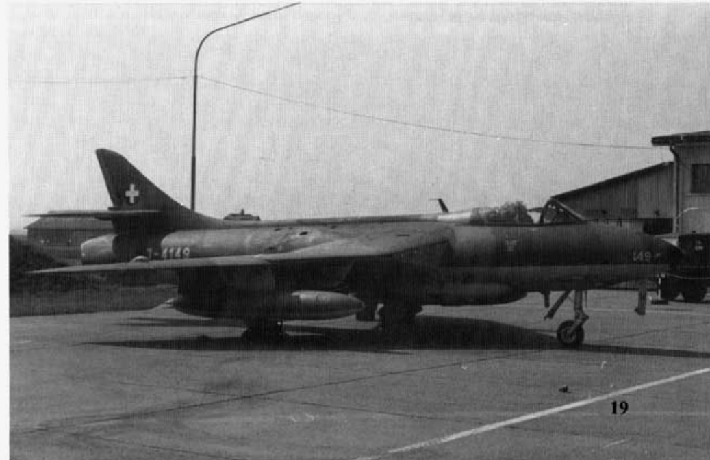
Over the years, Swiss Hunters have been upgraded and modified. One of these modifications was the addition of an extra underwing pylon inboard of the normal inboard pylon. (Mauro Ottagalli)
