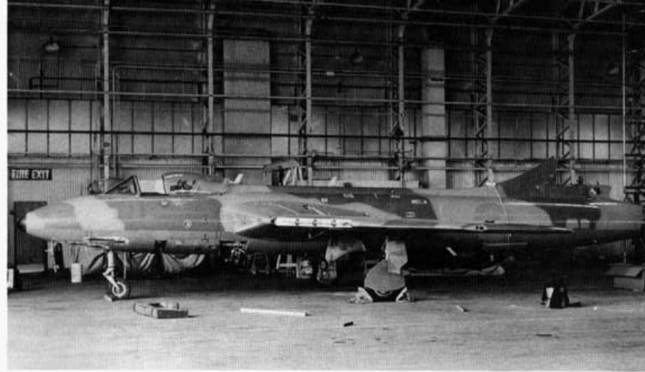
A Hunter FGA.78 of the Qatar Air Force undergoes major maintenance. The aircraft was a former RNethAF aircraft rebuilt to FGA.9 standard for Qatar. These aircraft were later replaced by Alpha Jets and Mirage F.1s. (MAP)
