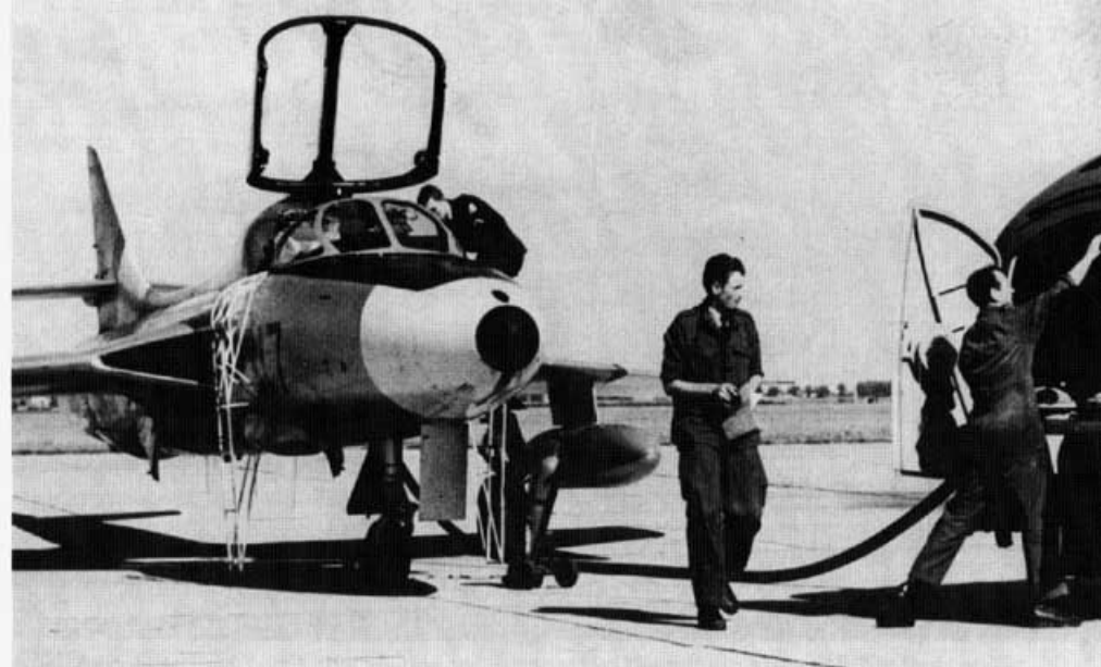
Ground crewmen prepare a Hunter T.7 (N-317) for a training sortie at an airbase in Holland. Dual boarding ladders are in place and the aircraft is being fueled from a fuel truck. As a safety measure a large fire extinguisher is positioned near the refueling point. (RNethAF)
