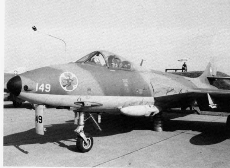
This Hunter of No 4 Staffel carried the unit insignia on the nose. The aircraft has been modified with radar warning antennas on the nose and chaff/flare dispensers installed in the link collector blisters. (Mauro Ottogalli)
