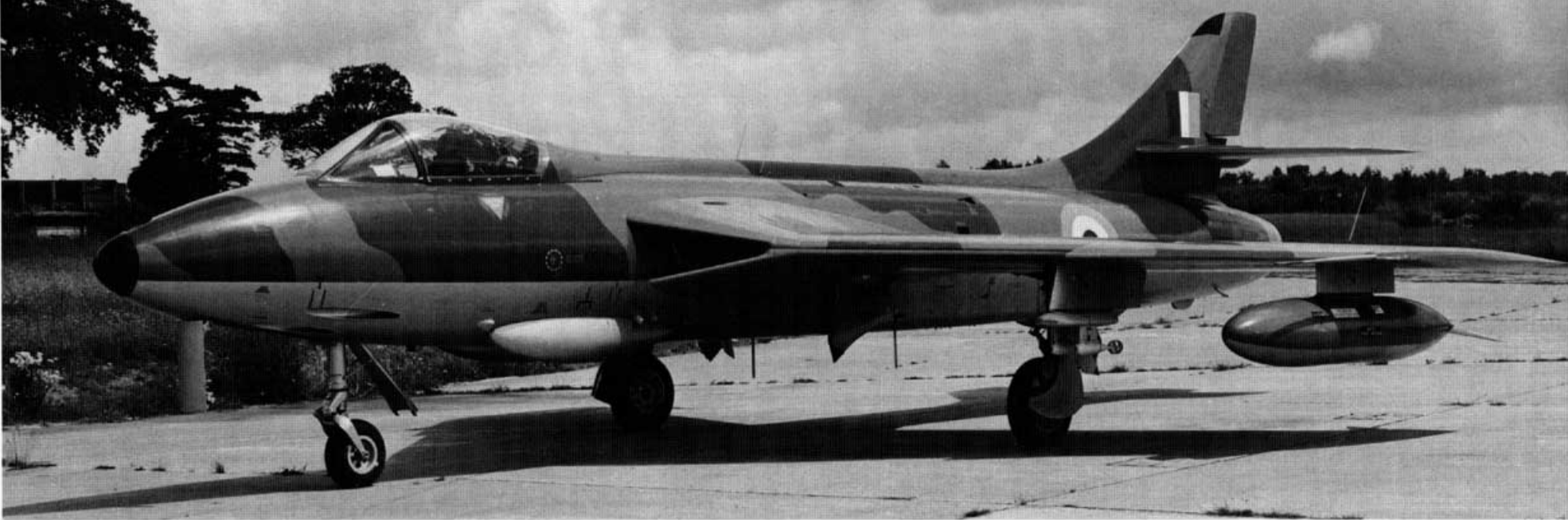
An Indian Air Force Hunter F.56 (F.6) armed with a dual practice bomb carrier on the inboard pylon and carrying 100 gallon fuel tanks on the outboard pylon. The Hunter F.6 and its export variants were the first Hunters to feature the outboard wing pylon. (BAe)
