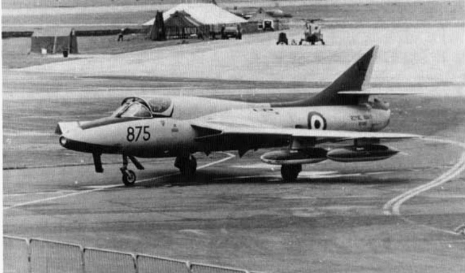
A Hunter T.8 (XF289) of the FRADU taxis out along the perimeter track at RNAS Yeovilton. The aircraft was converted from a Hunter F.4 and is equipped with a Harley light in the nose. The aircraft is overall Gray with Dayglo Orange areas on the nose, wings and fin. (Tim Laming)
