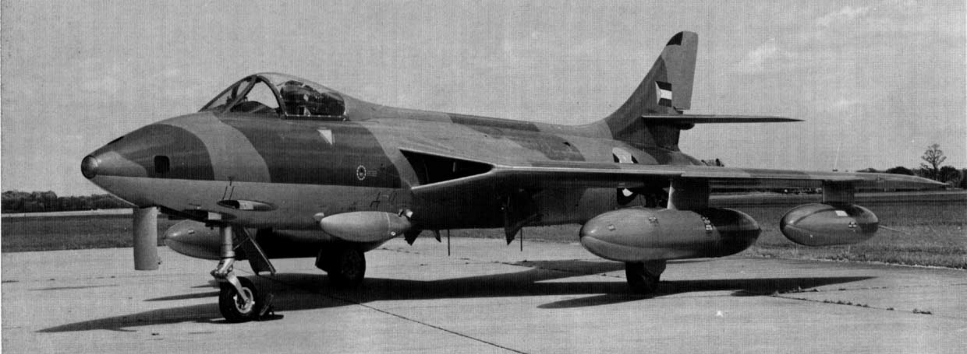
This Jordanian Air Force Hunter FR.10 reveals the arrangement of the forward oblique and left oblique cameras. The forward oblique camera has a sliding cover over the window to protect it. A number of these aircraft were later passed to the Sultan of Oman Air Force. (BAe)
