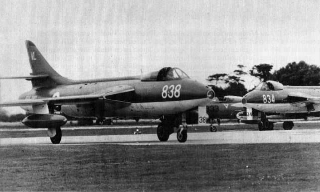
The Royal Navy operated a number of Hunter GA.11s from RNAS Yeovilton. The GA.11 had the gun armament and link collector blisters deleted and had a large search light, known as a Harley light installed in the nose. (Tim Laming)
