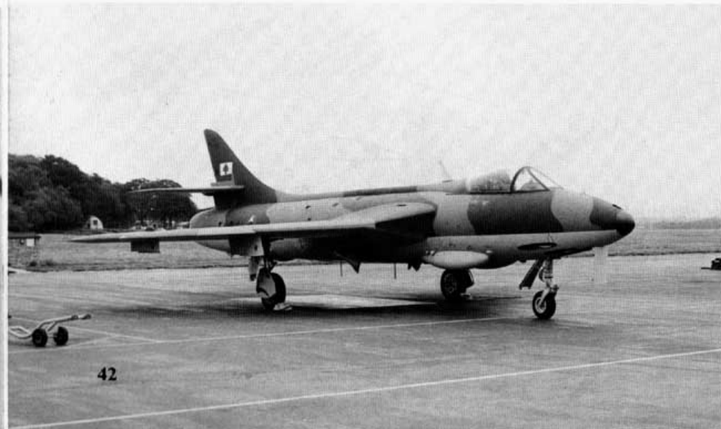
FGA.70s featured a large blade antenna on the spine, two whip antennas under the fuselage and a "towel rail" antenna on the port fuselage side. Unlike the earlier Hunters flown by Lebanon, the fin flash on the FGA.70s was horizontal. (BAe)
