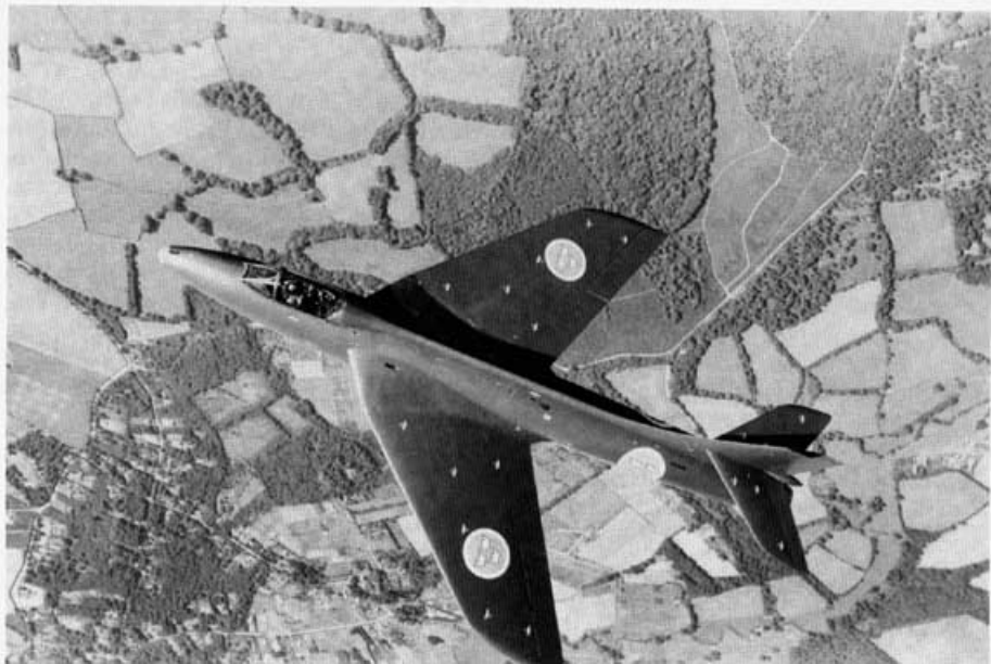
Swedish Hunter F.50s carried a camouflage of Dark Green uppersurfaces over light Blue-gray undersurfaces. These are the only Hunter variants to carry a single color uppersurface camouflage. (BAe)
