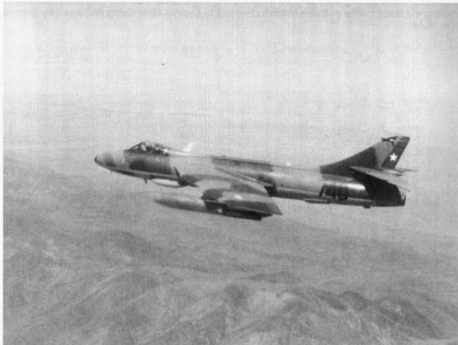
This Hunter FGA.71 (J-740) of the Chilean Air Force has been upgraded with a Caiquen II radar warning receiver antenna on the fin as part of the the Aquila update program (via Jeff Ethell)
