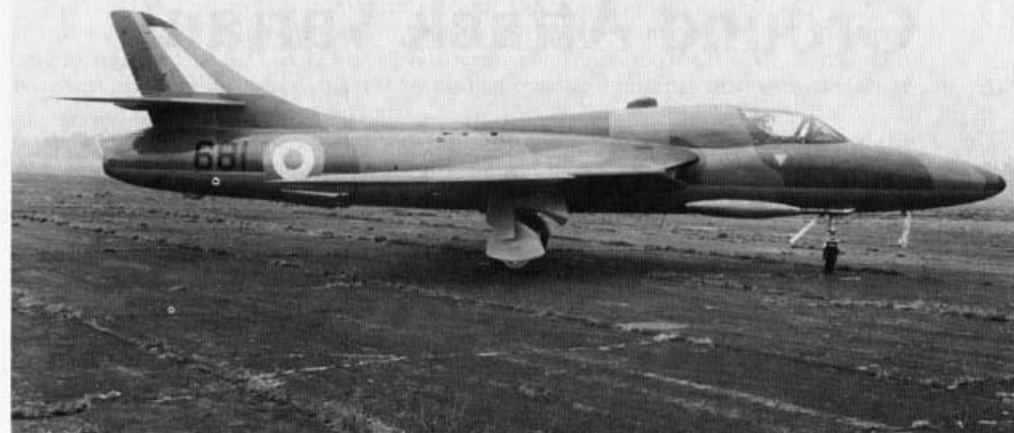
This Hunter T.62 was rebuilt from an F.4 airframe for delivery to Peru. This was the sole Hunter trainer operated by Peru and was modified with a directional compass in a blister behind the canopy. Hunter 681 carried standard British camouflage with Red, White, Red fin stripes. (BAe)
