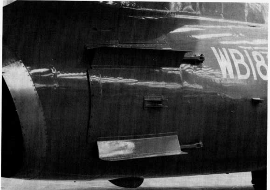
The Hunter F.3 prototype featured modified airbrakes mounted on the fuselage sides, which replaced the single piece ventral airbrake normally carried on the fuselage underside. (Author)
