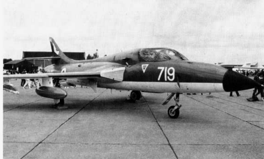
With the introduction of the Sea Harrier into Fleet service, a number of Hunter T.8s were modified with Blue Fox radars and radomes. This Hunter T.8 (XL580) was modified under the designation T.8M and assigned to No 899 Squadron. The aircraft also carries a Sidewinder missile simulator on the outboard wing pylon. (Author)
