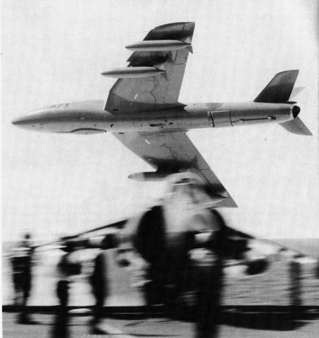
A Hunter T.8C (XF893) of the FRADU makes a low fast pass by the stern of the British carrier HMS ILLUSTRIOUS during a naval exercise off the coast of Britain. The tail hook is an identification feature of the Hunter T.8 and was used for field carrier landing practice. (Author)
