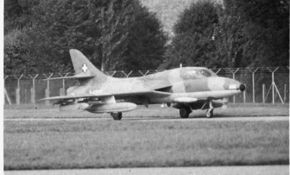
This Swiss Air Force Hunter T.68 is carrying an Electronic Countermeasures Pod on the outboard wing pylon. Swiss Hunter trainers are armed with twin Aden 30mm cannons in semi-recessed housings under the forward fuselage. (Author)
