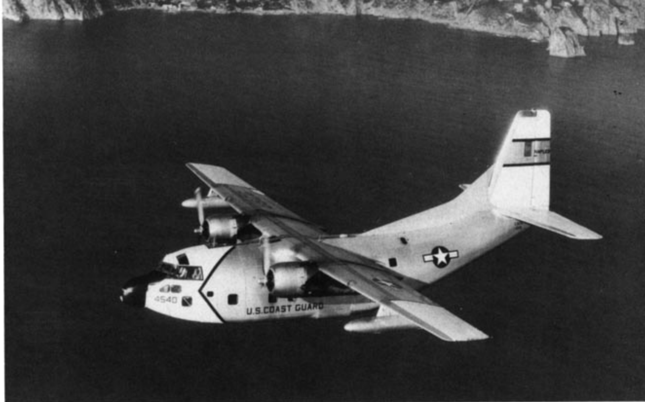
During 1958, the United States Coast Guard (USCG) began receiving the HC-123B. The HC-123B was simply a C-123B airframe modified with an AN/APN-158 search radar and radome in the nose. This HC-123B (55-4540) was assigned to the USCG base at Naples, Italy. (USCG via R.L. Scheina)
