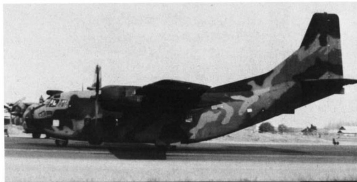
In 1966, a single C-123B was fitted with a special movable housing containing high intensity lamps carried on the lower tailgate. These lamps provided a long lasting constant light source capable of lighting a two mile diameter when the aircraft was at 12,000 foot altitude. The disadvantage over flares was the lights were affixed to the aircraft making it easy to track by enemy anti aircraft gunners. (USAF)
