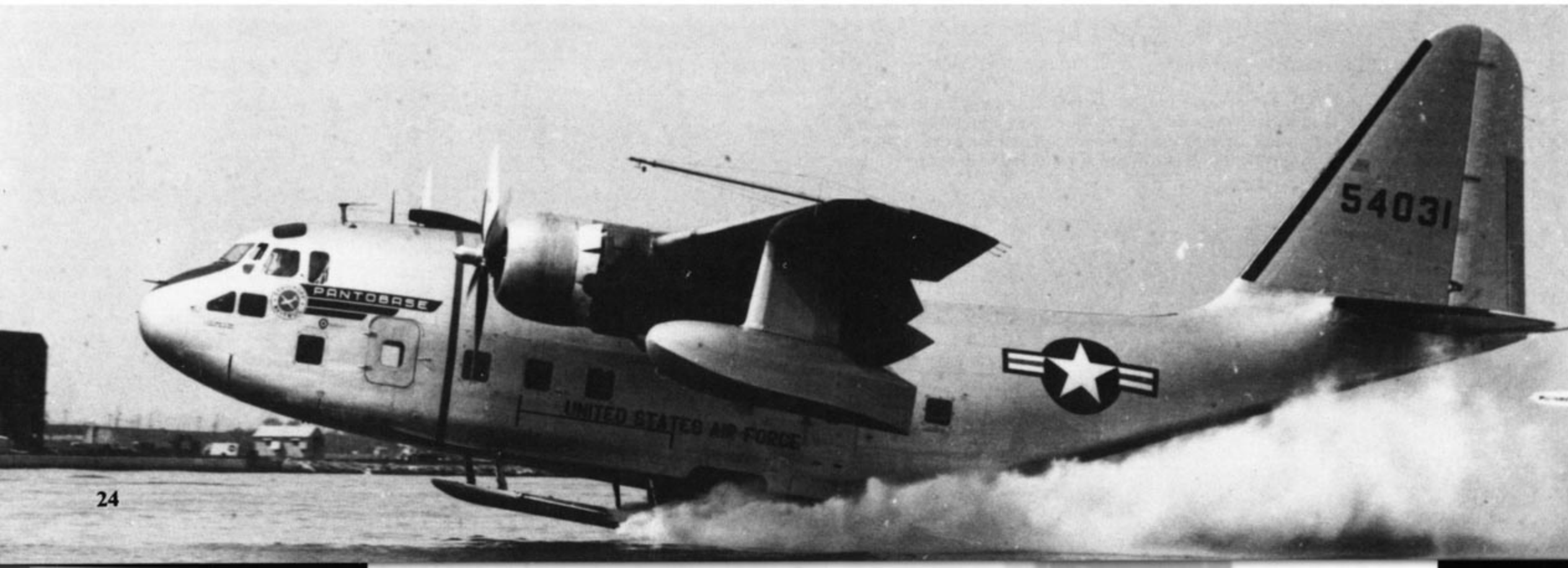
With its skis extended, the YC-123E lifts off from the Delaware River during flight tests at the Philadelphia Navy Yard in 1955. The underfuselage skis acted like a hydro-foil, lifting the aircraft off the water at a speed of some twenty knots. (USAF)
