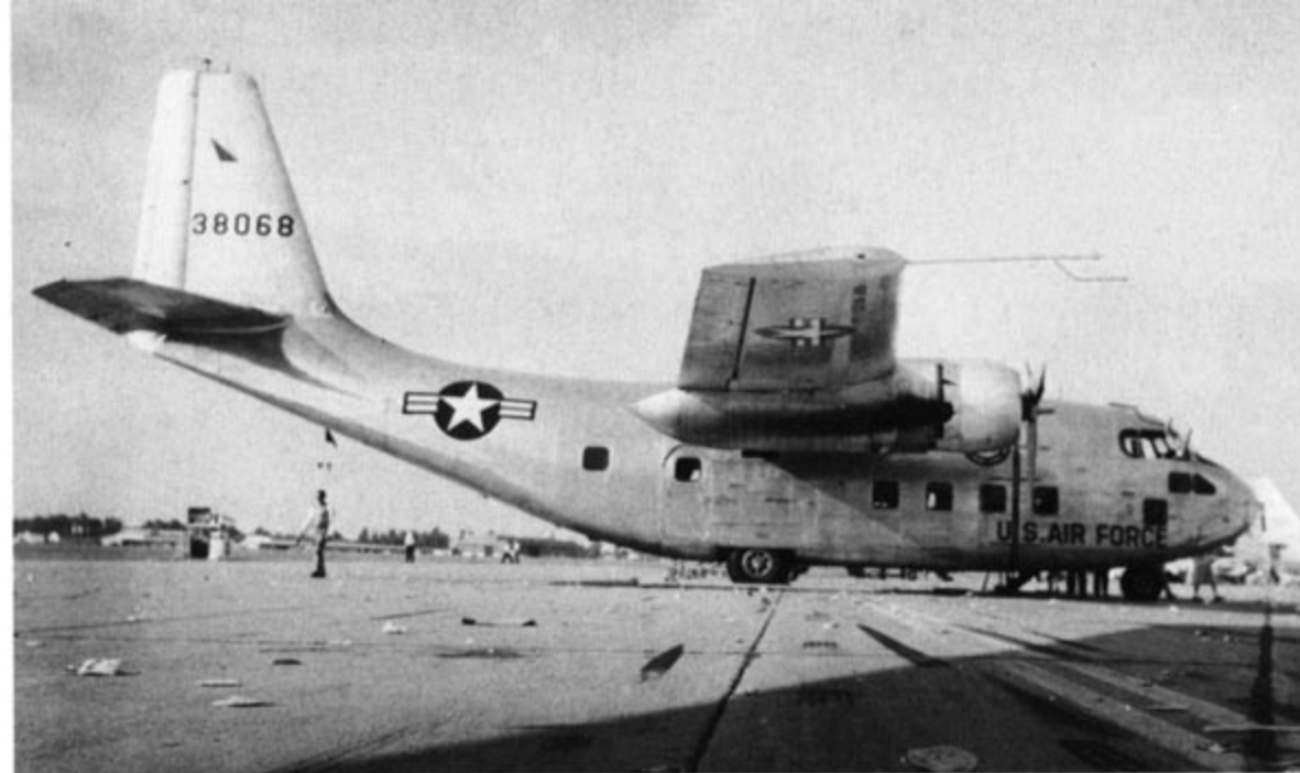
The sole YC-123D (53-8068) was the re-engined XC-123A. The jet pods used on the XC-123A were replaced with Pratt & Whitney R2800 radial engines and the vertical stabilizer was altered to the early C-123B configuration. The YC-123D was fitted with a Boundary Layer Control (BLC) system. (David Menard)
