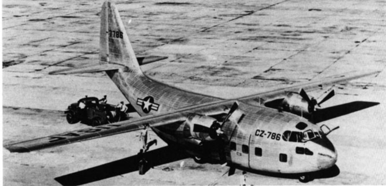
The first production XCG-20 glider was fitted with a pair of air cooled Pratt & Whitney R-2800-83 Double Wasp radial engines and first flown on 14 October 1949. The Chase Aircraft Company under the direction of Michael Stroukoff had developed the MS-8 as both a powered and glider assault transport for the USAF. (National Archives)
