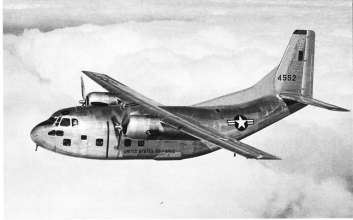
The first Fairchild C-123B made its first flight on 1 September 1954, piloted by E.R. (Dutch) Gelvin. The Fairchild C-123B differed from the Chase aircraft in the addition of a dorsal fin. The fin was added to correct a lateral control problem found in the Chase C-123 aircraft. (Fairchild)
