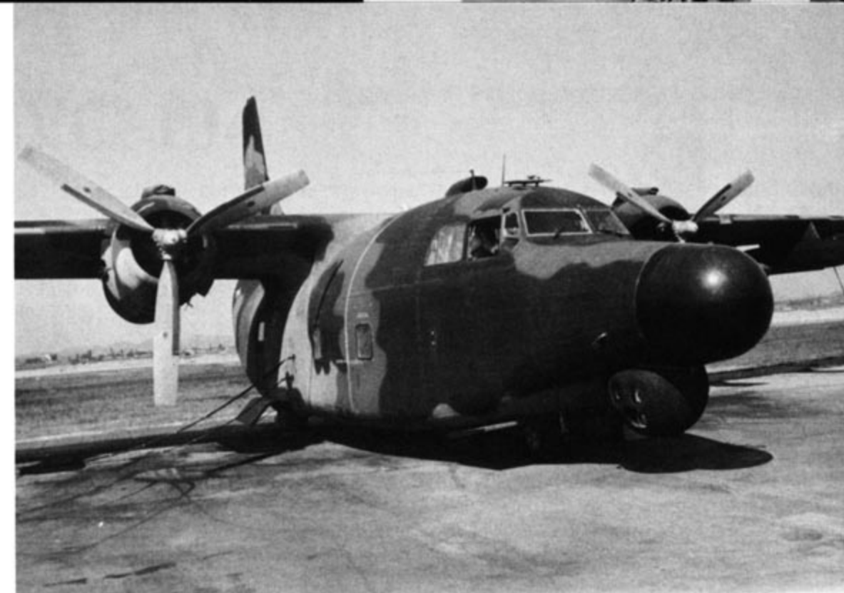
The chin sensor turret is rotated to look to the starboard side of the aircraft. The thimble nose radar housed a surface search radar with a Moving Target Indicator (MTI) function. Often initial contact with a target was made with the radar, then further tracking was done with the sensor turret. (Larry Davis)
