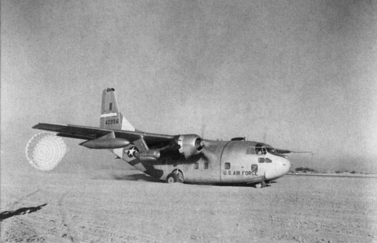
The YC-123H (54-2956) was also evaluated under desert conditions during 1963. The wide track landing gear system increased stability on the ground and the auxiliary jet pods proved invaluable for both safety and performance. (NASM)
