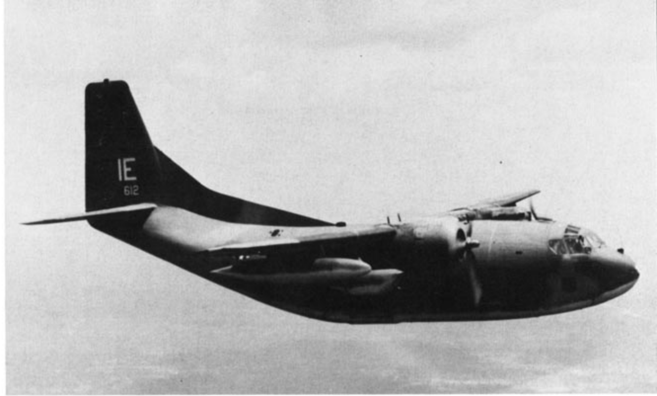
A C-123K (54-612) of the 319th Special Operations Squadron flies over the North Florida countryside on a crew training flight. This aircraft has an FM radio whip antenna mounted on the nose. FM radios were used to contact ground forces. (USAF via R. Bankston)
