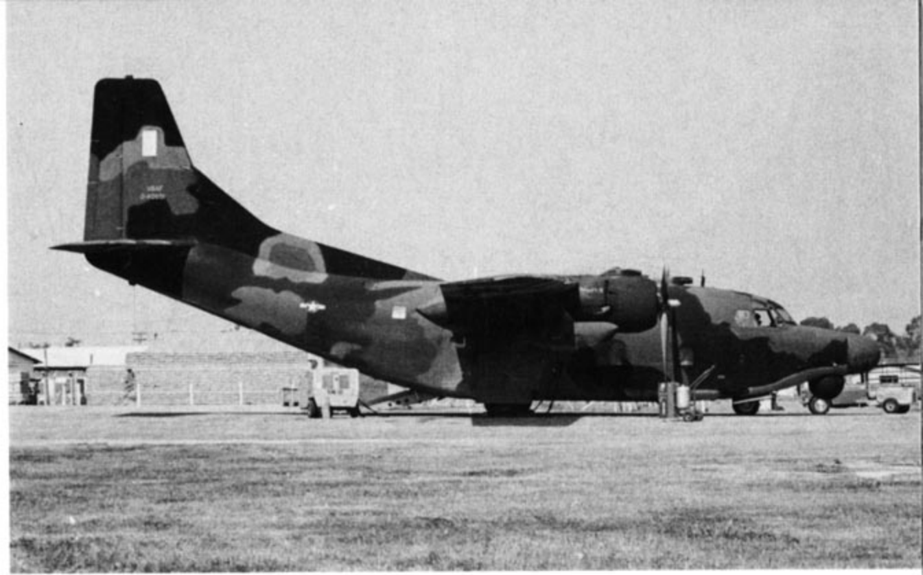
NC/AC-123K (54-691) was later fitted with a chin turret containing a Low-Light-Level Television (LLLTV), laser range finder and infrared scanner. The combination of the infrared scanner, LLLTV and bomblets enabled the two NC/AC-123Ks to destroy a large number of North Vietnamese trucks during the 1969-70 period. (Norm Taylor)
