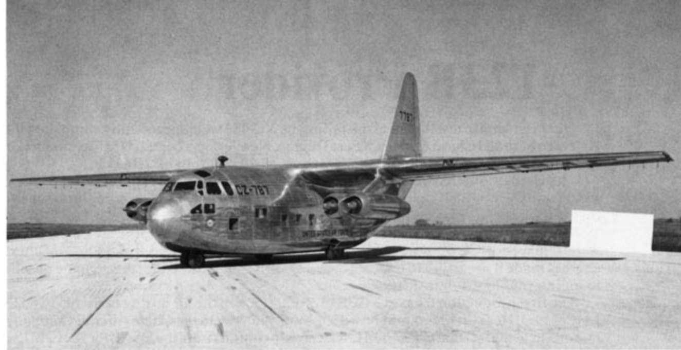
The second production XCG-20 glider (47-787) was fitted with four J47-GE-11 jet engines (the same as the Boeing B-47) under the designation XC-123A. The aircraft was the first U. S. built jet powered transport and had a top speed of over 500 mph. Fuel was carried in a tank mounted under the cargo bay floor since no provisions had been made in the wings for fuel. (National Archives)
