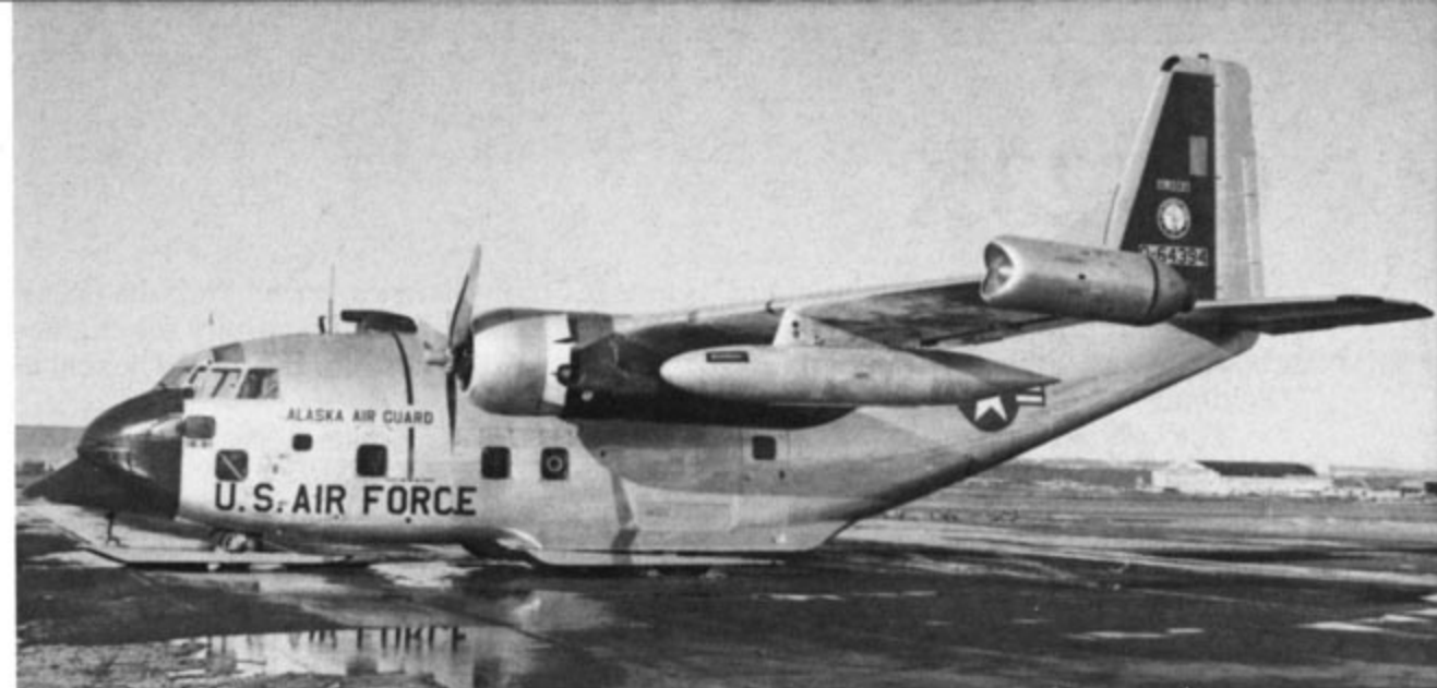
A ski equipped C-123J (56-4394) of the Alaskan ANG sits on the rain soaked ramp at Anchorage, Alaska during March of 1970. The wheel landing gear protruded through the skis allowing the C-123J to land on hard surface runways as well as snow. (Norm Taylor)
