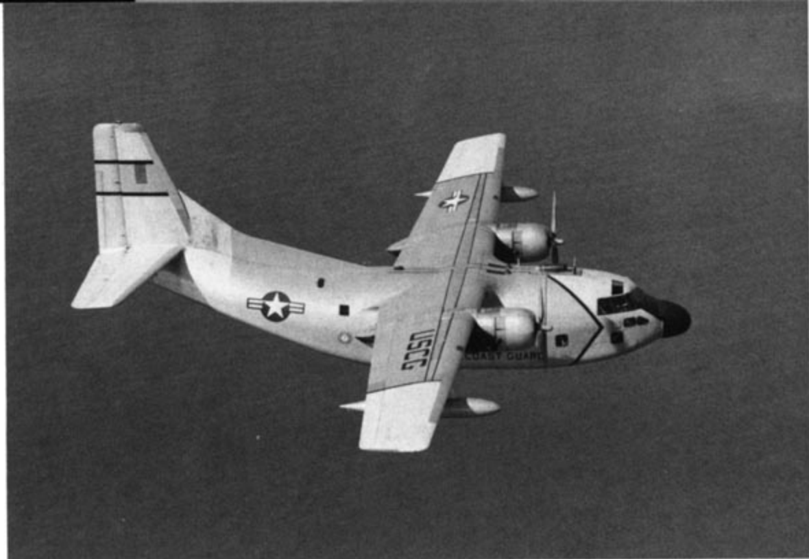
HC-123B aircraft were used by the USCG in the search and rescue role, as well as the support transport role. The aircraft were overall Natural Metal with the nose, wing tips and tail in Yellow. The nose and wings had the Yellow outlined in Black. This HC-123B was assigned to Honolulu, Hawaii. (USCG via R.L. Scheina)
