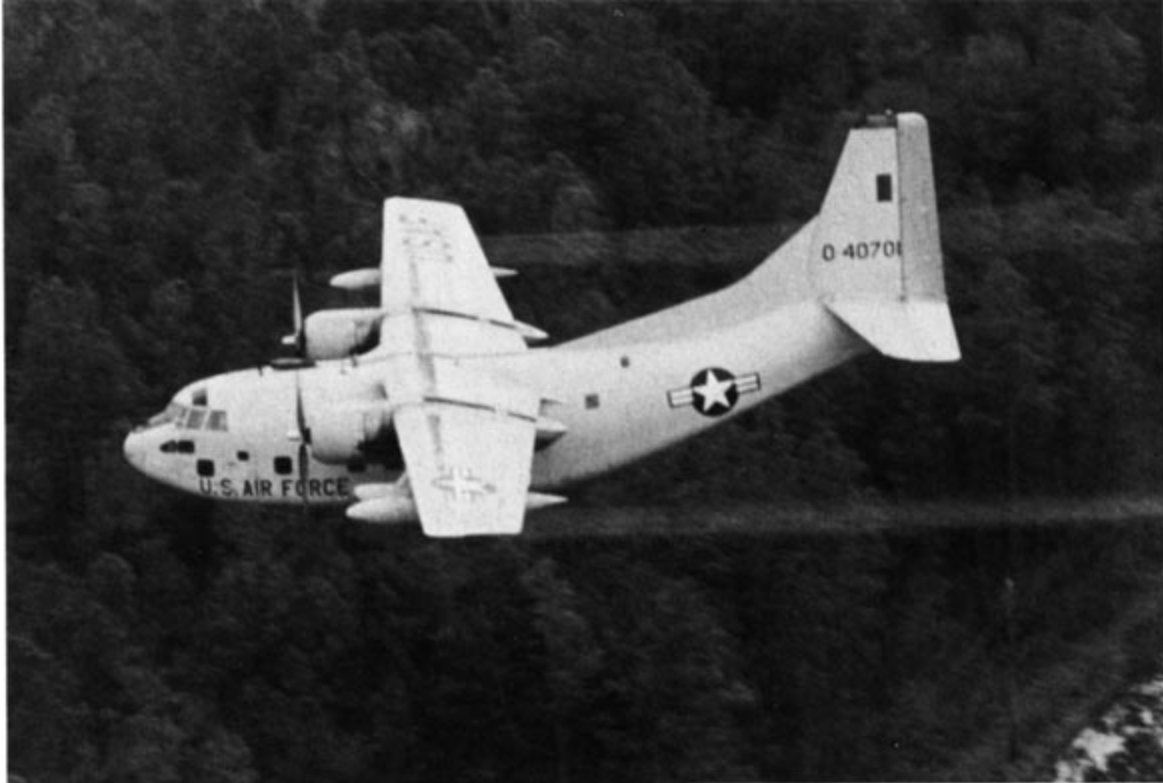
A UC-123K (54-701) sprays for mosquitos at Fort Stewart, Georgia during March of 1976. By 1976, Air Force and USAF Reserve transport aircraft were being painted in overall Light Gray. The 0 preceding the serial number on the fin indicated that the aircraft is over ten years old. (USAF)
