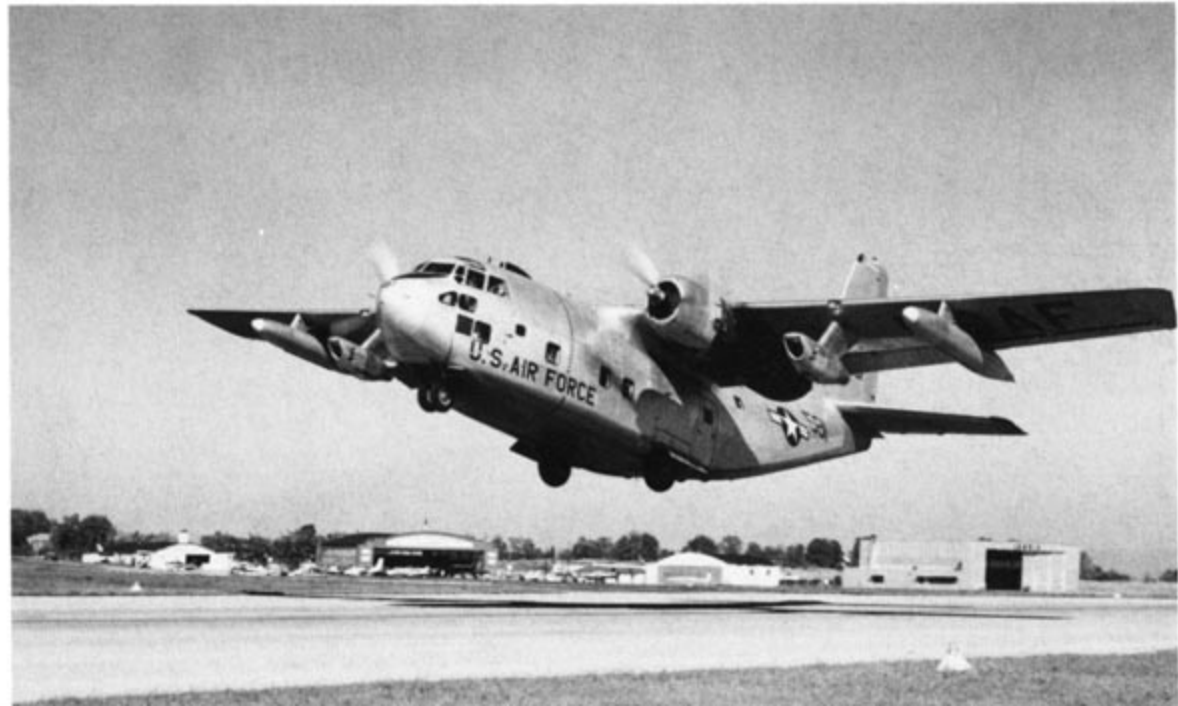
A newly converted C-123K (54-581) takes off from the Fairchild facility during 1966. The small openings on the sides of the General Electric J85-GE-17 jet engines are blow in doors which open when the engines are at high throttle settings to take in the maximum amount of air. (Fairchild)
