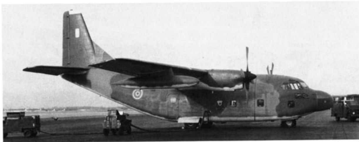
The C-123T had the Pratt & Whitney R2800S radial engines replaced with Allison T56-A-7B turboprop engines. The conversion work was done by Mancro Aircraft of Paramount, California during 1980. The aircraft was to feature a "wet" wing for additional fuel. (David Menard)
