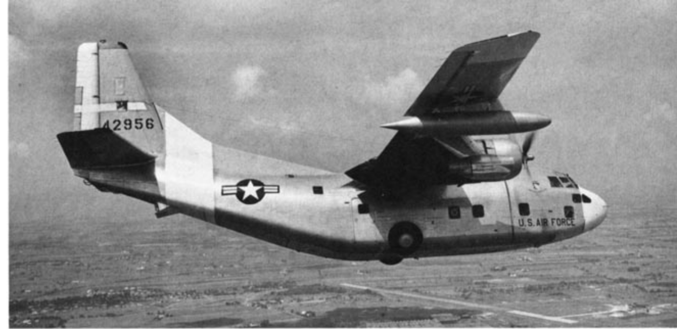
The pilot of the YC-123H has opened the braking parachute door (on the lower rear fuselage) in preparation for landing. The aircraft was overall Natural Metal with Orange bands on the nose, fuselage and wings. The wide track landing gear components were from a Lockheed C-130. (Fairchild)
