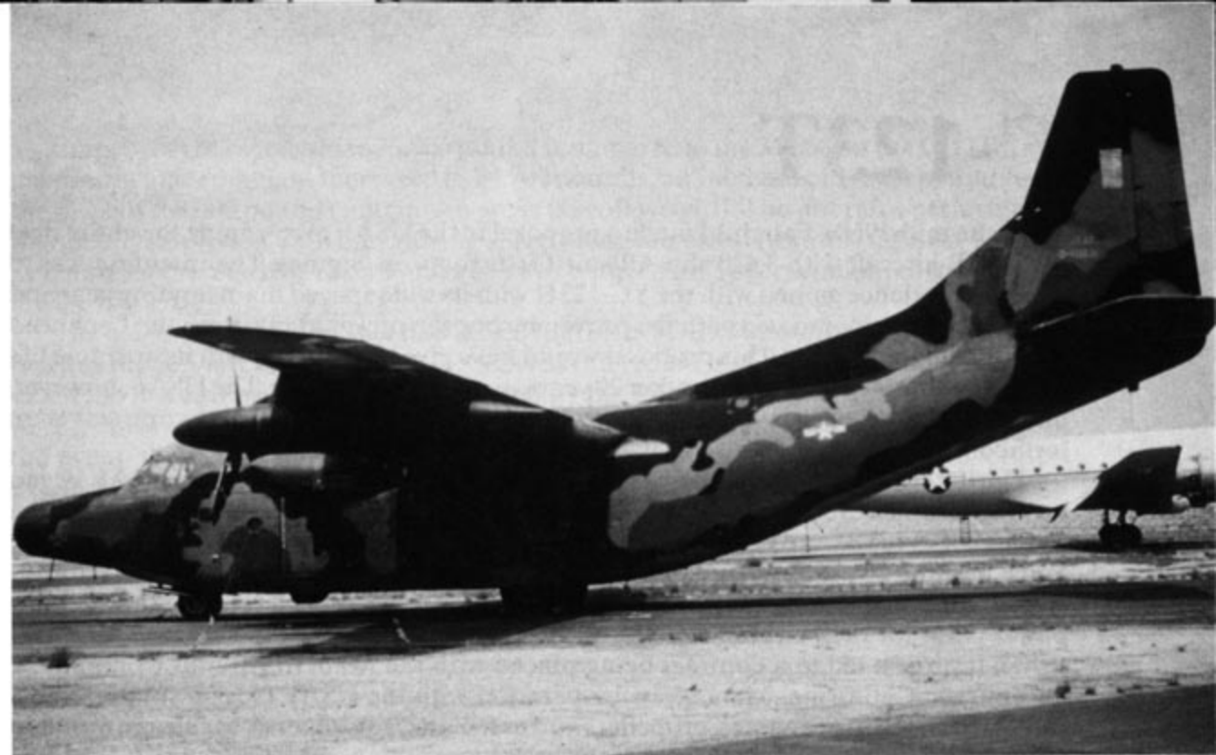
There were two aircraft modified under Project Black Spot and the highly modified C-123Ks were, at various times, designated either as AC-123Ks or NC-123Ks. 54-691 was outfitted with an extended nose radar housing and infrared sensors. (Via Wayne Mutza)
