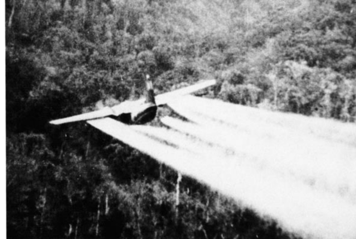
A UC-123K makes a spray run over a Vietnamese jungle. The defoliant would cause the leaves to fall, denying the Viet Cong hiding places. UC-123K spray planes flew at altitudes as low as 100-150 feet and speeds of 120 knots, making them easy targets for anti-aircraft fire. (Via Jack Spey)
