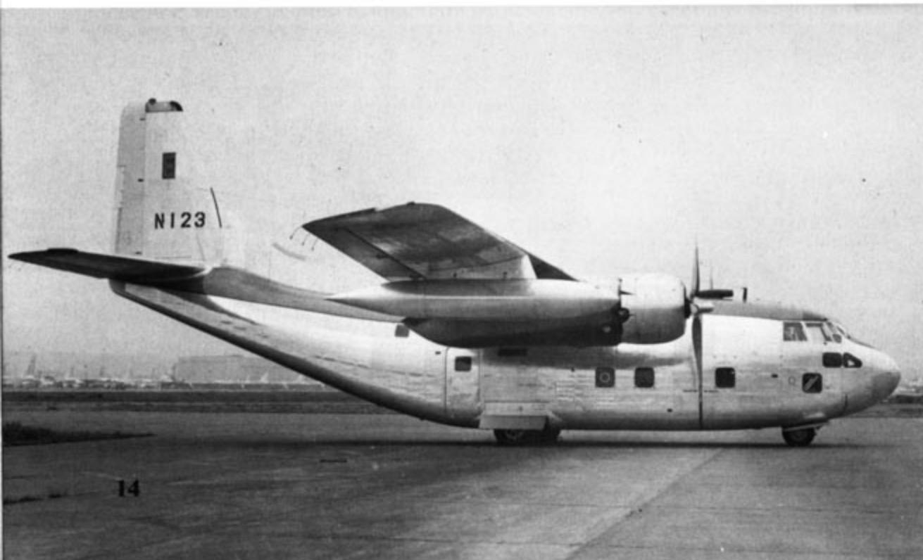
The Federal Aviation Administration (FAA) used this C-123B (55-4558/N123) from the late 1950s until the early 1970s in Alaska to check Instrument Landing Systems (ILS) and other aids to navigation. The aircraft was later converted to C-123J standard. (Balogh via Menard)
