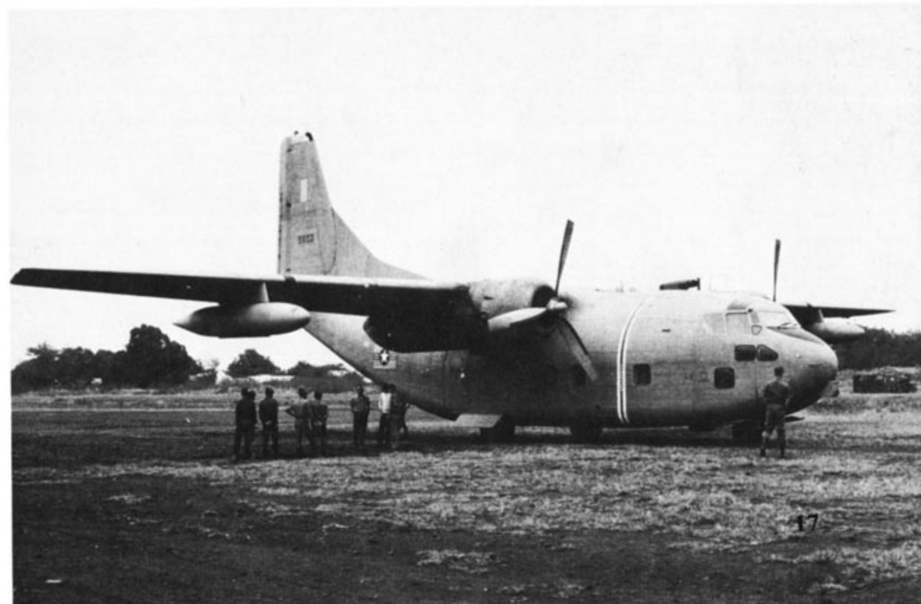
The first "anti-trail" aircraft to operate over the Ho Chi Minh Trail was this NC-123B which was fitted with a nose mounted infrared sensor. 54-652 was passing through the City Airstrip at Ban Me Thout, South Vietnam during 1964. The aircraft was painted in an overall Dark Gull Gray and carried VNAF insignia in a placard holder. (Author)
