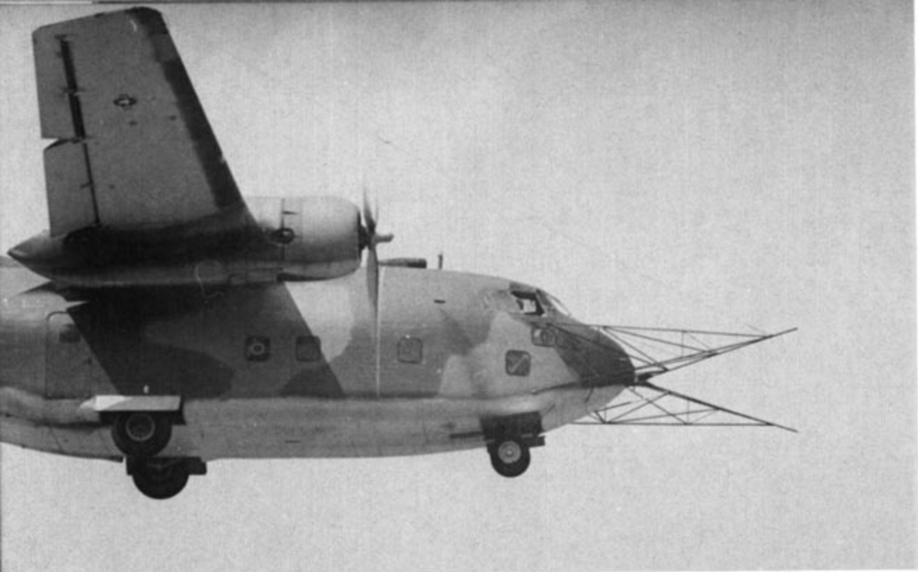
A modified C-123B (54-683) comes in for a landing at Shaw AFB, South Carolina on 26 September 1968. The aircraft was test fitted with the "Fulton Device" mounted on the nose. It was designed to snag a balloon lifted cable to rescue downed airmen. The aircraft was assigned to 4410th Special Operations Training Group, Hurlbert Field, Florida. (Jim Sullivan)
