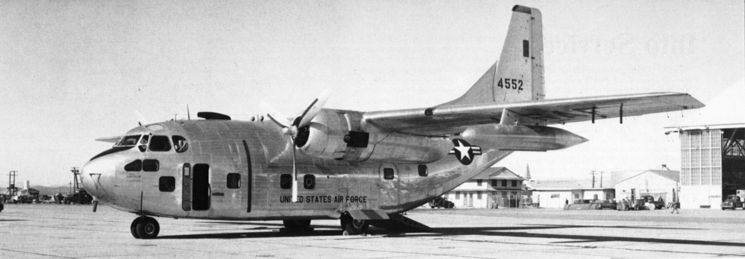
The first Fairchild C-123B (54-552) on the ramp at Edwards AFB, California during early 1955. The rear portion of each engine nacelle contained the primary engine fuel and could be jettisoned in an emergency. The aircraft could also carry two 400 gallon underwing fuel tanks. (USAF via Cheryl Gumm)
