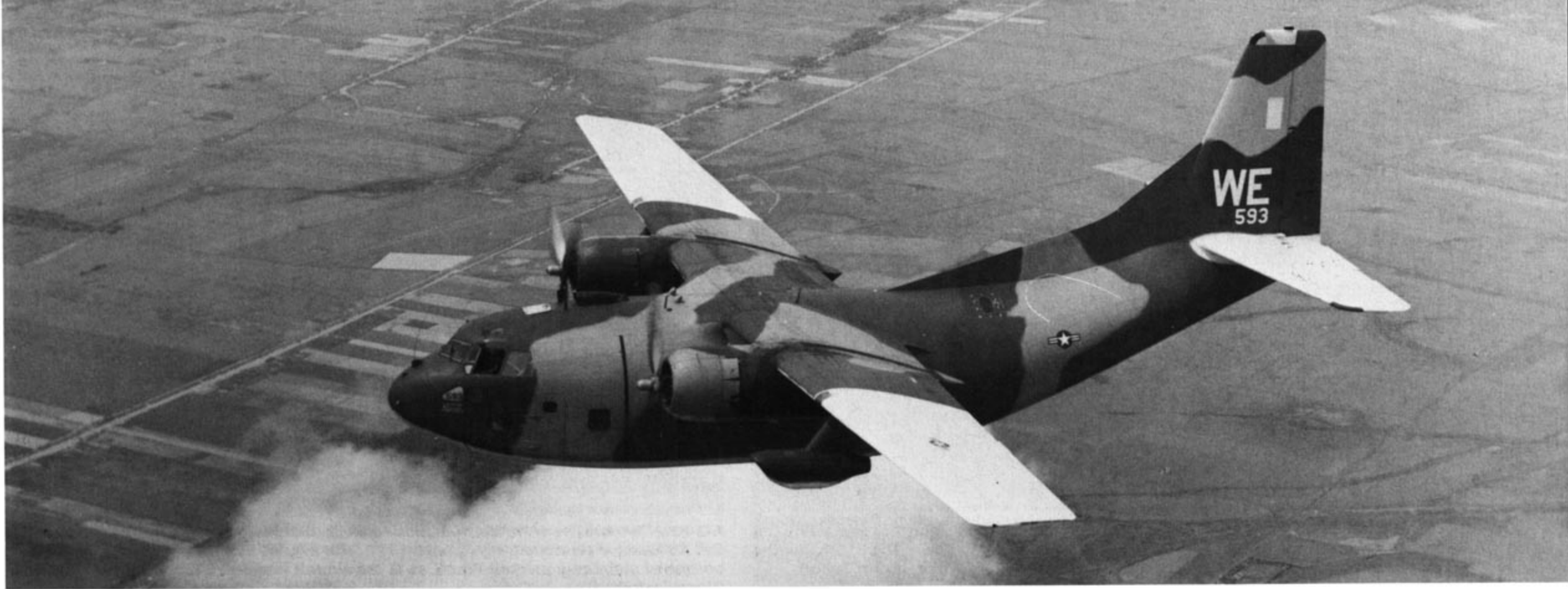
Some of the Tactical Transports Operating in the forward control zones of Vietnam, such as this C-123K (54-493), had a portion of the upper wing surface and stabilizers painted White as a recognition aid. This aircraft was assigned to the 315th SOW, Phan Rang. (USAF)
