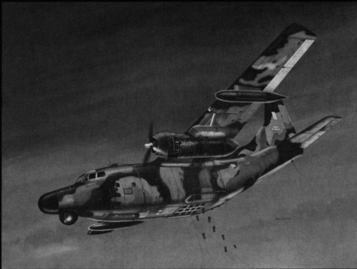
One of the project Black Spot aircraft drops part of its load of bomblets on an enemy target along the Ho Chi Minh Trail. Depending on the type of Cluster Bomb Unit (CBU) loaded, the NC/AC-123K could carry between 2,600 and 6,300 one pound bomblets.
