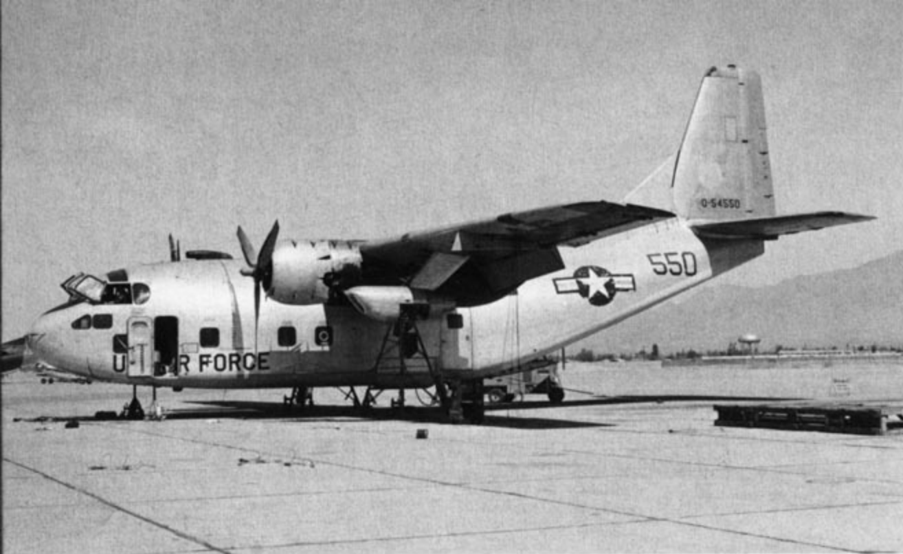
A C-123K (55-4550) undergoes refurbishment at Davis-Monthan AFB, Arizona on 25 March 1971. The aircraft would later be repainted in SEA camouflage and sent to Vietnam. It appears that the aircraft was undergoing a landing gear retraction test. (Lock via N. Taylor)
