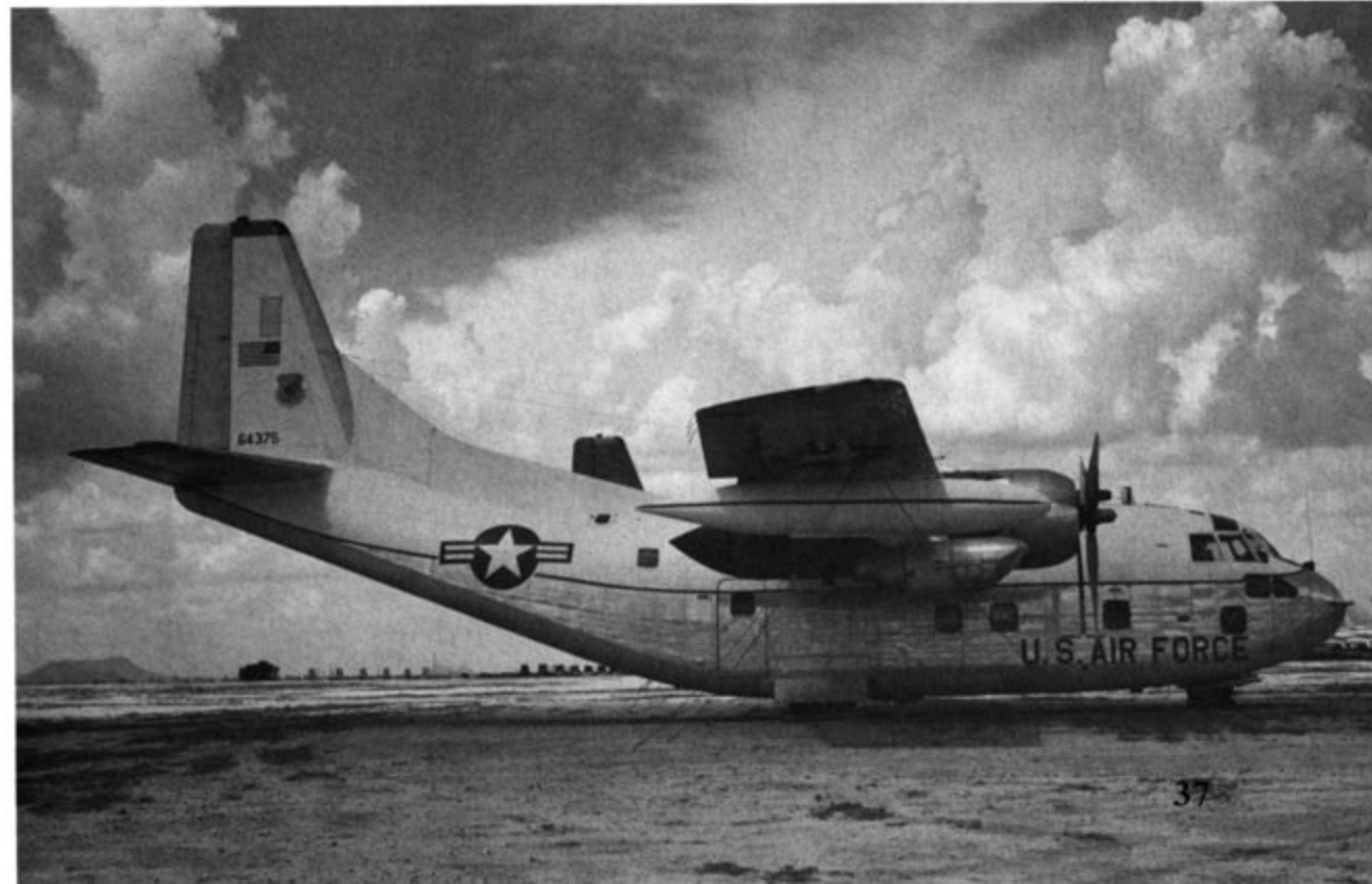
General Westmoreland's VC-123B was converted to C-123K standards, becoming the sole VC-123K. The aircraft featured a slide in module containing airline seats and airconditioning for passenger comfort. The aircraft had the upper fuselage painted White which led to its name, the White Whale . (Norm Taylor)
