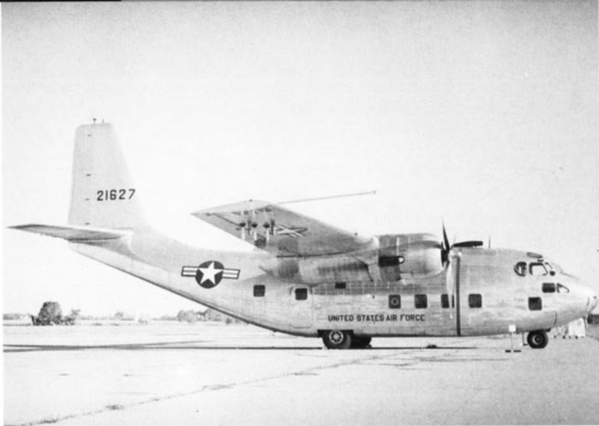
The C-123B was powered by two 2,500 hp Pratt & Whitney R-2800-99W air cooled radial engines. In May of 1953, after five C-123Bs had been produced, Chase Aircraft was purchased by Henry J. Kaiser and the USAF promptly cancelled the 300 aircraft production contract. (Balogh via Menard)
