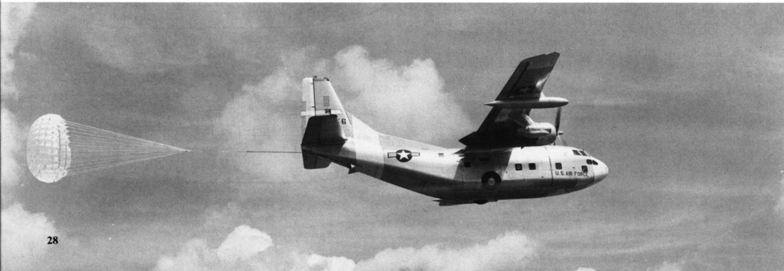
The YC-123H deploys its twenty-eight foot deceleration parachute as it prepares to land. The parachute enabled the YC-123H to make a far steeper angled approach which decreased the time the aircraft was exposed to enemy small arms fire. (NASM)
