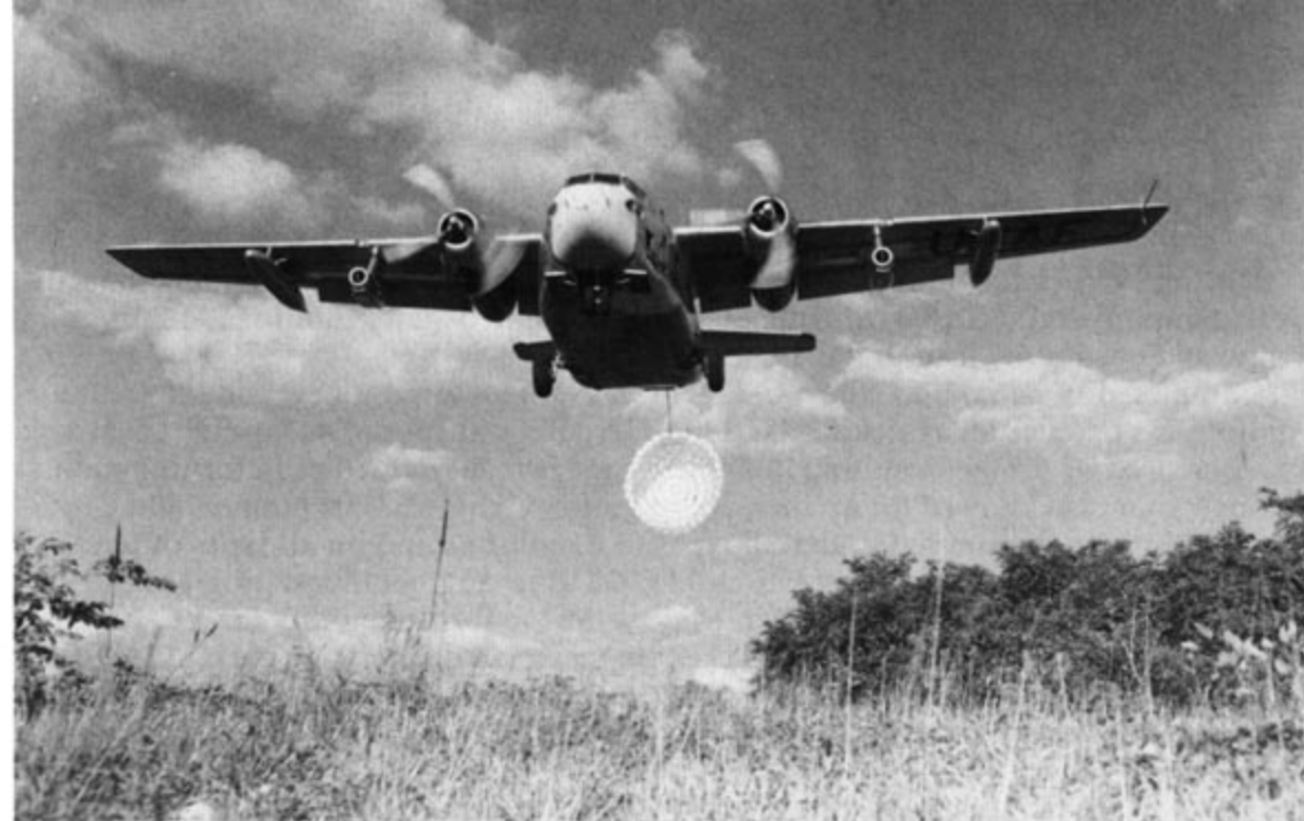
The YC-123H was evaluated in South Vietnam in the Counter Insurgency (COIN) support role during the early months of 1963. The aircraft flew over 180 missions and flew over 500 flight hours during the evaluation. During the evaluation, the YC-123H was flown at an average gross weight of 65,000 pounds. (NASM)
