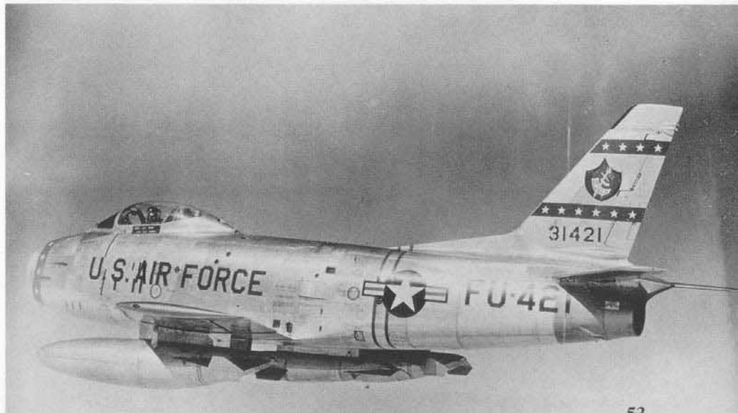
An F-86H-10 of the 10th FBS/50th FBW at Hahn AB, West Germany in the mid-1950s. The aircraft is configured for long range flight with four underwing drop tanks. Although certainly a good aircraft, the F-86H simply came too late and was quickly replaced by the North American supersonic F-100 Super Sabre. (via David Menard)
