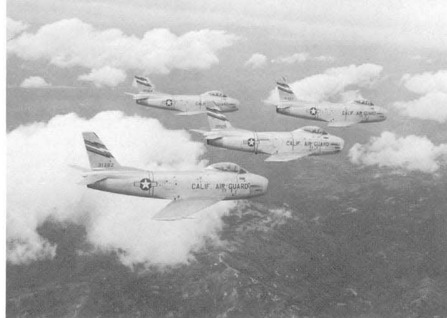
F-86Hs were rapidly phased into service with Air Guard units beginning in 1956 as F-100s became available for active USAF units. These F-86H-10s are assigned to the 195th FIS/California ANG. These aircraft have been painted overall Silver lacquer for corrosion control. (NAA)
