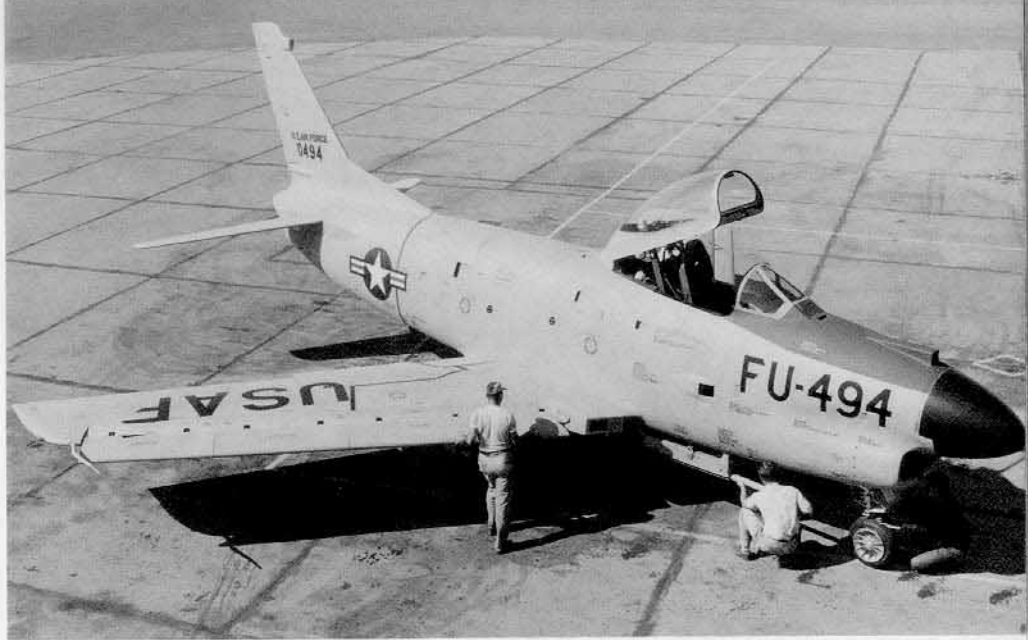
North American mechanics load the rocket tray on this overall Day-glo Red F-86D-1 Sabre at Edwards Air Force Base in the early 1950s. The fairings on the wing and fuselage house cameras to record the results of air-to-air rocket firing tests. (NAA)
