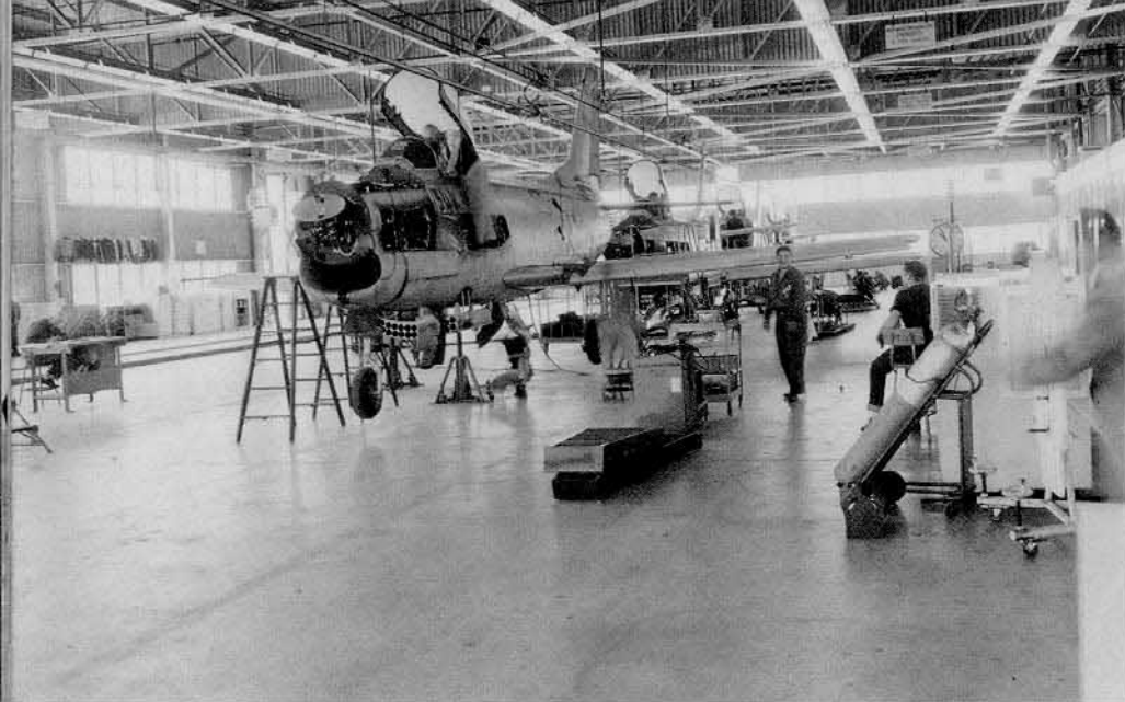
F-86Ds move into the radar installation point on the F-86D assembly line at Inglewood. The use of a 30 inch radar dish antenna meant that the intake had to be widened horizontally to provide sufficient air to feed the afterburning J47-GE-17 engine. (NAA)
