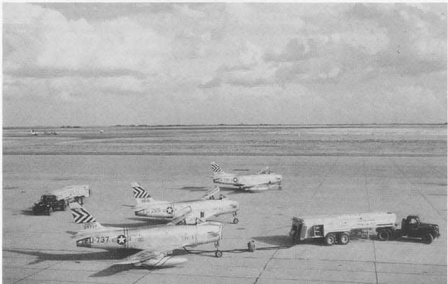
JP-4 fuel tankers refuel a trio of 428th FBS/474th FBW F-86H-5s at Clovis AFB during 1954. Repeated problems with the M39 cannon installation resulted in cracked gun bay walls and even fuselage cracks. This, plus developmental problems with the J73 engine, brought a quick end to the USAF service life of the F-86H. (NAA)
