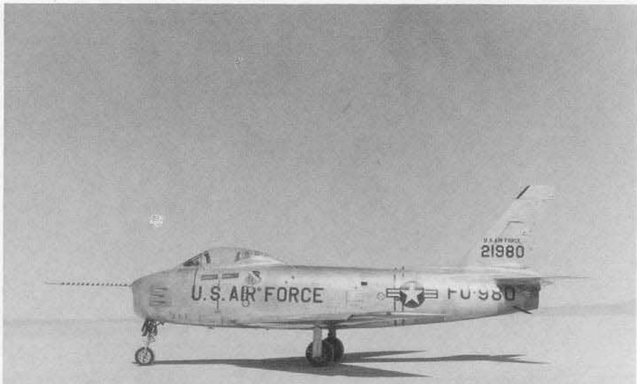
The YF-86H-1 service test aircraft at Edwards AFB during 1954. The early production F-86H-1s retained the six .50 caliber machine gun armament, which was replaced by M39 cannons beginning with the 117th aircraft off the production line. (USAF)
