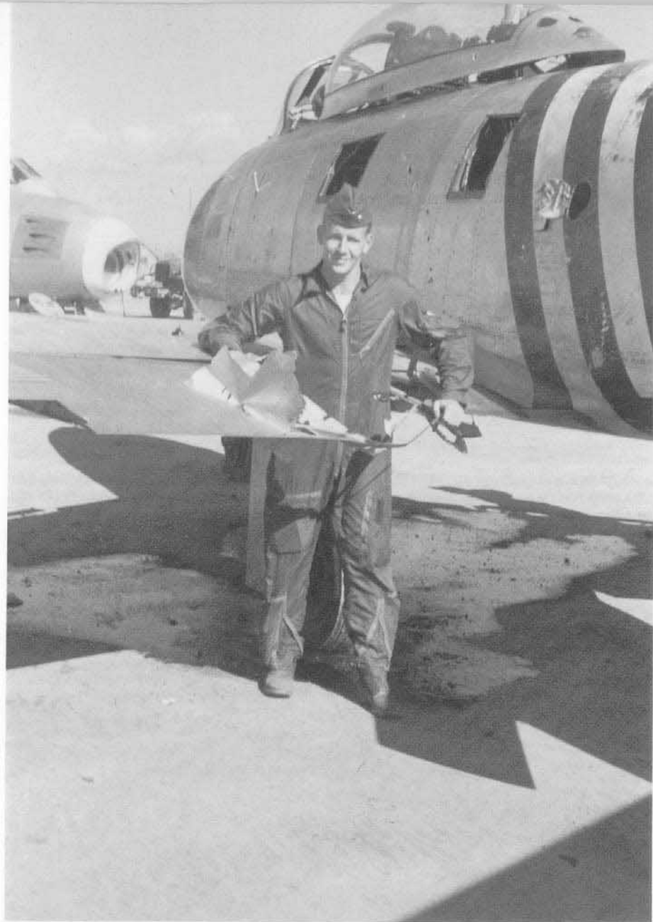
The F-86A could absorb a lot of battle damage. This 4th FIG pilot is standing in what was left of his port flap after one hit from a 37mm cannon shell from a MiG-15. The Sabre still made the 200 mile flight back to Kimpo despite losing almost two thirds of the flap. (Robert L. McKinney)
