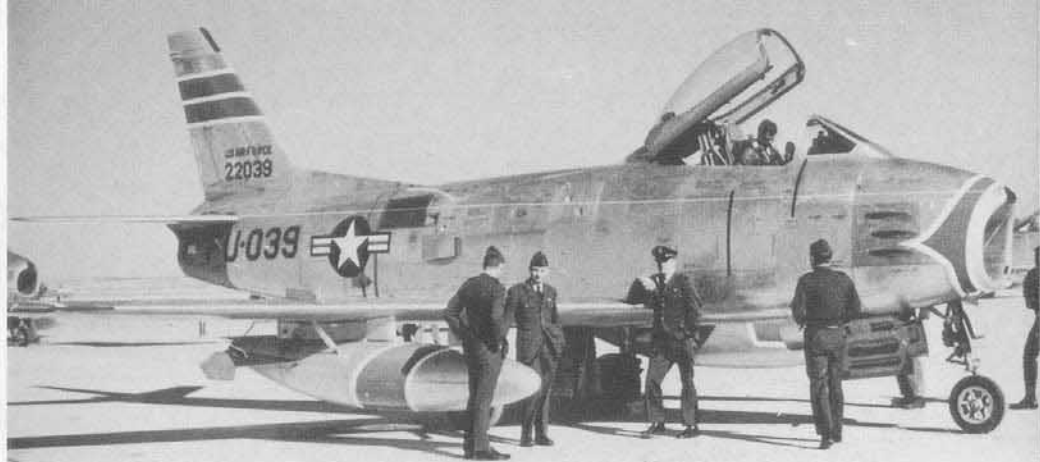
An F-86H-1 of the 312th FBW based at Clovis AFB, New Mexico during 1954. Initial production aircraft had the '6-3' wing with fences, which was later replaced by the F-40 wing with slats. The F-86H was atomic capable and could toss bomb the 1,200 pound "special store" using the LABS system. (COL E.M. Hanley)
