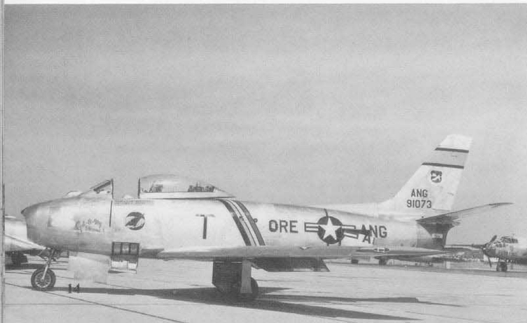
Gal-O-My Dreams was an F-86A-7 flown by LTCOL S.C. Austin when he commanded the 123rd FIS/Oregon ANG at Portland in 1955. The F-86A-7 was an F-86A that had undergone overhaul at Fresno and was modified with an AN/APG-30 radar and A-1CM gun sight. (Brian Baker)
