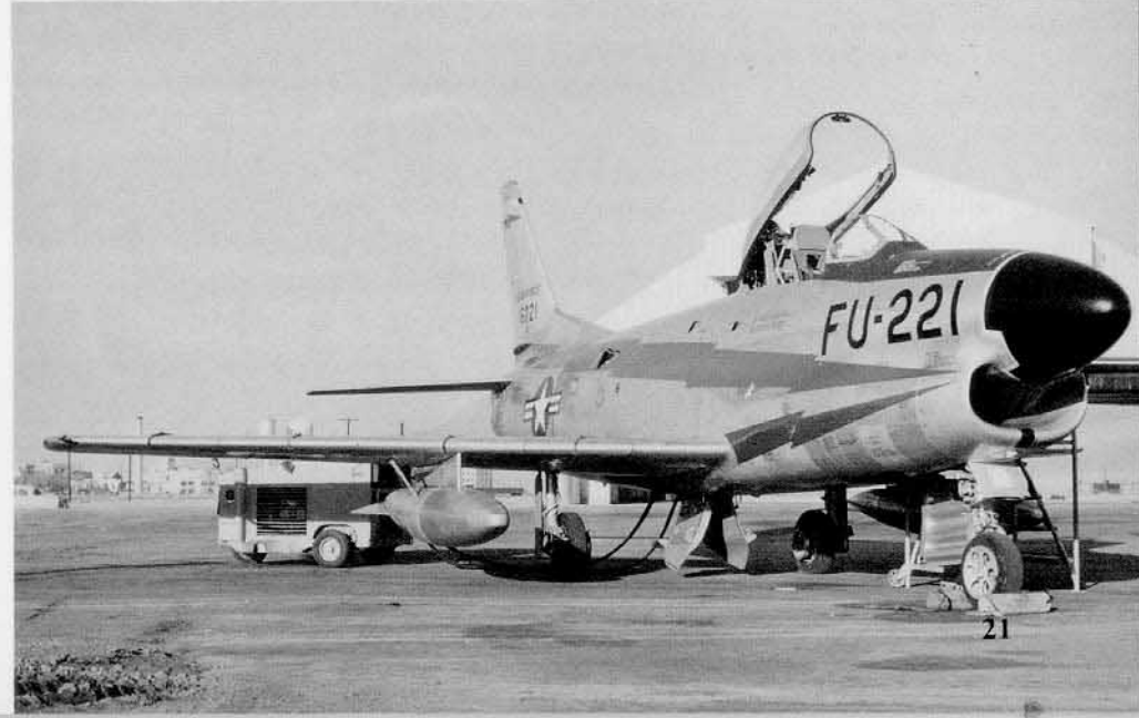
An F-86D-35 of the 93rd FIS at Kirtland AFB, New Mexico in 1957. The D-35 replaced the older radar with an omni-directional radar set. The lightning bolts on the fuselage and the wingtips are in Red. (USAF)
