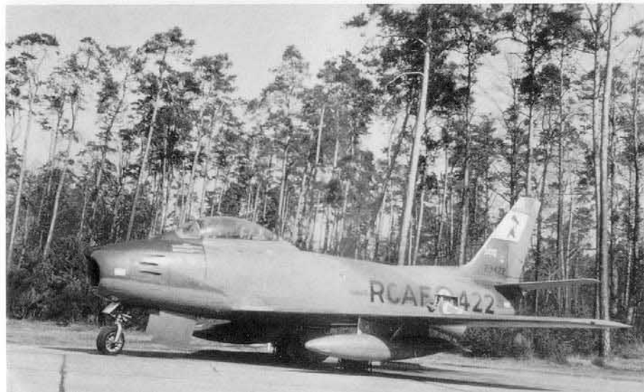
An RCAF Sabre Mk 6 of No 422 Squadron at Baden-Sölligen during 1962. The Mk 6 differed from earlier Sabre variants in having a 7,275 lbt Orenda 14 engine. The Mk 6 was the last Canadair Sabre produced and was widely exported. (Brian Baker)
