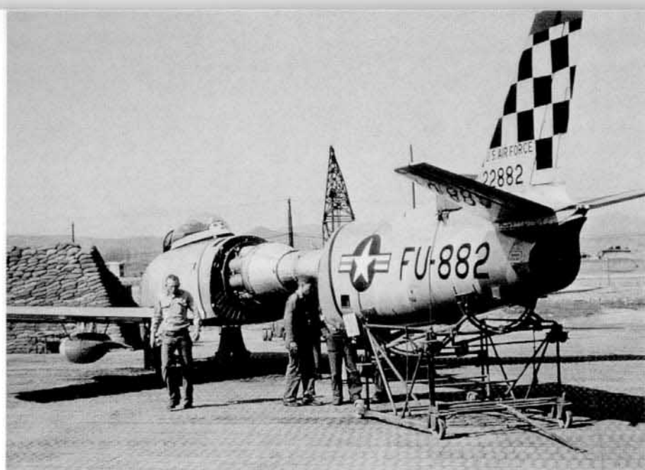
This F-86E is undergoing an engine change. The rear fuselage has been pulled away at the "break point" and placed on a special cart. The Sabre was assigned to LT Henry Buttlemann who became the youngest ace of the war when he shot down his fifth MiG on 30 June 1953. (COL Henry Buttlemann)
