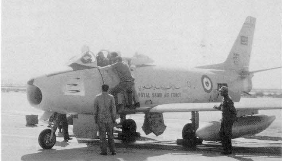
The Royal Saudi Air Force was equipped with F-86F fighter bombers taken from USAFE inventories and fitted with the F-40 wing. U.S. maintenance instructors show a Saudi pilot and crew chief the workings of the Sabre cockpit at Riyadh in November of 1966. The aircraft was overall Light Gray with Green lettering. (Frank McDonald)
