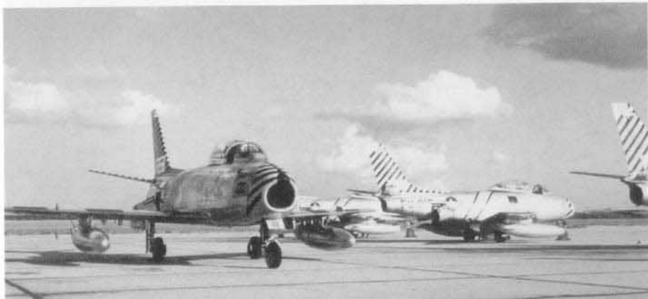
A Black and Yellow striped F-86F-30 fighter bomber of the 391st FBS/366th FBW taxis past Sabres of the 389th FBS at Alexandria AFB, Louisiana. The F-86F-30 had two additional underwing pylons for carrying bombs or fuel tanks. (NAA)
