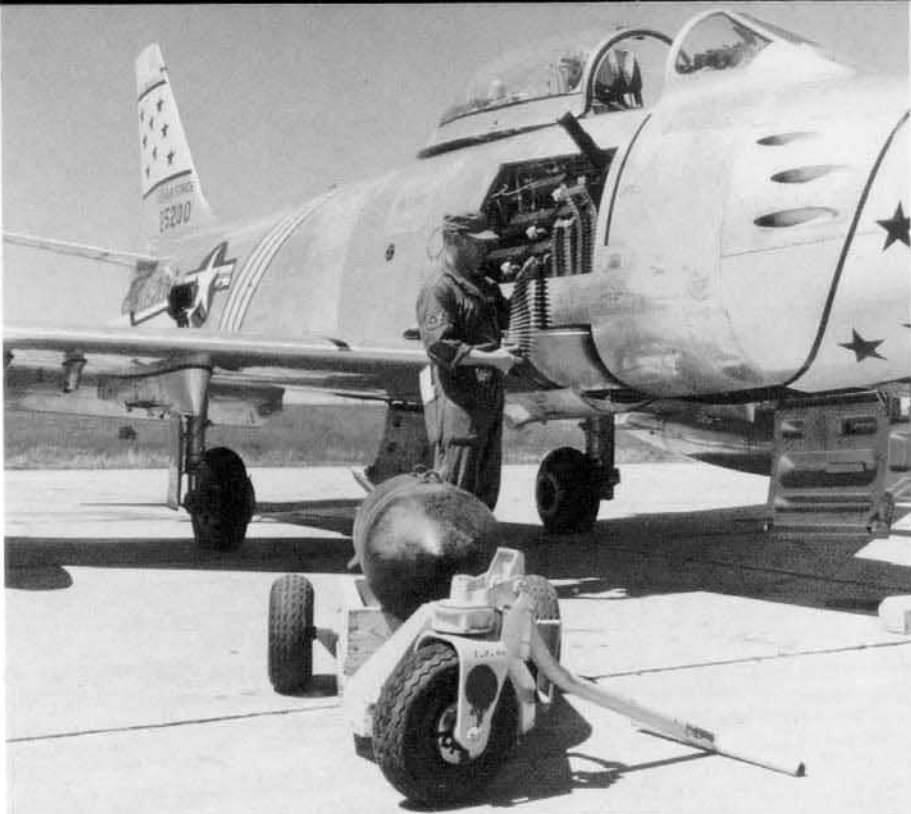
An F-86F of the 531st Fighter Bomber Squadron/21st Fighter Bomber Wing is rearmed with .50 caliber ammunition. The bomb in the foreground is a 500 pound GP bomb and will be loaded on the inboard wing pylon in place of the usual drop tank. (NAA)
