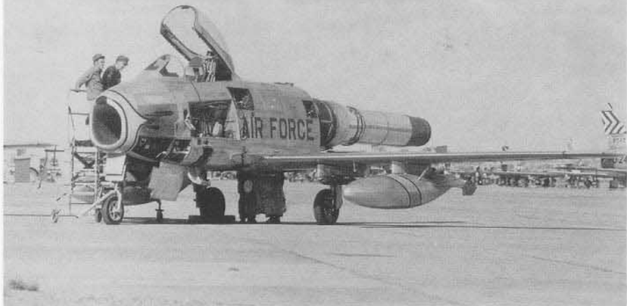
Ground crewmen work on a completely stripped F-86H of the 474th Fighter Bomber Wing on the open ramp at Clovis AFB. The J73-GE-3 engine was much larger than the J47 and was rated at 8,900 pounds dry thrust. Like the earlier F-86Ds, the F-86H used a clamshell type canopy. (NAA)
