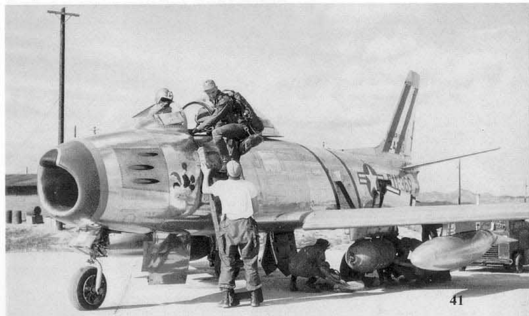
Armorer's prepare to load a M117 1,000 pound GP bomb on the inboard pylon of The Georgia Peach , an F-86F-30 of the 36th Fighter Bomber Squadron/8th Fighter Bomber Wing at K-13, Korea during June of 1953. (USAF)
