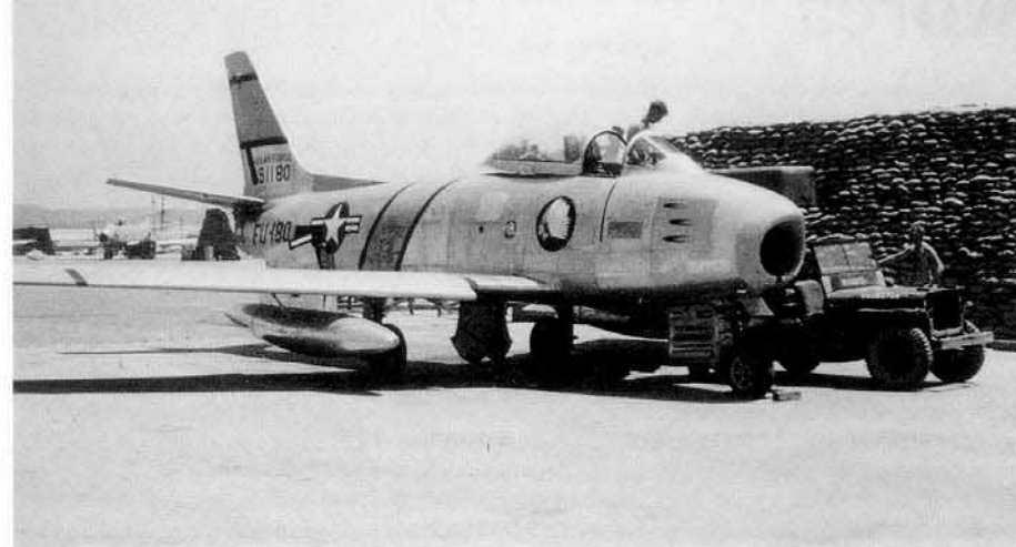
LITTLEBUTCH , an F-86A of the 335th FIS, carries the markings adopted by the 4th FIW during 1952. The Black and Yellow FEAF ID bands were carried on the wings and fuselage, with another Black/Yellow band on the tail to denote an aircraft assigned to the 4th. (Karl Dittmers)
