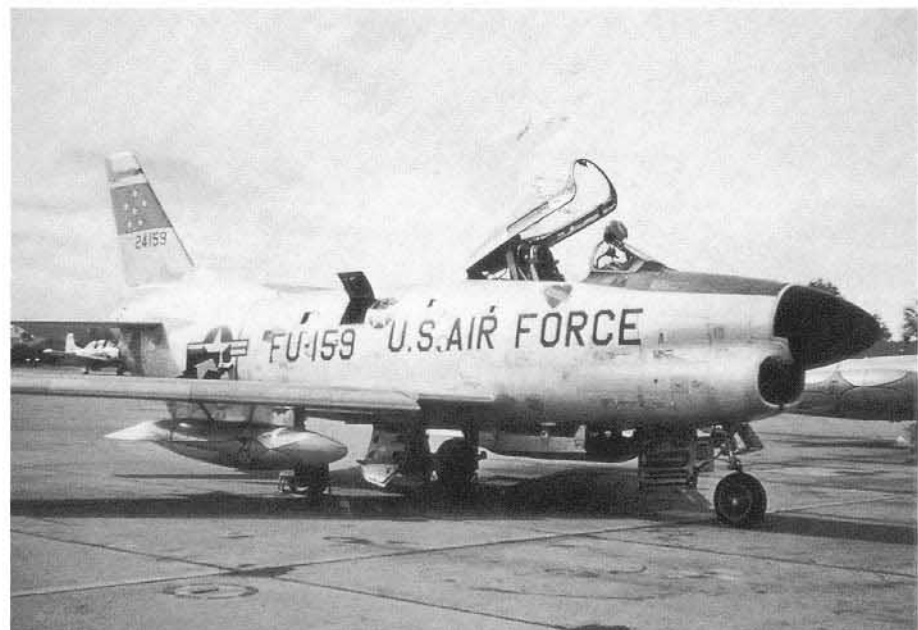
An F-86D of the 5th FIS on the ramp at McGuire Air Force Base, New Jersey. The flying A on the drop tank identified this aircraft as being part of A flight. The 2.75 inch FFAR rocket tray is in the lowered or firing position. (LCOL E. Bosetti)
