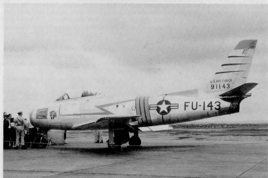
This F-86A was assigned to the squadron commander of the 60th Fighter Interceptor Squadron at Westover Air Force Base, Massachusetts during 1951. The wing leading edge slats and trailing edge flaps are fully deployed. (Jim Sullivan)
