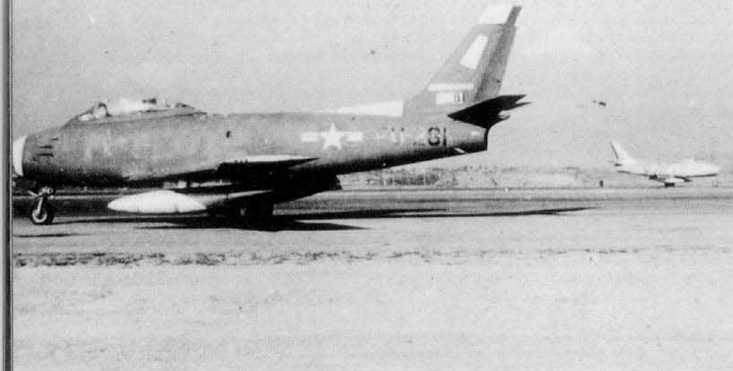
During the Summer of 1951 several F-86As, RF-80s and AT-6s had their upper surfaces painted Olive Drab in an attempt to camouflage them from the higher flying MiGs. The experiment failed miserably and the painted Sabres actually stood out more than a natural metal aircraft. The paint cost some 20 mph in top speed. (Eiflein)
