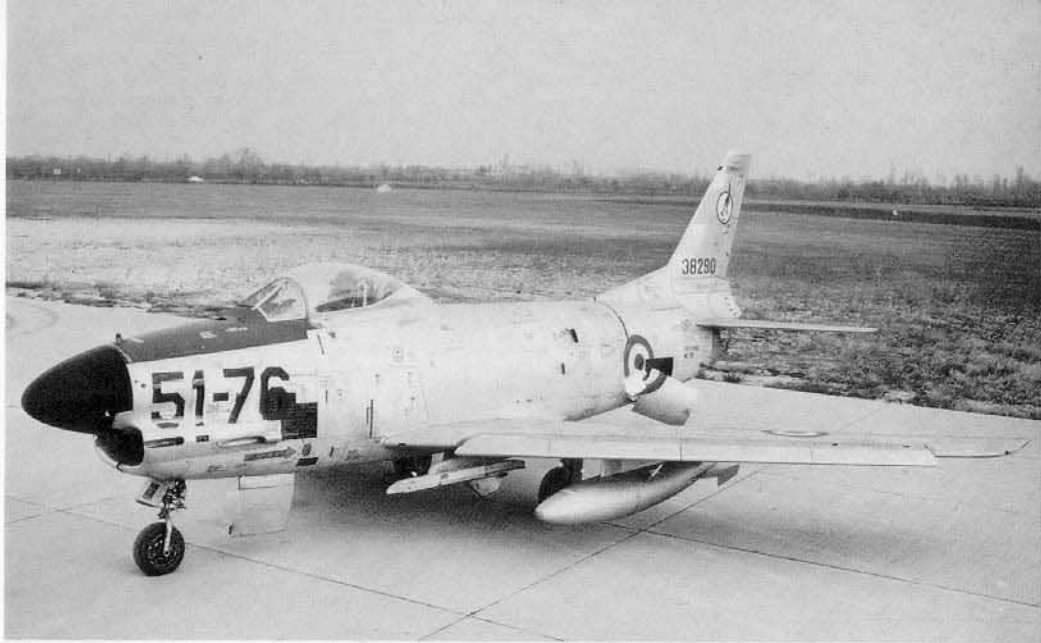
This Italian Air Force F-86K was part of the initial production batch of Fiat-built aircraft. Fiat built a total of 221 F-86Ks while North American built an additional 122. This aircraft has both the F-40 wing and Sidewinder missile rails. (IAF)
