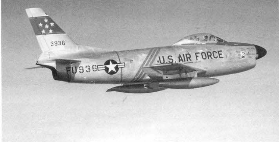
This F-86D-60 was flown by the commander of the 539th FIS at Stewart AFB, New York. The F-86D-60 featured improved radio equipment and other avionics and was the final production variant of the F-86D. (E. Sommerich)
