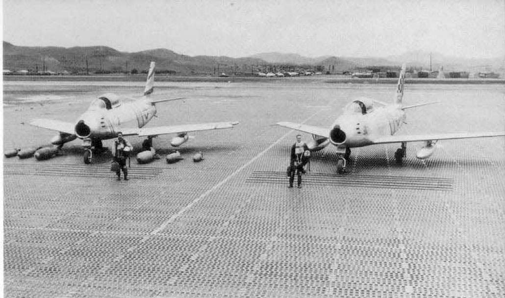
An F-86F-30 flown by the commander of the 8th FBW, COL Walter Benz is displayed next to an F-86F-10 flown by COL George Ruddell. The F-30 is carrying "Misawa" drop tanks (made in Japan) while the F-10 is carrying the original NAA combat drop tanks. (NAA)
