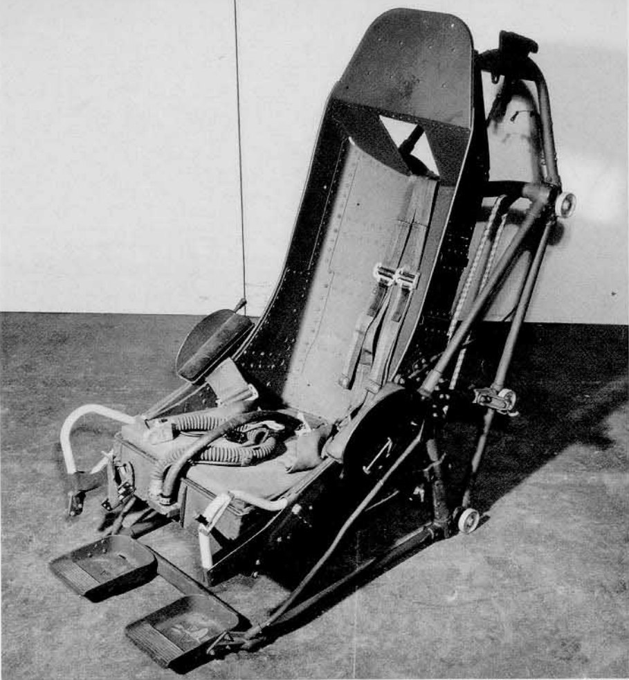
The North American ejection seat used in the F-86D series was different from the type of seat used in the F-86 day fighter variants. (NAA)
