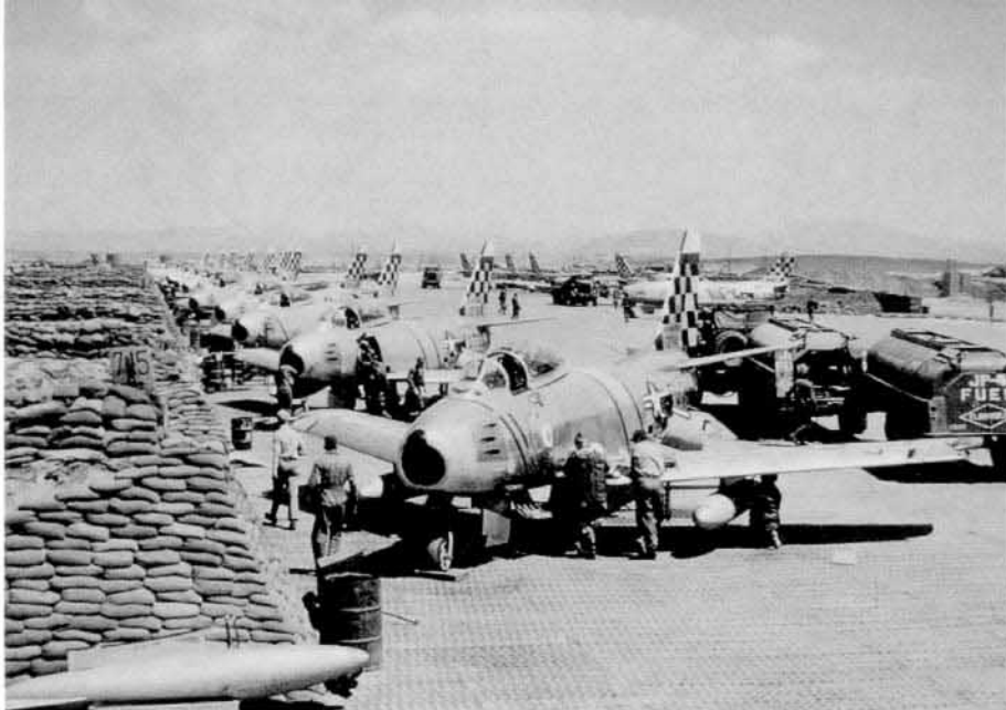
Pilots man their F-86Es of the 25th FIS on the flight line of Suwon Air Base, Korea during the Spring of 1953. The aircraft in the foreground is an F-86E-10 with an optically flat armored windscreen. (COL Hank Buttleman)
