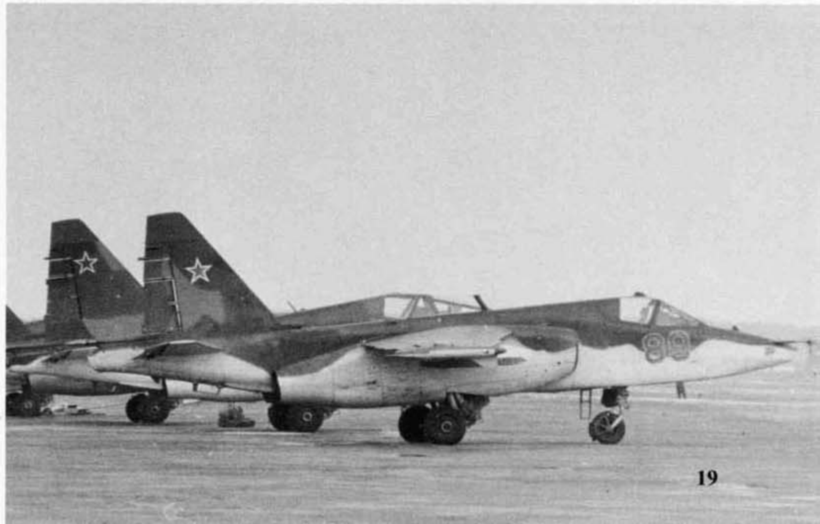
Several Frogfoot As share the ramp at their home base with a Frogfoot B trainer. The trainer has a taller fin and shorter rudder than the Frogfoot A. Normally, there are several trainers (either Frogfoot Bs or L-39s) assigned to each attack regiment. (A.A. Zirnov)
