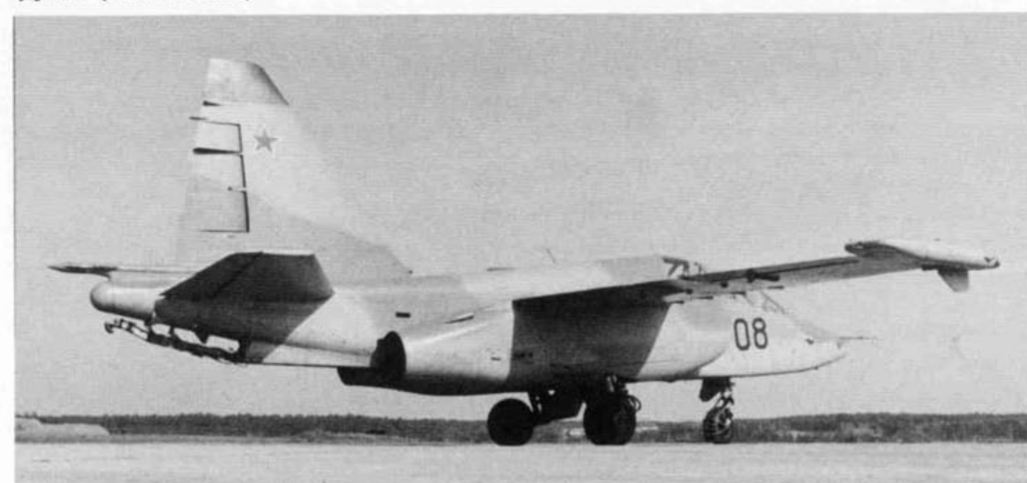
The installation of the arrestor hook led directly to the aircraft's designator Su-25UTG since the G stood for Gak or Hook. The naval trainer carried no internal armament or underwing pylons (Sukhoi OKB)
