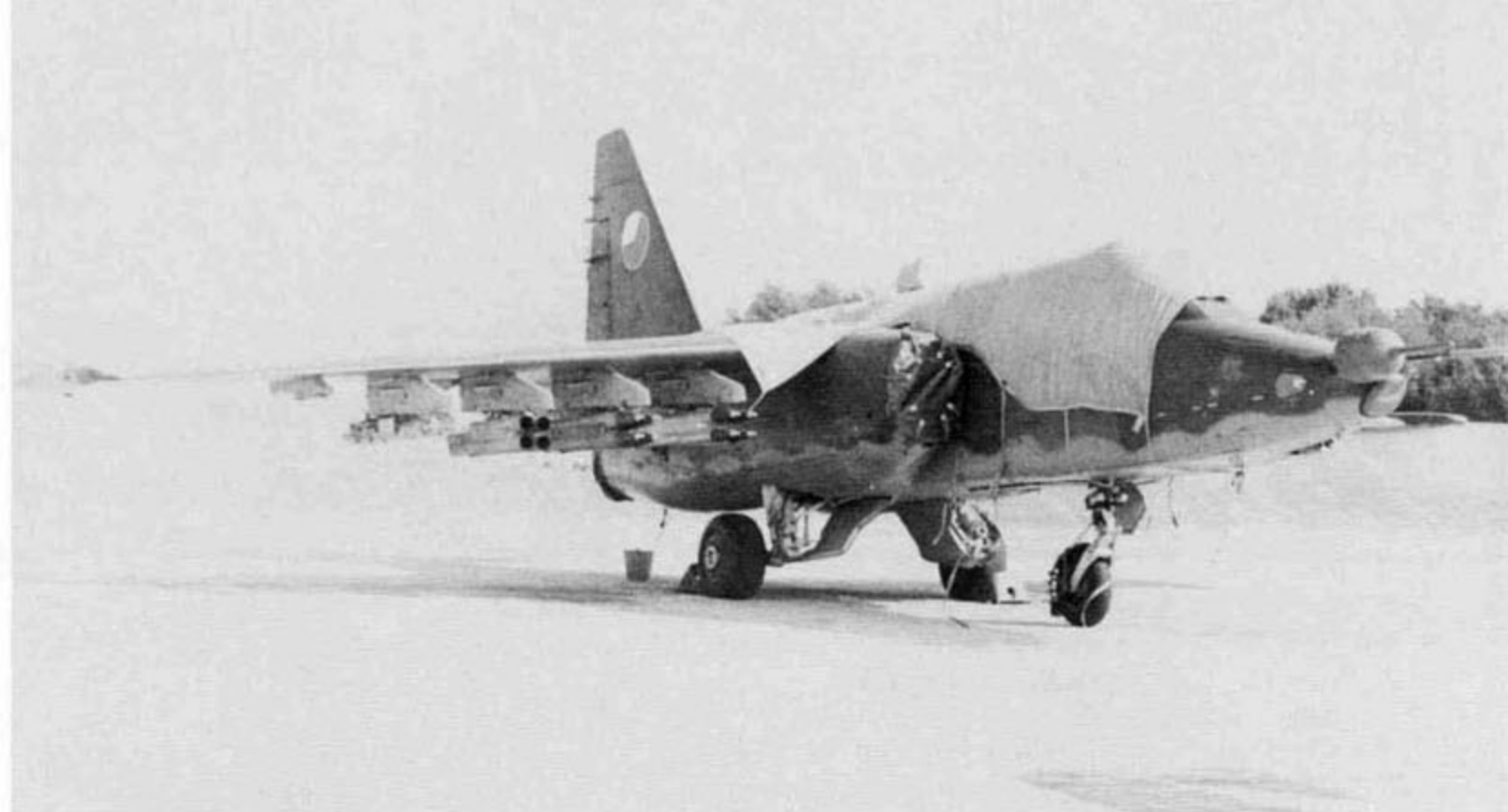
This early Su-25K has the air data sensors and laser range finder/designator window covered by Red protective covers. The RM-122 four tube rocket launchers on pylons one, two and three are for S-13 unguided air-to-ground rockets. (Antonin Fidransky)
