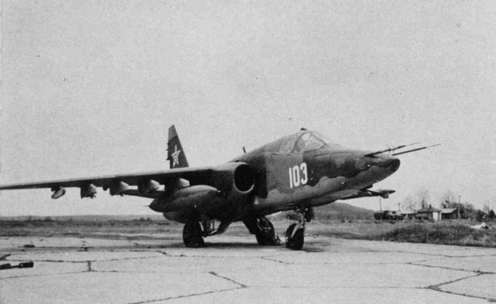
A Bulgarian Air Force Su-25K, White 103, on the ramp at Bezmier Air Base in central Bulgaria. This Frogfoot A carries no ordnance, but is equipped with the usual PTB-1150 fuel tank. The national markings were applied on the lower wing surfaces and on the stabilizer. (Wojciech Luczak)
