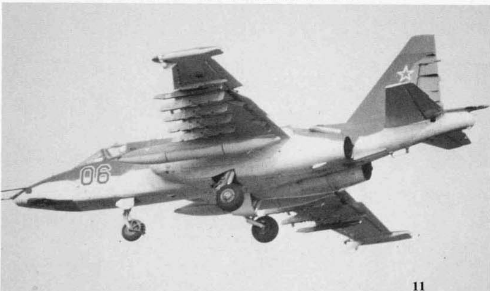
After the end of the Afghanistan War, a number of T-8s were assigned to the 368th ShAP at Demmin-Tutow, Germany. The large cooling air intakes on the late preproduction T-8 are unique to this variant and were not used on production Su-25s. (Jens Schymura)
