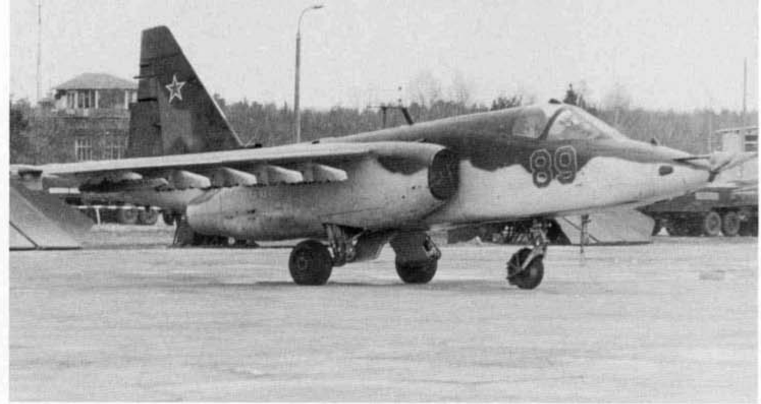
This Su-25 Frogfoot A, Red 89, has the air intakes covered by Red protective covers designed to keep foreign object out of the intake while the aircraft is parked. (A. A. Zirnov)
