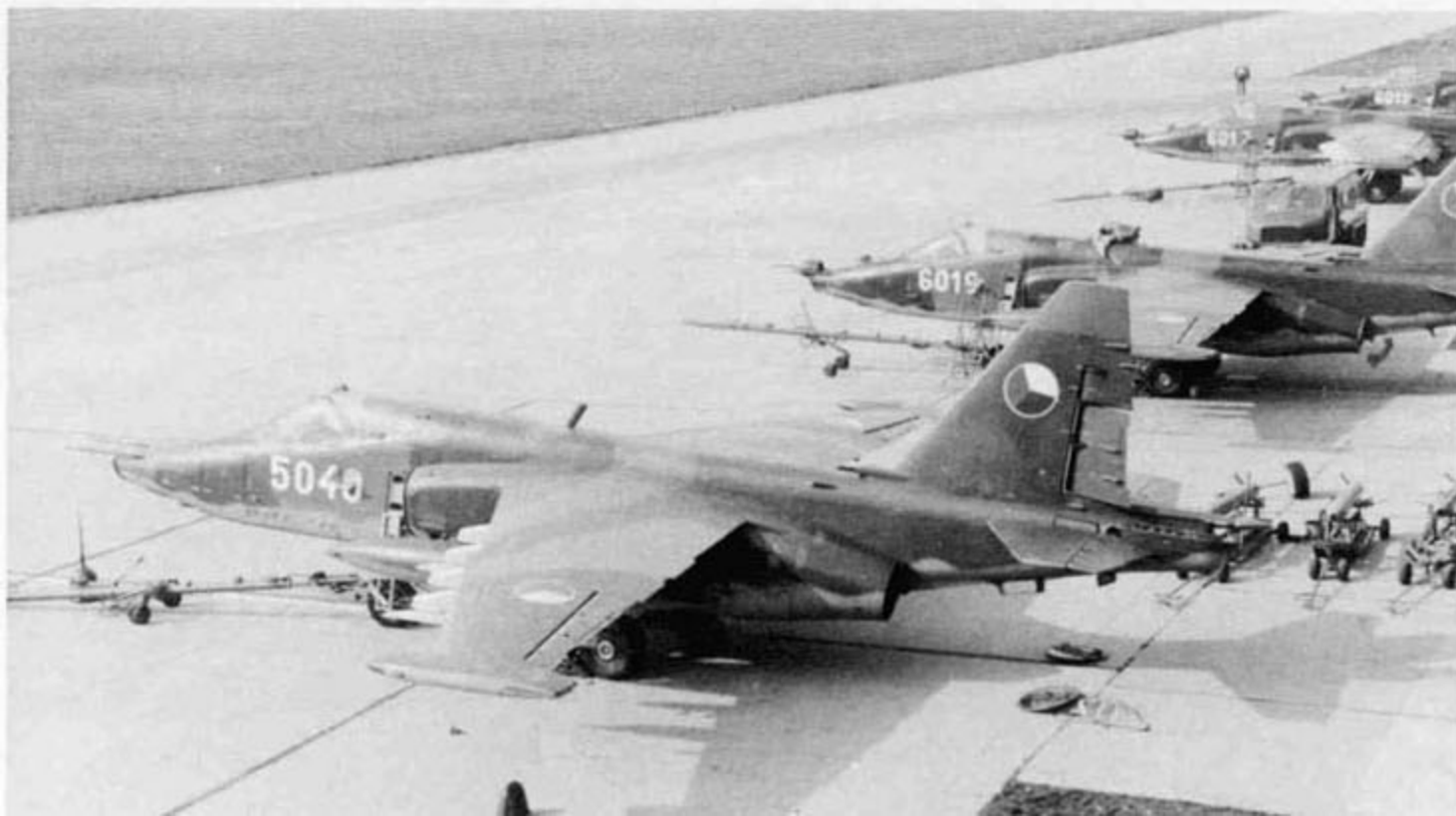
A lineup of four early production Su-25Ks, White 5040, White 8018, White 6017 and White 8019 of the 1st Squadron, 30th Attack Regiment, Czech Air Force. The aircraft in the foreground, White 5040, is equipped with APU-68-UM2 rails on pylons two and four to carry the S-240 unguided air-to-ground rockets which are on the trolleys next to the aircraft. (Pavel Polach)
