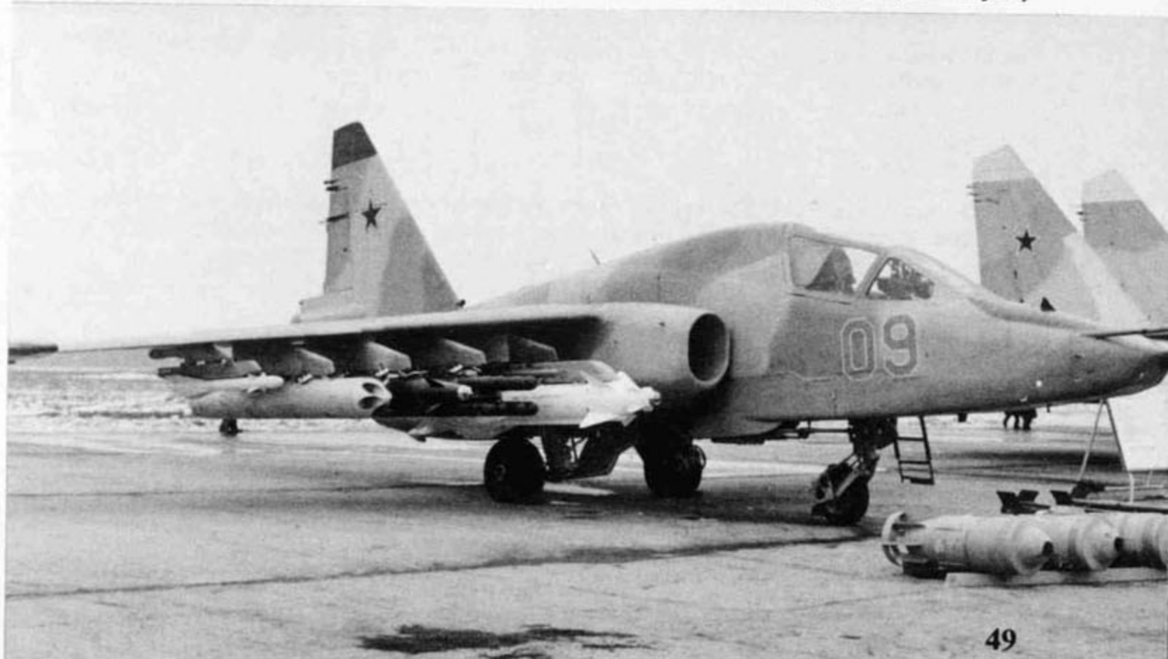
The Su-25TM, Blue 09, on display armed with an AS-14 Kedge on the inboard pylon, PTUR Vikhr anti-tank missiles on the next pylon, an AS-10 Karen on pylon three, a four shot B-13L rocket pod for S-13 rockets and a R-60 (AA-8 Aphid) on the outboard pylon. (D. Grinyuk)
