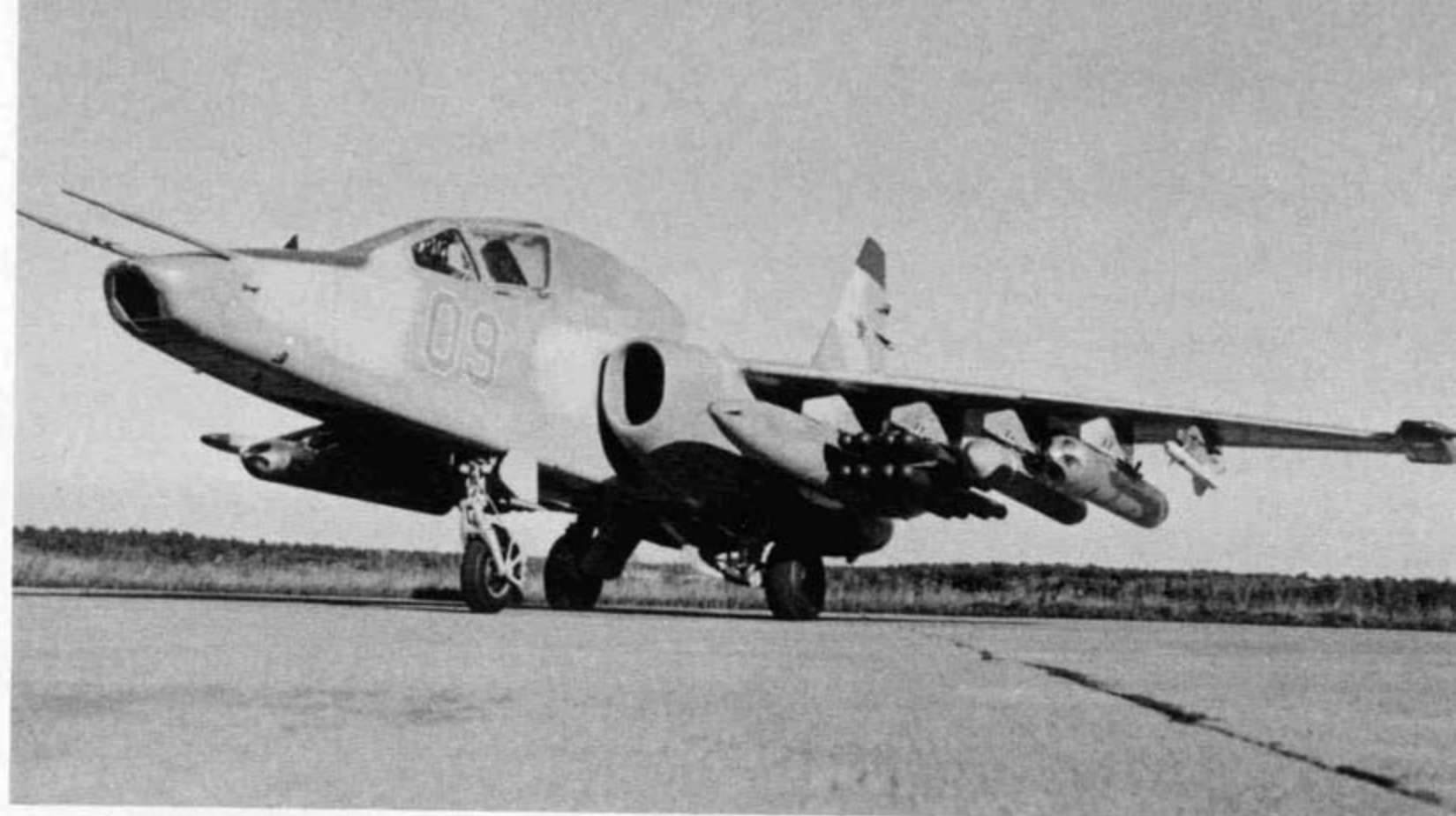
The Su-25TM prototype on the ramp at the Zhukovski Flight Test Center while undergoing factory tests. The aircraft is configured with underwing fuel tanks, PTUR Vikhr anti-tank missiles, S-25 unguided air-to-ground rockets, B-13L four shot rocket pods and R-60 (AA-8) air-to-air missiles (Sukhoi OKB)
