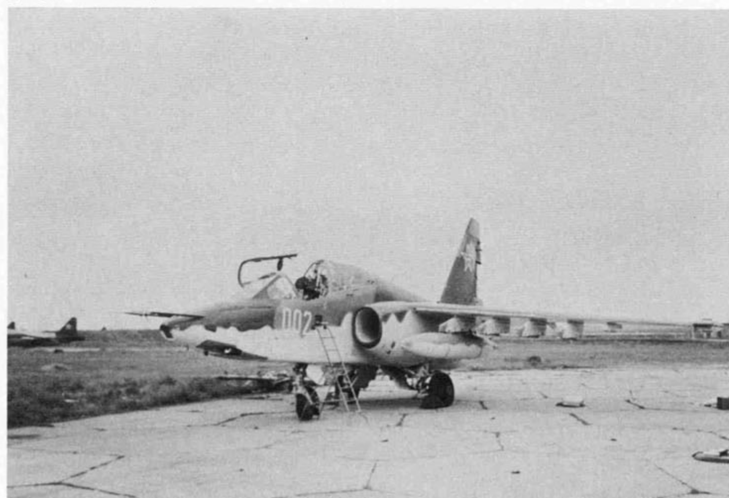
This Bulgarian Su-25UBK, White 002, was one of four Frogfoot Bs purchased by Bulgaria for pilot training. The tactical number, 002, is White with a thin Blue outline. This is an early production SU-25UBK with the early three pole Odd Rods IFF antenna in front of the canopy. (Wojciech Luczak)
