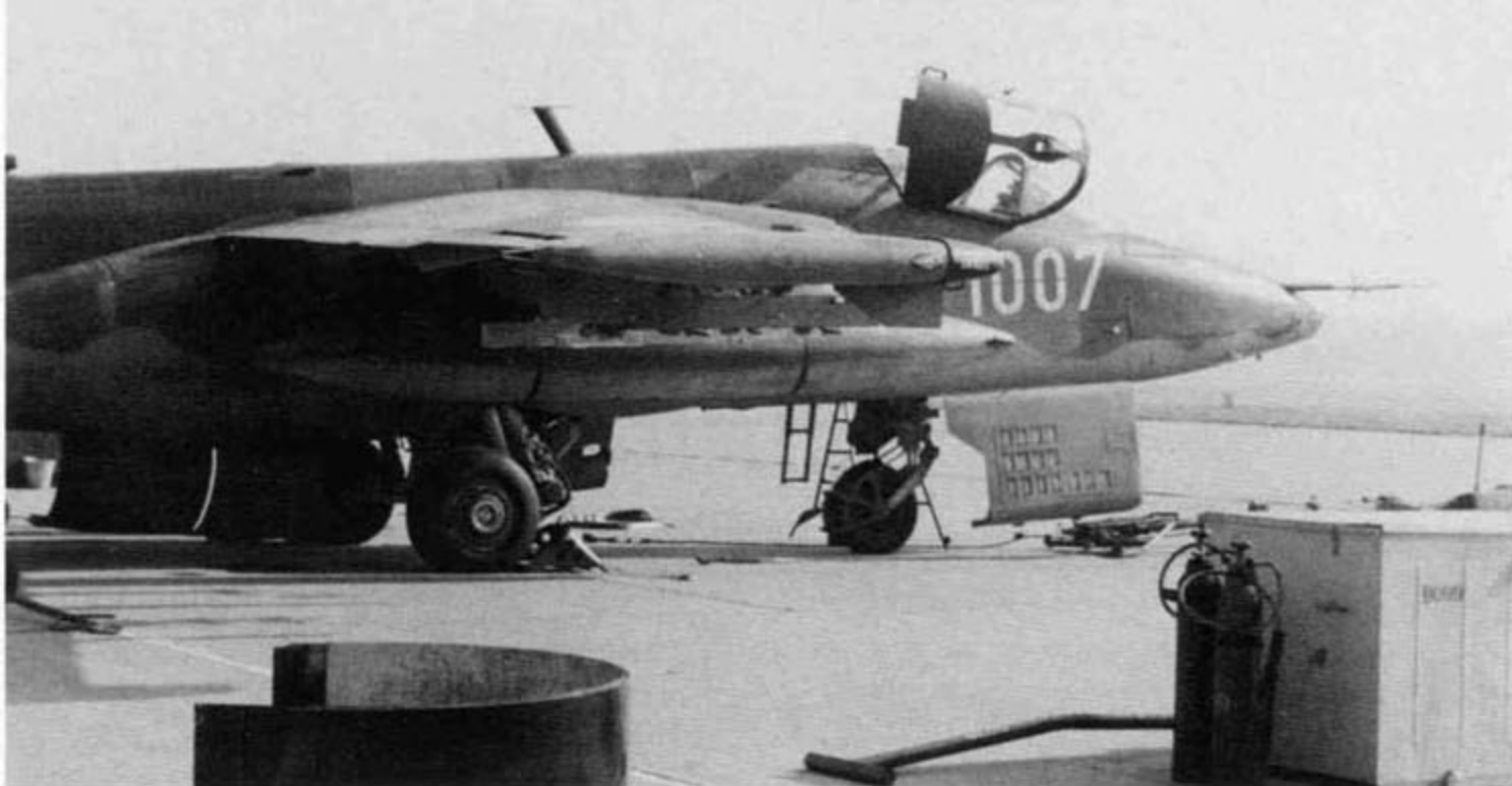
This Su-25K, White 1007, of the 3rd Squadron undergoes maintenance on the ramp at Pardubice. The equipment box, tow bar and fire extinguisher all carry the tactical number of the aircraft assigned to this parking spot, White 9099. White 1007 has the cannon ammunition bay hatch open as are several of the port engine bay hatches. (SIGN via Roman Sekyrka)
