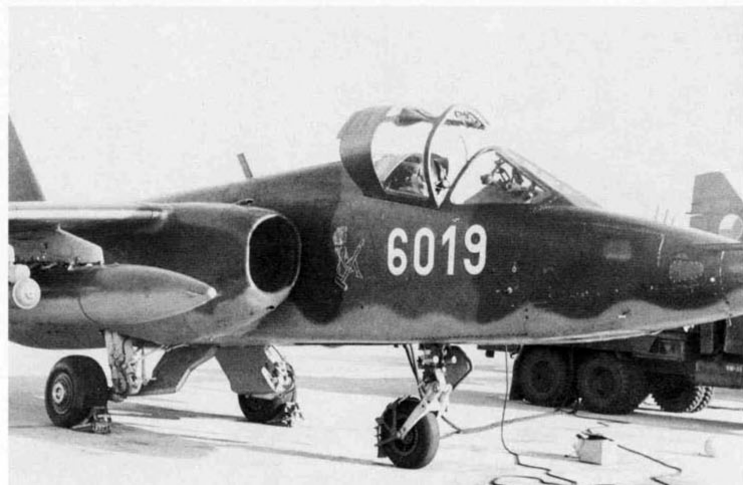
White 6019 has carried at least three different forms of nose art, including this White nude. All were in the same location on the fuselage and none lasted for a long time. The Frogfoot A is equipped with PTB-1150 drop tanks and an MBD-3 bomb rack with four FAB 100, 220 pound bombs. (Pavel Polach)
