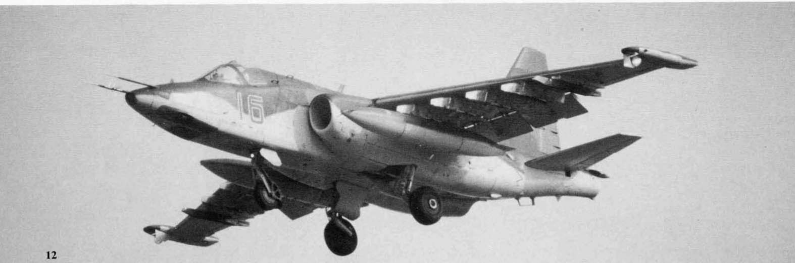
This T-8, Red 16, of the 368th ShAP, carries the same camouflage as the others assigned to the unit, although it also has Red warning triangles painted on the air intake and on the exhaust. The retractable landing lights on the wing tip pods are deployed for landing. (Jens Schymura)
