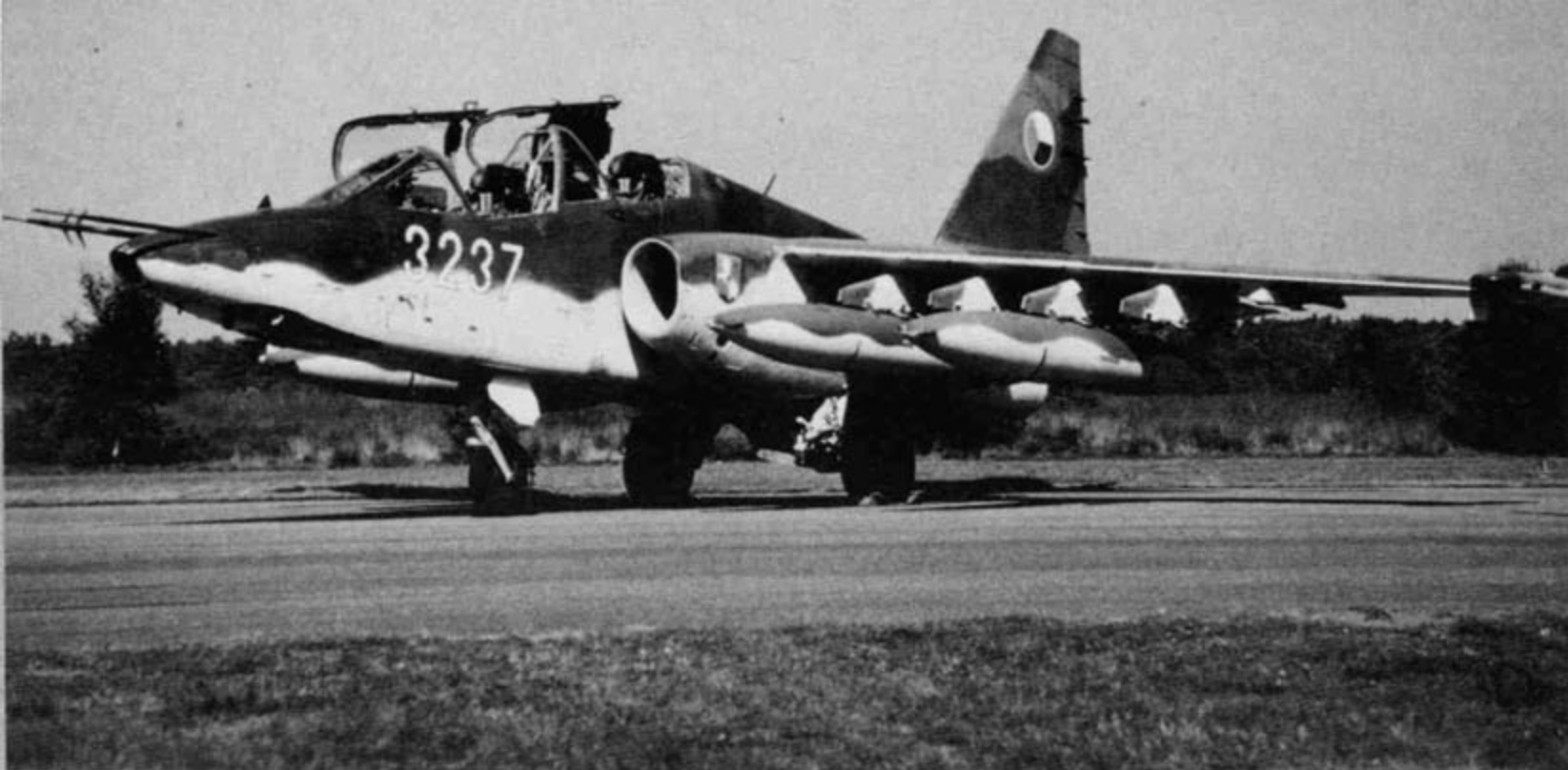
A Czech Air Force Su-25UBK, White 3237, on the ramp at Pardubice. The aircraft is in the standard ferry configuration with four PTB-1150 fuel tanks. The city crest of Pardubice is carried on the port air intake only. (Martin Baumann)
