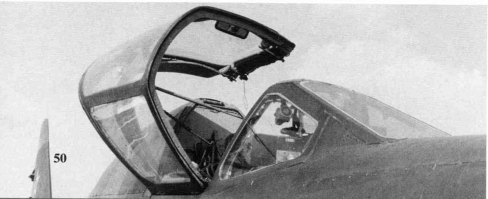
The canopy of the Su-25TM has the rear view mirror mounted on the inside canopy frame while the Su-25 Frogfoot A had the mirror in a fairing on top of the canopy. (Harry Wisch)
