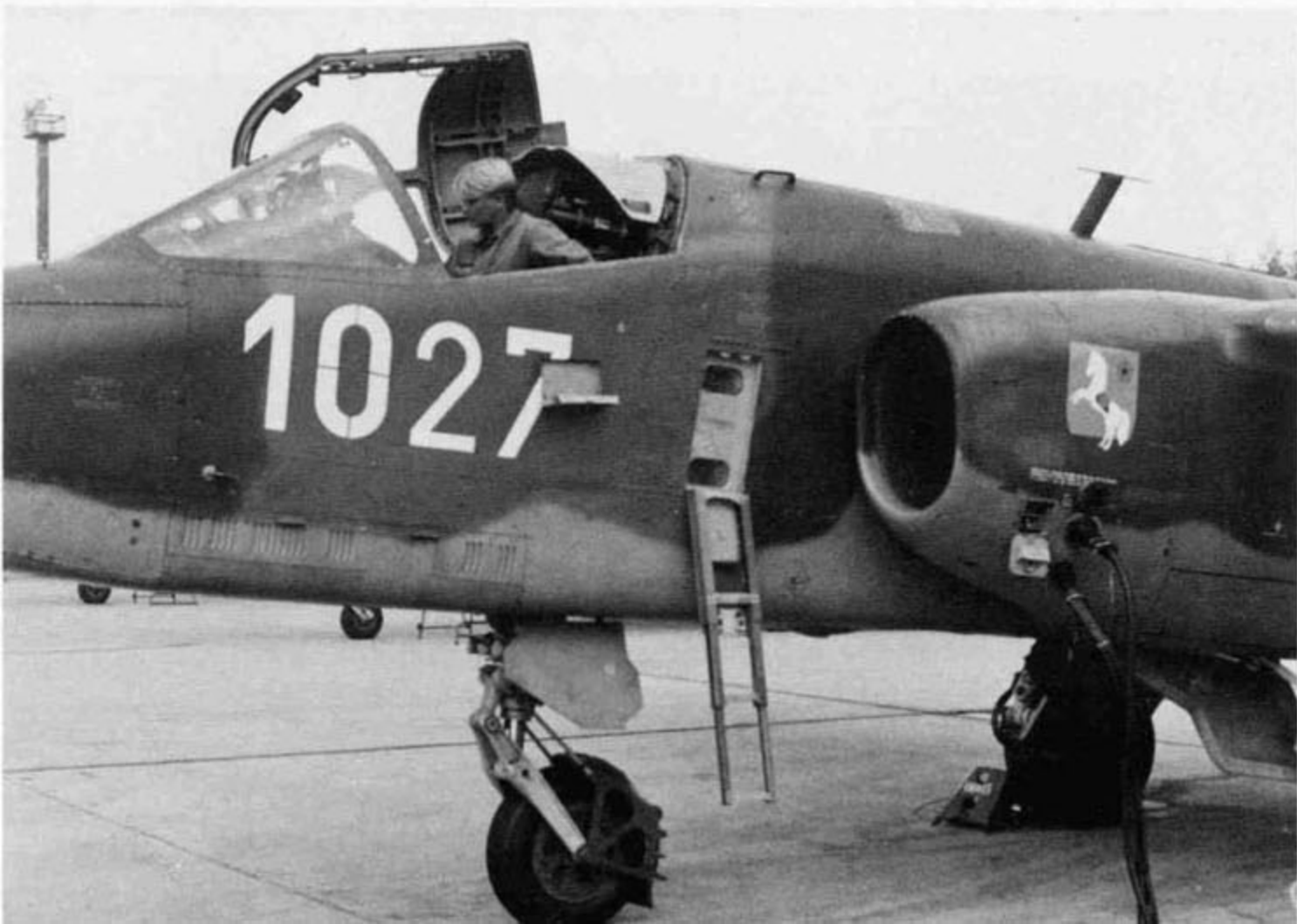
External power cords are attached to the external power outlets on this Su-25K, White 1027, of the Czech Air Force. The pilot's boarding ladder was fully retractable, folding up into the bay in the side of the fuselage. The aircraft carries the late style crest of Ostrava which has no White outline. (Jaromir Stepan/ZLINEK Magazine)
