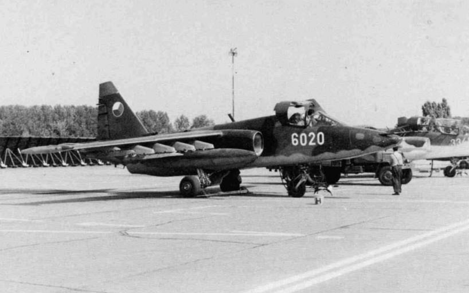
The Su-25K, White 6020, was the last Frogfoot A of production Batch 60 to be delivered to the Czech Air Force. The aircraft was assigned to the 1st Squadron, while the Su-25UBK two seat trainer, White 3348, was assigned to the 3rd Squadron. White 6020 carries an APU-68-UM2 rail for a S-24 240MM rocket on number three pylon and an APU-60-1M R-60MK AAM rail on the outboard pylon. (SIGMA via Roman Sekyrka)
