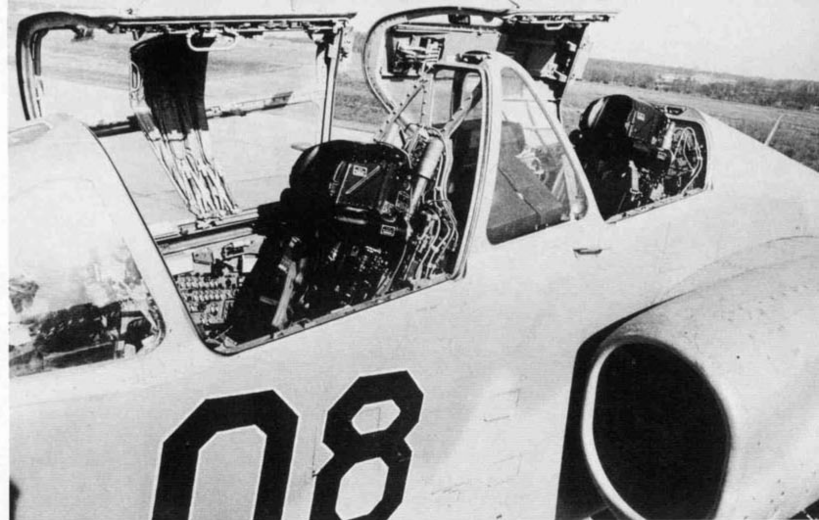
The Su-25UTG was equipped with K-36 ejection seats in both cockpits. To preserve cockpit pressurization in the event of a canopy failure, the cockpits each had their own system and were separated by an armor glass panel between the cockpits. (Sukhoi OKB)
