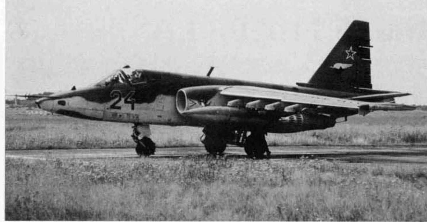
This Su-25, Red 24, of the 357th ShAP at Brandis, Germany is armed with an FAB-100 220 pound bomb on pylon number three and an empty UB-32A rocket pod on pylon number four. The aircraft carries a Grach emblem on the air intake duct just behind the Red warning triangle. (Rene van Woezik)
