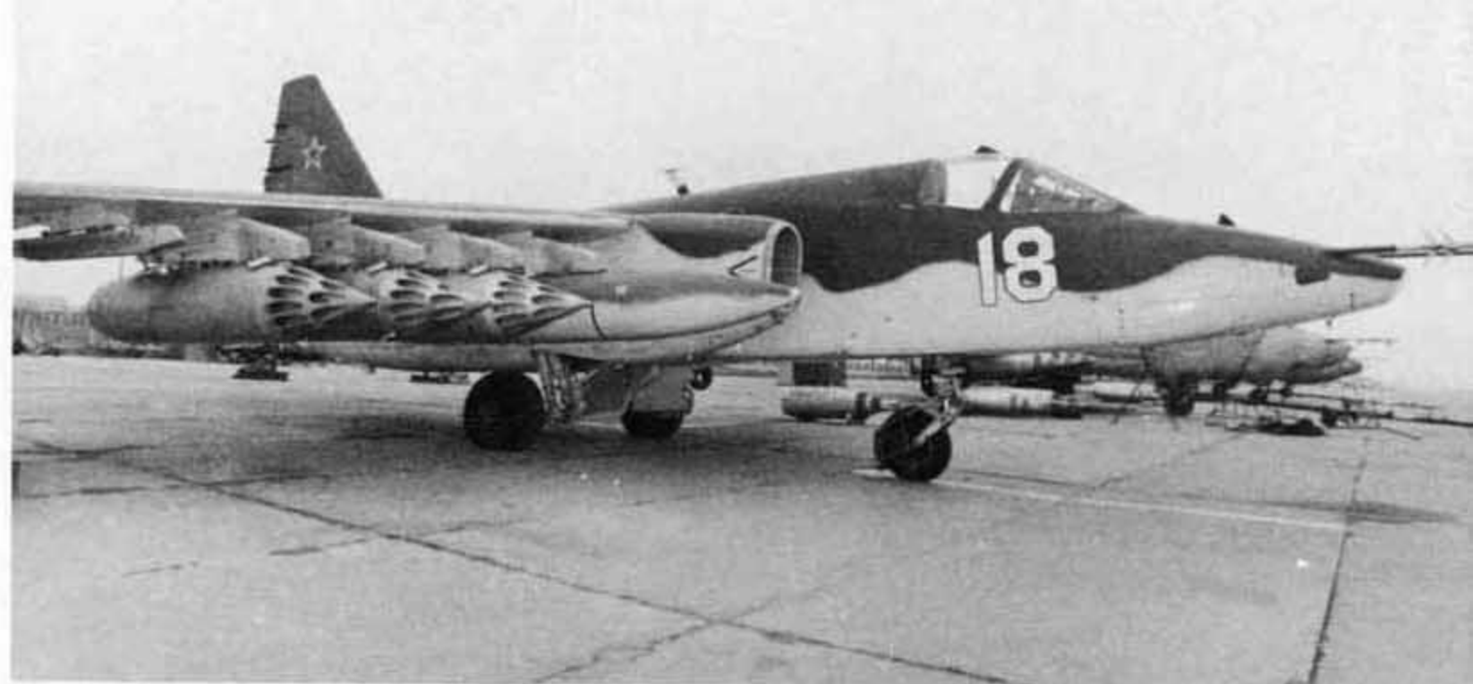
White 18, a Su-25 Frogfoot A of the 60th ShAP, was based at Sital-Zhay Air Base in Azerbaijan during February of 1990. The aircraft carries six B8M1 rocket pods, a typical load for a ground attack mission. The air intake warning triangle is in Black. (D. Grinyuk)
