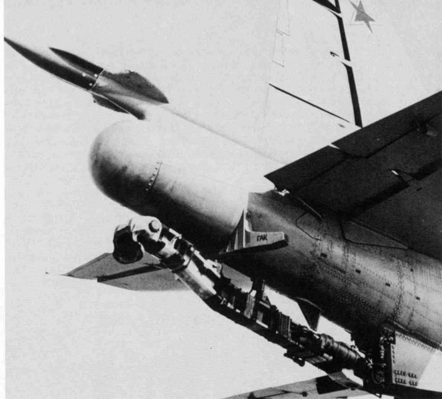
The arrestor hook on the Su-25UTG was a heavy unit. The braking parachute was deleted on the naval prototype and the container faired over. The antennas on the post above the arrestor hook are for the Sirena tail warning radar system (Sukhoi OKB)
