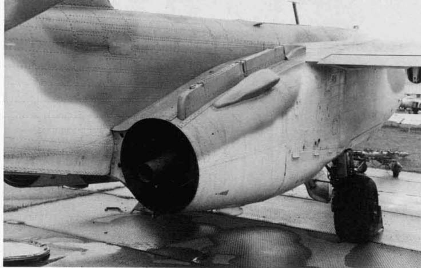
Because of the threat from Stinger missiles in Afghanistan, the Frogfoot A was modified to both reduce the IR signature and to provide some self defense from these missiles. A large cooling air intake was installed on the upper rear engine nacelle along with a smaller intake at the bottom of the nacelle. A cooling tube was installed in the exhaust stream and ASO-2V chaff/flare dispensers were fitted to each side of the nacelle. (Harry Wisch)
