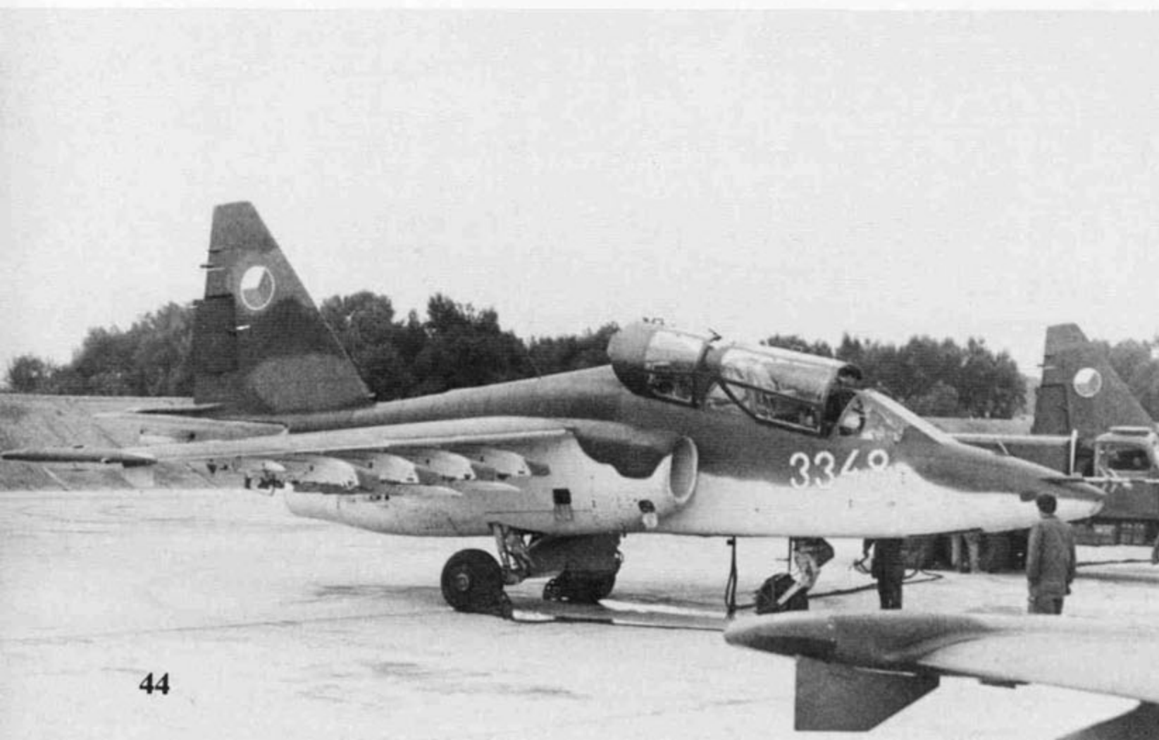
White 3348 is refueled and serviced on the apron at Pardubice. The aircraft is configured with APU-68-UM2 missile rails on the number two and three pylons. The Su-25UBK is fully combat capable and can carry the same weapons as the single seat Su-25K. (Pavel Polach)
