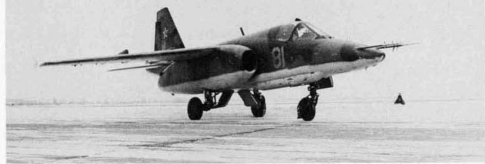
The T-8-1 prototype, Yellow 81, carried no underwing pylons and had the cannon mounted in a gondola under the starboard side of the nose. The wing had two wing fences, with the larger fence being outboard on the wing. (Sukhoi OKB)
