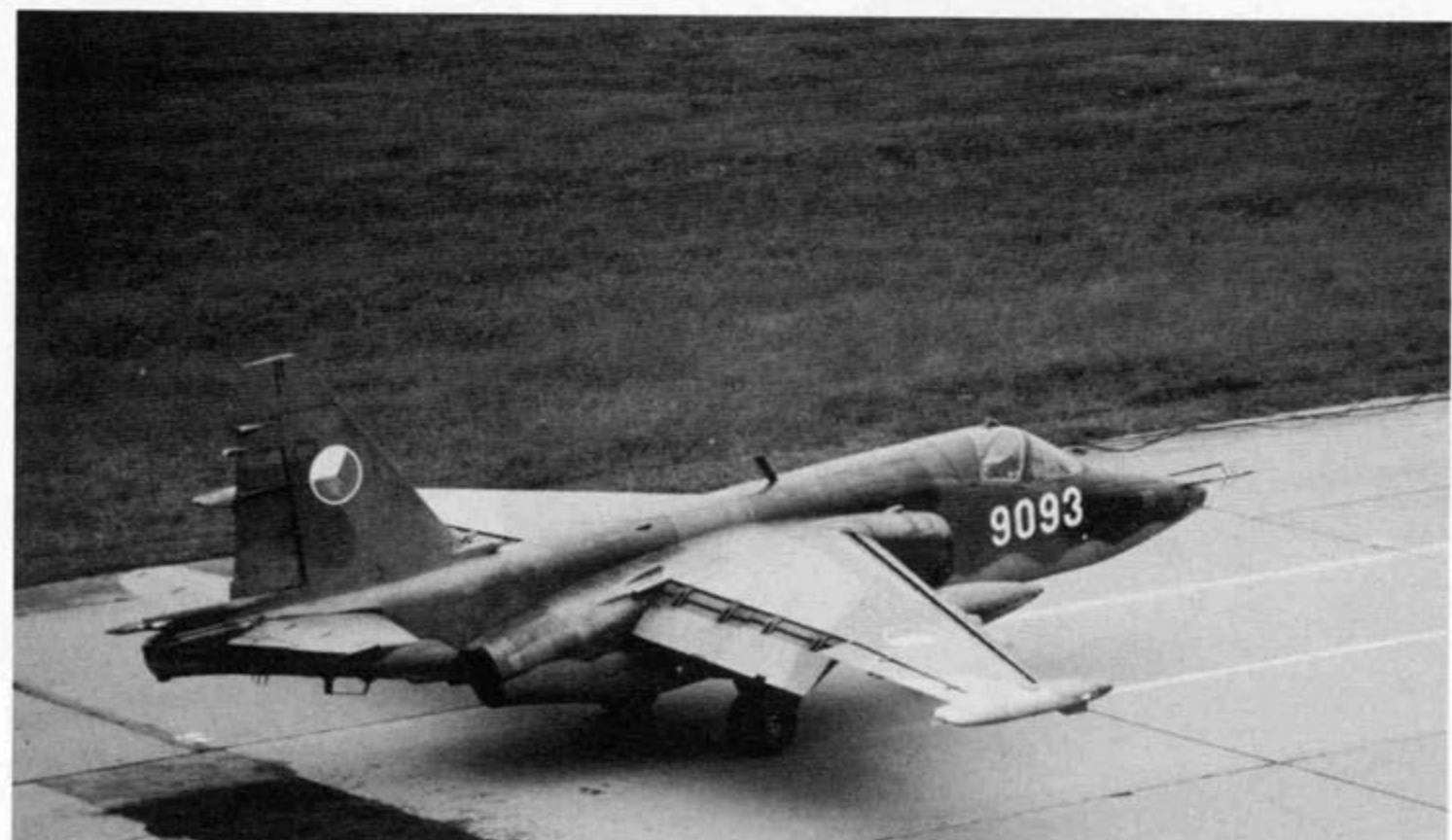
An Su-25K, White 9093, rolls out at Pardubice with the flaps lowered and the speed brakes closed. This aircraft belongs to the 3rd Squadron, 30th Attack Regiment, and was delivered in the Summer of 1987. The tactical number is in the later stencil style. (SIGN via Roman Sekyrka)
