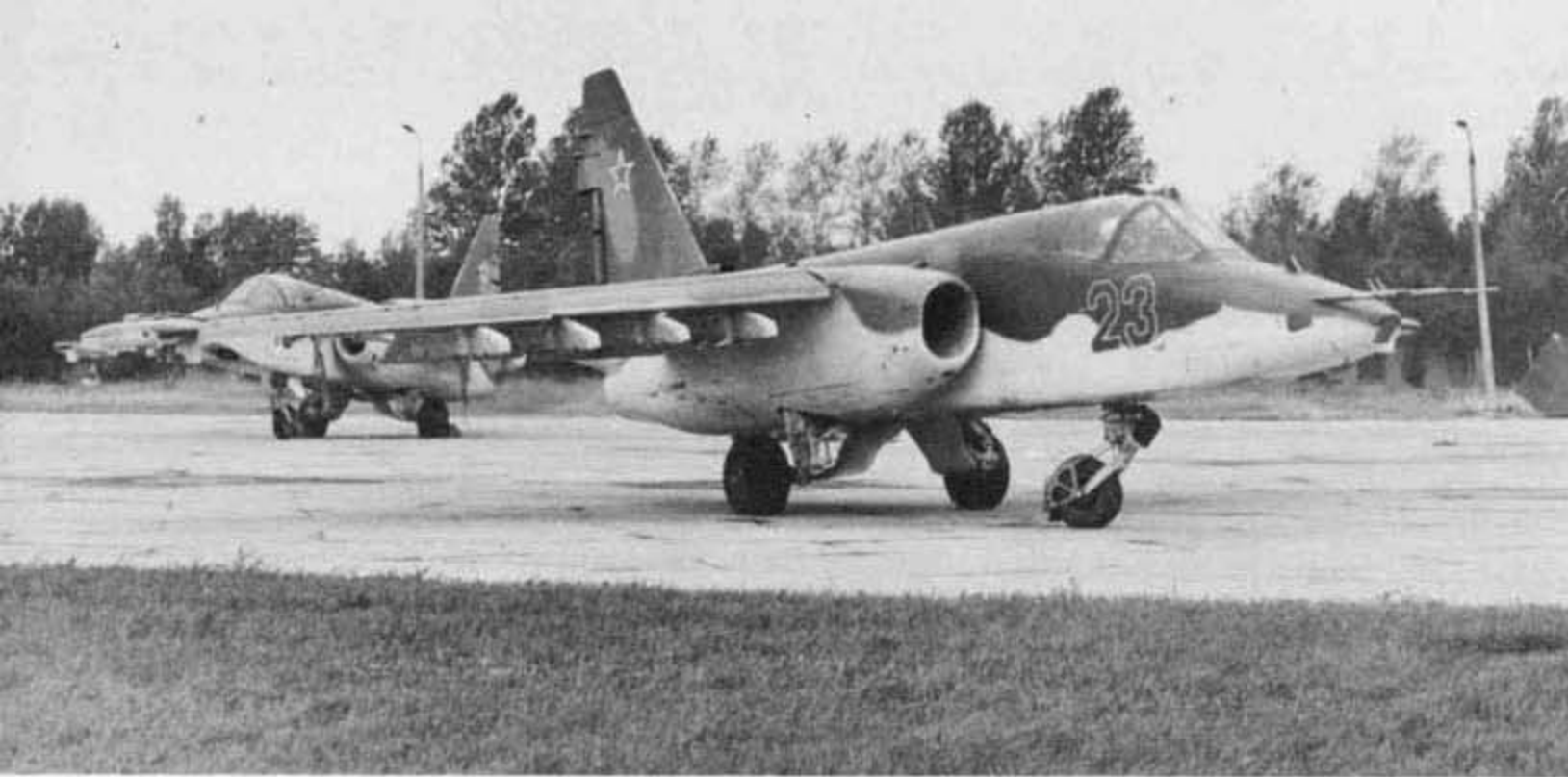
An Su-25 Frogfoot A, Red 23, taxis off the ramp of its home base for a training mission. The tactical number on the nose has a thin White outline and the aircraft is equipped with the later blade style IFF antennas. (A.A. Zirnov)
