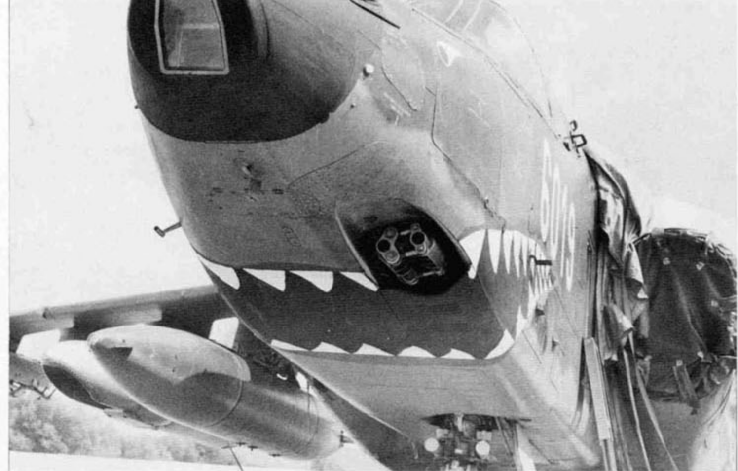
Early Su-25s and Su-25Ks had a two piece muzzle on the AO-17A twin barrellled 30mm cannon. The gun was offset to port with the ammunition supply (250 rounds) on the starboard side. This Czech Su-25K, White 6019, also has an SPPU-22 twin barrellled 23mm cannon pod on the number two pylon. The pod contains a GSh-23 cannon and 260 rounds of ammunition. (Pavel Polach)
