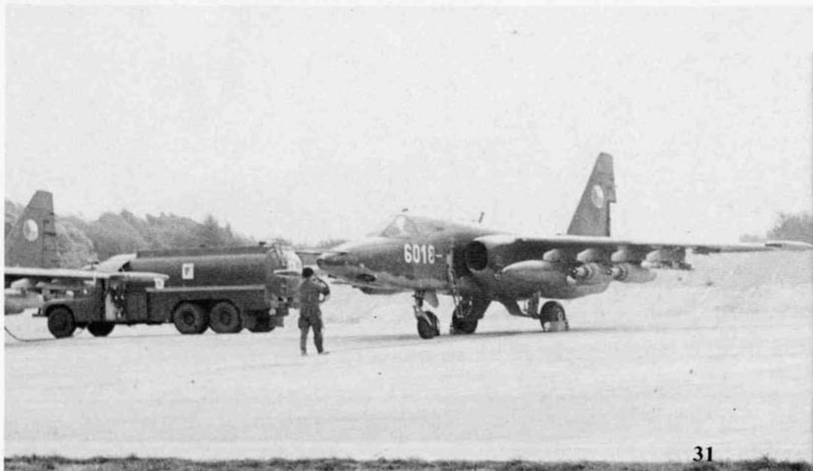
An Su-25K, White 6018, of the 1st Squadron, 30th Attack Regiment on the ramp at Pardubice Air Base. The aircraft is armed with UB-32A rocket pods and an MBD-3 multiple bomb rack capable of carrying four 220 pound bombs on the number four pylon. The fuel truck in the background is a TATRA T-148 fuel truck. (Pavel Polach)
