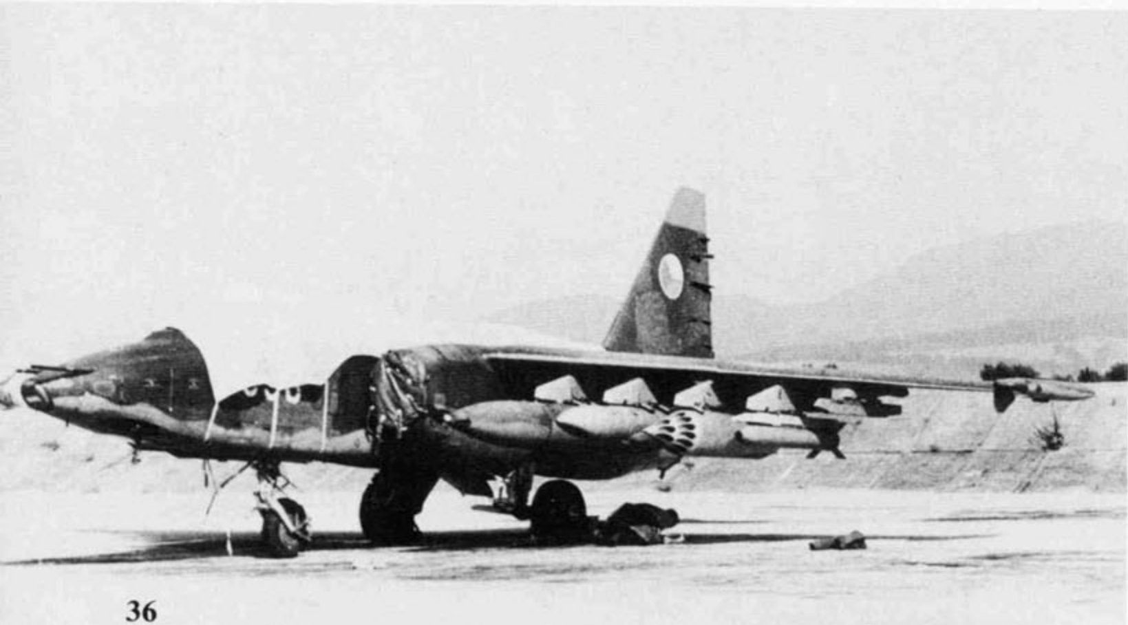
This Su-25K has the air intakes and canopy covered with protective canvas covers. It is armed with an SPPU-22 twin GSh-23 23mm trainable cannon pod on the number two pylon, a B-8M1 twenty-shot rocket pod on the number three pylon and an S-24 240mm unguided air-to-ground rocket on the number four pylon. (Pavel Polach)
