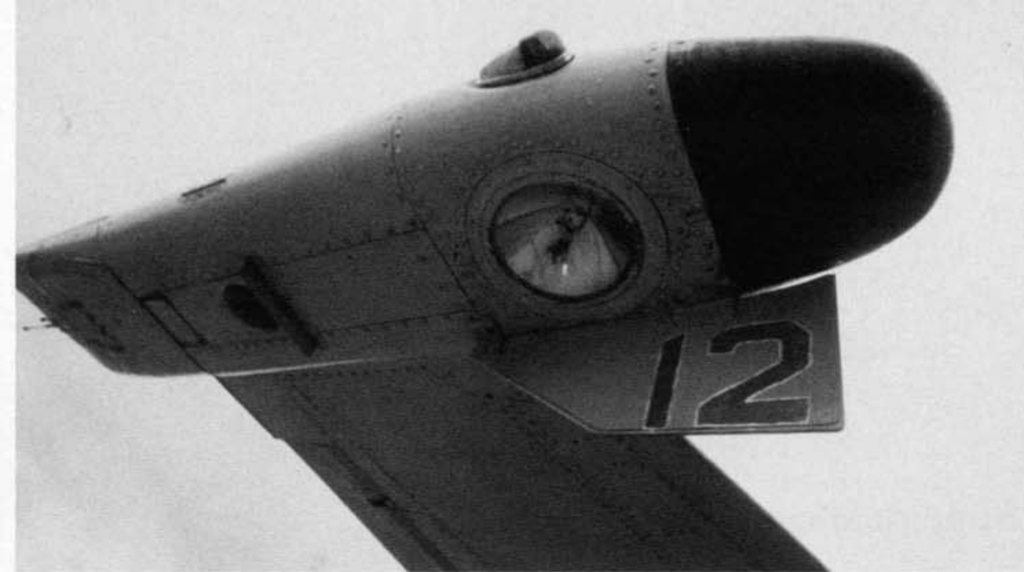
The late Su-25 had a modified wingtip pod with a sheet metal anti-glare panel between the aircraft and the retractable landing light. Additionally, the Su-25 differs from the T-8 in that the earlier aircraft did not have the round antenna in the center of the pod. (Marcus Fülber)
