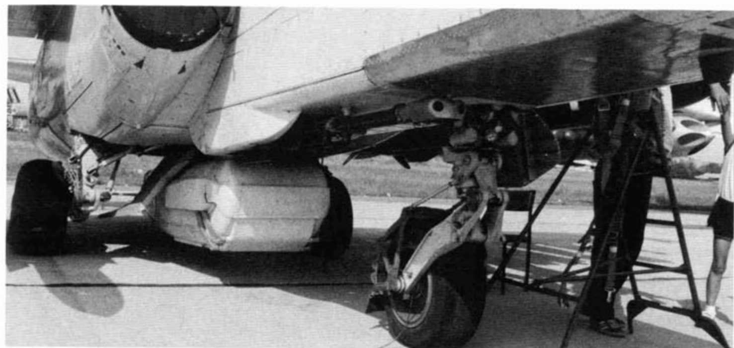
The AO-17A 30mm twin barrellled cannon is externally mounted and offset to starboard. (Harry Wisch)
