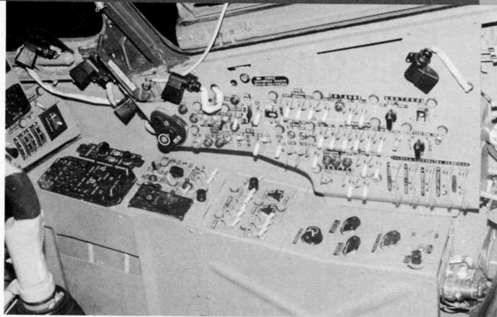
The cockpit layout of the Frogfoot is similar to that of the Sukhoi Su-22M-4 Fitter K. The starboard main console is Gray/Green with White toggle switches and Black knobs. The emergency canopy jettison handle at the upper right is in Red. (Josef Simon/ZLINEK Magazine)
