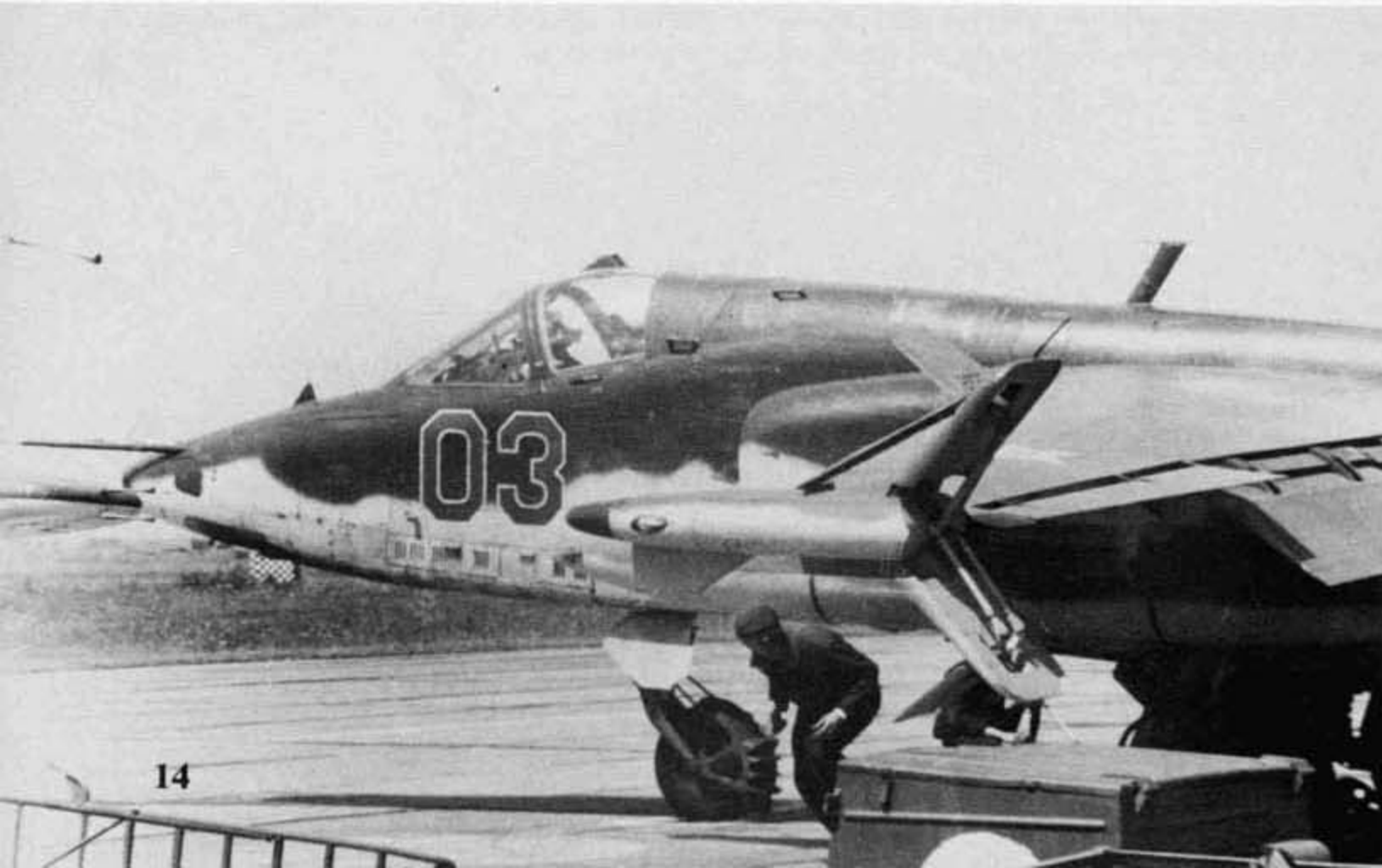
Ground crewmen prepare a late production Su-25 Frogfoot A for its next mission. The four part wingtip speed brakes are fully deployed and the aircraft is equipped with the SRO-2 blade type IFF antenna on the nose. (V. I. Pashenko)
