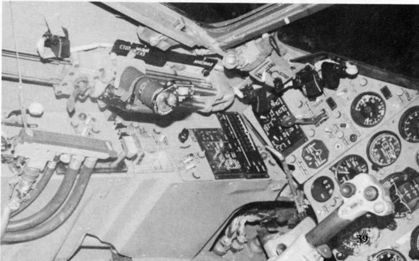
The port main console of the Su-25K contains the throttles for the R-95Sh engines and oxygen controls. Soviet fighter and fighter-bombers (both MiG and Sukhoi designs) all have a similar cockpit layout, making transition training from one type to the other much easier. (Josef Simon/ZLINEK Magazine)
