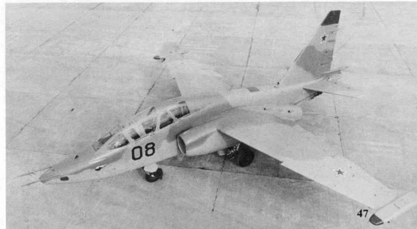
The Su-25UTG naval trainer prototype, Blue 08, was converted from the Su-25UT advanced trainer. The aircraft rolled out carrying a three tone Blue upper surface camouflage over Light Blue undersurfaces. The position of the national markings on the wing upper surface is standard for all Soviet Su-25 variants. (Sukhoi OKB)
