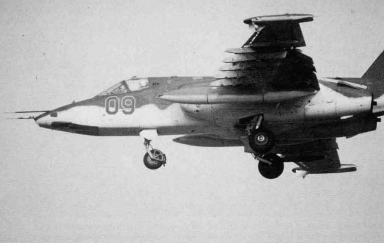
A T-8, Red 09, of the 368th ShAP, 16th Air Army at Demmin-Tutow, Germany. On most practice missions flown by this unit, the aircraft are configured with a pair of PTB-1150 drop tanks on the inboard underwing pylons. One of the main shortcomings of the Frogfoot A is its short endurance. (Jens Schymura)
