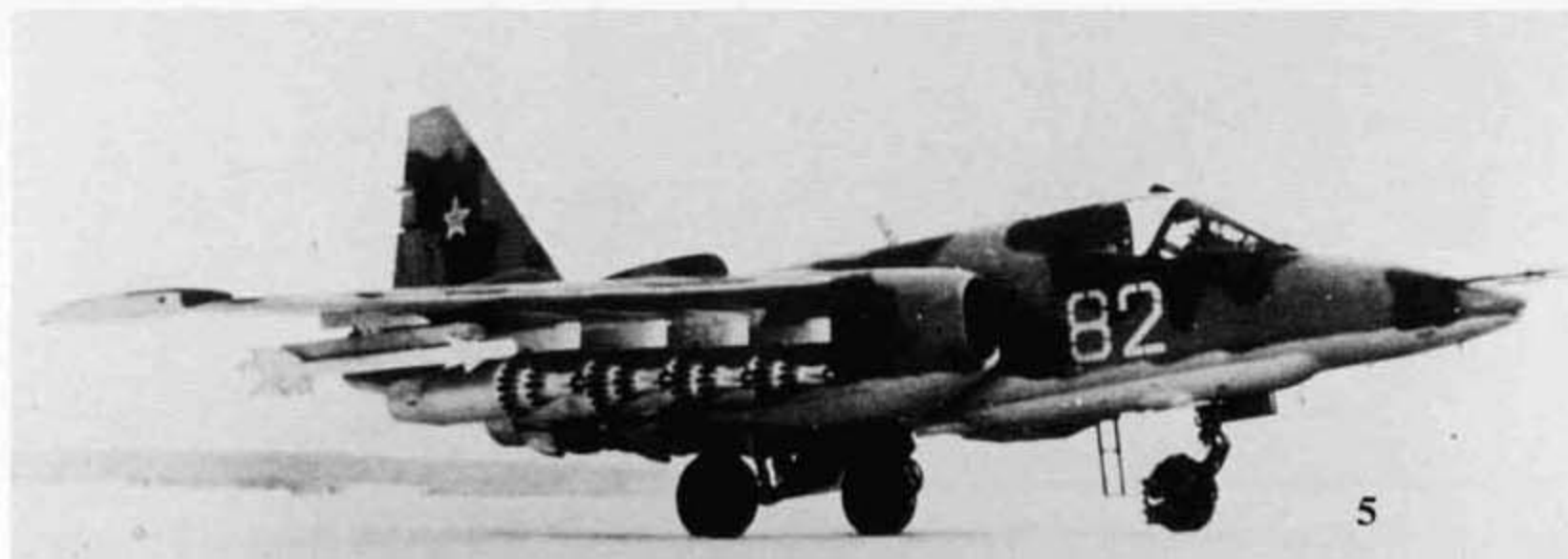
The second prototype, T-8-2, Yellow 82, differed from the first prototype in that the wing fences were revised with the larger fence now being inboard. The aircraft carried four large weapons pylons and a fifth smaller pylon for an AA-2 air-to-air missile. The fin was enlarged and the rudder was altered. The wing tip pods held avionics and the rear halves acted as speed brakes. (Sukhoi OKB)
