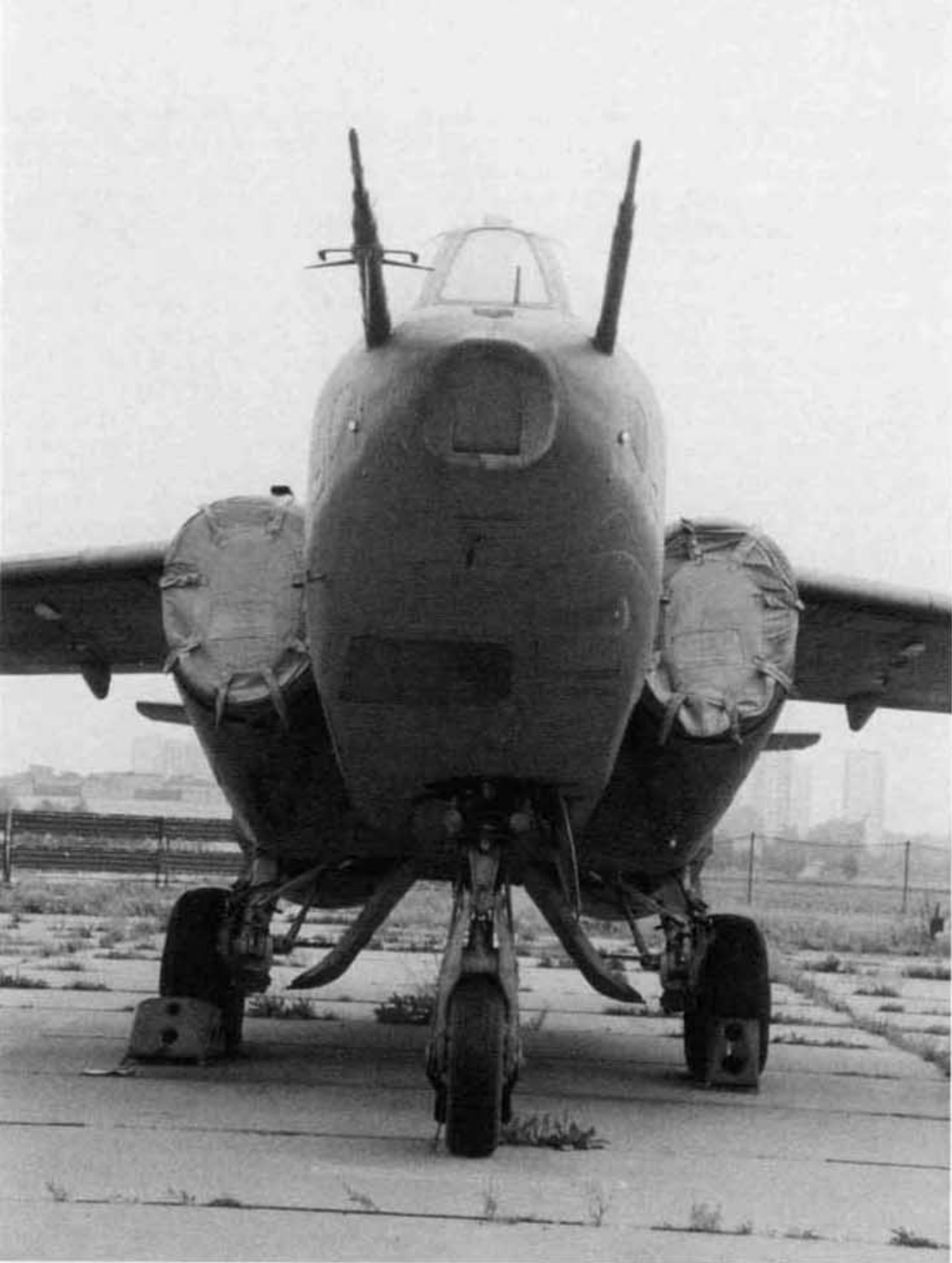
Red 12 was an Su-25BM target tug which had the internal 30mm cannon deleted to save weight and the cannon port faired over. These aircraft were used to tow aerial targets for both air-to-air and ground-to-air gunnery practice. (Harry Wisch)
