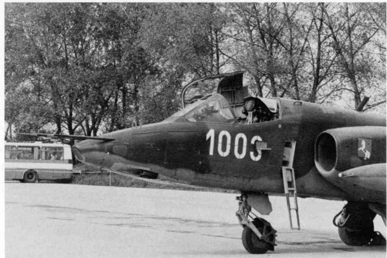
This late production Czech Air Force Su-25K, White 1003, is equipped with the later style one piece cannon muzzle. The natural metal panel in front of the gun port is a blast panel to prevent damage to the aircraft skin from the muzzle blast of the cannon. (Otakar Saffek)
