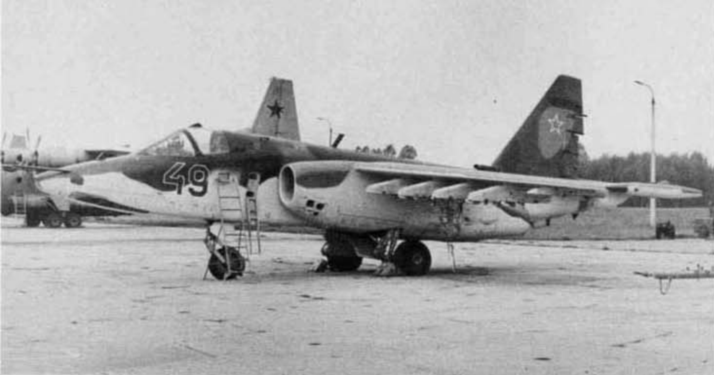
Although the built-in boarding ladder on this Su-25 Frogfoot A is deployed, a second portable ladder has been put in place alongside the aircraft. In actual service the built-in ladder was rarely used and it was deleted on later variants. (A. A. Zirnov)
