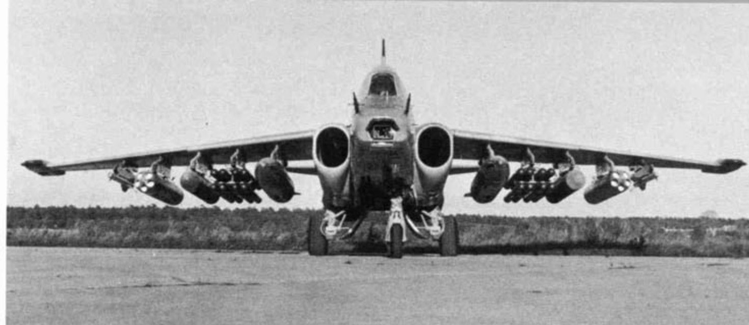
For armament testing the Su-25TM was configured with underwing fuel tanks, PTUR Vikhr anti-tank missiles, S-25 unguided air-to-ground rockets, B-13L four shot rocket pods and R-60 (AA-8) AAMs (Sukhoi OKB)
