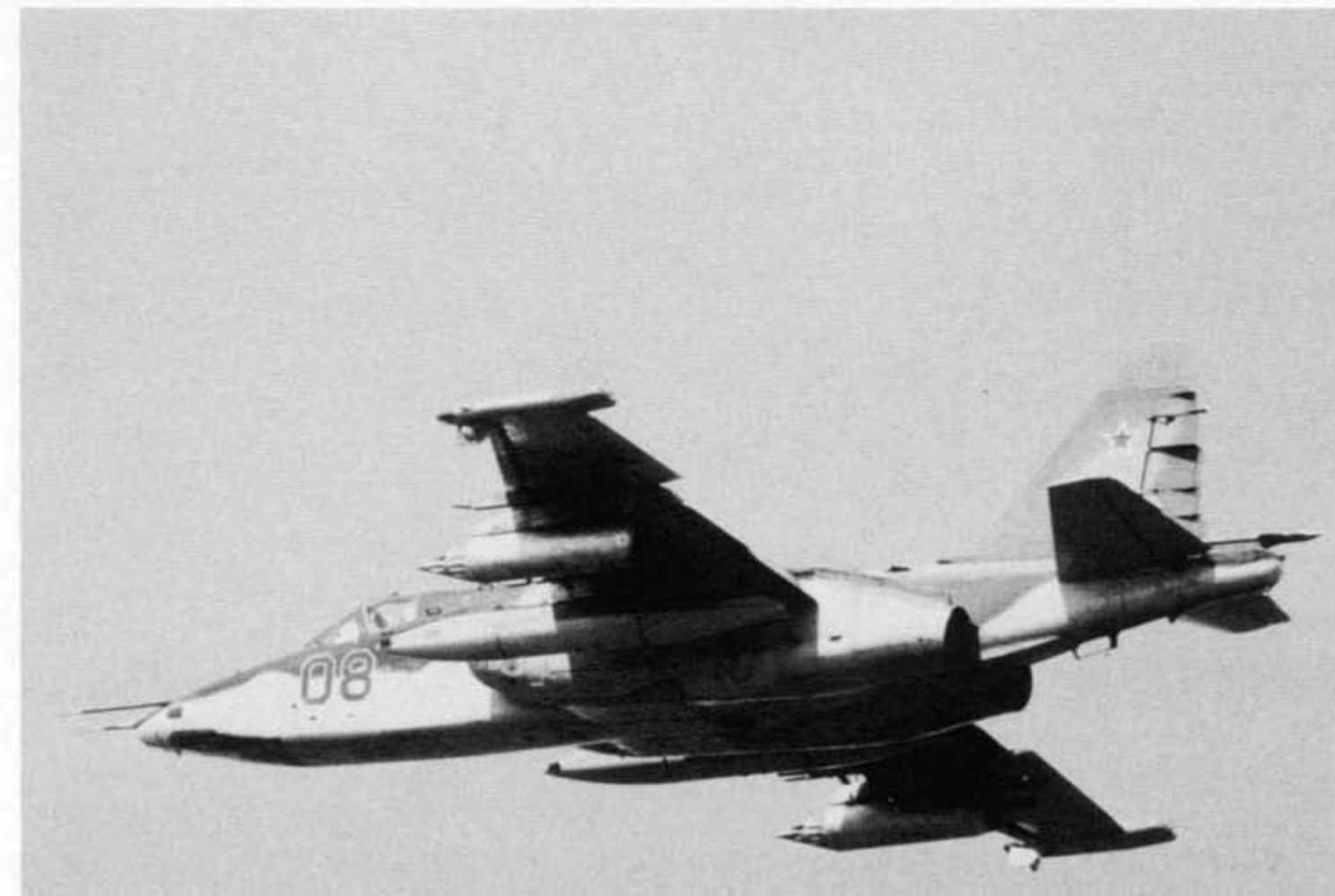
This Su-25, Red 08, is armed with twenty-shot B-8M1 80mm rocket pods on each number four pylon. Although the landing gear is up, the retractable landing light is still in the down position. (Martin Baumann)
