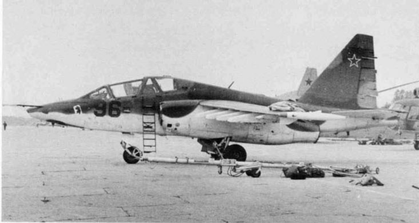
This early production Su-25UB Frogfoot B, Red 96, carries the early style three pole Odd Rods IFF antennas on the nose and under the tail. The wingtips of this trainer are painted White. (A.A. Zirnov)
