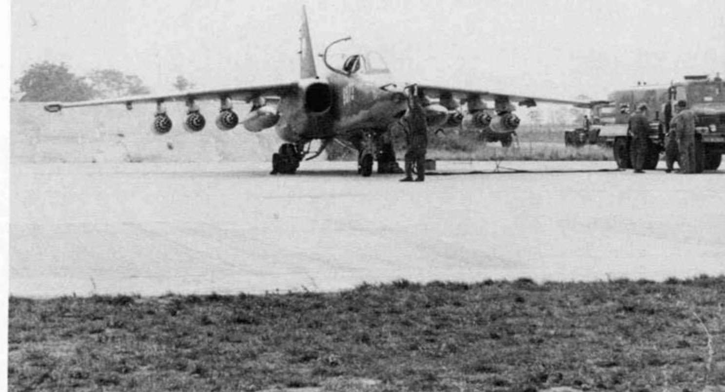
An Su-25K, White 8073, is refueled prior to a training mission while the ground crew relax by the aircraft. This aircraft carries PTB-1500 fuel tanks and six UB-32A thirty-two shot 57mm air-to-ground rocket pods. (Pavel Polach)
