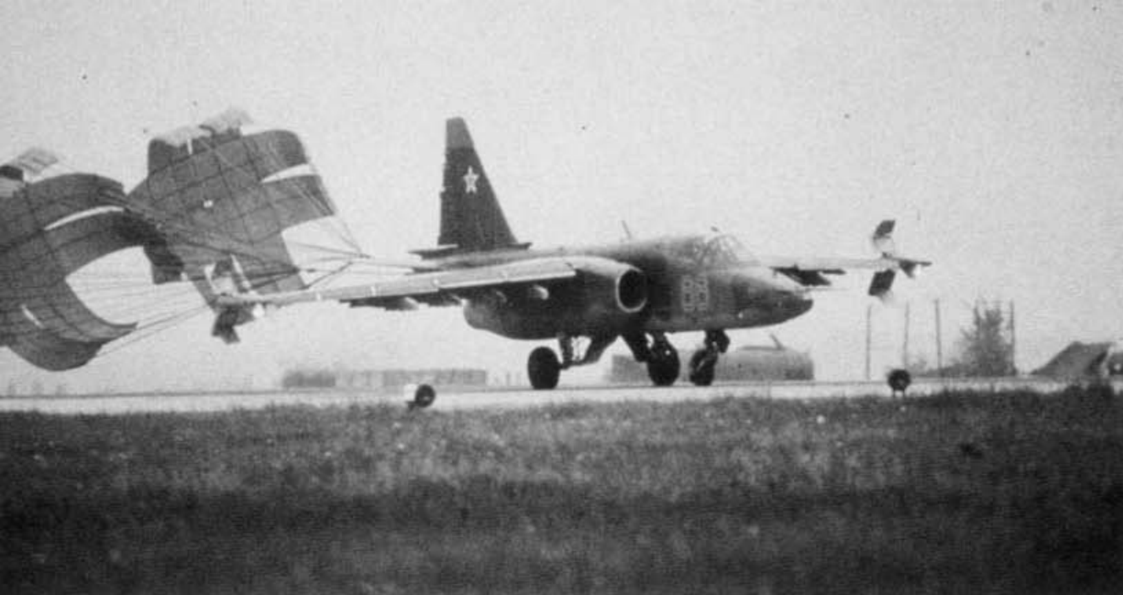
An Su-25 Frogfoot A, Blue 66, lands at Kubinka with the wingtip speed brakes and braking parachutes fully deployed. The Tan colored braking parachutes used on production Su-25s are larger than the earlier Red/White parachutes used on preproduction T-8s. (Steven Zaloga)
