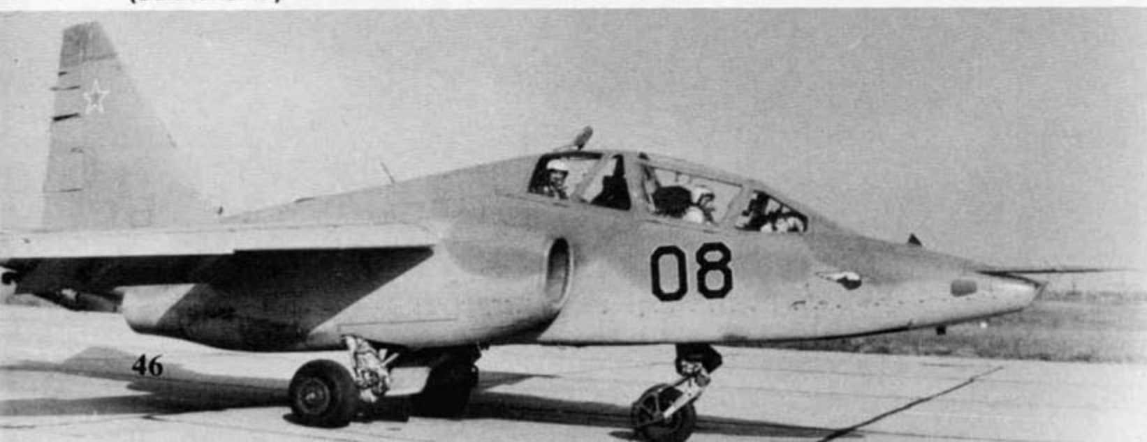
The Su-25UTG taxis out for a test flight with the rear seat periscope in the raised position. (Sukhoi OKB)
