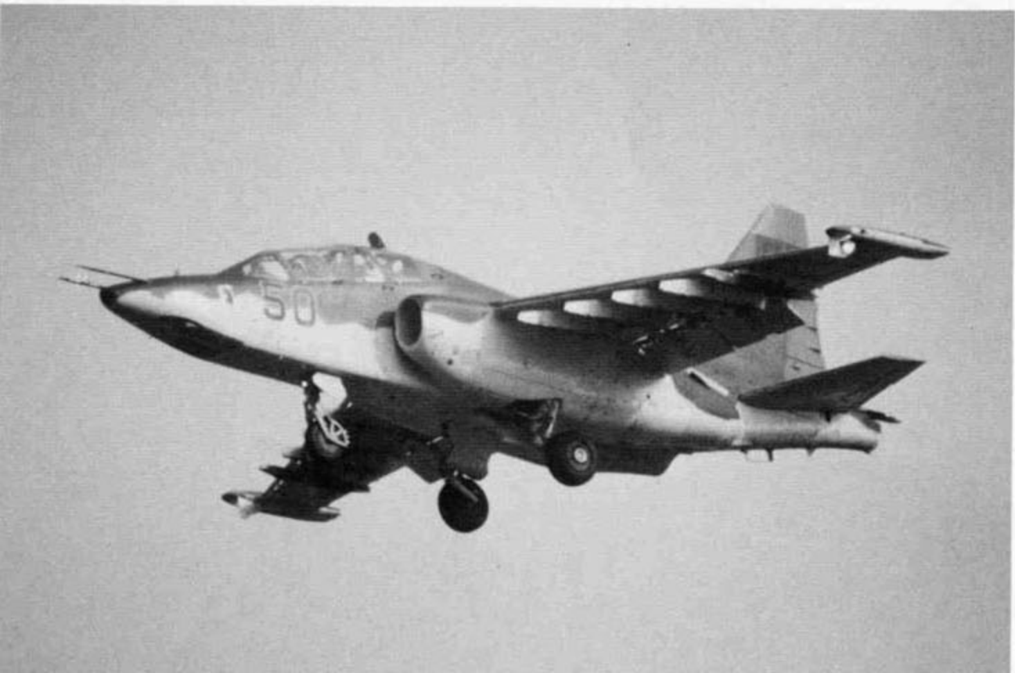
Red 50, an Su-25UB, on final approach to Demmin-Tutow Air Base, Germany, with the rear cockpit periscope raised. This Frogfoot B had been modified with the two chaff/flare dispensers on the upper rear engine nacelle. Additionally, the aircraft is carrying an APU-60-1M missile rail on the outboard wing pylon. (Jens Schymura)
