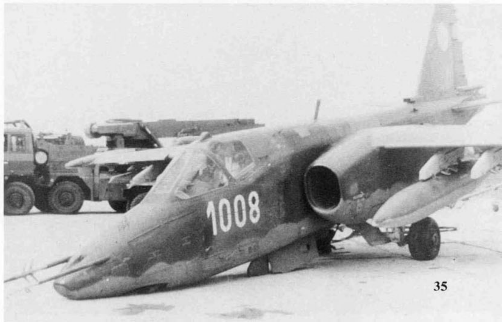
The nosewheel on White 1088 collapsed while the aircraft was parked on the ramp at Pardubice. The TATRA T 815 mobile crane in the background will be used to hoisted the aircraft so that ground crewmen can lower the nosewheel and install the safety pins. (Pavel Polach)
