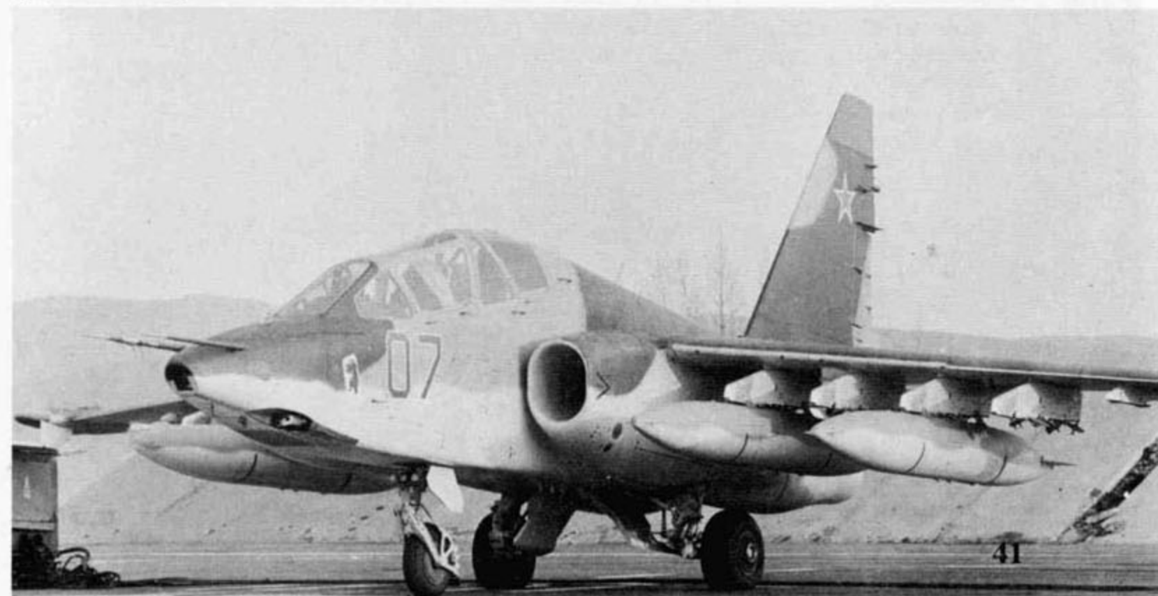
A recently completed Su-25UB, Red 07, parked on the ramp of the Sukhoi facility at Ulan Ude. The aircraft is configured for a ferry flight with four PTB-1150 drop tanks. The Black bear insignia on the nose is a factory emblem, not a unit badge, and is carried on the port side only. (Victor Kulikov)
