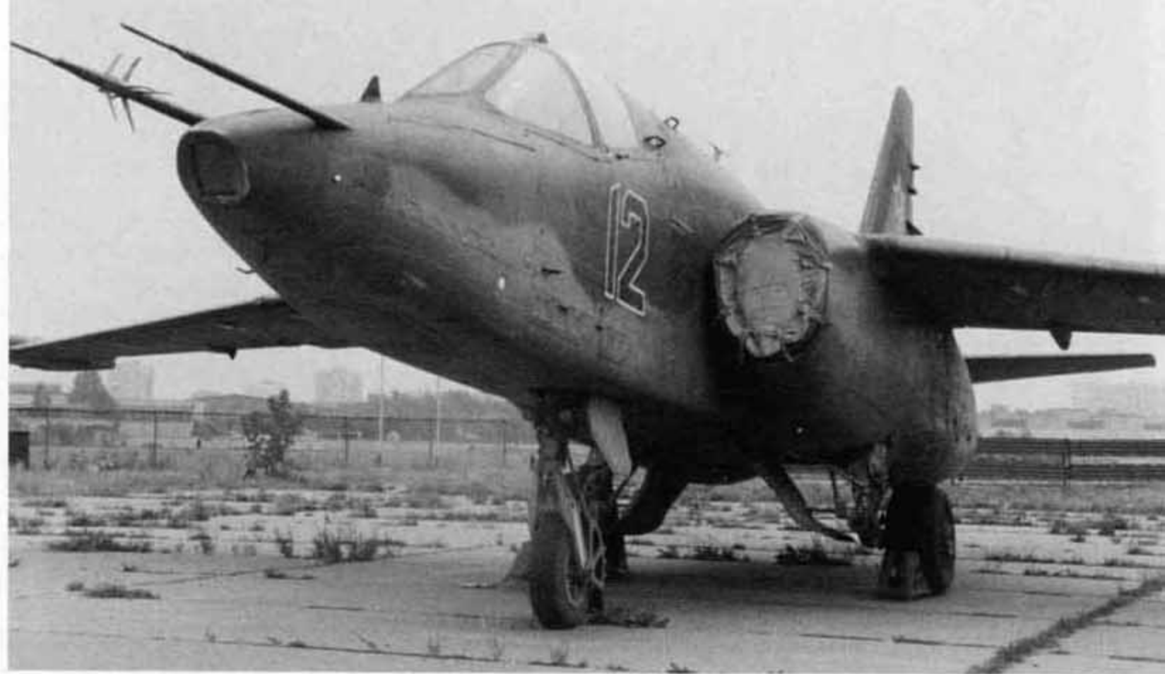
In addition to having the gun deleted and faired over, the Su-25BM had the laser range finder/designator removed and the window blanked out. When in use, the towed target and cable reel was suspended from one of the underwing pylons. (Harry Wisch)
