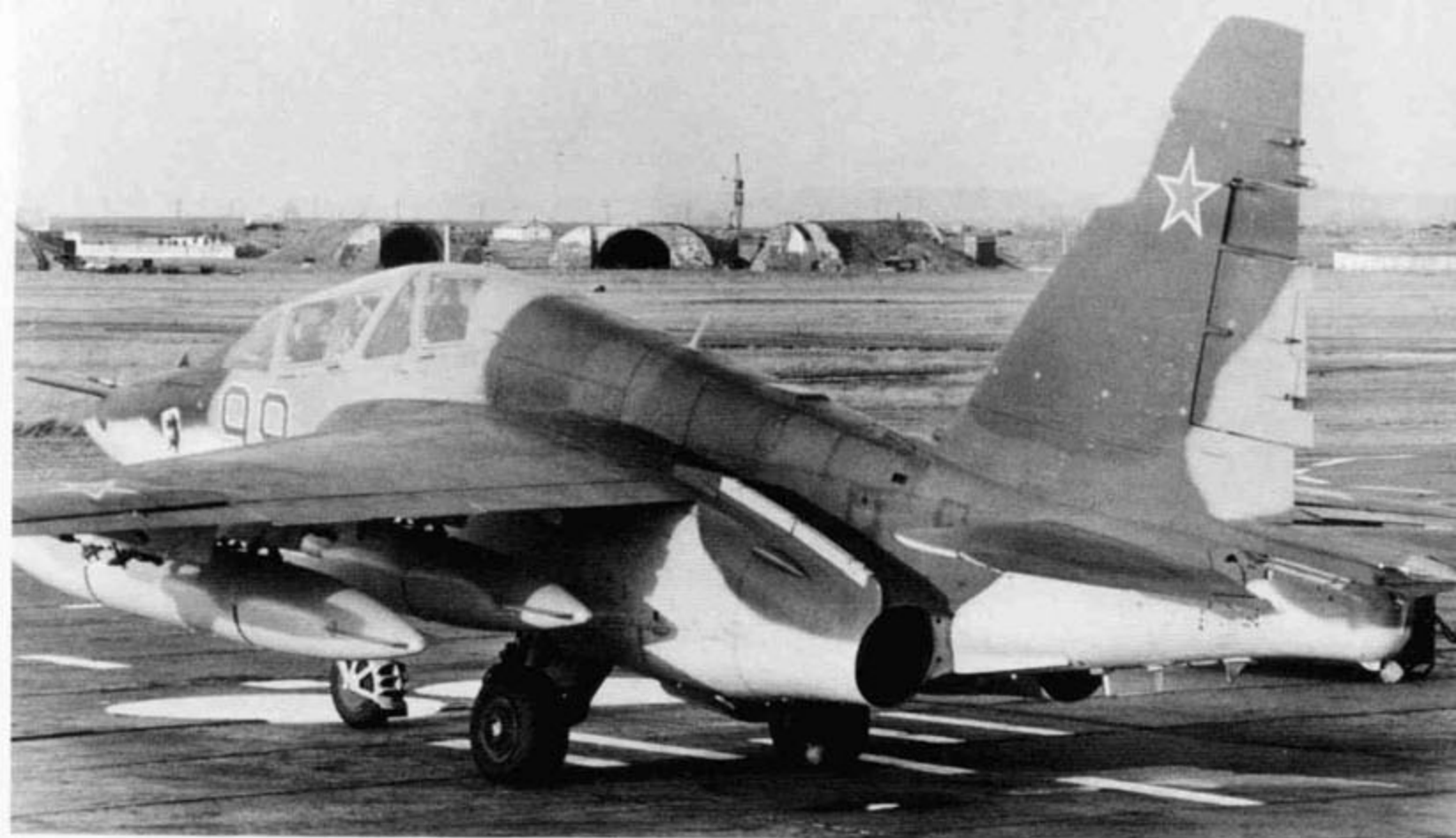
This late production Su-25UB, Red 99, on the ramp at Ulan Ude has factory installed ASO-2V chaff/flare dispensers on the upper rear engine nacelle and the later blade style IFF antennas on the nose and under the tail. One of the difference between the Su-25 and Su-25UB was the taller vertical stabilizer on the Frogfoot B. (Victor Kulikov)
