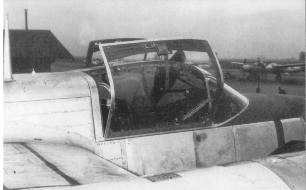
Unlike the earlier canopy, the clear canopy opened outward to both sides, allowing easy escape for both crewmen. This "clamshell" style canopy quickly gained favor with the crews and was retrofitted to earlier aircraft soon after it was introduced on the production line. (Mikesh)
