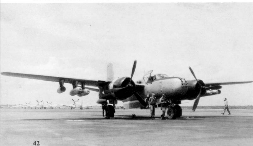
Ground crewmen go over a B-26B prior to a mission out of Bien Hoa Air Base, South Vietnam. The Air Commandos flew a mixture of six and eight gun nosed B-26Bs. The aircraft were modified with special wing racks so they could carry heavier ordnance loads. (USAF)
