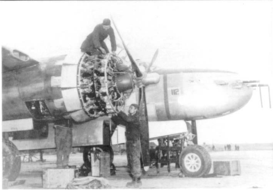
Ground crewmen perform maintenance on an early A-26B Invader in France during late 1944 or early 1945. The A-26 was powered by either the 2,000 hp Pratt and Whitney R-2800-27 or 2,000 hp Ford R-2800-71 radial. The engines drove twelve and a half foot propellers which differed from the prototype in that they did not have large spinners. (Tweedy via AFM)
