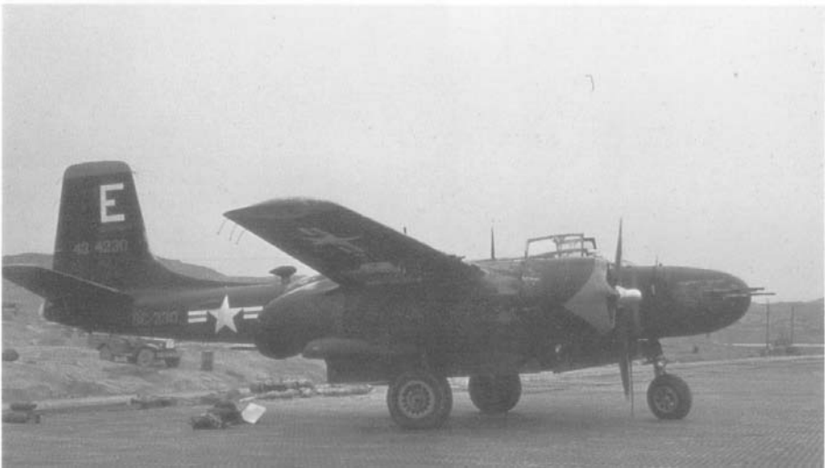
Gradually the two Invader groups shifted over to night work as the Communists began to move men and material only at night. As a result, the aircraft were repainted Gloss Black. This six gun nose B-26B from the 13th BS, 3rd BG awaits the arrival of its crew for a night interdiction mission. (USAF via Bell)
