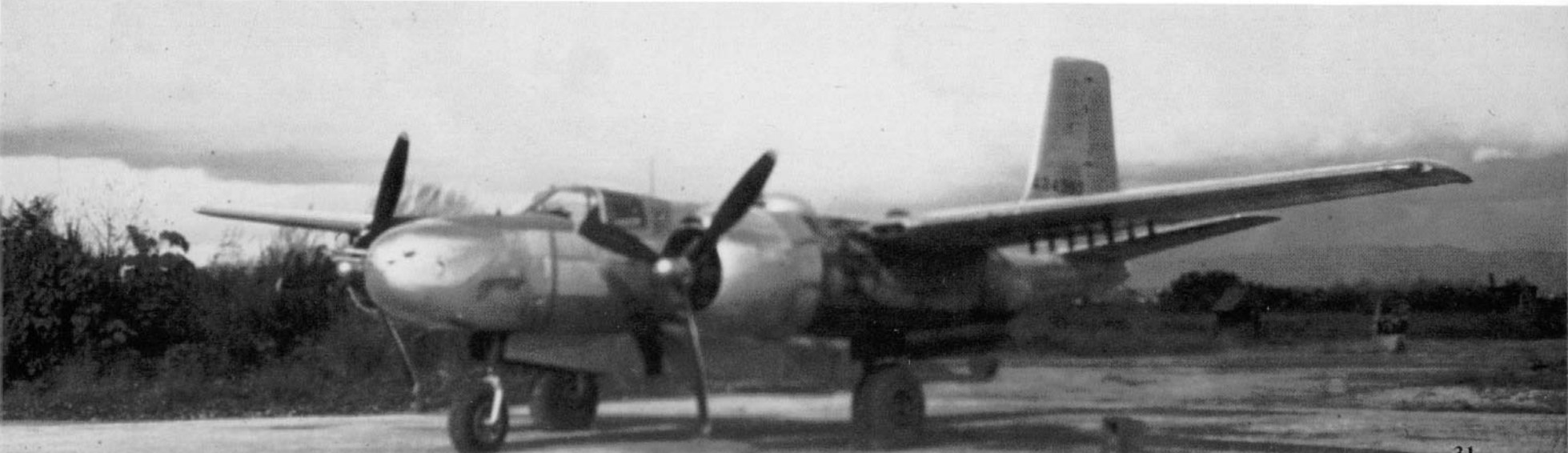
An overall Natural Metal six gun A-26B, possibly of the 319th BG, parked off the side of the runway on Okinawa. The aircraft was fitted with the zero length rocket launchers for five inch HVAR rockets under the outer wing panels.
