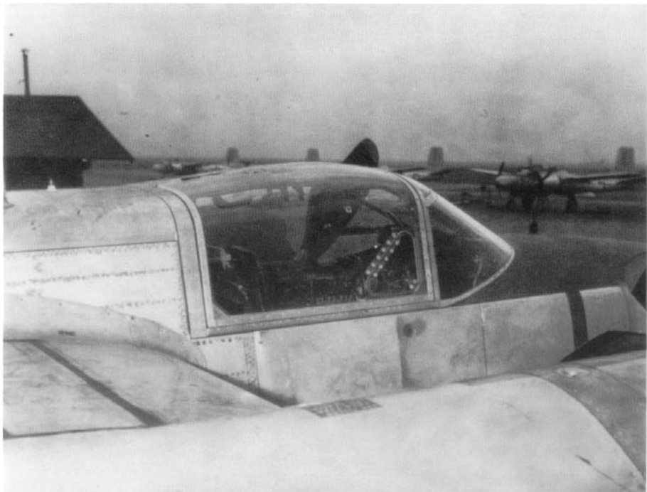
To solve the cockpit emergency exit problem, Douglas tried a number of different canopy styles. Finally they settled on this clear blown canopy that increased head room and pilot visibility since it eliminated the heavy framing. (Mikesh)
