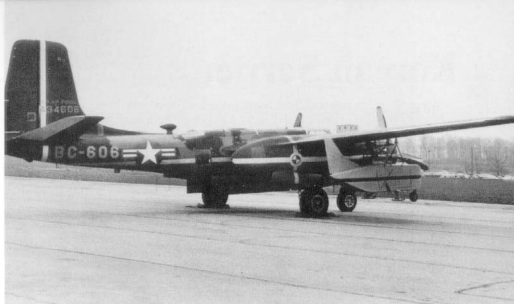
A number of Invaders were used to test the feasibility of underwing cargo pallets which could be carried by combat aircraft into forward bases. The small wooden container used a combination of skids and wheels to land. (AFM)
