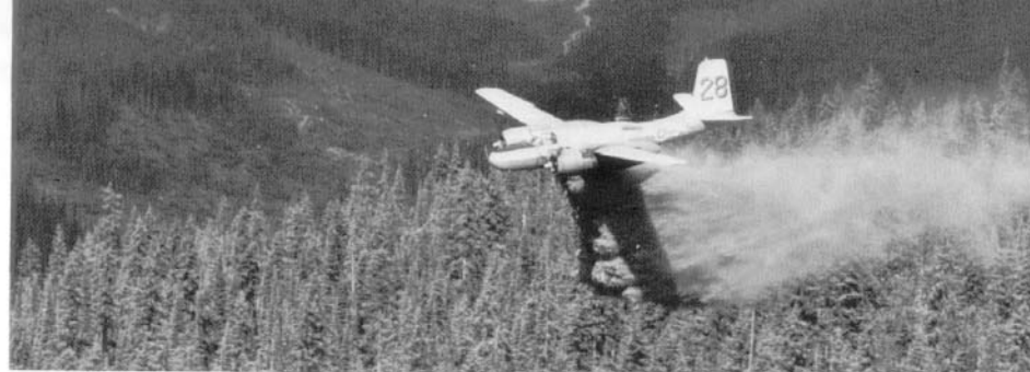
A large number of Invaders were converted for use as fire bombers to help fight forest fires in the U.S. and Canada. One of the larger users of the type was Conair Aviation of British Columbia who flew Red and White Invaders. (Conair)
