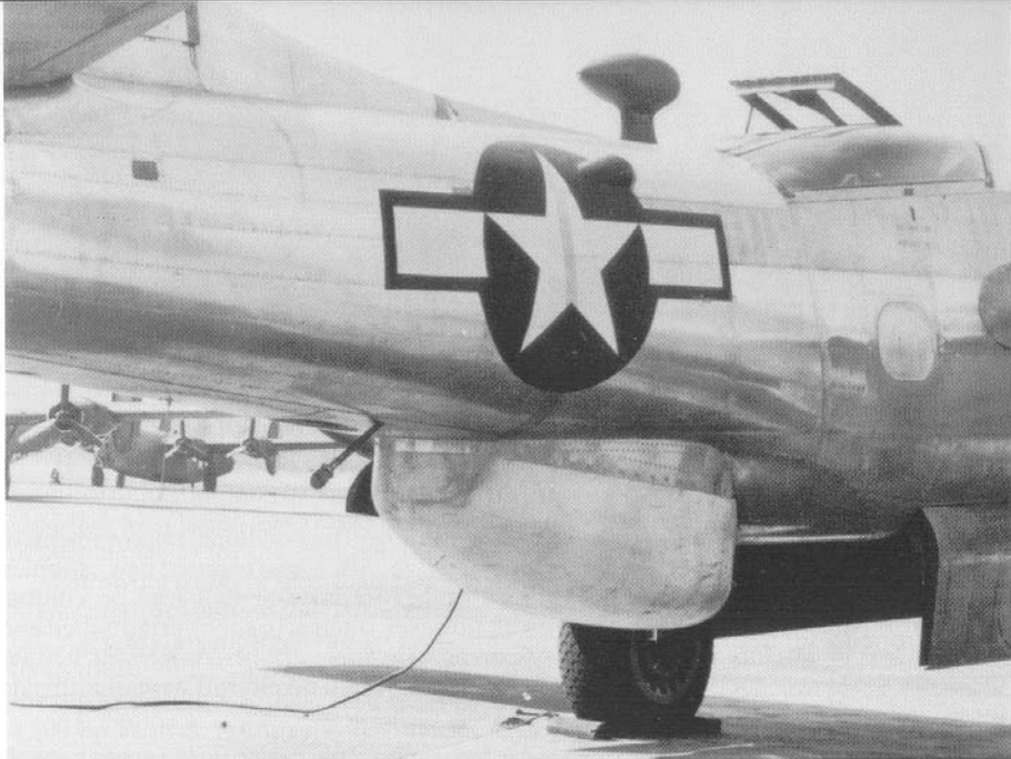
The FA-26C carried various electronic reconnaissance equipment and radars installed in pods or blisters. Some were carried under the wings, in the bomb bay and in the nose. (USAF)
