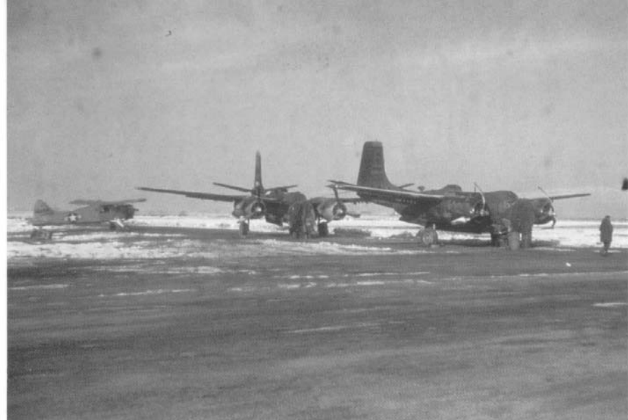
Besides enemy fire, the B-26s faced horrible weather conditions. Following a heavy snow, these two B-26s struck high snow drifts which sheered off the nose gear. In the ensuing crash the entire nose section broke away and at least one navigator/bombardier lost his life. After these two incidents, no one was allowed to ride in the nose during takeoff or landing. (Geidel)
