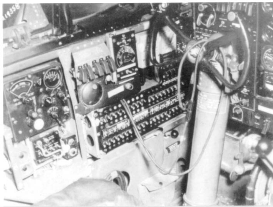
Like the A-20 Havoc, the A-26 had only a single set of controls on the left side of the cockpit while the right side had a jump seat for the navigator. The reflector gunsight was located directly above the control column at the top of the instrument panel. (Mikesh)
