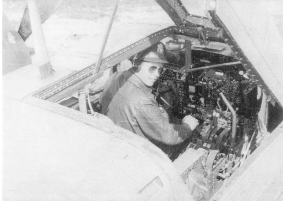
On early A-26 Invaders a large piece of bulletproof glass could be positioned in front of the pilot for additional protection from flak or bullets. It is visible directly in front of the pilot of this early Invader of the 416th Bomb Group. (E. & K. Bishop)
