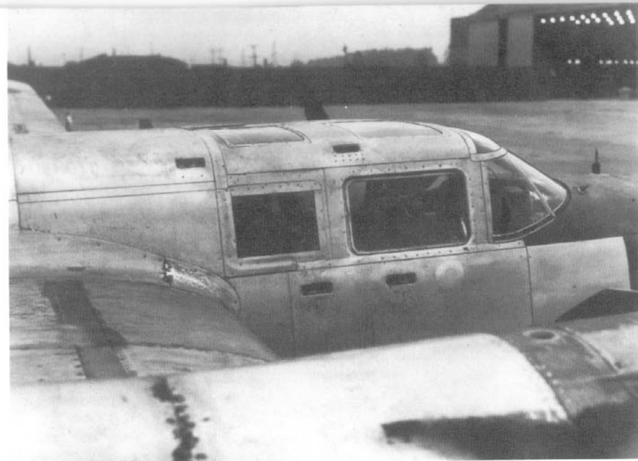
Early production Invaders were fitted with a heavy framed "flat top" style cockpit canopy which only opened on the right side. The heavy framing severely restricted the pilot's visibility. (Mikesh)
