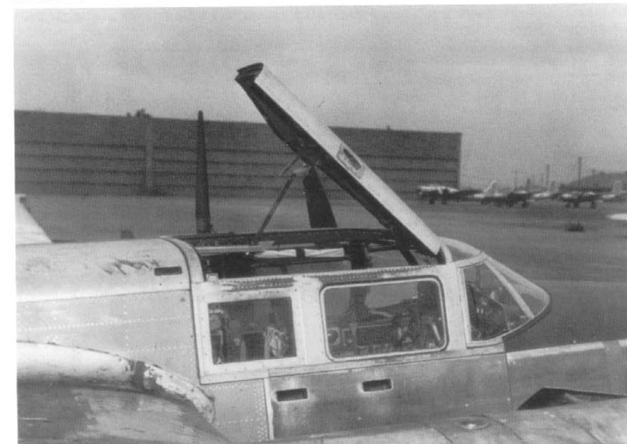
The heavy framed canopy opened upward on the starboard side, making escape during an emergency almost impossible for the pilot who was seated on the port side. (Mikesh)
