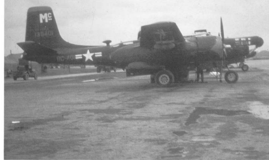
A number of B-26Cs from the 3rd BG were fitted with special electronics and radar gear in a modified nose section for night detection work. The original nose was modified with additional framing and the upper section was been extended to house the radome. (Kerr)
