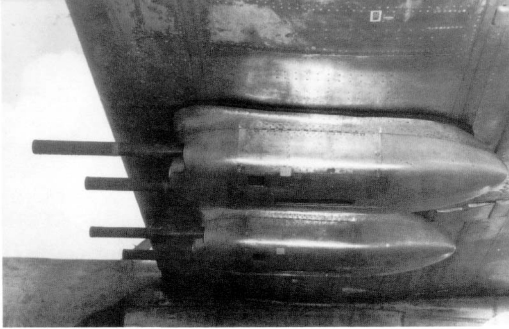
To augment the Invader's forward firepower, one or two gun pods housing two .50 caliber machine guns each could be carried under the outboard wing panels. Each pod was fed ammunition from magazines in the wings. While the gun pods increased firepower, they cut the Invader's speed. (Mikesh)
