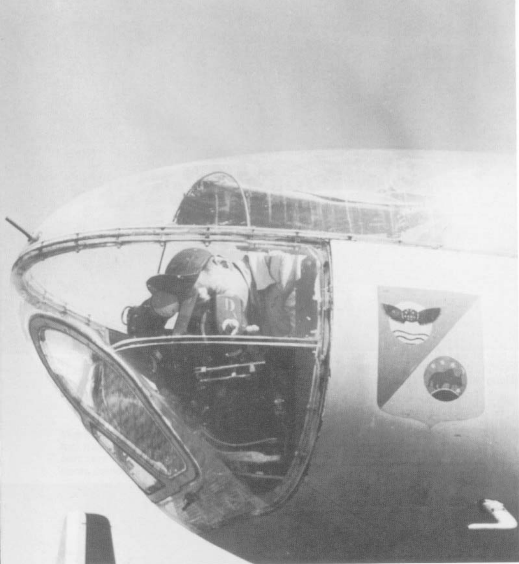
The A-26C Invader replaced the solid gun nose with a bombardier's compartment which housed a Norden bombsight and related equipment. The clear plexiglass nose was composed of two sections which were riveted together. The lower forward section had an optically flat panel for the bombsight. This A-26C carries the insignia of GB 1/25 Tunisie , a French unit that flew Invaders in Indochina. (ECPA)
