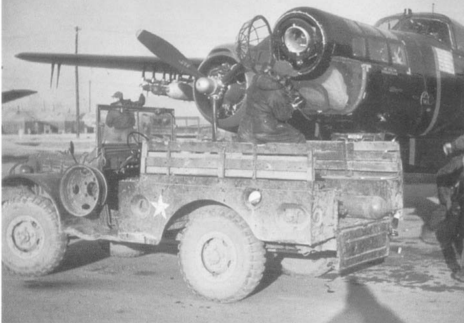
Ground personnel work on the radar in the nose of one of the specially modified radar equipped B-26s. The radar tracking gear was mounted in a gimble arrangement and could rotate through a large arc to detect ground targets. (Kerr)
