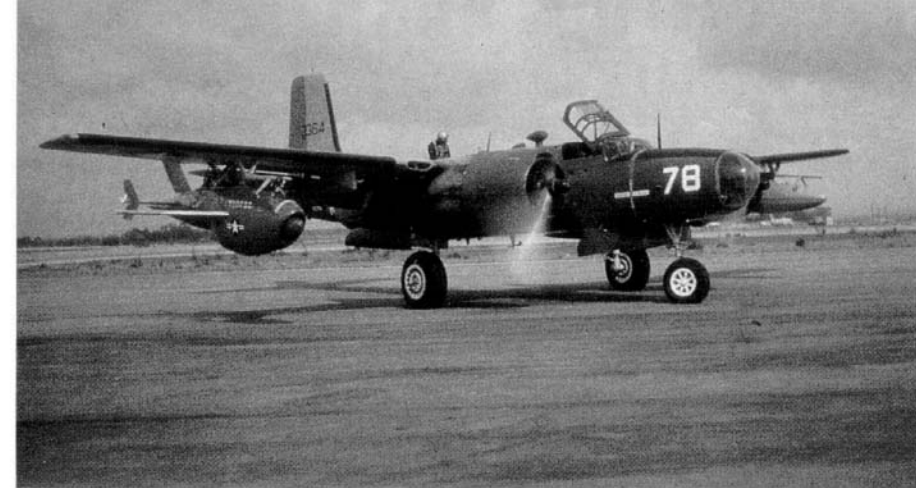
In Navy service the drone controller aircraft were designated JD-1Bs until 1962 when the services realigned the aircraft designation system. At that time they were redesignated as DB-26Js. Normal practice in the Navy was to carry a drone under the starboard wing and a control pod under the port wing. (JEM Aviation)
