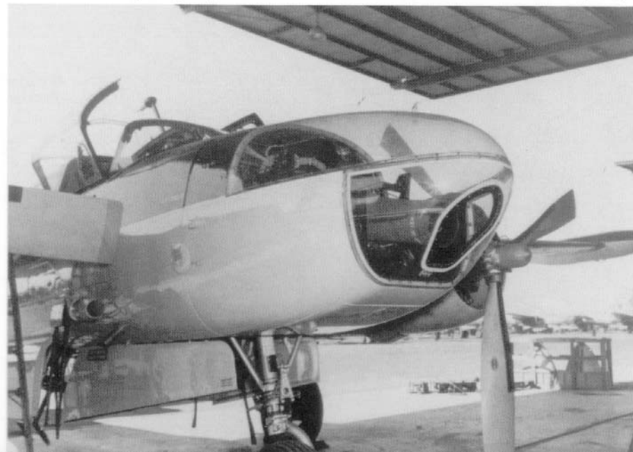
A K38 forward oblique reconnaissance camera could also be located in the nose, looking out the bombardier's optically flat panel and a P2 vertical camera was located in the tail. (AFM)
