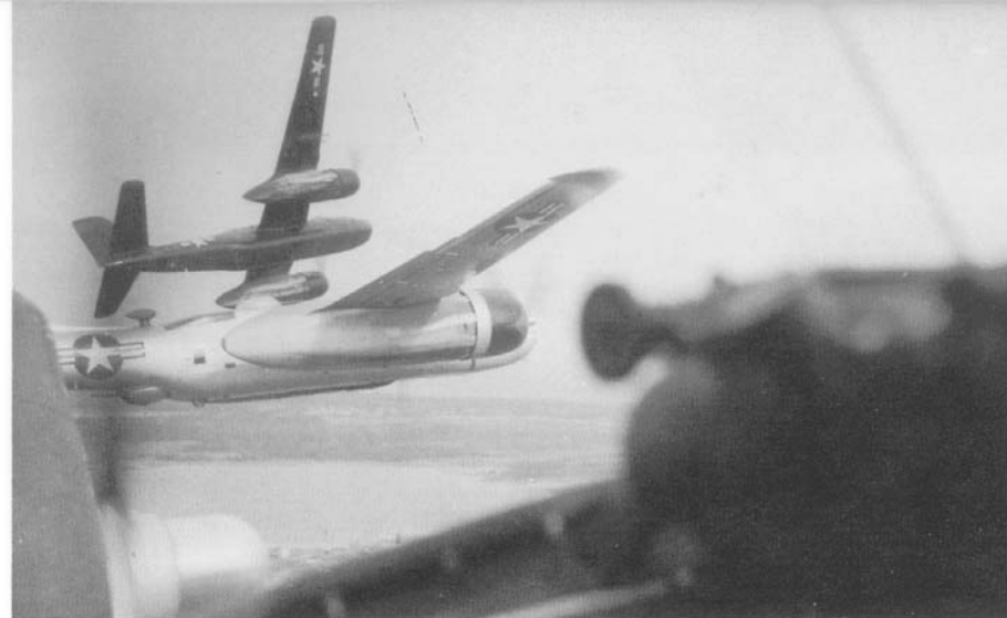
Two glass nosed B-26s peel off from the formation for landing at Langley, revealing the gun pods carried on the B-26 in the background. For an aircraft of its size the Invader was extremely maneuverable. The 345th later re-equipped with the Martin B-57 jet bomber. (Mikesh)
