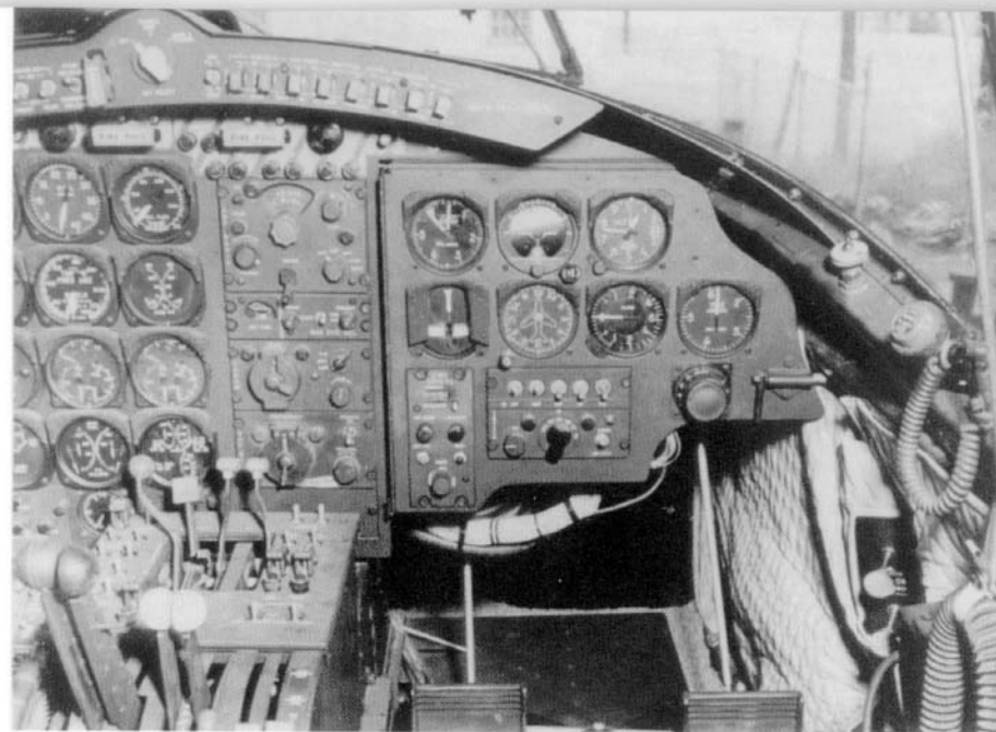
The cockpit was modified with dual controls and upgraded instruments but the layout remained basically similar to the original. The new instrumentation was installed in a panel on the right side of the cockpit. (AFM)
