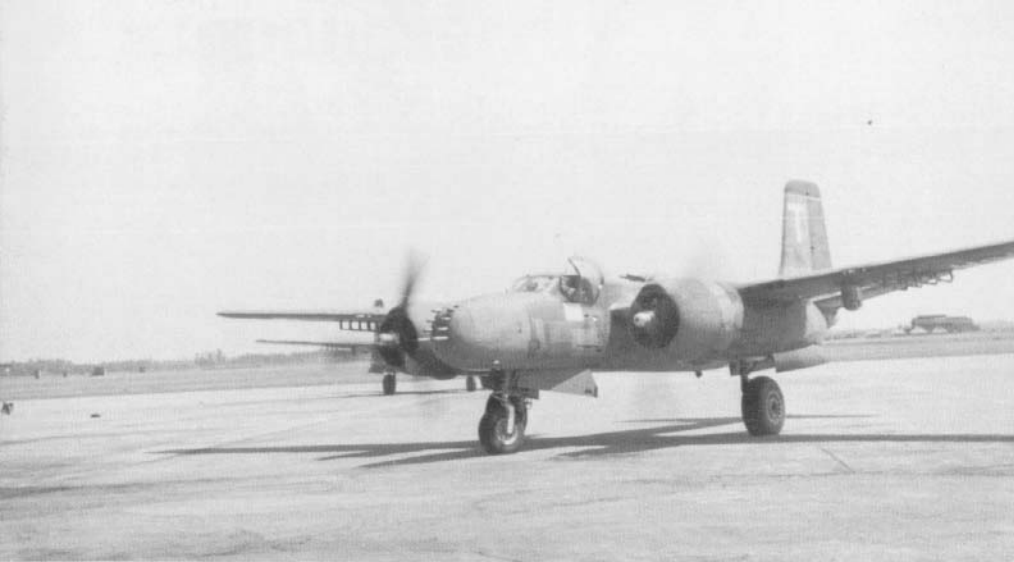
An Olive Drab over Neutral Gray eight gun B-26B of the 13th Bomb Squadron, 3rd Bomb Group taxis in after a mission over Korea. The 13th Bomb Squadron had the fin tip painted Red as a unit identification marking. The 3rd Group flew both camouflaged and overall Natural Metal aircraft. (R.V. Powell via R.V. Powell III)
