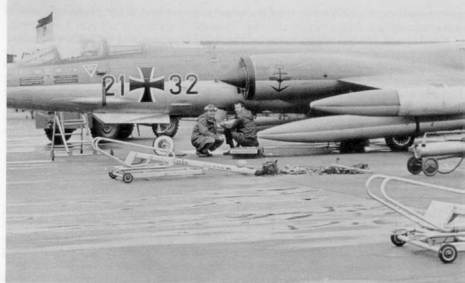
An RF-104G of the German Navy is prepared for a mission during the NATO Big Click photo reconnaissance meet. The light colored bands on wing tanks are Dayglo Orange. The RF-104G did not carry the M61 gun system and had the gun port faired over. The fairing behind the nose wheel door that covered the KS-67 cameras has been removed. (Udo Weisse)
