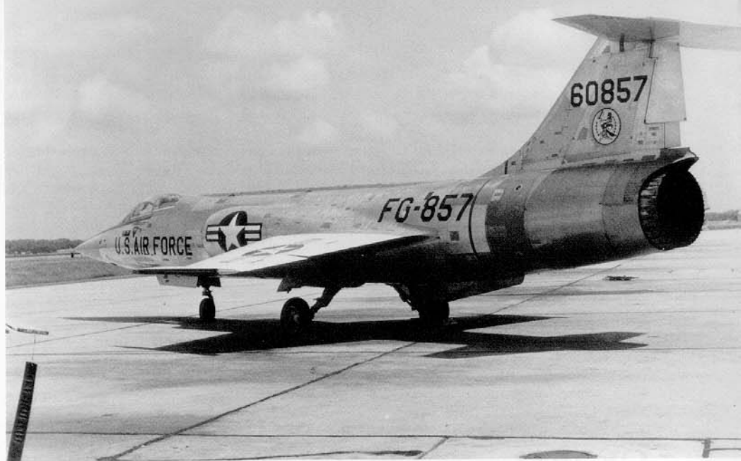
This F-104A of the 56th FIS has the M61 cannon port faired over and missile rails for AIM-9 Sidewinders on the wingtips. The Starfighter had the performance to be an interceptor, but its weapons limitation (two AIM-9B Sidewinders), short range and lack of an effective radar limited the F-104A to the point of defense role. 0587 served with the 56th, the 157th, the 331st and the 319th before being destroyed in a crash in 1968. (Fridell Collection)
