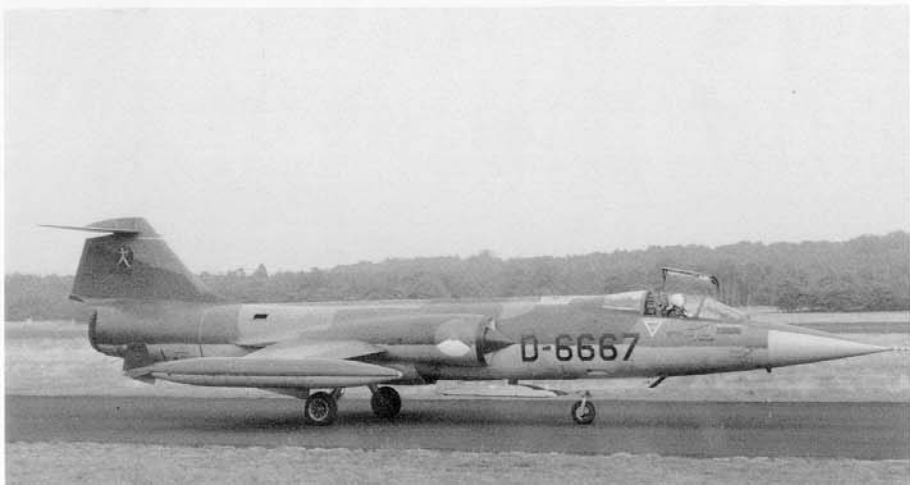
An F-104G of No 323 Squadron, Royal Netherlands Air Force taxis out for a training mission. No 323 Squadron provided a major part of the Netherlands' air defense system and their Starfighters were optimized for the intercept mission. This aircraft is equipped with AIM-9 Sidewinder fuselage pylons and wingtip fuel tanks. The white stripe at the top of the fin is common on Dutch F-104s. (Lee Bracken via Frank Garcia)
