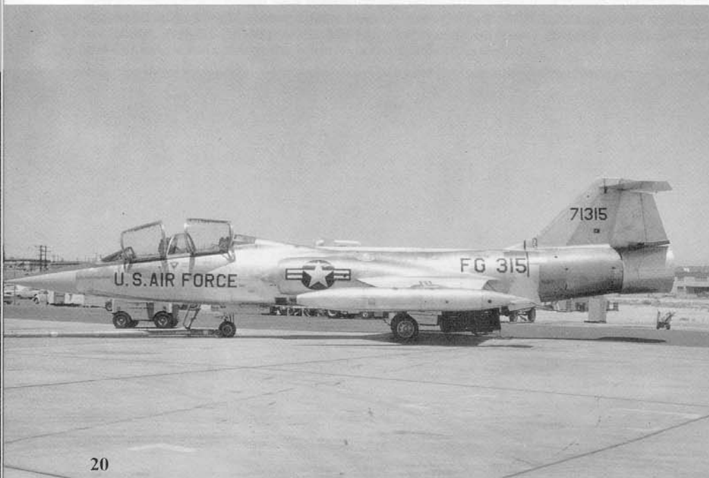
This F-104D (57-1315) on the ramp at China Lake was assigned to the AFFTC as a photo chase aircraft and carries the Air Force Systems Command insignia on the fuselage. The structure surrounding the afterburner nozzle was an experiment aimed at reducing the F-104's considerable infrared signature. (USN/Fridell Collection)
