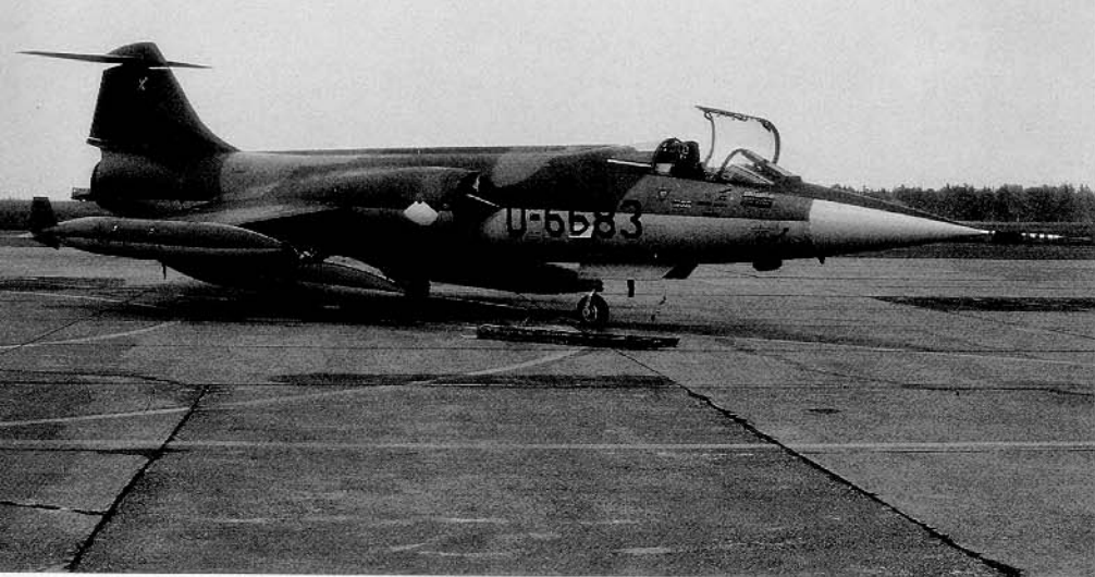
This No 312 Squadron F-104G had the wing tank fins painted Gloss Yellow, with Black tiger stripes applied over the base color for participation in a NATO Tiger Meet. The aircraft carries the standard NATO camouflage of Dark Gray and Dark Green uppersurfaces over Light Gray undersurfaces. (Jack Morris)
