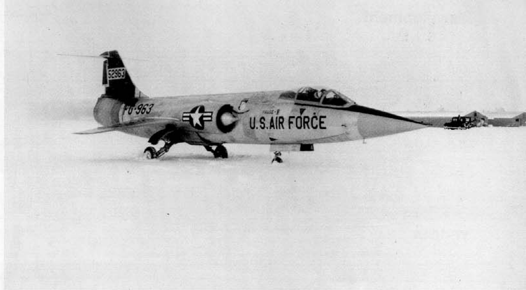
One of the seventeen YF-104As (55-2963) on the ramp at Elmendorf AFB, Alaska, for cold weather testing. This aircraft was assigned to the Air Force Flight Test Center (AFFTC) and carried Arctic markings applied on the tail surfaces. The legend Phase V above the U. S. Air Force probably refers to the stage of testing the aircraft was in. (Isham Collection)
