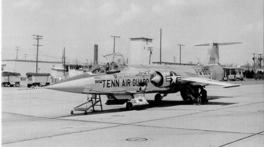
This F-104A of the 151st FIS Tennessee Air National Guard, previously deployed to Taiwan during Operation JONAH ABLE, served with several ADC and ANG units and finally was destroyed in a crash while assigned to the 319th FIS. The aircraft has the M61 cannon port faired over which was typical of most early F-104As. (Isham Collection)
