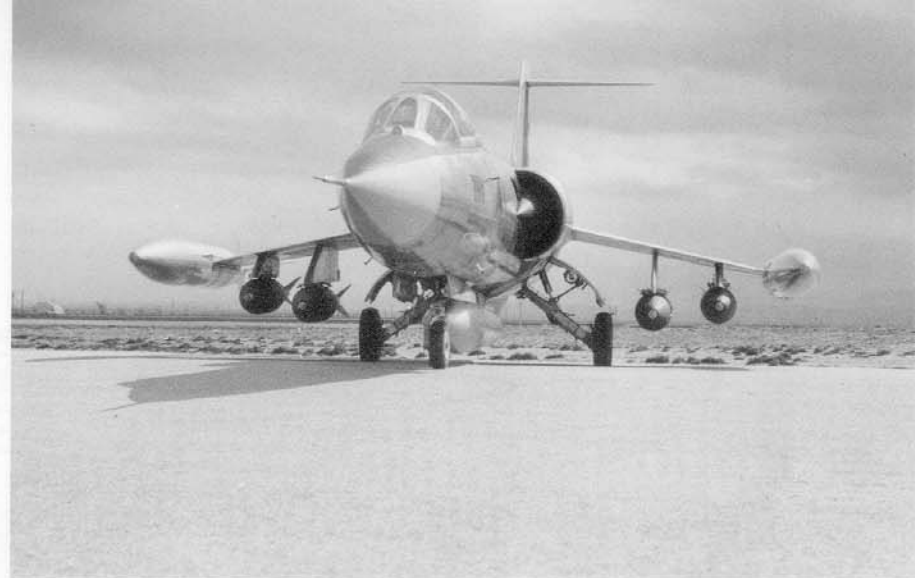
An F-104G fully loaded with 750 pound M117 bombs on the four underwing pylons and a fuel tank on the under fuselage centerline pylon. The F-104G was among the fastest tactical fighters in the world, but this load would have rendered the aircraft subsonic! The gunport for the M61 cannon is faired over on this Starfighter. (Lockheed via Friddell)
