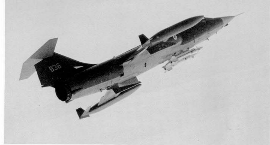
Late in their operational careers, Norwegian CF-104Gs were camouflaged in a Dark Olive Green over Light Gray scheme. This aircraft of No 331 Squadron is armed with a pair of late model AIM-9 Sidewinder missiles and has been modified with an ECM blister on the radome under the nose and Radar Airborne Warning (RAW) blisters on both sides of the tail cone. (Defense Command, Norway)
