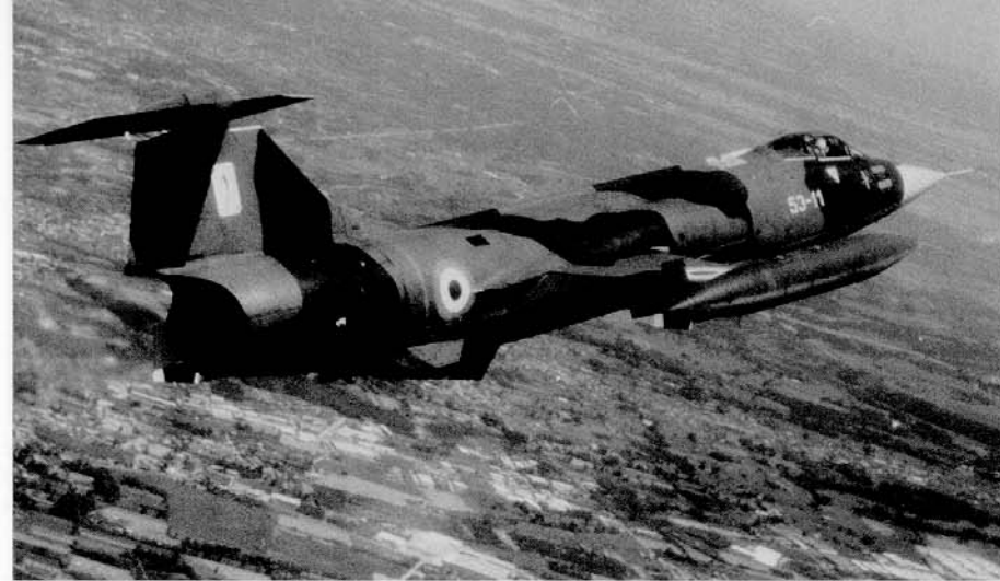
Italy's F-104S is, in many respects, the most potent of all the Starfighters variants and its mission comes closer to that of the original F-104 concept than other NATO operators. This F-104S of the 53rd Stormo was based at Cameri. One of the modifications done to the F-104S was the addition a pair of small fins located on either side of the ventral fin. (Italian Air Force)
