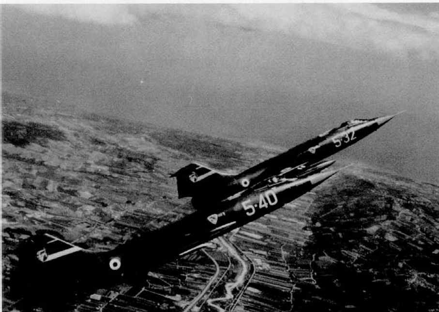
These F-104S Starfighters of the 20th Gruppo carry the 5th Stormo Diana the Hunter badge on the vertical tail with Yellow stripes coming off the badge. The pitot tubes are striped in Red and White, with a break in the center of the tube. Camouflage patterns on Italian F-104s are standardized but are not exact from aircraft to aircraft. (Italian Air Force)
