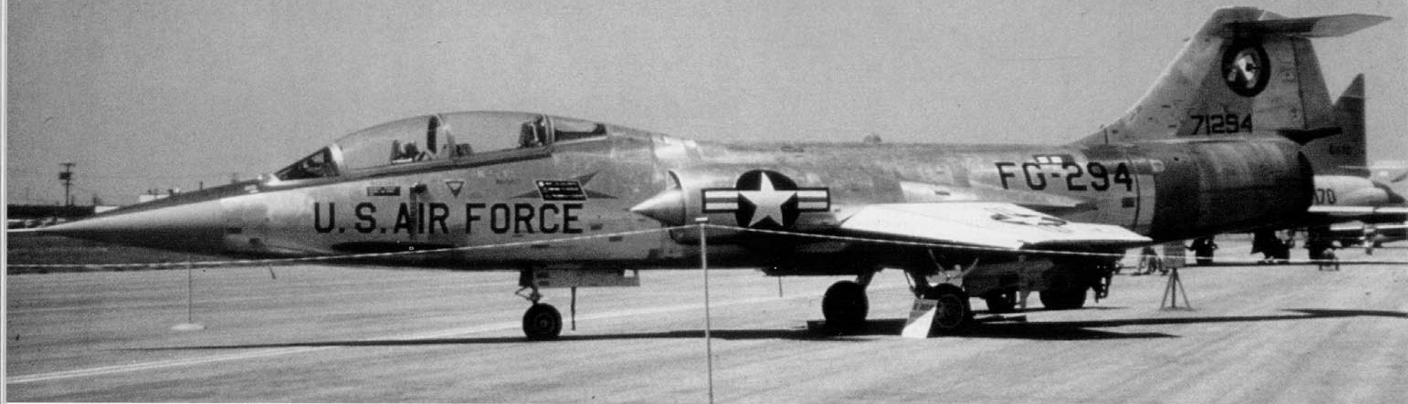
An F-104B of the 83rd Fighter Interceptor Squadron on display during an open house air show. The F-104B canopy had a narrow frame between the two individual cockpit canopy sections. The two seat Starfighter had the M61 cannon deleted and the opening faired over. (Via Larry Davis)
