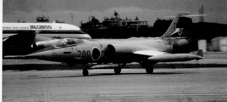
This F-104J (76-8700) of No 207 Squadron at Haha was painted Light Gray with White wings during 1979. Most of the stenciling on this F-104J was in Japanese, unlike NATO F-104Gs which carried at least a portion of their stenciling in English. (Toshiki Kudo via Rick Morgan)
