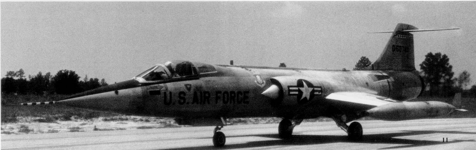
A piloted QF-104A drone (56-741) taxis in at Eglin AFB, Florida. The QF-104 also had provision for a pilot to allow the aircraft to be ferried between bases. The QF-104's color scheme of overall Dayglo Orange with White wings faded quickly, giving the aircraft a tattered and ragged appearance. (Marty Isham)
