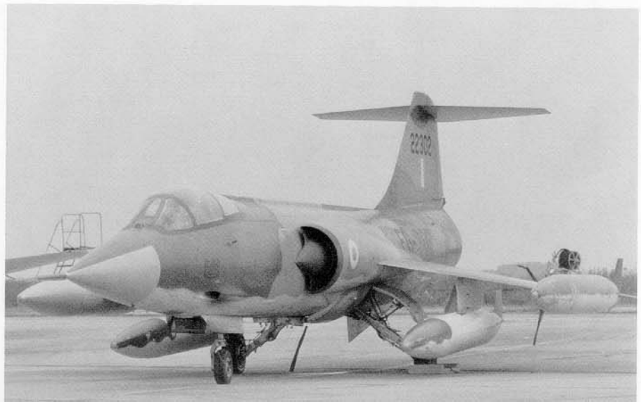
This Greek Air Force Starfighter of No 336 Squadron, No 116 Combat Wing was based at Araxos. Greek F-104Gs carried a camouflage scheme similar to the USAF Southeast Asia camouflage and carried a Buzz number on the rear fuselage. The lower half of the radome was Light Gray, with a Black anti-glare panel on the radome only. (John Kerr Collection)
