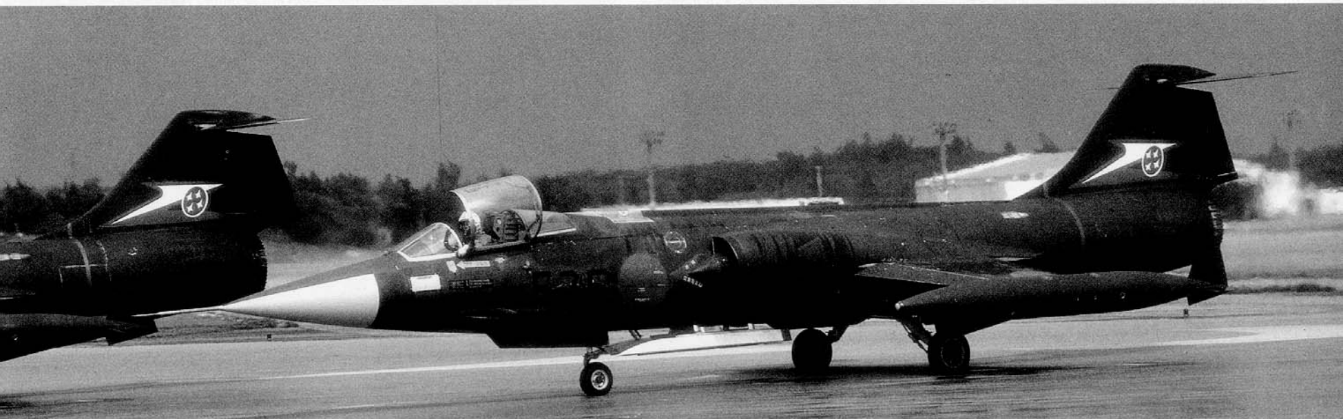
Another experimental camouflage scheme carried by F-104Js of No 207 Squadron was overall Dark Green. The Japanese national insignia was not outlined and all numbers were in black. This camouflaged tended to weather rapidly leaving the aircraft with a very streaky appearance. (Toshiki Kudo via Rick Morgan)
