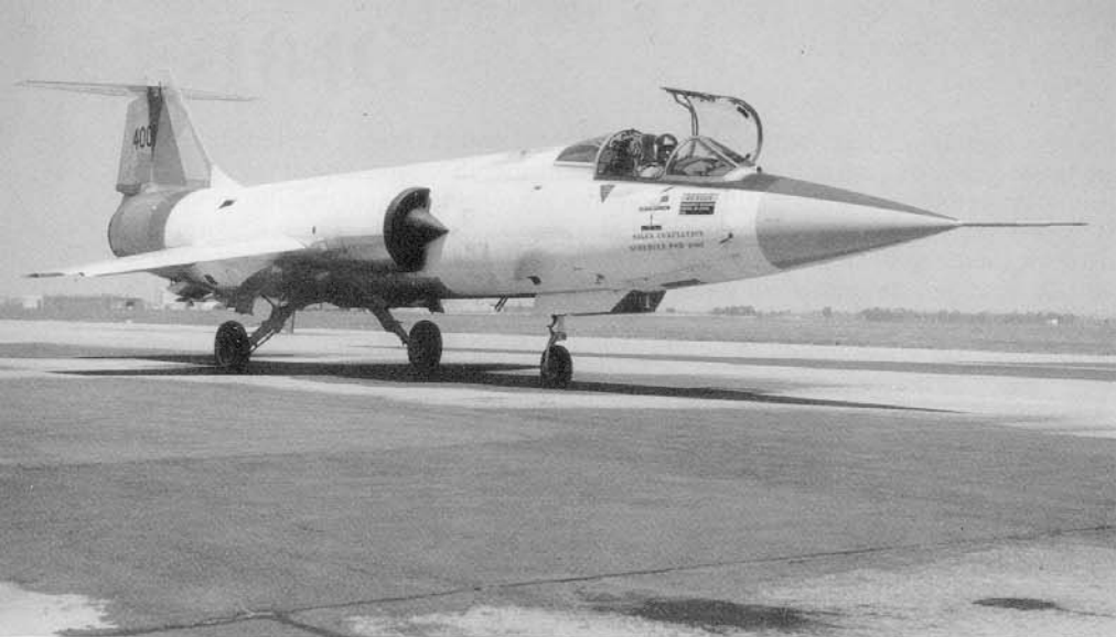
This F-104G was the first Military Assistance Program aircraft built by Lockheed and was completed on 10 August 1962. The dark areas on the intake lips are heating elements which were unique to MAP variants of the F-104G. The doors are still open on the braking parachute housing under the rear fuselage. (Isham Collection)
