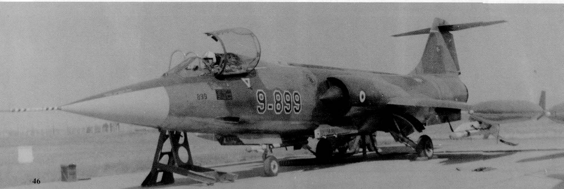
A Turkish F-104S of the 191st Squadron on alert armed with a pair of AIM-9 Sidewinders on the outboard missile rails. Turkish F-104S Starfighters carry reduced size national insignia, have the base/aircraft code number in Black outlined in White on the nose and the individual aircraft number repeated in Black just under the windscreen. (Oguz Meric)
