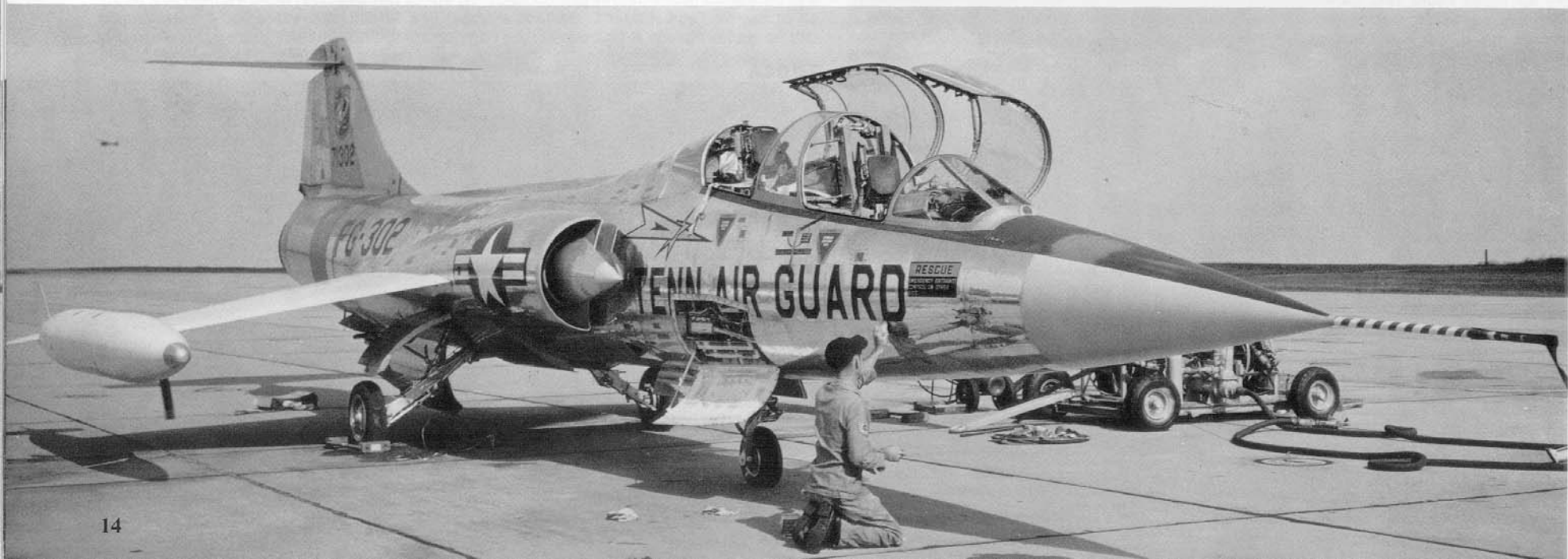
This F-104B of the 134th Fighter Group, Tennessee Air National Guard on the ramp of its home base, has the tip tanks painted white to match its White wings and has been retrofitted with an F-104D style canopy. This aircraft (57-1302) served with the 538th FIS, the 197th FIS (where it was crashed and rebuilt), the 331st FIS and the 4760th CCTS. It was finally was transferred to Jordan where it crashed March of 1967. (134th FG via Minert via Isham)
