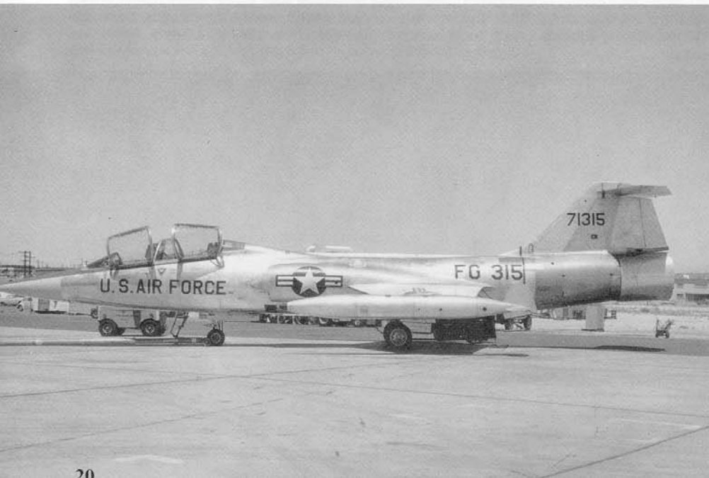
This F-104D (57-1315) on the ramp at China Lake was assigned to the AFFTC as a photo chase aircraft and carries the Air Force Systems Command insignia on the fuselage. The structure surrounding the afterburner nozzle was an experiment aimed at reducing the F-104's considerable infrared signature. (USN/Friddell Collection)
