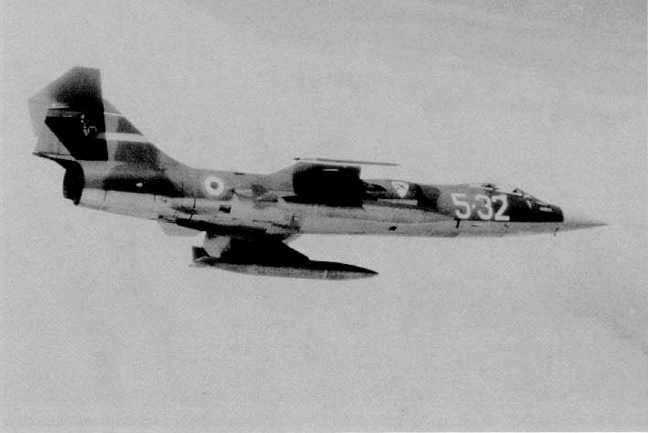
An F-104S of the 5th Stormo carries underwing fuel tanks and no other stores. The Yellow tail stripe extends in front and behind the Stormo badge although it is barely noticeable unless the aircraft is seen directly from or slightly below a level position. The code numbers on the nose are in White. (Italian Air Force)
