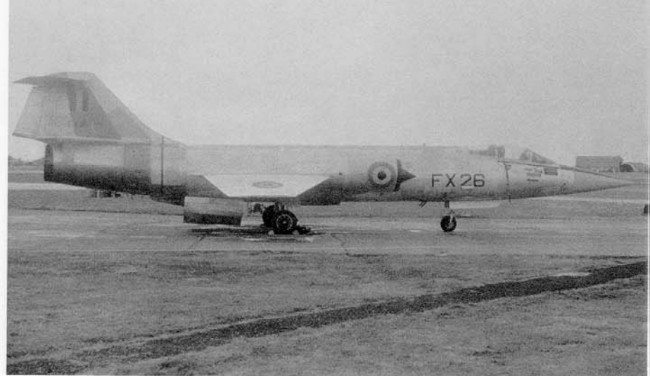
Most European air forces operated the F-104G in Natural Metal at one time or another. This F-104G, FX26 of No 1 Wing, Belgian Air Force carries no unit markings of any kind. The lack of wing tanks, however, indicates that it was an interceptor from either Nos 349 or 350 Squadrons. (Kerr Collection)
