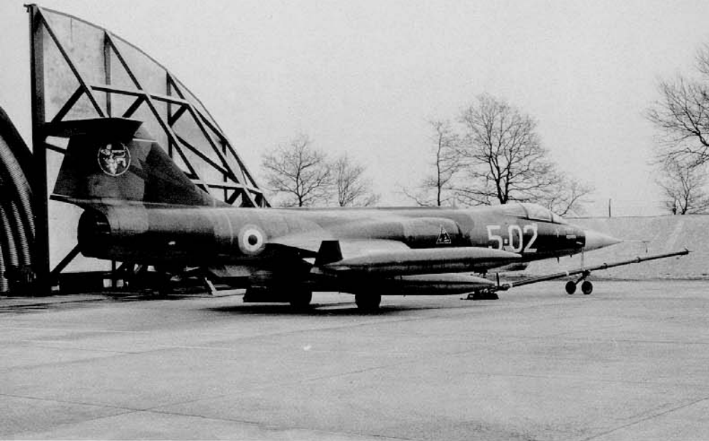
An F-104S/AS1 of the 5th Stormo, 102nd Squadron on the ramp outside a Hardened Aircraft Shelter (HAS). The 102nd Squadron is assigned the air-to-ground mission and the F-104S/AS1 is well suited to this role since the M61 cannon is reinstalled in this variant of the F-104S. (G. Beerens)
