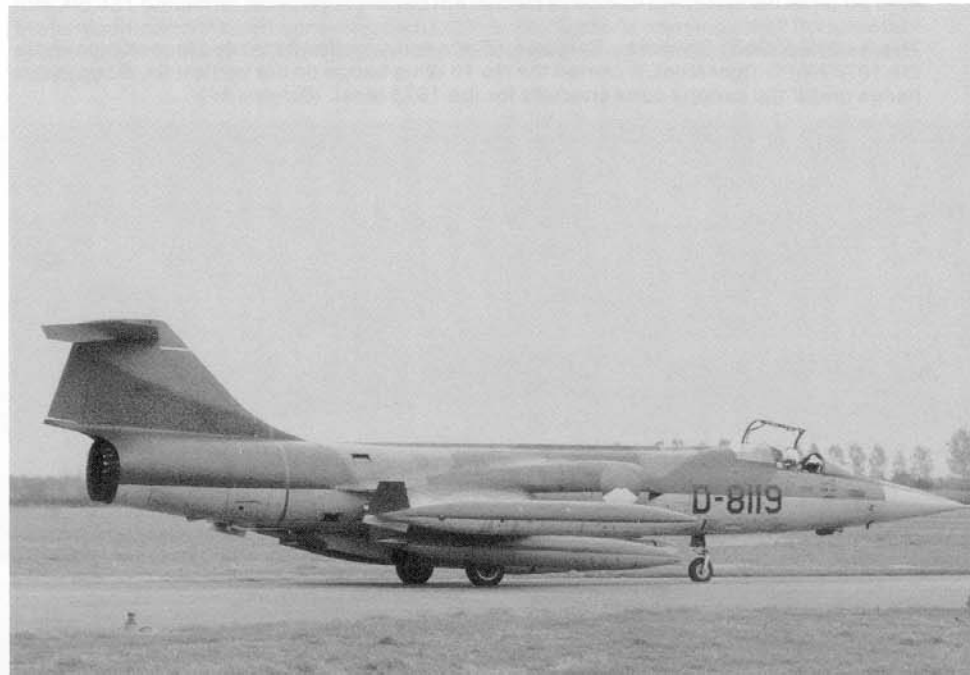
This Fokker-built F-104G of No 306 Squadron is equipped with an under fuselage camera pod and was based at Volkel. D-8119 carries no unit markings and is configured for long range operations with four external fuel tanks. This F-104G was one of the Dutch F-104s sold to Turkey during 1983. (Lee Bracken via Frank Garcia)
