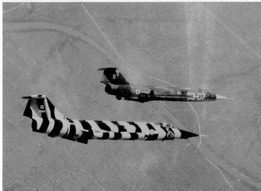
A tiger-striped CF-104 of No 439 Squadron flies past Hohenzollern Castle, Germany during June of 1977. The small wing makes the Starfighter relatively stable at low altitudes, making the CF-104 well suited for low altitude high speed ingress into a target area in time of war. This aircraft is fitted with rear-mounted Radar Warning (RAW) blisters and a under nose ECM blister. (Canadian Armed Forces)
