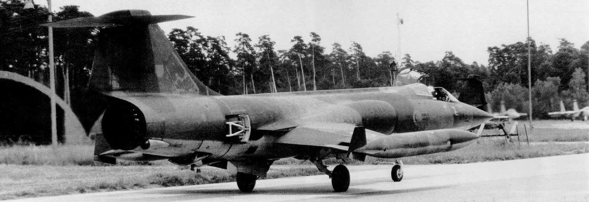
A CF-104 taxis in at CFB Lahr (West Germany) during September of 1980. The aircraft is painted in a two-tone Green and Gray upper surface camouflage over Light Gray undersurfaces and is carrying a practice bomb dispenser on the centerline station and rocket pods on the wing pylons. (Canadian Armed Forces)
