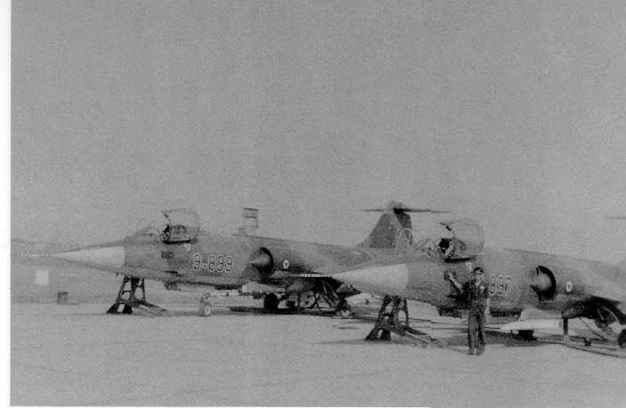
The F-104S was purchased by the Turkish Air Force to update its Starfighter fleet. Normal Turkish F-104S Starfighters do not carry the AIM-7, but use the underwing missile pylons carry a pair of AIM-9 Sidewinders. These aircraft belong to the 191st Squadron based Balıkesir. (Oguz Meric)
