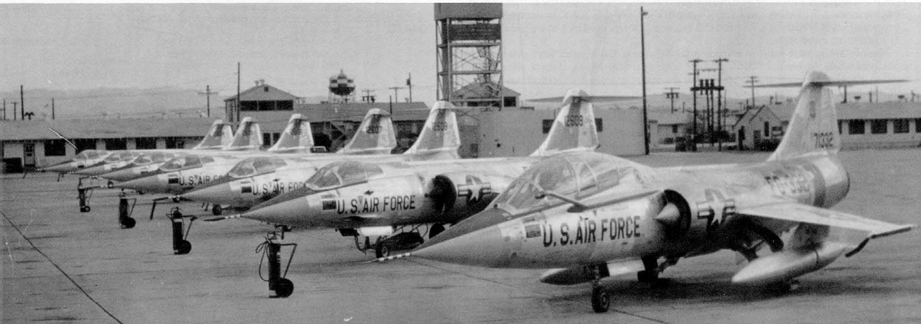
The German government realized early on that Germany was not the best place to teach new pilots how to fly the Starfighter. This F-104D from the 479th TFW was a German-owned, USAF operated F-104G on the ramp at Luke AFB. The F-104D is unusual in that it is configured with wingtip Sidewinder rails and underwing pylon fuel tanks. (Isham Collection)
