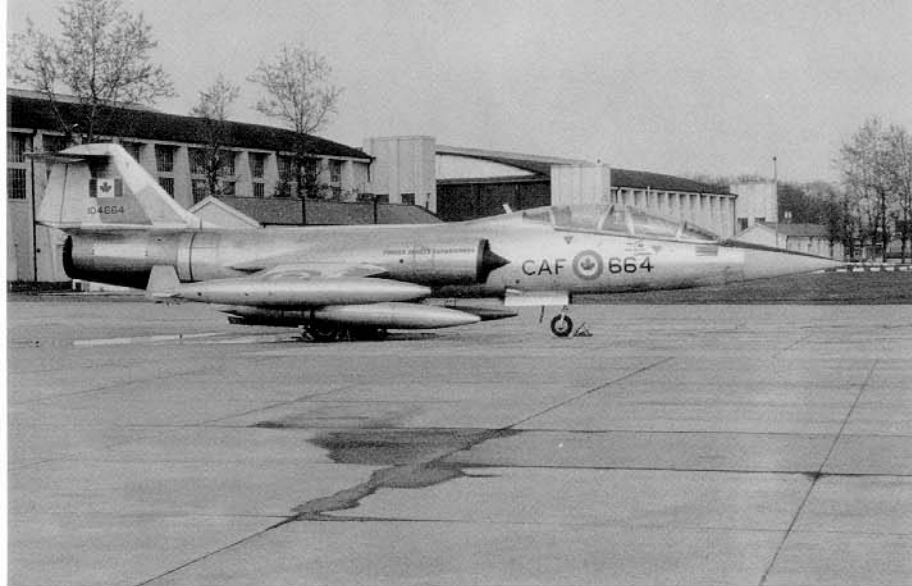
This CF-104D trainer carried the CAF legend in French on the starboard fuselage and in English on the port side in Red with Black shading. The CAF legend and aircraft number on the nose and aircraft serial on the tail were in Black. Canadian Starfighters had the prefix "104" applied in front of the aircraft's serial number starting in 1968. (John Kerr Collection)
