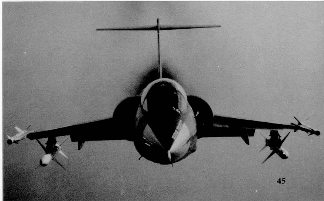
This F-104S carries the standard weapons load, a pair of AIM-9 Sidewinders and a pair of AIM-7F Sparrows, for Italian Air Force interceptors. The flaps and leading edge slats are fully deployed, indicating the aircraft is in slow speed flight. The smoke trail behind the F-104S is a trade mark of the J-79 engine. (Italian Air Force)
