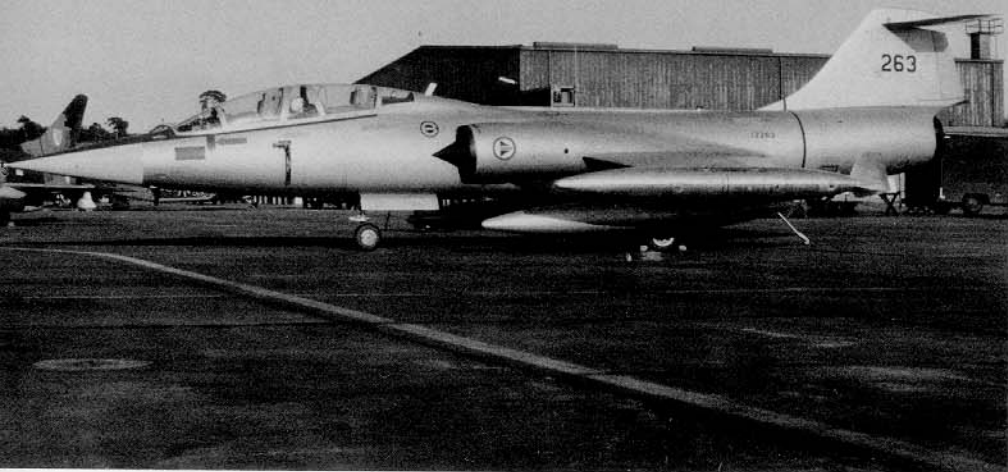
This overall Natural Metal TF-104G of No 331 Squadron Royal Norwegian Air Force carries no markings other than the serial on the fuselage and the individual aircraft number (last three digits of the serial) on the fin. The radome below the anti-glare panel is in Gloss Light Gray. (E. Jose)
