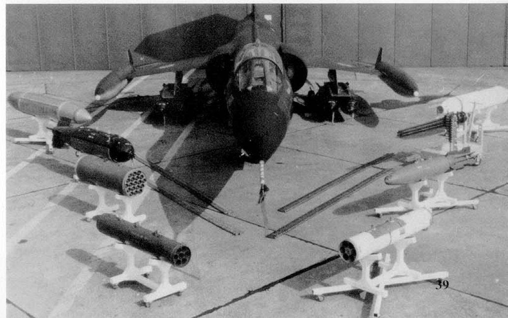
When the Canadians changed their European based Starfighters from Nuclear Strike to conventional ground attack in 1971, the M61 cannon was retrofitted into the aircraft. This display shows the gun and conventional ordnance carried by the CF-104, although the seven round rocket launcher was used for training only. (Canadian Armed Forces)
