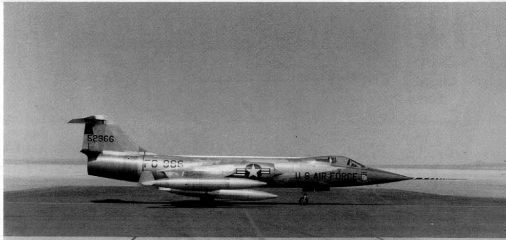
Many early Starfighters led multiple lives, 55-2966 was a YF-104A originally assigned to the Air Force Flight Test Center. The entire nose appears to have been painted Red-Orange and it was equipped with underwing tanks and a non-standard test boom in place of the pitot tube at Edwards AFB during May of 1959. During 1961, the aircraft was modified to QF-104A drone standards. (AFFTC/Isham Collection)
