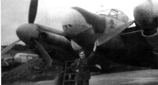
This Mosquito NF 30 had a cartoon figure painted on the fuselage under the cockpit. Some NF 30s had thimble nose radomes while others, such as this aircraft, had the bull nose radome fitted. (D. Howley)
