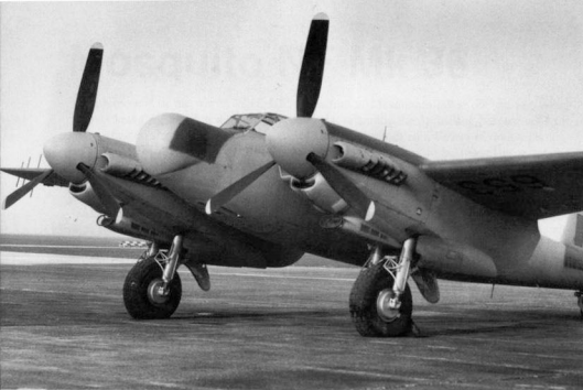
The Mosquito NF 38 was basically an NF 36 with uprated two-stage Merlin engines and AI Mk IX radar. Most NF 38s went to overseas customers and very few served as front line night fighters with the RAF.
