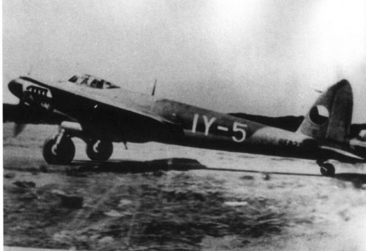
The Czech Air Force operated a number of Mosquito FB Mk VIs that they brought back from England after the end of the Second World War. These aircraft were given the local designation B/LB 36 and were flown until replaced by Soviet Il 2 and Il 10 aircraft during 1950.
