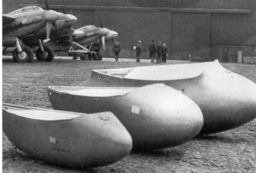
The three types of drop tanks used by Mosquitoes were the 50, 100 and 200 (Imperial) gallon tanks.
