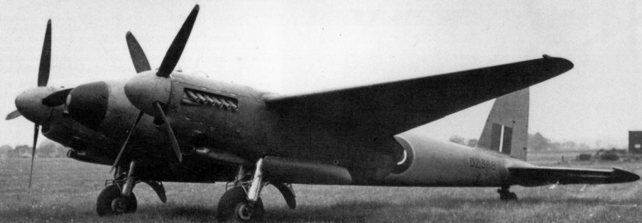
Long Span Wing Merlin 73 Two Stage Engine Four .303 inch Machine Gun Pack
