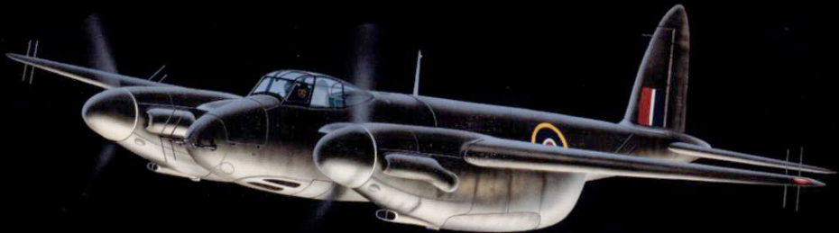
Mosquito NF IIs carried an overall Black camouflage and had the antennas for the MK IV air intercept (AI) radar on the nose and wing tips.
