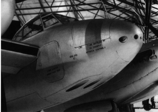
The business end of the armed Mosquito T Mk III (TW117) held by the Royal Air Force Museum at Hendon, London, lacks the familiar barrels of the four .303 inch Browning machine guns. Some Mosquito T Mk III were armed for the gunnery training role. (Peter Cooksley)
