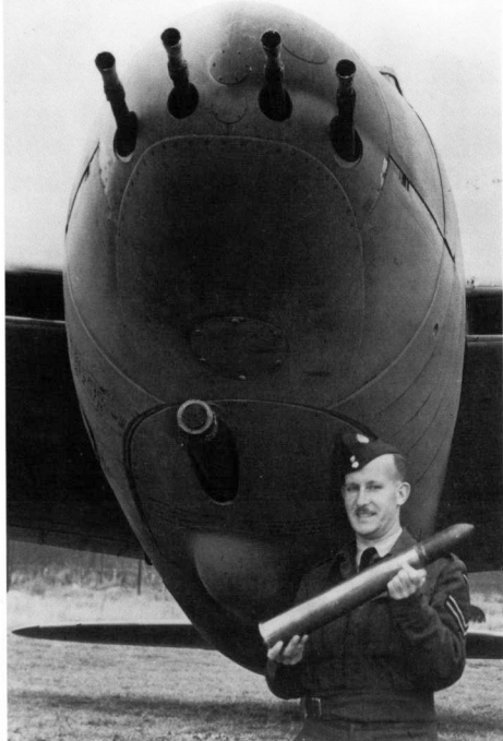
An RAF armorer holds one of the 57mm shells fired by the Molins gun carried on the Mosquito FB Mk XVIII. These aircraft were nicknamed Tsetse Mossies and carried a total ammunition load of twenty-five rounds for the cannon.
