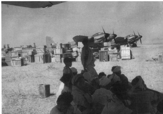
A pair of SEAC Mosquito FB VIs surrounded by supplies and Burmese bearers on a forward airstrip during March of 1945. Interestingly, both Mosquitoes (believed to be from No 82 Squadron) retain exhaust flame-dampers in an area of operations where these were not needed. (Aeroplane)
