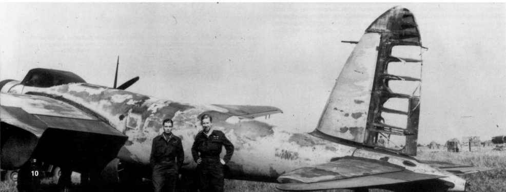
This Mosquito NF XIII of No 264 Squadron landed on a Normandy airstrip on 8 August 1944 after shooting down a Ju-88 bomber. The German aircraft exploded and the Mosquito crew was unable to avoid the blast. The resulting fireball burned off the fabric of the rudder and most of the aircraft's paint.
