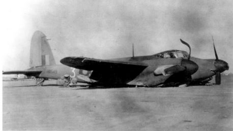
This Fb Mk VI (HR549/3) of No 1672 Conversion Unit at Yelahanka, India made a belly landing after its port wing tip was damaged and the main landing gear failed. The engines were still running at the time of the crash and both propellers are bent. It is unlikely that a Mosquito could be repaired after receiving this degree of damage. (Robertson)
