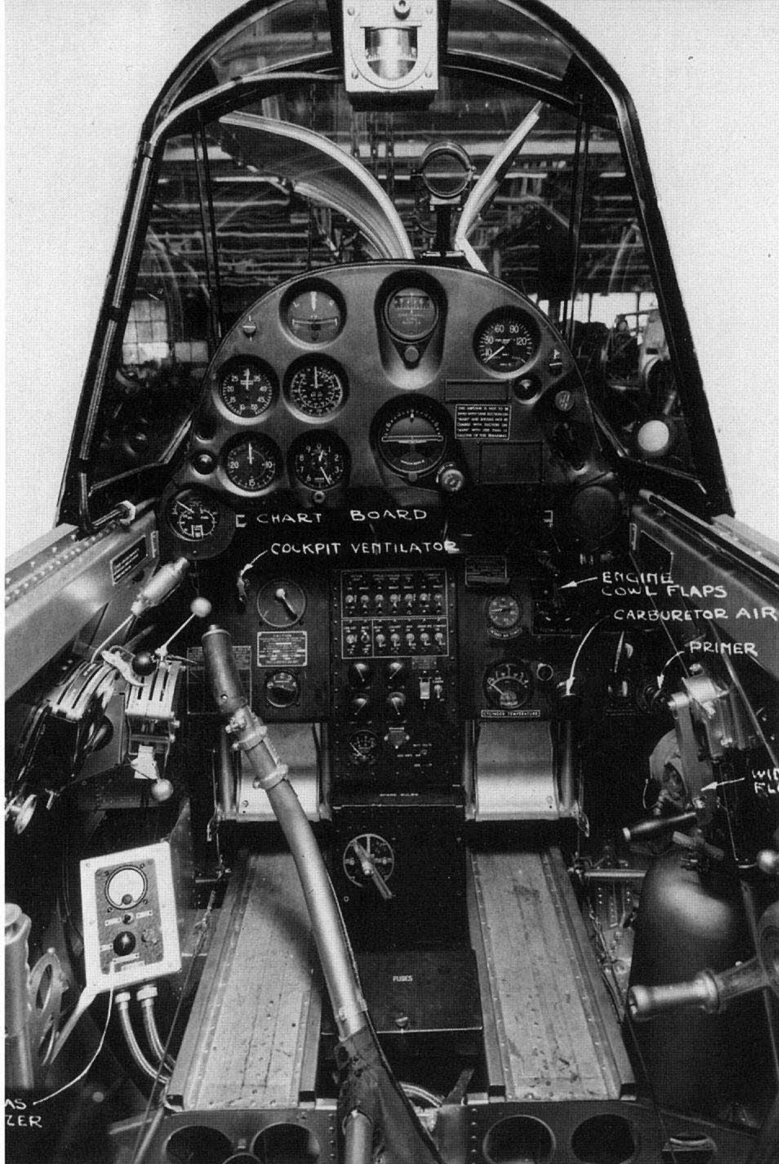
The front cockpit of a SBC-3 Helldiver. The circular object above the instrument panel was the telescopic gun sight. The rudder peddles were located just below the instrument panel. (National Archives via R.J. Cressman)
