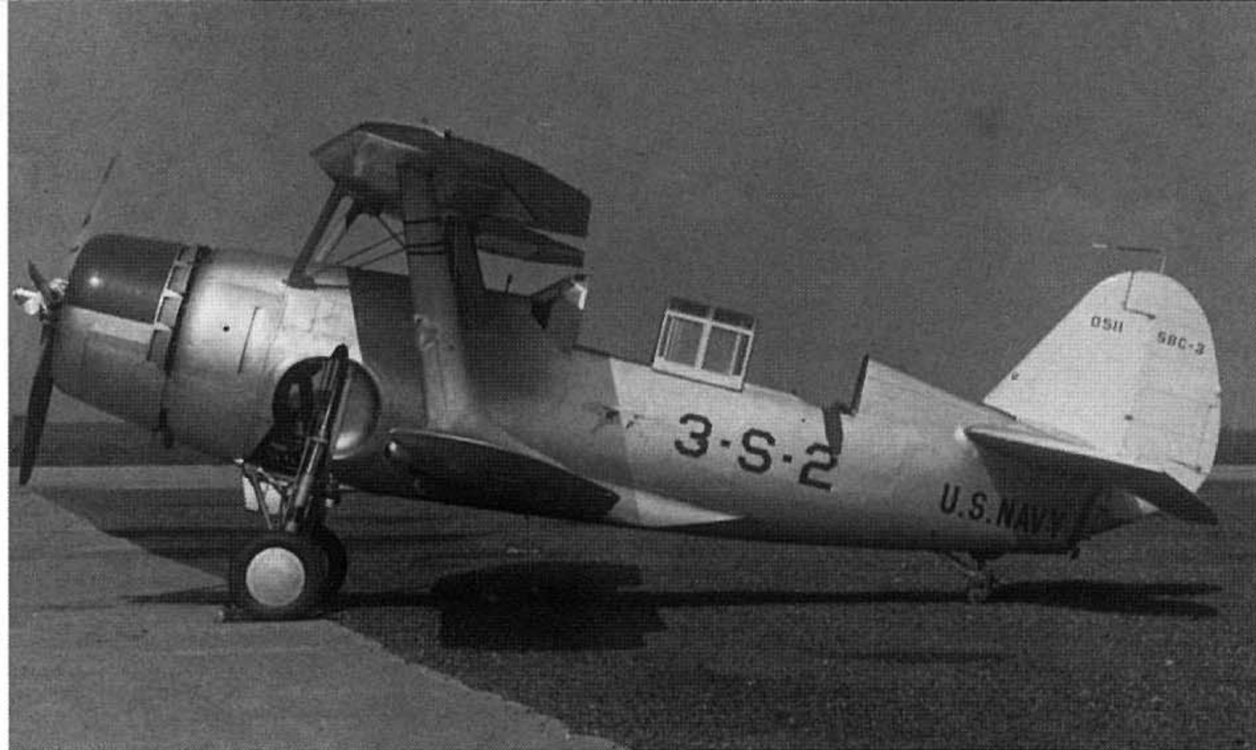
This is aircraft number 2 of section one of VS-3 during 1938. The top of the cowling was Red and the "Pointer Dog" squadron insignia was carried on the fuselage side below the pilot's cockpit. This aircraft was lost at sea on 29 August 1939, while serving with VS-5. Originally delivered on 29 August 1937, it had logged a total of 381.7 flight hours before its loss. (W.T. Larkins)
