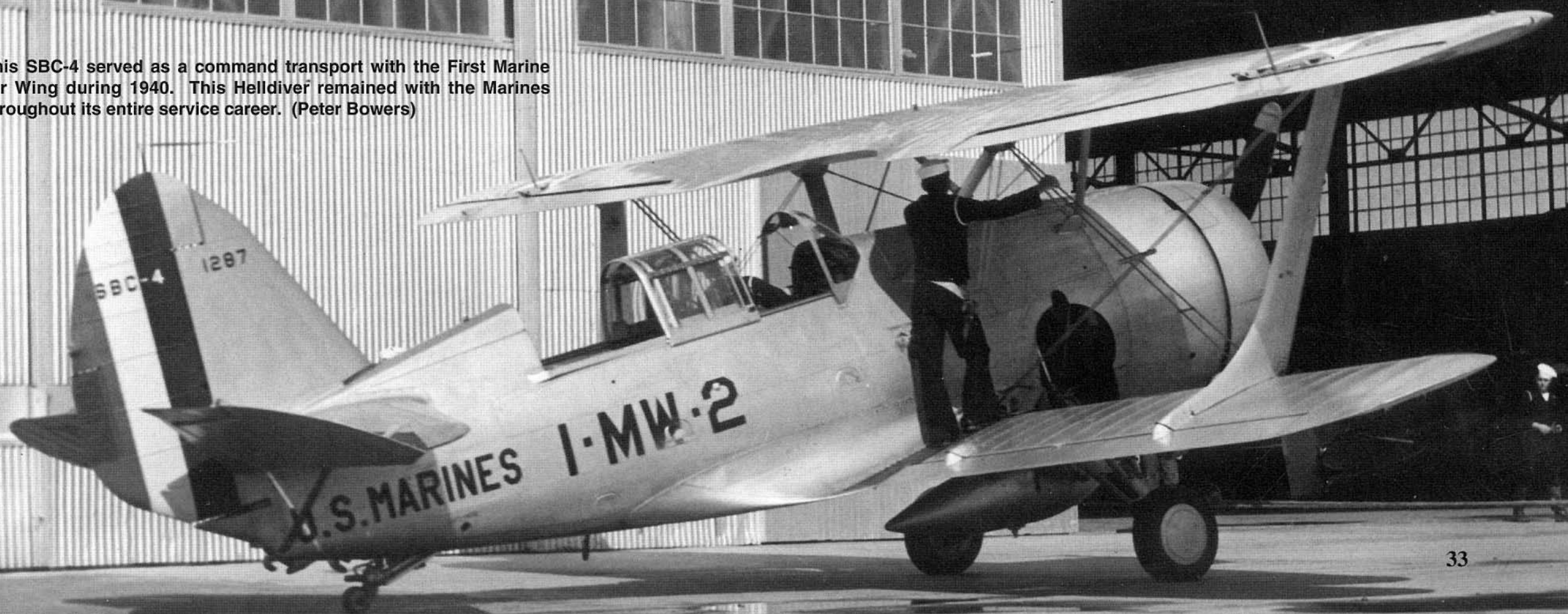
Navy mechanics change the engine on a SBC-4 at NAS Norfolk, Virginia during 1941. Aboard ship it took approximately 140 man hours to change the engine, since only three men at a time could actually work on the project. (Navy)
