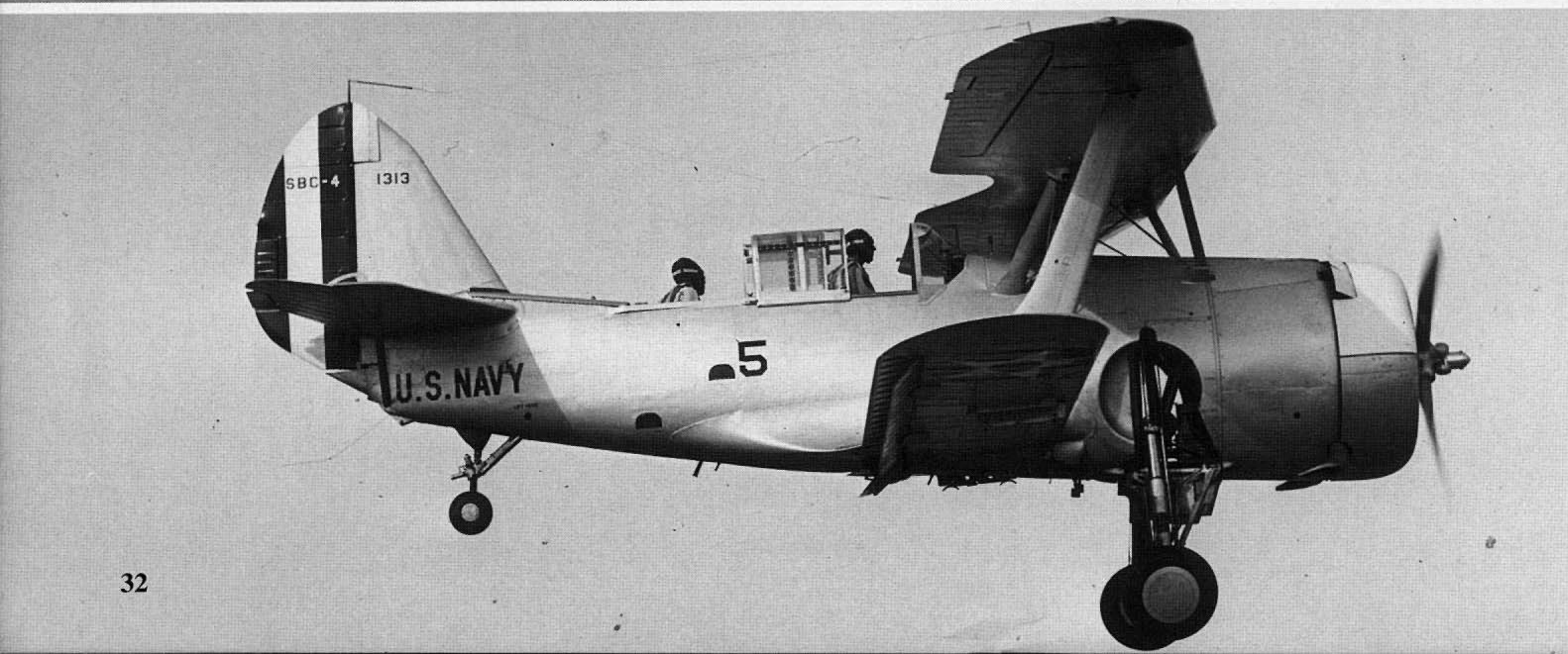
NRAB Oakland's SBC-4 Number 5 comes in for a landing with everything down but the arresting hook (it did not have one). The turtledeck behind the rear cockpit has been folded down. (W.T. Larkins)
