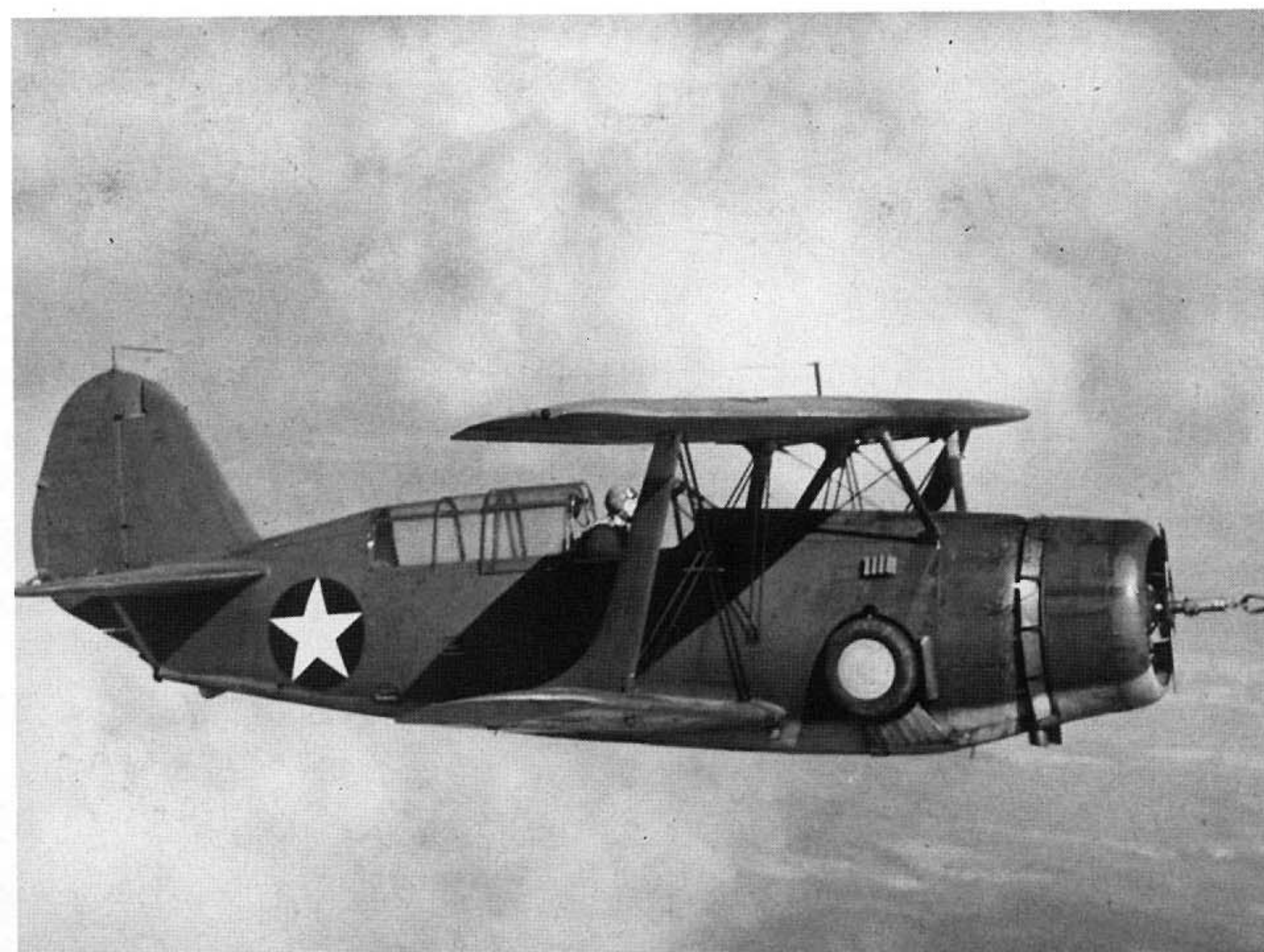
This SBC-3 was towed back to its home base after the engine seized on a cross-country flight. The propeller was removed and a PBY-5A served as the tow aircraft. The aircraft was camouflaged in Non-specular Blue Gray over Light Gray. The national insignia indicates that the incident took place between mid-May of 1942 and June of 1943. (Navy/National Archives)
