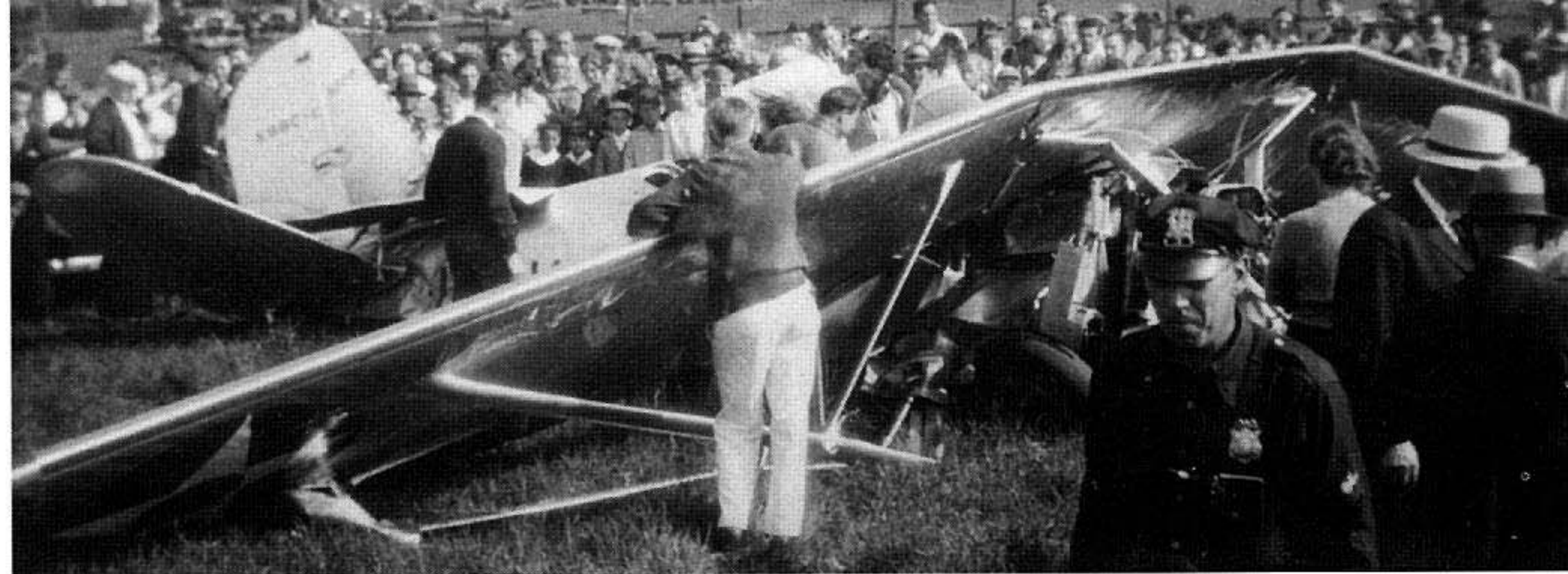
The XSBC-1 crashed on 14 June 1934, after a propeller blade separated in a high speed dive. The pilot escaped with a broken arm and leg. (Thorell Aircraft Photos via Peter Bowers)
