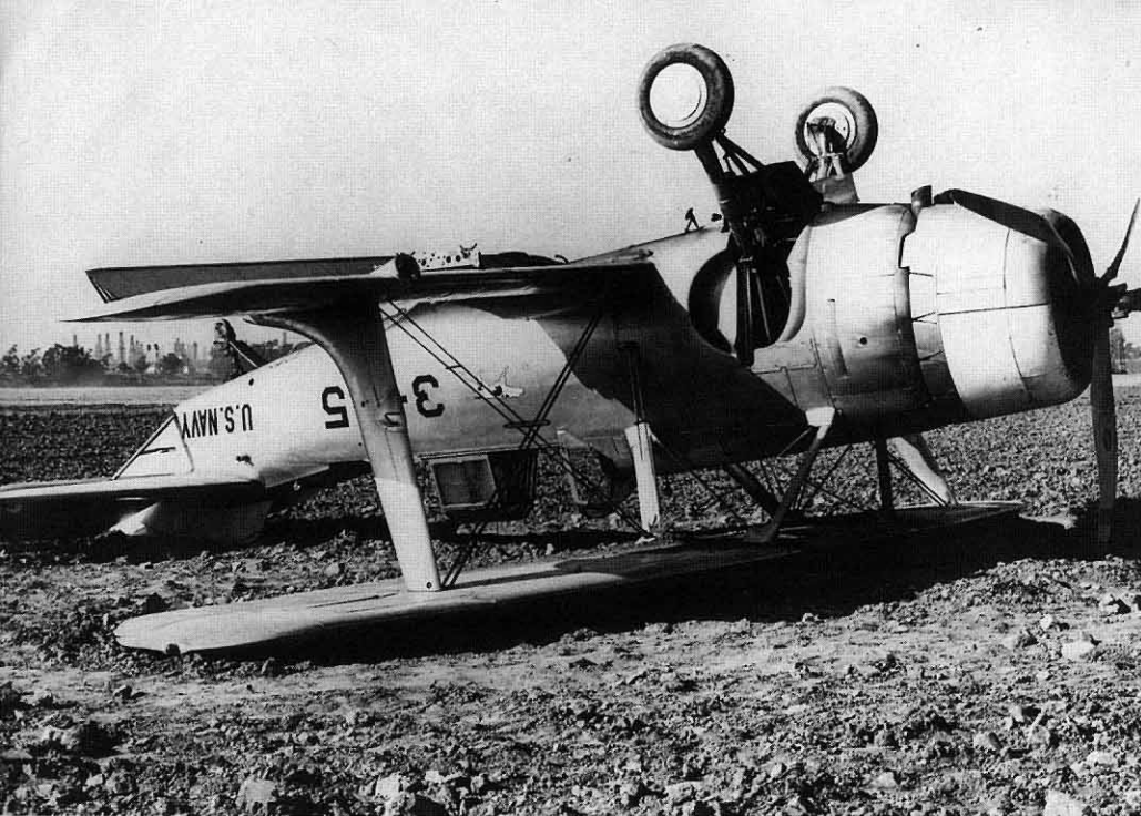
This SBC-3, Three-Sail-Five of VS-3, rests on its upper wing after turning over on landing. The damage was limited to the upper wing and vertical fin. The aircraft has a bomb rack installed on the lower wing undersurface. (Navy via D. W. Lucabaugh)
