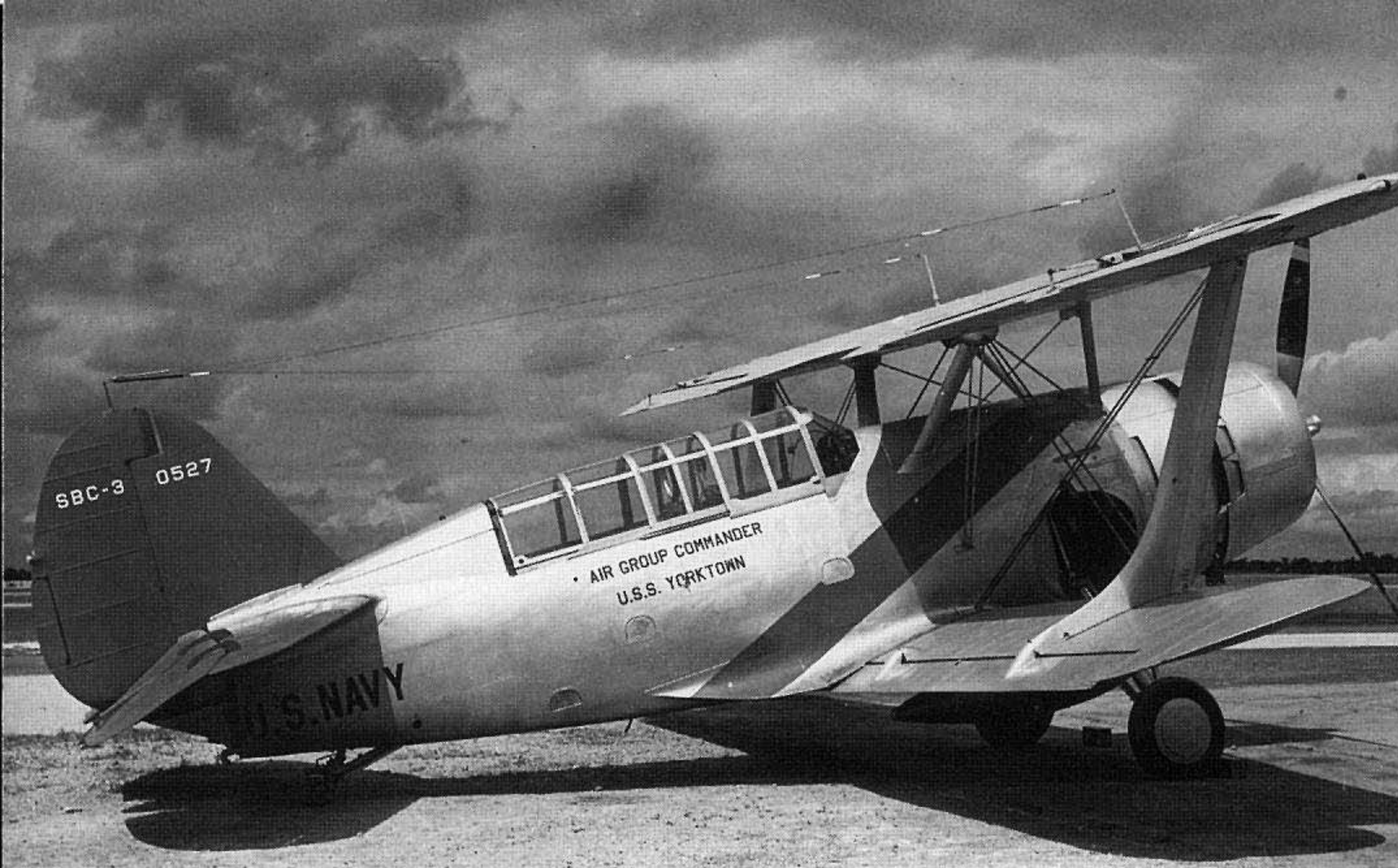
This SBC-3 Helldiver (BuNo 0527) was flown by the Air Group Commander of USS YORKTOWN during 1940. The diagonal fuselage stripe and tail were in Red, the color assigned to all squadron aircraft attached to USS YORKTOWN (CV-5) at the time. (D. F. Kauer via W. T. Larkins)
