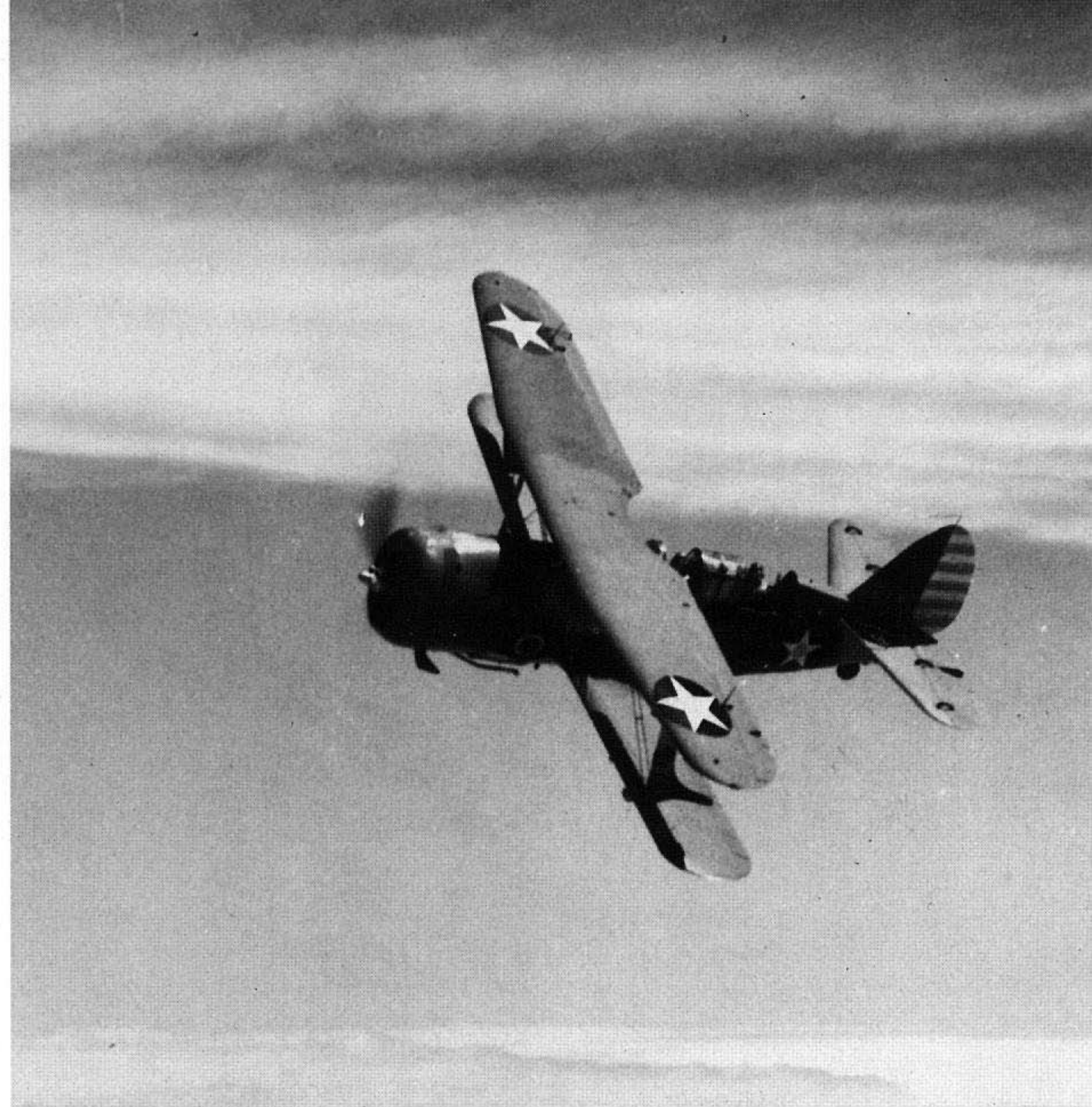
This SBC-4 was assigned to the Headquarters Squadron of the First Marine Air Wing during early 1942. At this time there were two SBC-4s assigned, BuNos 4222 and 4225. The aircraft was camouflaged in Non-specular Blue-Gray over Non-specular Light Gray with full rudder stripes. The tail stripes were carried between 5 January 1942 and 15 May 1942, after which time they were deleted. (USMC)
