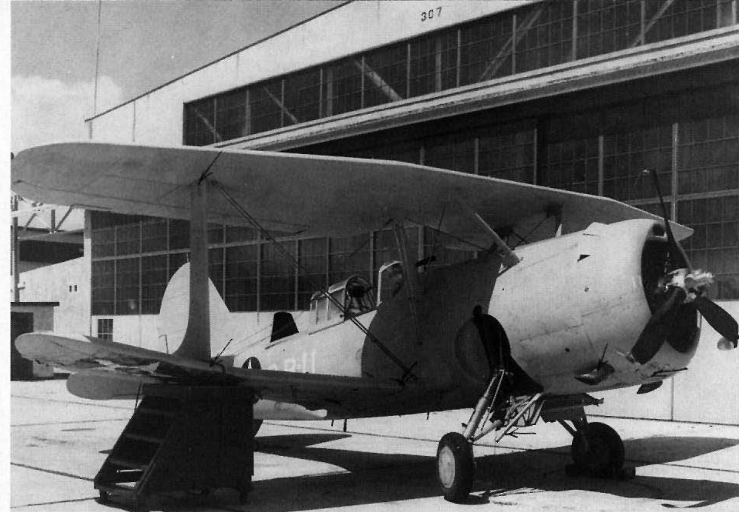
3-B-11 rests on a work stand after a landing accident at Naval Air Station North Island, San Diego, California. The landing gear truss failed during landing, leading to a collapse of the gear. The damage was not too severe and the aircraft was repaired and placed back into service. (Navy via D.W. Lucabaugh)
