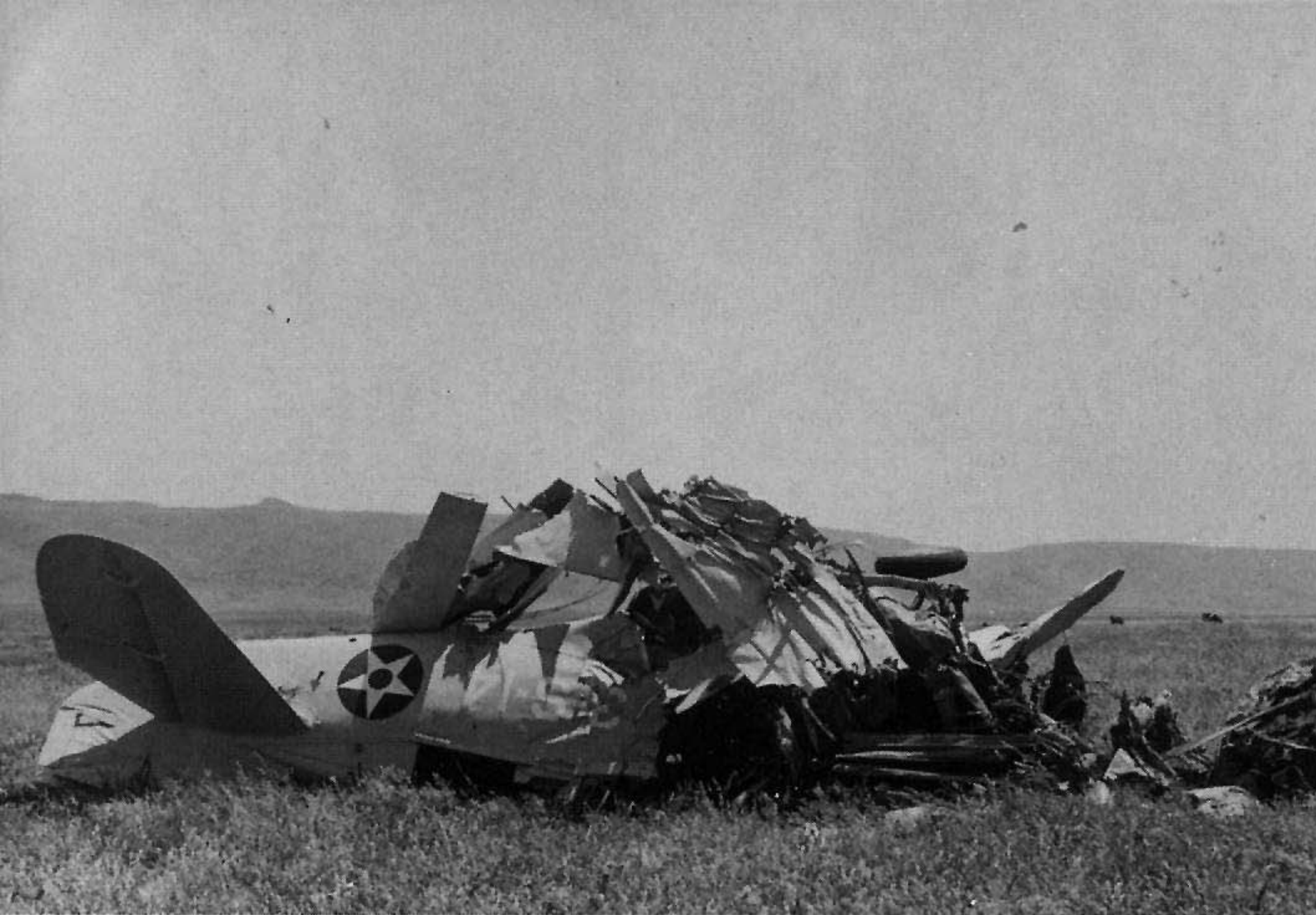
This SBC-4 was totally destroyed after the crew abandoned the aircraft in flight near the California/Mexico border on 5 May 1941. The aircraft had been delivered on 25 February 1941 and had only 49.3 hours on the airframe at the time of the accident. Cause of the crash was engine failure. (Navy via D.W. Lucabaugh)
