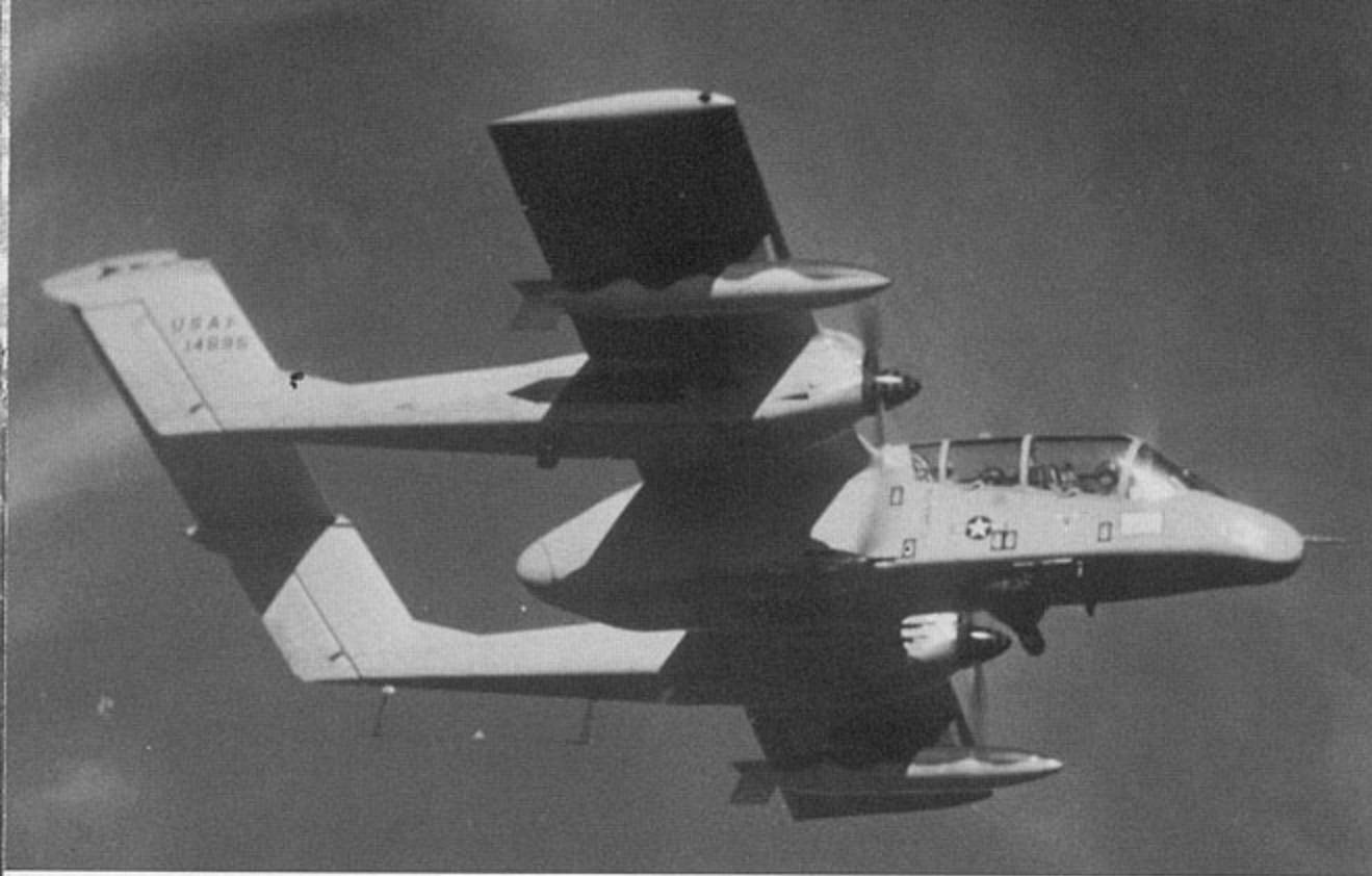
The Air Force also tried to improve the effectiveness of the Bronco at night and in poor weather under the Pave Nail configuration. Operated by the 23rd Tactical Air Support Squadron the laser pod under the fuselage was used to locate or designate a ground target. Fifteen of these aircraft were acquired and used until 1974. (USAF)
