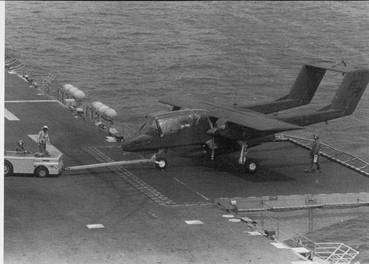
Marine OV-10As and later OV-10Ds have been active in flying off the Tarawa Class Amphibious Assault Ships (LHAs). This OV-10A is being towed by a MD-3A tractor to a new parking position aboard USS NASSAU (LHA-4) during 1983. (USN)
