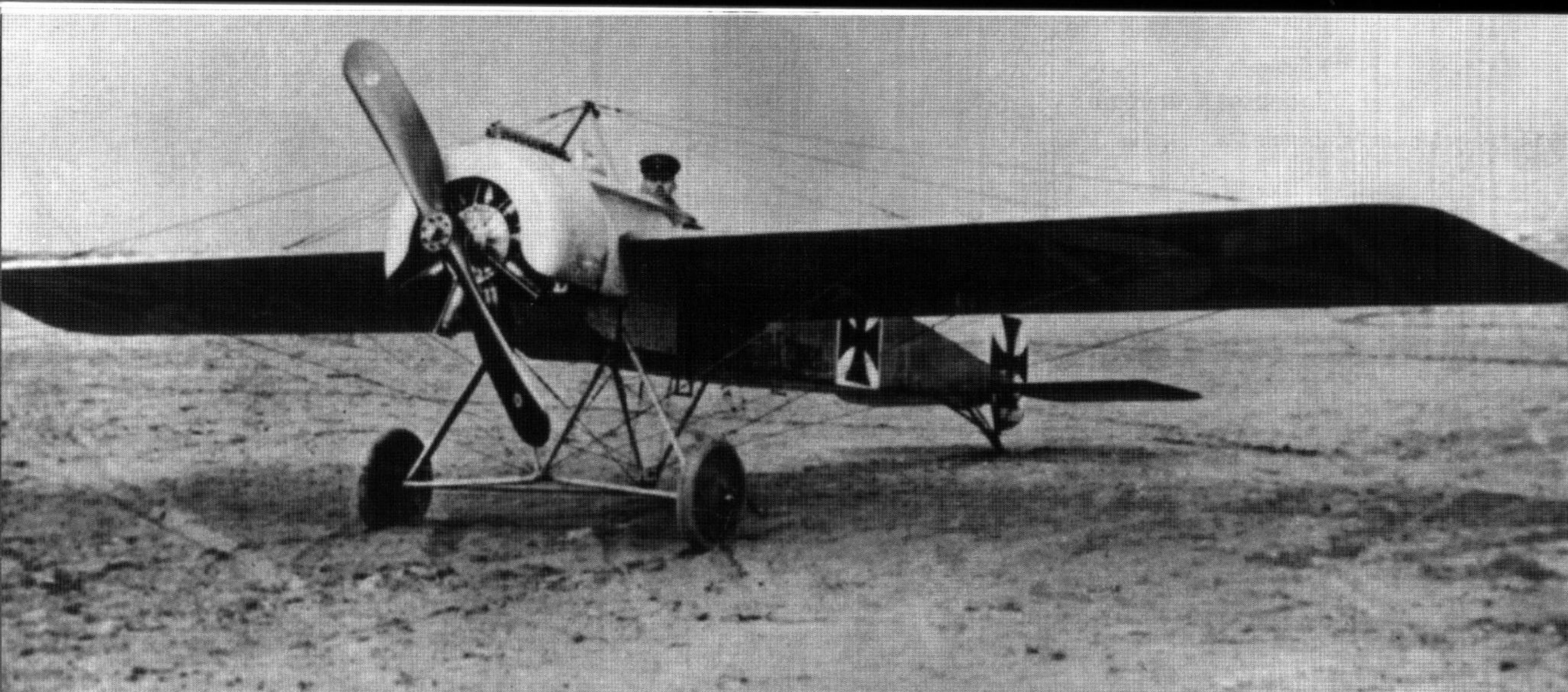
An unknown German Army pilot in the cockpit of a Fokker M.14V (E.III). It is believed that this aircraft is E.III 20/15, an early production aircraft. (Bowers)
