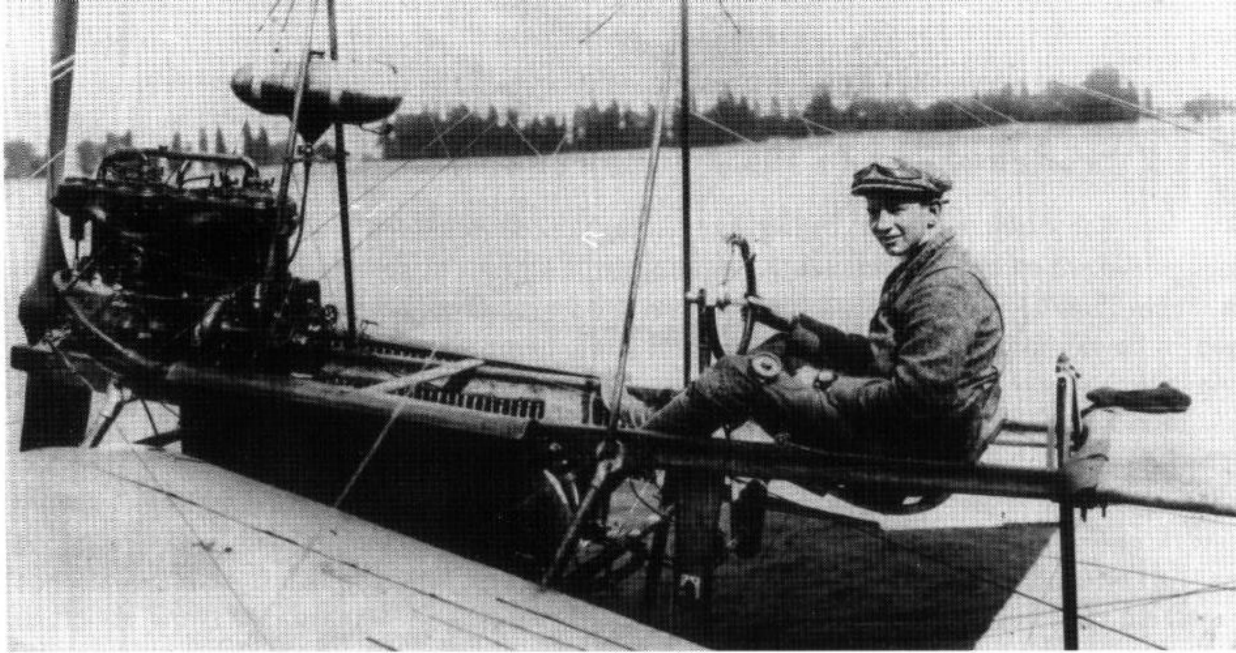
Anthony Fokker in the cockpit of the original Spin 3 in August of 1911. The aircraft used "wing warping" for control, and was steered by a control wheel. (Bowers)
