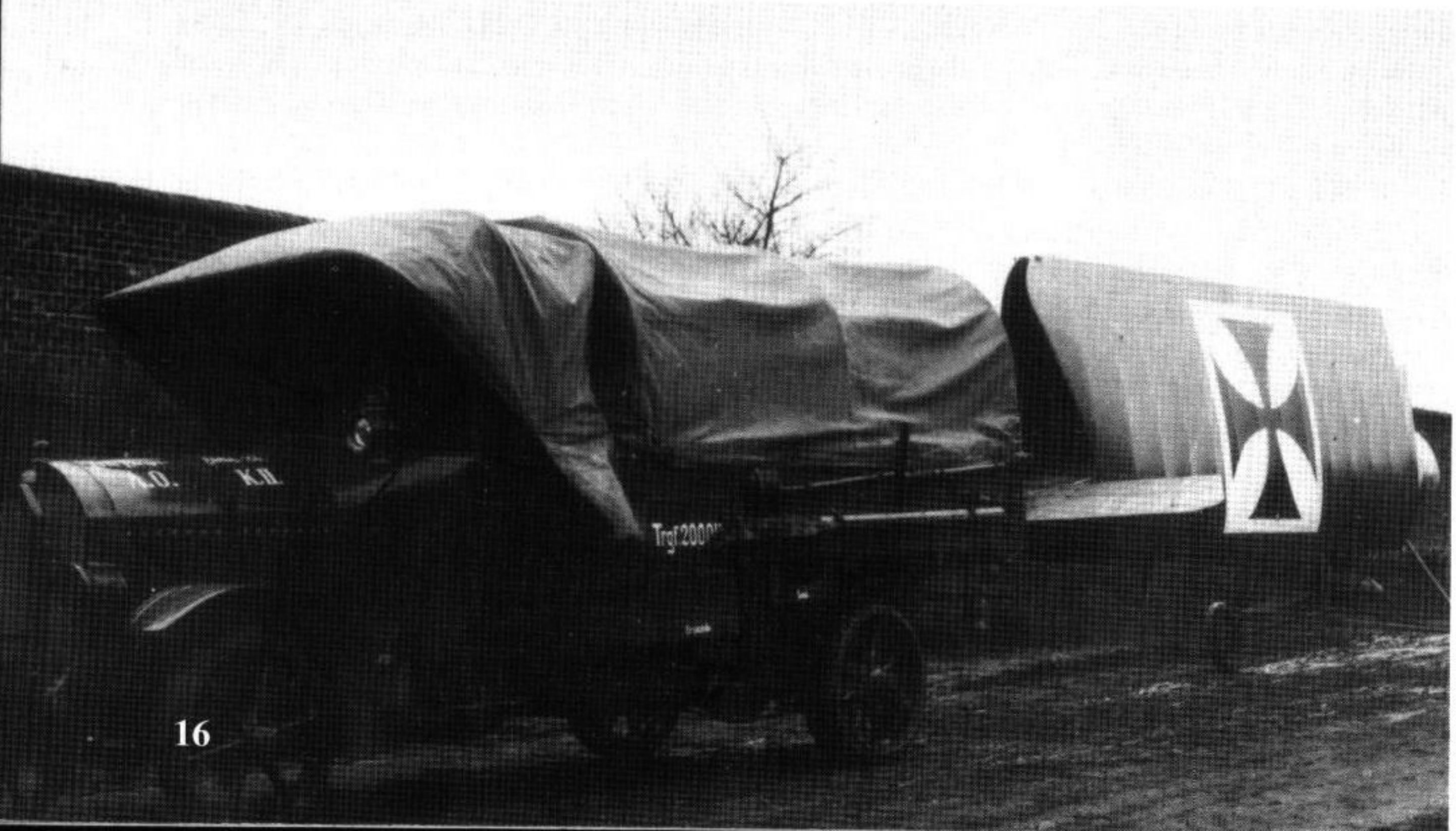
A truck with an M.5K.MG (E.1) in tow ready for delivery to a front line unit. This was a common method of delivery for new production aircraft. (Grosz)
