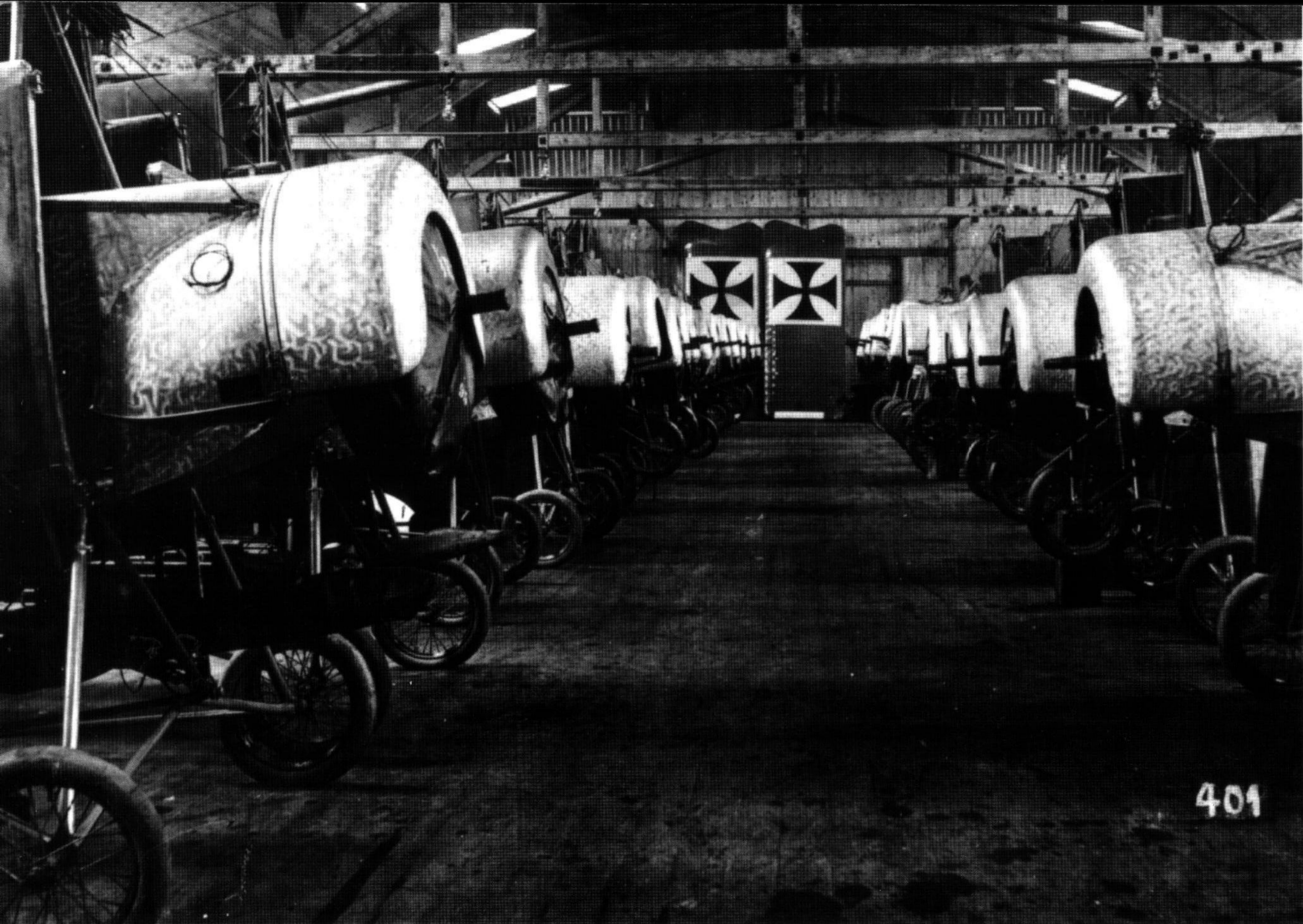
Fokker M.8s (A.I.s) under construction in the Fokker factory at Schwerin. The M.8 was a artillery-spotter aircraft with side-by-side seating for its two man crew. The aircraft was some forty percent wider than the Fokker E series fighters. The aircraft were used operationally by Feldfliegerabteilungen 40 and 41 until late 1915. (Fokker).
