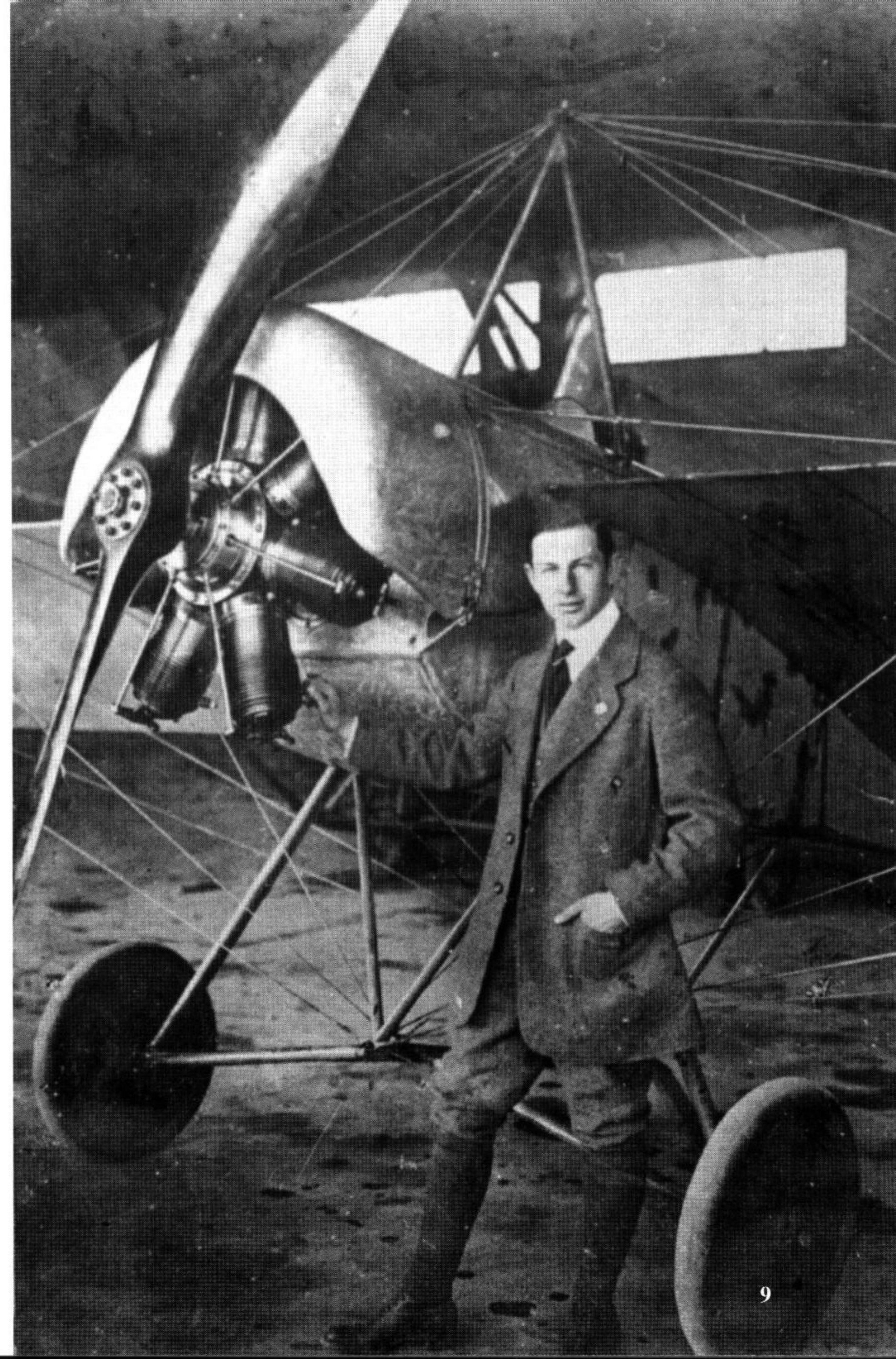
(Above and Right) Anthony Fokker poses with a Fokker M.5L (A) unarmed reconnaissance scout on the factory grounds. The M.5L had a longer wing span and much taller support strut in front of the cockpit than the M.5K. (Bowers)
