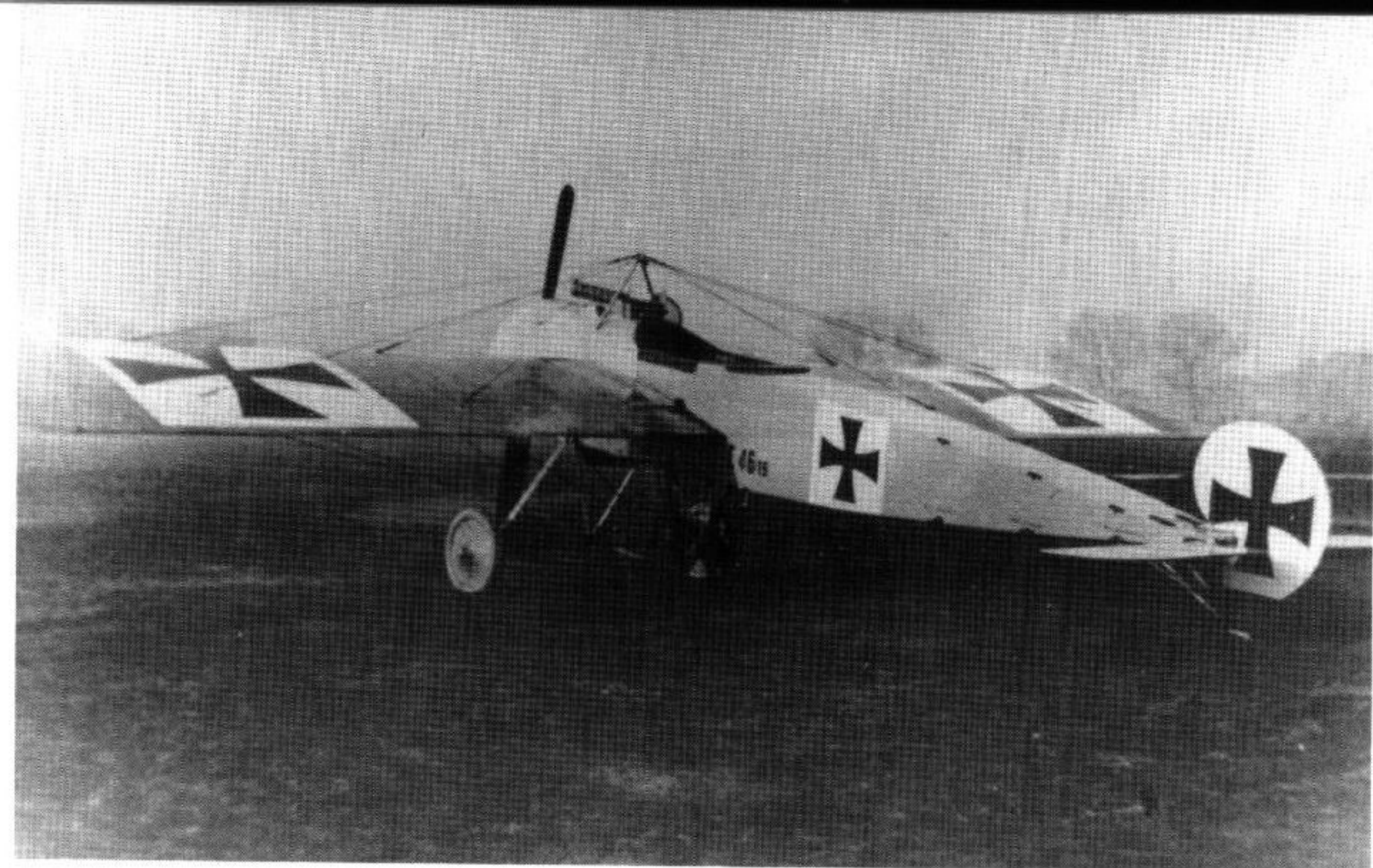
The longer "bathtub" cockpit of the M.5K/MG (E.1) is quite evident. This aircraft was serial 46/15. (Bosers)
