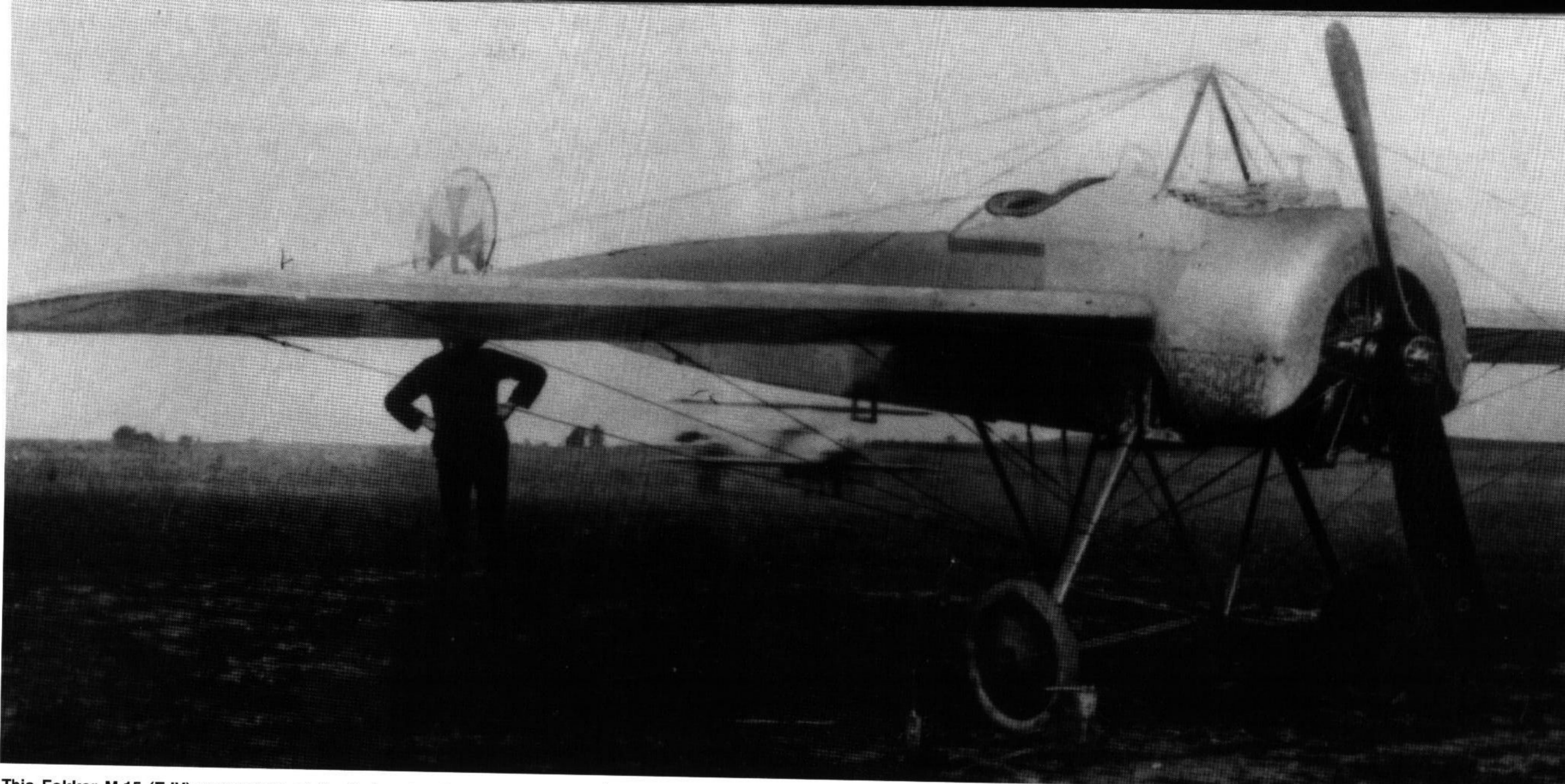
This Fokker M.15 (E.IV) was set up at the factory to shoot a number of documentation photos of the three machine gun installation. Although Boelcke tested such a gun installation, he reportedly disliked it. (Fokker)
