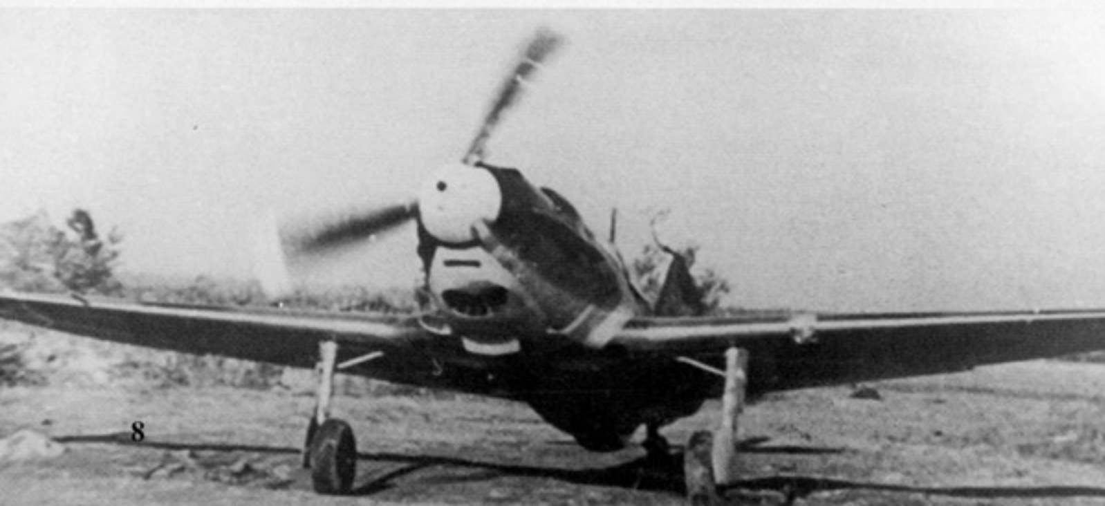
A LaGG-3 (1st Series) runs up its engine as it is prepared for a mission. The propeller was painted White and the muzzle of the engine mounted Berezin UBS 12.7MM machine gun is visible in the center of the spinner. (Robert Bock)
