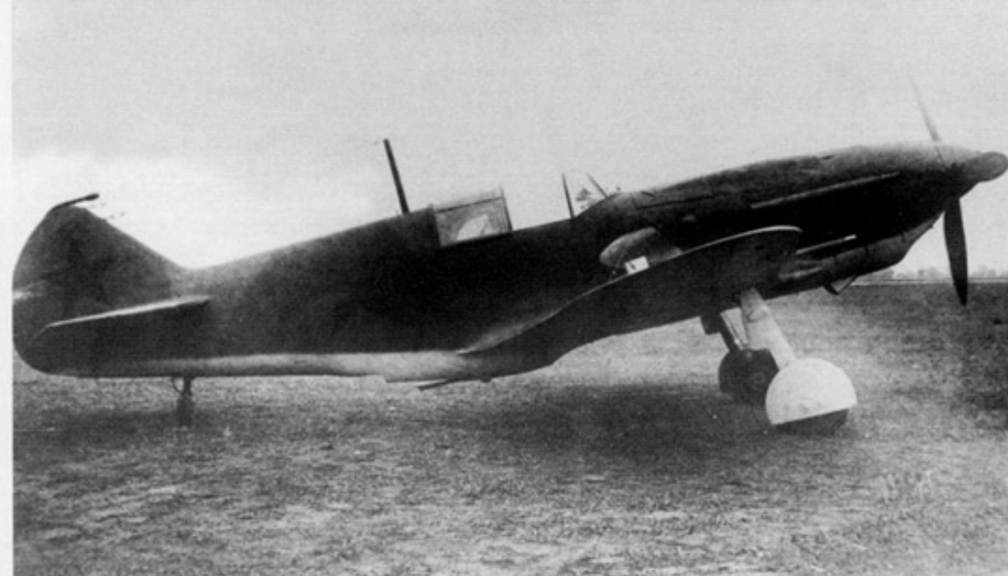
A LaGG-3 (6th Series) assigned to the Flight Research Institute at Zhukovsky for trials with the leading-edge automatic slats, a feature which was later made standard on the 22nd Series LaGG-3. (Ivan Ivanov)
