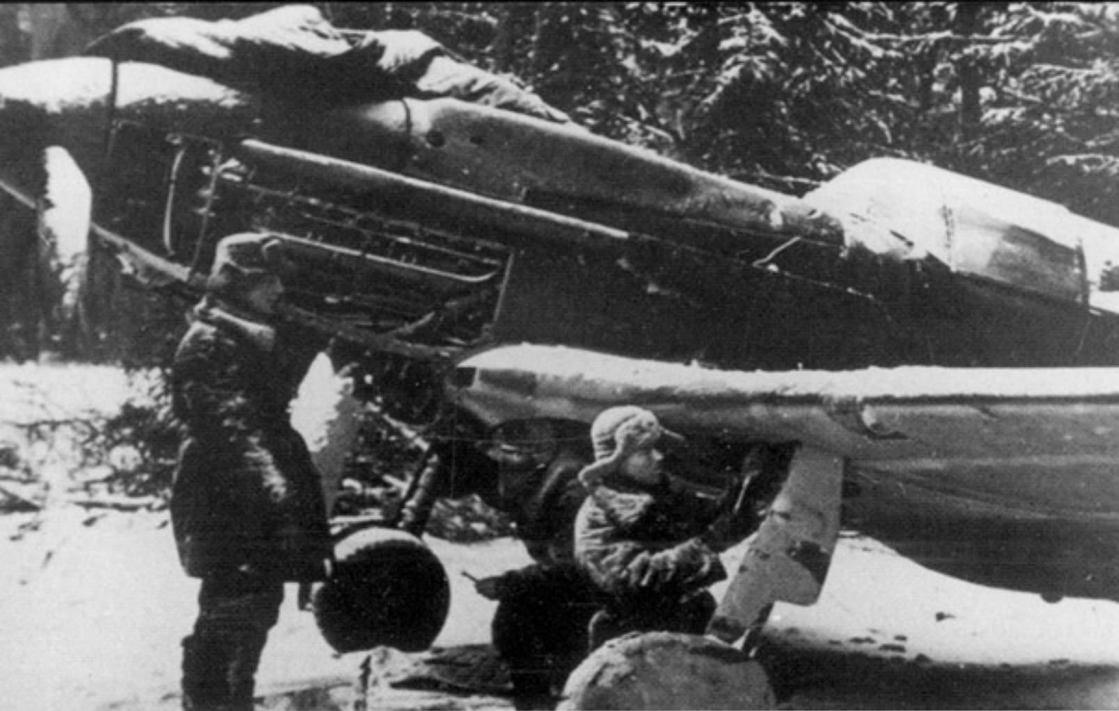
Ground crewmen perform maintenance work on a LaGG-3 (4th Series) in the harsh winter conditions of early 1942. The aircraft was assigned to the defense of Moscow. The rectangular wing root air intakes were introduced on the 4th Series LaGG-3. (Ivan Ivanov)
