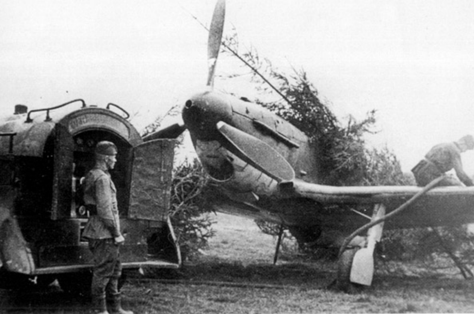
Camouflaged with foliage, this late production LaGG-3 (35th Series) was refueled on an airstrip on the Kalinin front in May of 1943. The air intake just above the wing root was a feature found on late production LaGG-3s. (Ivan Ivanov)
