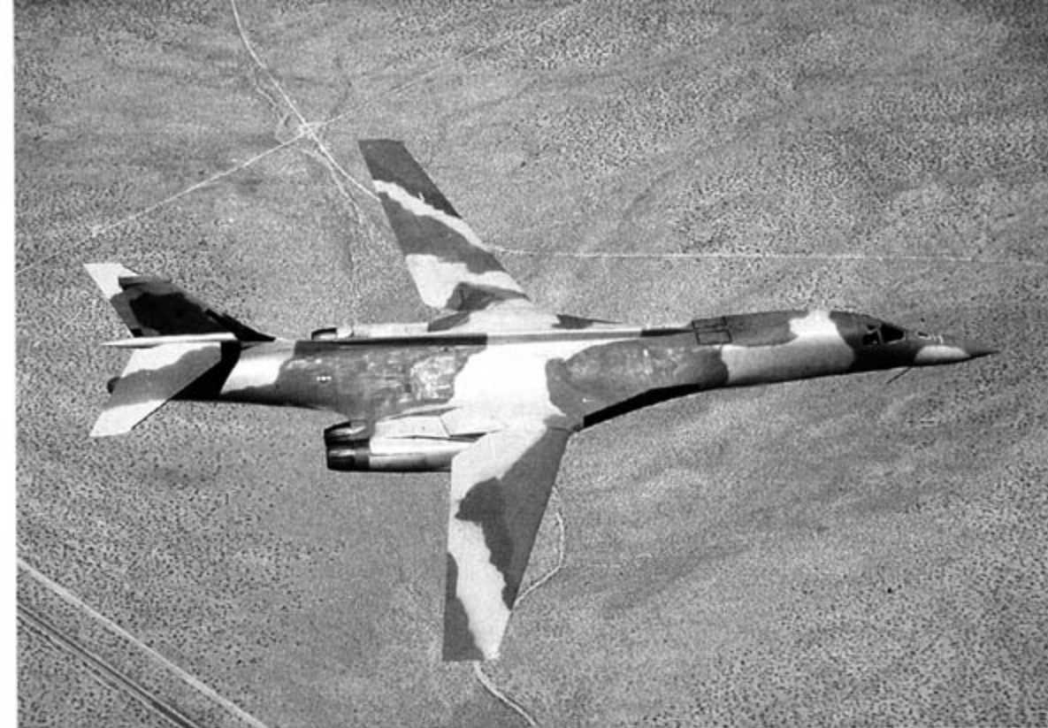
The number four B-1A (76-0174) was also painted in the desert camouflage, which covered the radome on this aircraft. The 'Crosseye' ECM system spine was later removed from the bomber and the waveguide incorporated into the fuselage. This B-1A – the first with ejection seats – later appeared in the three-tone 'Strategic Scheme' applied to B-1Bs. (USAF)
