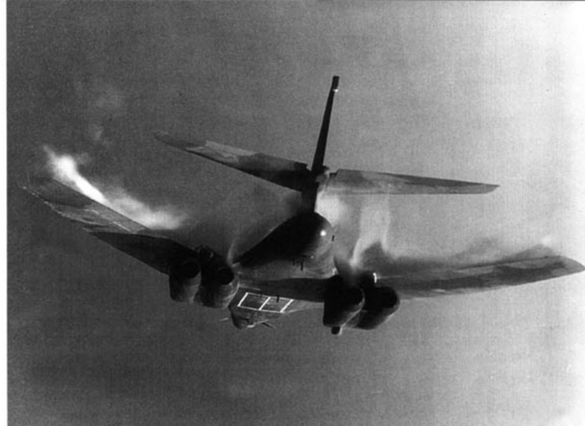
This B-1B (85-0068) performs at the airframe's maximum Gravity Force (G) limit in a wind-up turn during a test of the Stall Inhibit System (SIS). A combination of high G and high humidity creates a veil of condensation on the upper wing and fuselage surfaces. The SIS and a Stability Enhancement Function (SEF) were added to the B-1B as a result of increasing the maximum gross weight from 360,000 pounds (163,296 kg) in the earlier B-1A to 477,000 pounds (216,367.2 kg) in the B-1B. (USAF)
