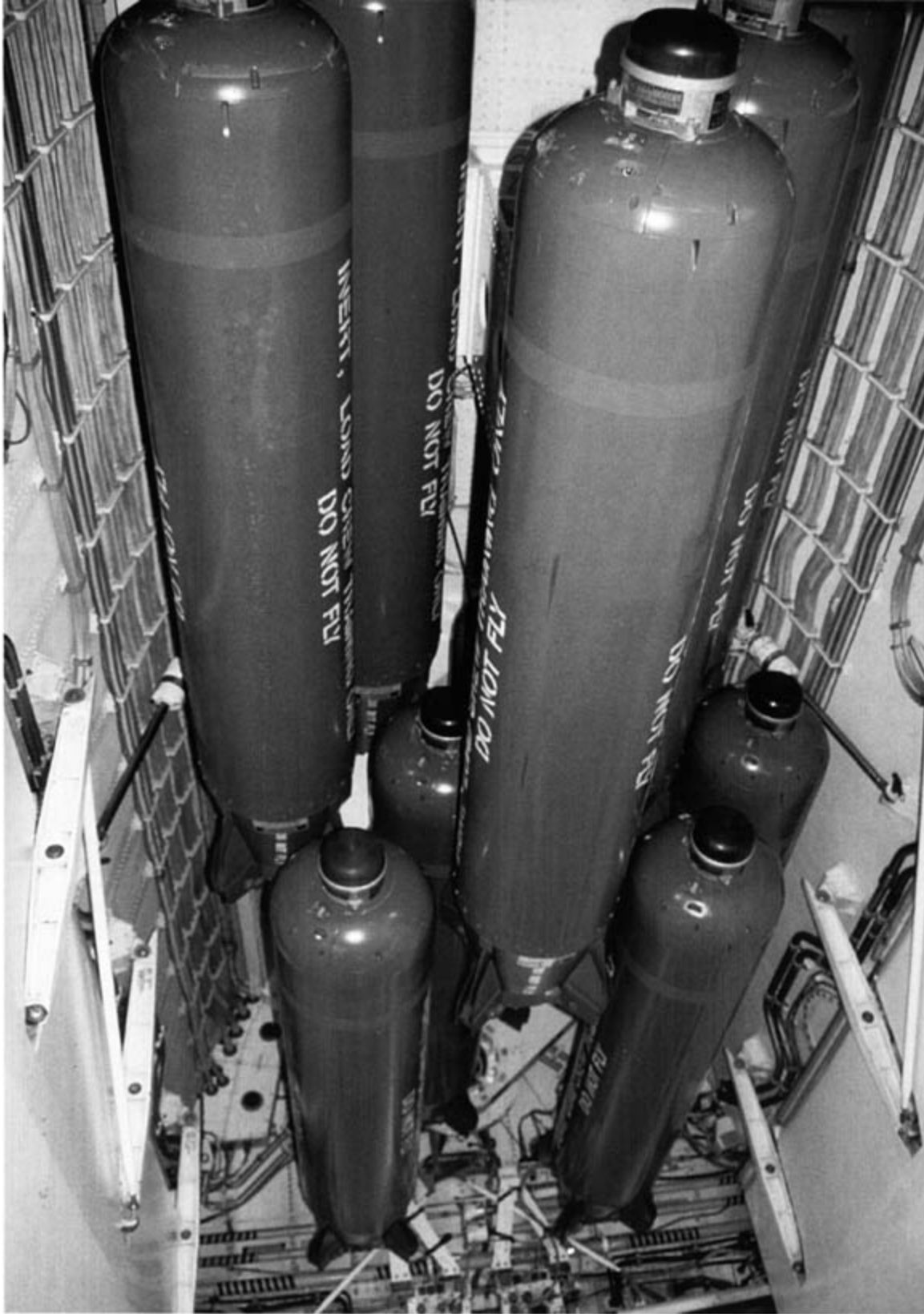
Inert CBU-89 'Gator' cluster bombs are loaded on a CWM installed in a B-1B. These training bombs have Dark Blue (FS35109) rings immediately aft of the nose. Each CBU-89 carries 72 BLU-91 anti-armor munitions and 22 BLU-92 anti-personnel munitions. These munitions are stabilized and detonated by proximity and/or Infrared (IR) sensors. The CBU-89 is similar in size to the CBU-87 Combined Effects Munition (CEM), whose bomblets explode into both anti-personnel and incendiary fragments. (Lou Drendel)
