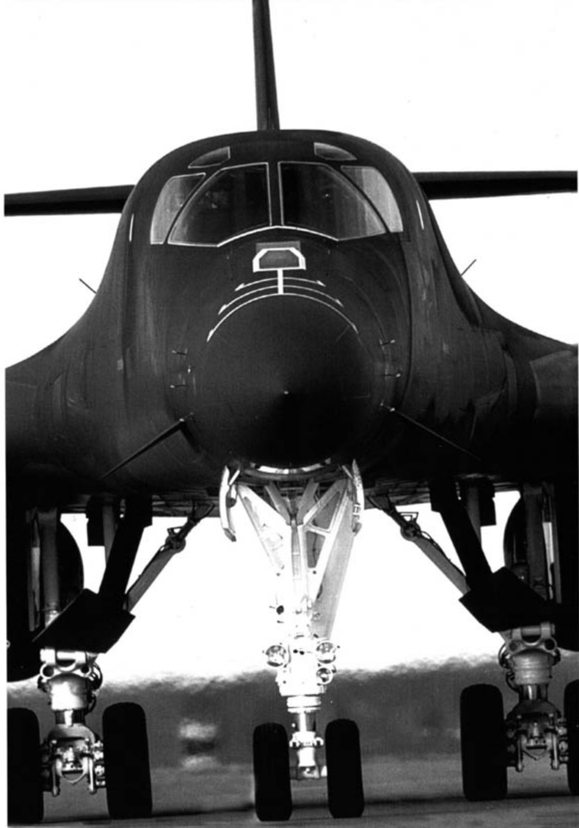
The B-1B nose landing gear can be steered 75° to port or starboard for directional control on the ground. The system is hydraulically operated and electronically controlled, with commands sent through the rudder pedals. Nose wheel steering is automatically disengaged when the landing gear is retracted. The landing gear track is 14 feet 6 inches (4.4 m) and the wheelbase is 57 feet 6 inches (17.5 m). (Rockwell)
