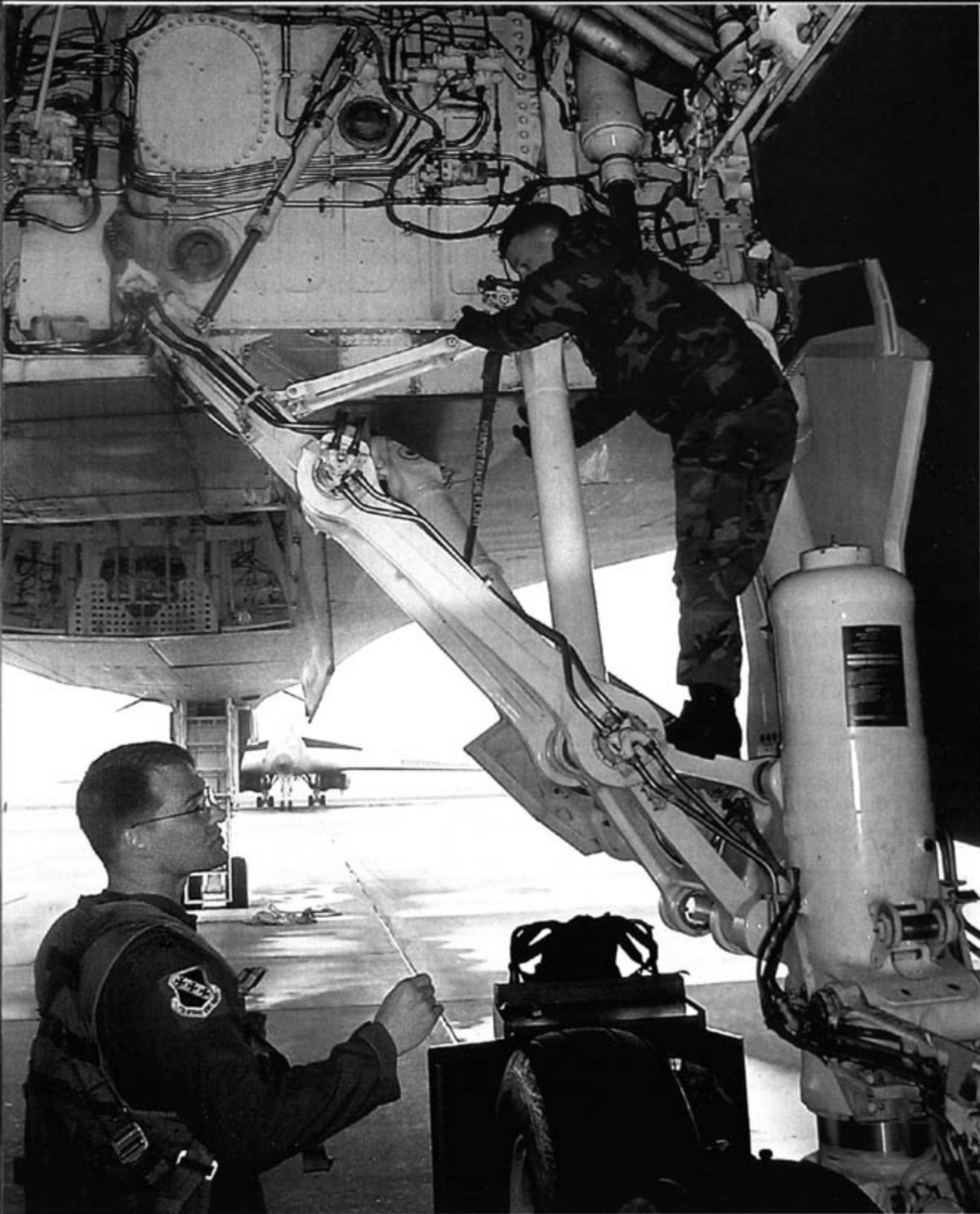
Major Scott Cameron checks the starboard main landing gear on his pre-flight walk around the B-1B while the crew chief pulls the safety pins from the gear. The crew chief stands on the A-frame side brace connecting the forward gear well bulkhead to the main strut. Landing gear assemblies and wheel wells are Gloss White (FS17875) to easily detect liquid leaks. The robust gear fully retracts under hydraulic power in 40 seconds. (Lou Drendel)
