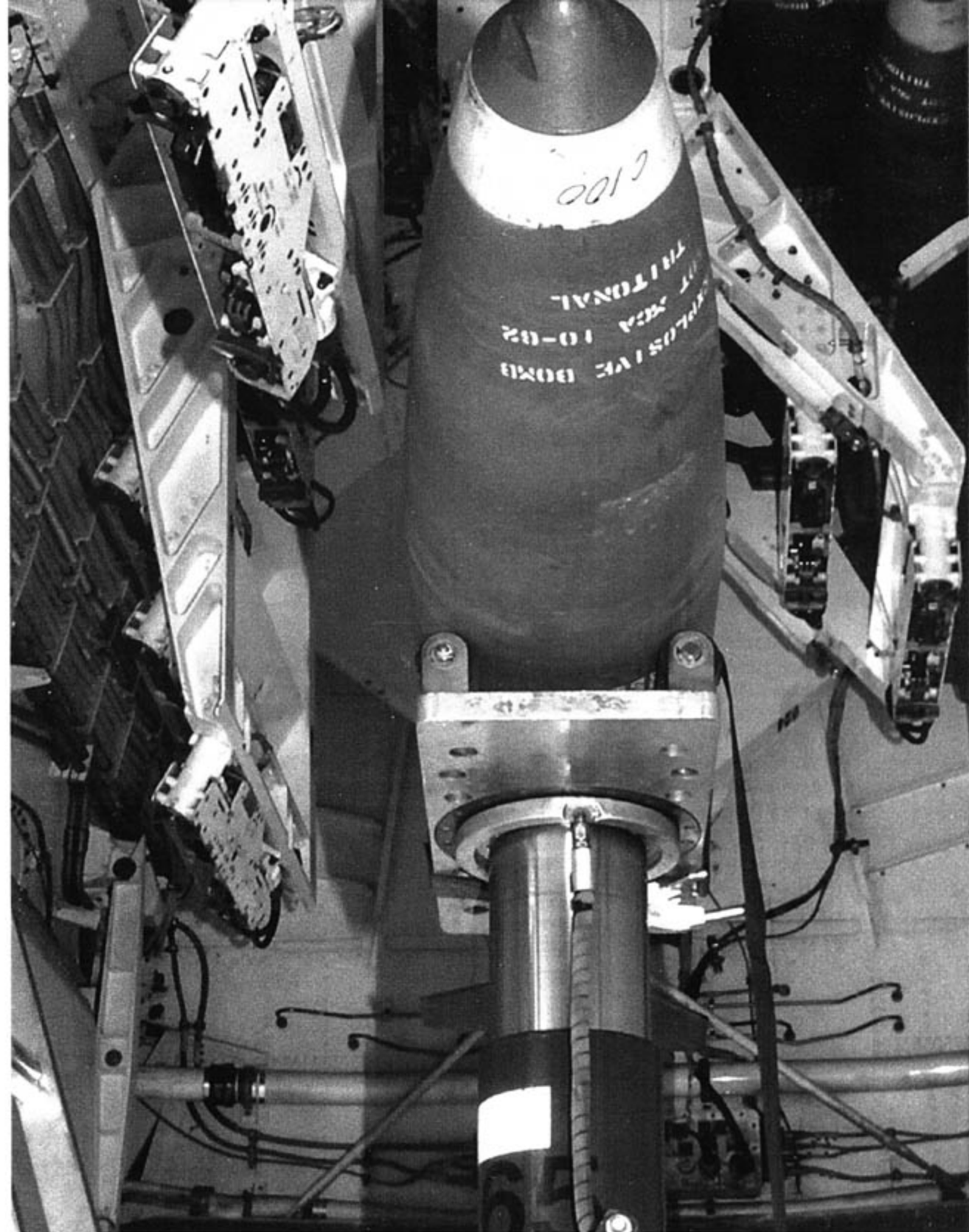
A Mk 82 bomb is hoisted aboard a swing arm on a CWM loaded aboard a B-1B. Two lugs on the bomb's upper surface are captured by an ejector rack, which is installed on one of the CWM's four swing arms. Ejector racks must be cleaned and reloaded before weapons can be reloaded on the CWM. Bombs are overall Olive Drab (FS34087) with Orange-Yellow (FS33538) nose rings on conventional explosive weapons. (via Jeff Warmka)
