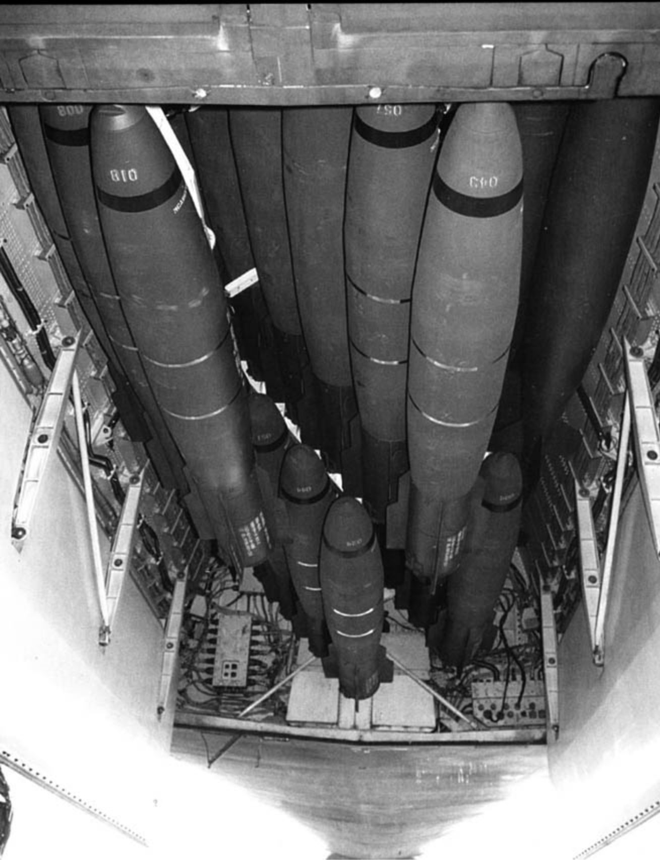
The intermediate weapons bay holds a full load of twenty-eight 500 pound Mk 82 Air Inflation Retard (AIR) bombs loaded on a Conventional Weapons Module (CWM). AIR bombs can be released at higher airspeeds than bombs equipped with the earlier Snakeye folding fins. Nose plug fusing is used on AIR bombs. Inert Mk 82s used for training have blue nose bands. (Lou Drendel)
