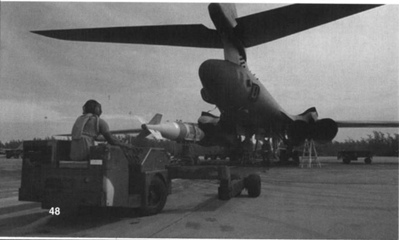
An Air Force bomb loader driving an MJ-1 lift truck delivers a 2000 pound JDAM to a B-1B prior to a mission over Afghanistan. Towed Decoy System (TDS) fairings are mounted on the port and starboard tail cone sides. Expendable countermeasures housed in the TDS fairings help protect the Lancer from Surface-to-Air Missiles (SAMs) – a threat which did not materialize during these missions. (USAF)
