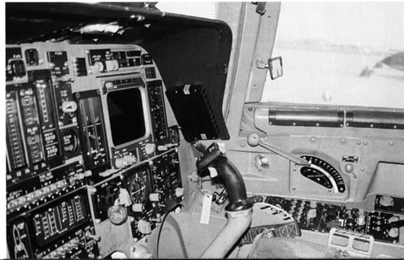
The co-pilot's panel and side console duplicates the pilot's controls and instruments. The large wing sweep control lever mounted above the side console is duplicated on the port side. A rear view mirror mounted above the lever knob provides visual verification of wing sweep. Large vertical displays flanking the VSD provide additional Airspeed/Mach and Altitude/Vertical Velocity information. (Lou Drendel)
