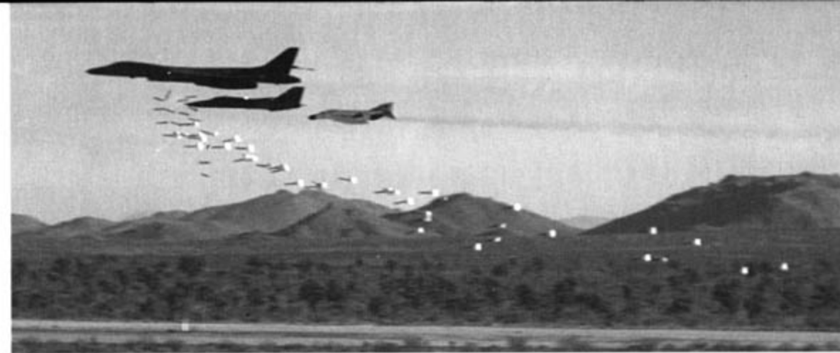
A B-1B releases a full bay's worth of Mk 82 AIR bombs over the Edwards AFB bomb range in California. The ballute (balloon/parachute) tails retard the bombs' fall long enough to allow the B-1 to escape the fragmentation pattern at low altitude. Flying chase are an F-111 Aardvark (nearest the B-1) and an F-4 Phantom from the 6512th Test Wing at Edwards AFB. (USAF)
