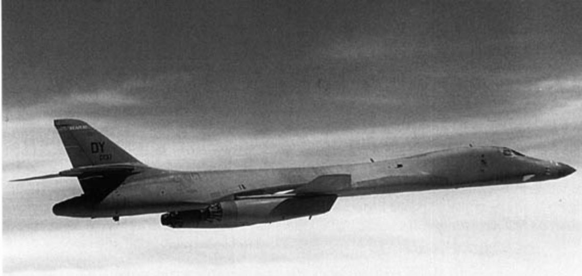
A B-1B (86-0137) assigned to the 13th Bomb Squadron 'Reapers' from Dyess AFB seeks in-flight refueling. The wings are swept at 25° for this cruise to the tanker rendezvous. The pilot or co-pilot may select any sweep angle between 15° and 67.5°, depending upon flight conditions. (Lt Col Tracy Sharp)
