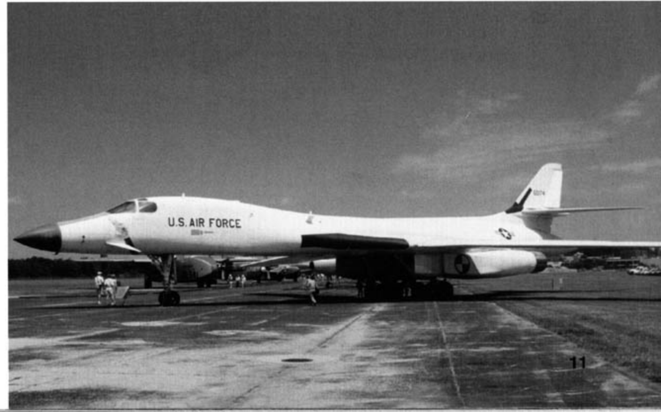
The fourth B-1A (76-0174) is displayed at the USAF Museum, located at Wright-Patterson Air Force Base (AFB), Ohio. The large black and white circle on the engine nacelle side is a registration mark used for photo interpreting during test missions. Black wing root and vertical stabilizer leading edge panels house various antennas. (Lou Drendel)
