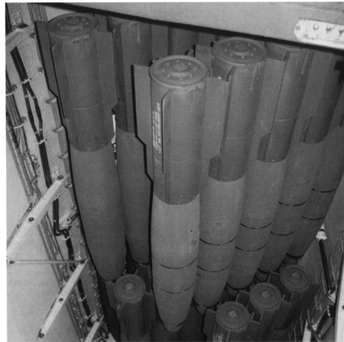
The intermediate weapons bay holds a full load of twenty-eight 500 pound Mk 82 Air Inflation Retard (AIR) bombs loaded on a Conventional Weapons Module (CWM). AIR bombs can be released at higher airspeeds than bombs equipped with the earlier Snakeye folding fins. Nose plug fusing is used on AIR bombs. Inert Mk 82s used for training have blue nose bands. (Lou Drendel)
