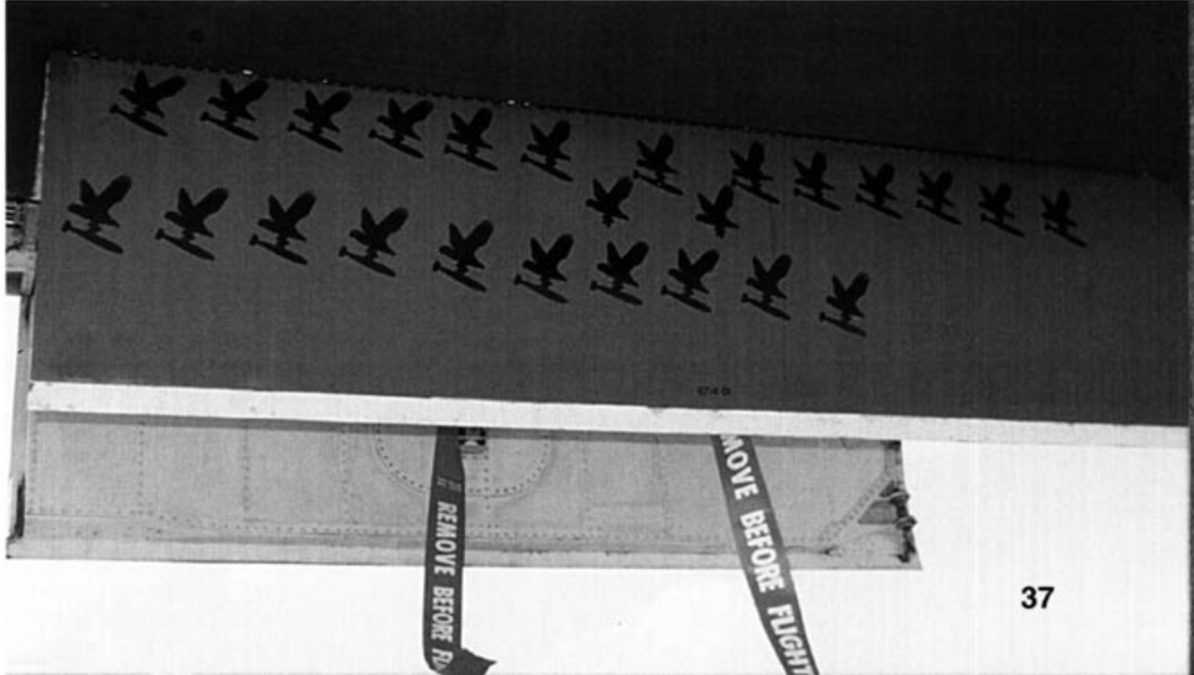
Twenty-five Kosovo War combat mission markers are painted on the nose landing gear doors of this 77th BS B-1B. The insignia is a black silhouette of the Squadron's War Eagle mascot with a bomb in its talons. Red streamers with REMOVE BEFORE FLIGHT in white are attached to nose gear locks, which prevent inadvertent gear retraction while the B-1B is on the ground. (Lou Drendel)
