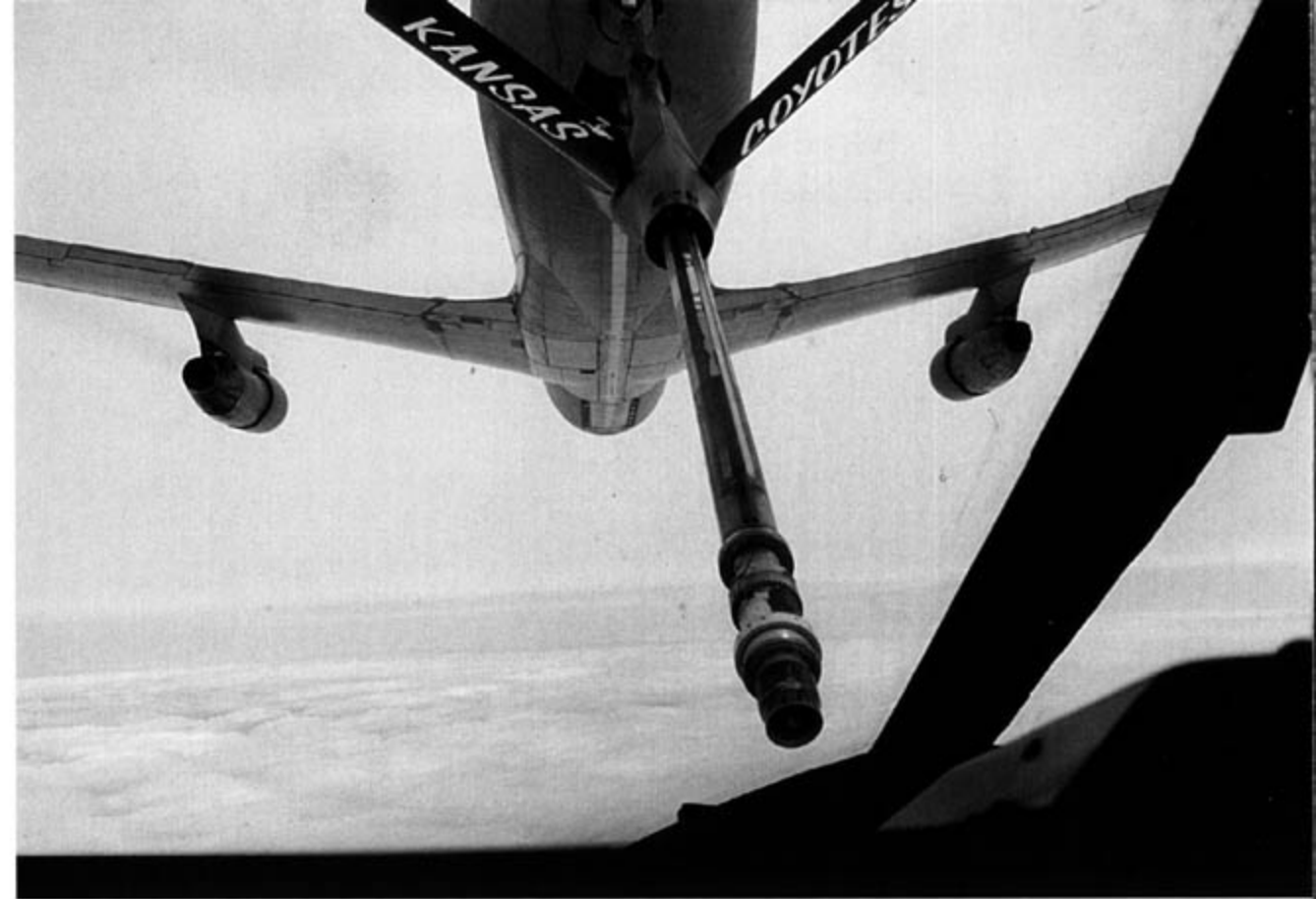
The aerial refueling boom of a Kansas ANG KC-135E (call sign Wiley 32 ) prepares to plug into Hawk 74's receptacle. Insertion of the refueling boom into the receptacle shuts off all transfer pumps, opens the Ballast Tank Isolation Valve, and opens all fill valves. As each tank fills, the fill valves shut off flow into the tank. Careful Center of Gravity (CG) management is critical during refueling to prevent losing aircraft control. (Lou Drendel)
