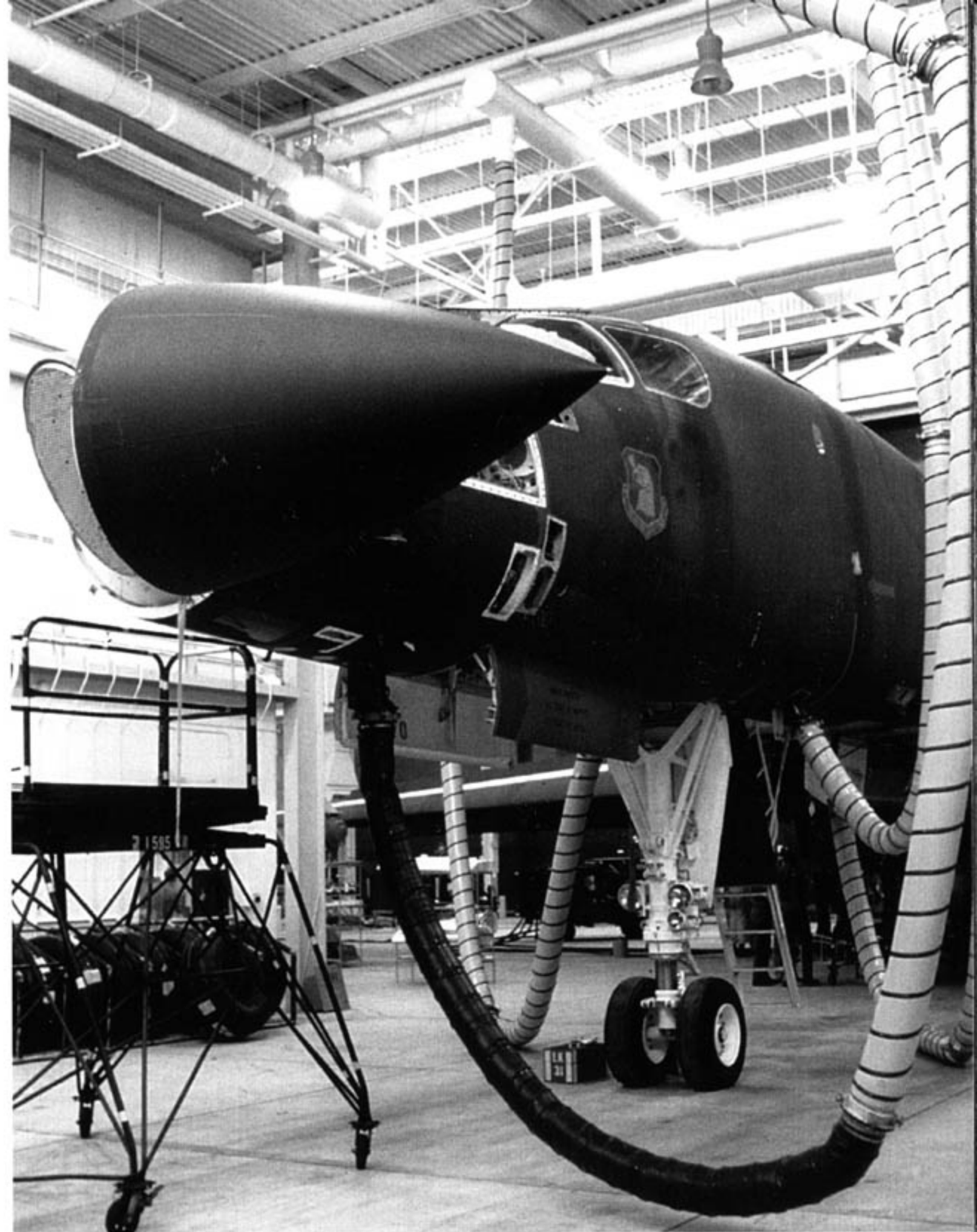
Air conditioning hoses run to a 96th BW B-1B during extensive maintenance operations. The radome opens to port for access to the Westinghouse AN/APQ-164 offensive radar. The oval radar antenna provides the B-1B's crew with low altitude, terrain following, and precision navigation. Several port nose panels are opened for access to avionics equipment. (Rockwell)
