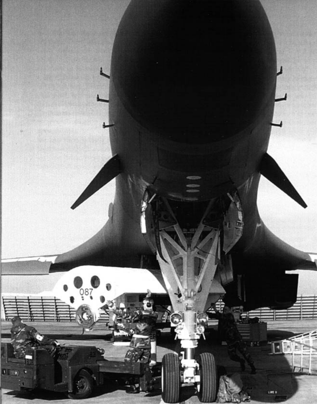
Armorers load an empty Conventional Weapons Module (CWM) aboard a 'Bone' at Fairford. CWMs can be pre-loaded with ordnance prior to installation; in practice, they are most often loaded empty, then fitted with bombs. During Operation ALLIED FORCE, all CWMs were in the conventional '28 carry' configuration, with twenty-eight 500 pound Mk 82 bombs. (via Jeff Warmka)
