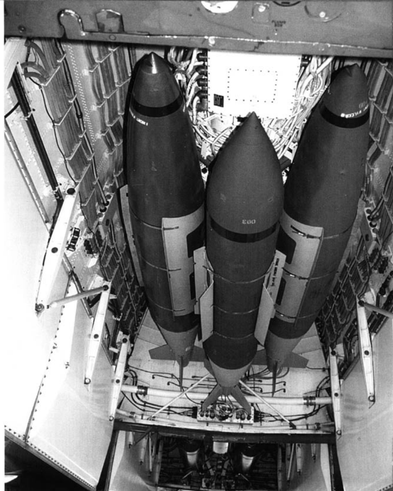
Three inert 2000 pound (907.2 kg) Joint Direct Attack Munitions (JDAMs) are loaded on a rotary launcher mounted in a B-1B's forward weapons bay. The JDAM adds centerbody strakes and a new tail unit to the standard Mk 84 'iron' (conventional) bomb. A Global Positioning System (GPS) receiver in the tail guides the weapon to its target, through the four pivoting tailfins. Additional JDAMs are mounted in the intermediate weapons bay. (Lou Drendel)
