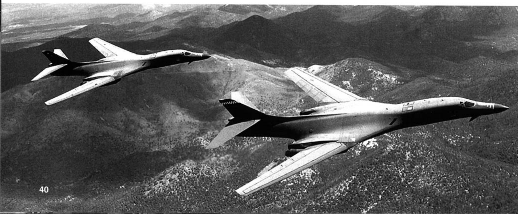
Two 7th Wing 'Bones' fly a training mission over the western United States. Average B-1B training missions are six hours long and consist of high and low altitude practice bombing, tactical formations, and aerial refueling. The lead aircraft has the blue and white checkerboard tail band of the 28th BS, 7th BW at Dyess AFB, Texas. Both B-1Bs have their wings swept at an intermediate setting for high speed cruising.
