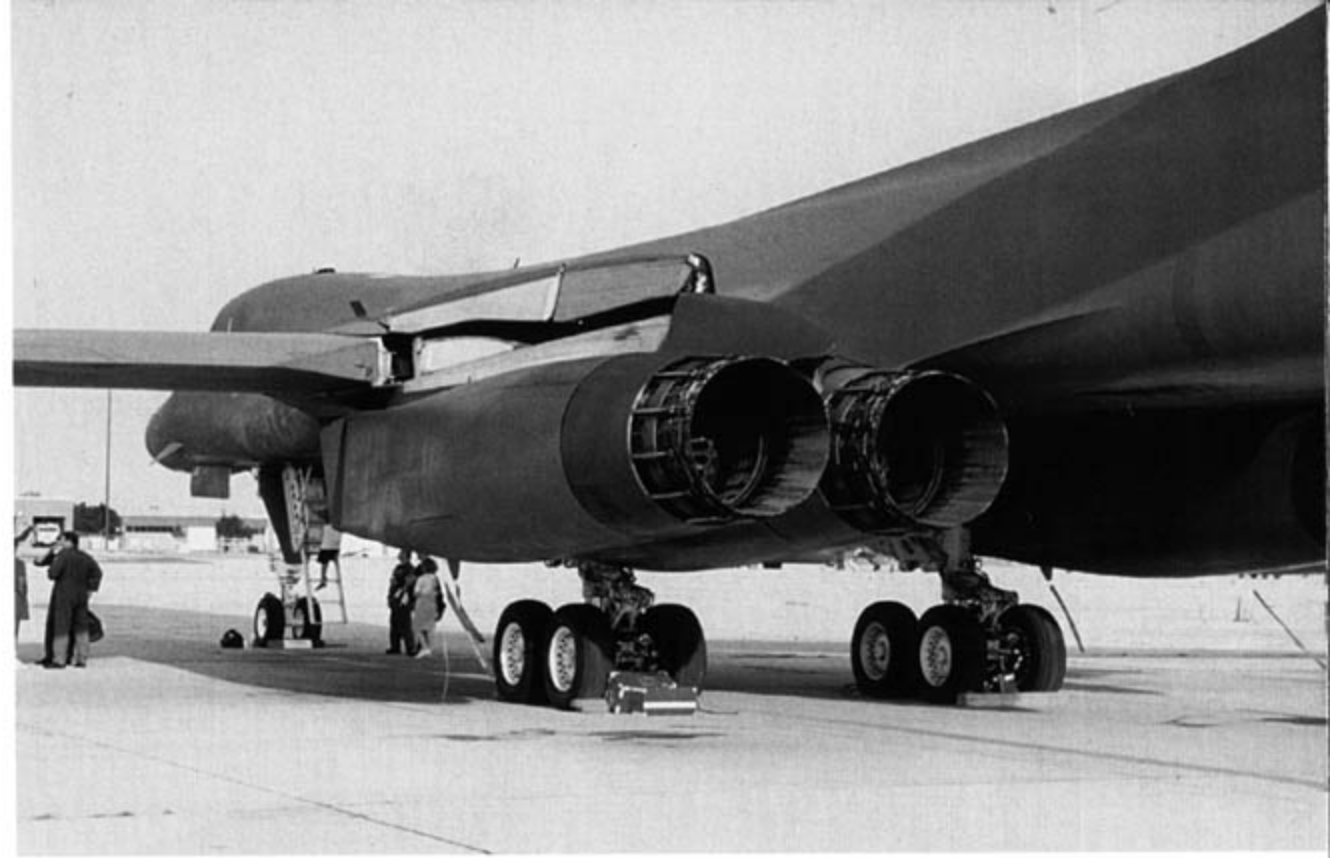
Canvas-covered inflatable rubber bladders seal the gap when the B-1B's wings are swept back. It replaced a less aerodynamic fairing used on the earlier B-1A. The engine exhaust nozzle actuator fairings ("turkey feathers") were removed from Lancers during the early 1990s, saving weight and maintenance time. The exhaust nozzle controls the expansion ratio of the engine exhaust gas during all operations. (Lou Drendel)
