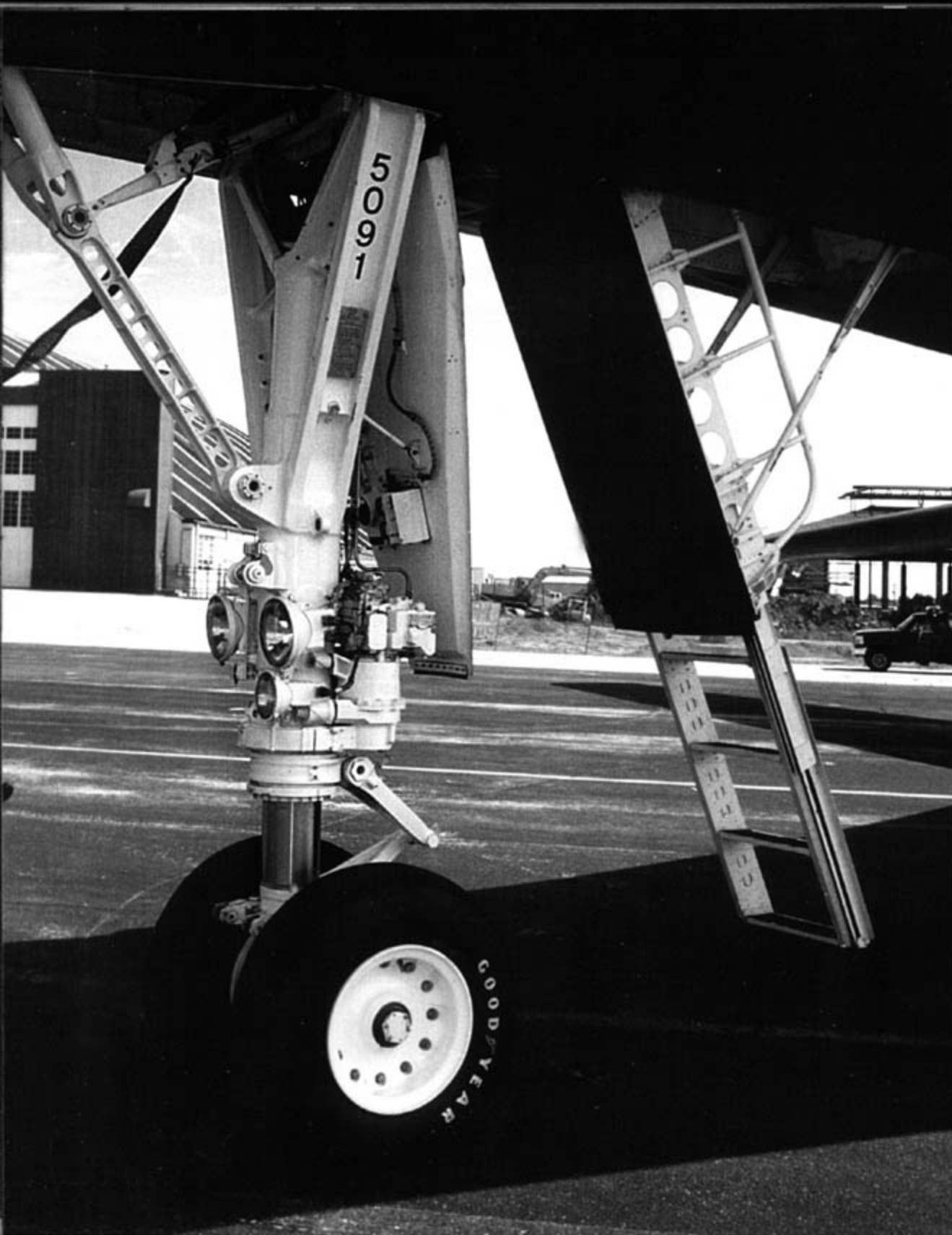
The B-1B's nose landing gear is similar to the earlier B-1A gear, although strengthened to handle increased aircraft weights. The drag link extending from the forward gear bay to the main strut is shorter on the B-1B. The nose gear retracts forward and upward into the fuselage, with emergency gear extension aided by the slipstream. The crew access hatch and retracting ladder is deployed aft of the nose gear strut. (Lou Drendel)
