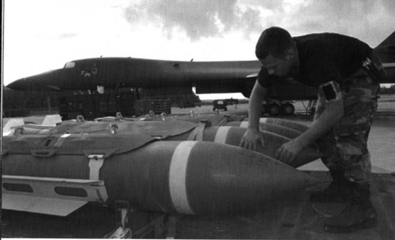
An ordnance specialist prepares 2000 pound (907.2 kg) Joint Direct Attack Munitions (JDAMs) for loading aboard a 77th Bomb Squadron B-1B at Diego Garcia. JDAMs are modified Mark 80 series 'iron' bombs fitted with centerbody strakes, which provide aerodynamic lift to the weapon. Tail-mounted Global Positioning System (GPS) receivers ensure precise JDAM delivery to the target. (USAF)
