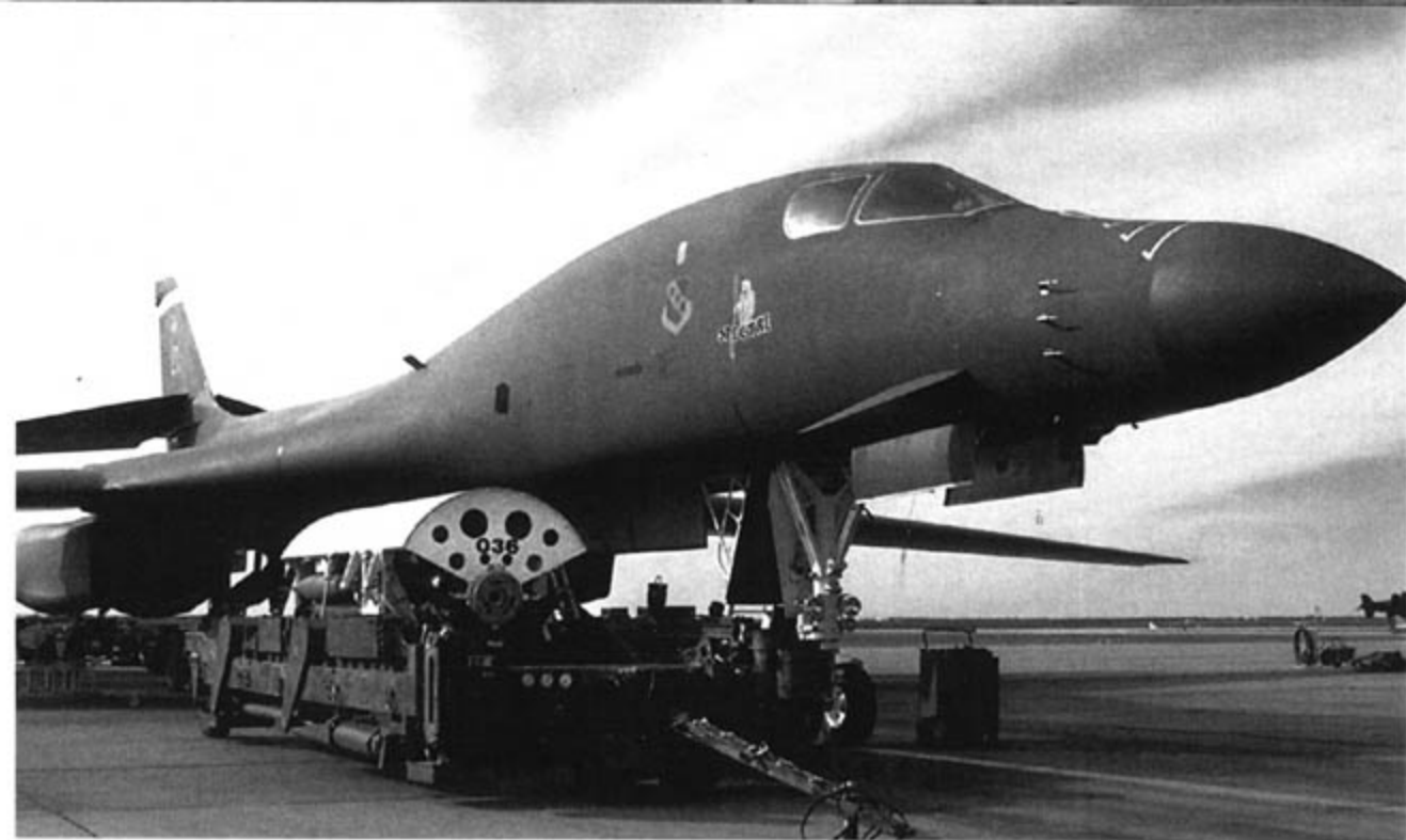
A Conventional Weapons Module (CWM) is prepared for loading aboard SPECTRE, a 7th Bomb Wing (BW) B-1B. The CWM is fitted with twenty eight 500 pound (226.8 kg) Mk 82 bombs. One module can be placed inside each of the Lancer's three weapons bays, allowing up to 84 bombs to be carried internally. CWMs have also been modified to carry ten Cluster Bomb Units (CBUs) and can also carry Mk 62 mines. (USAF)
