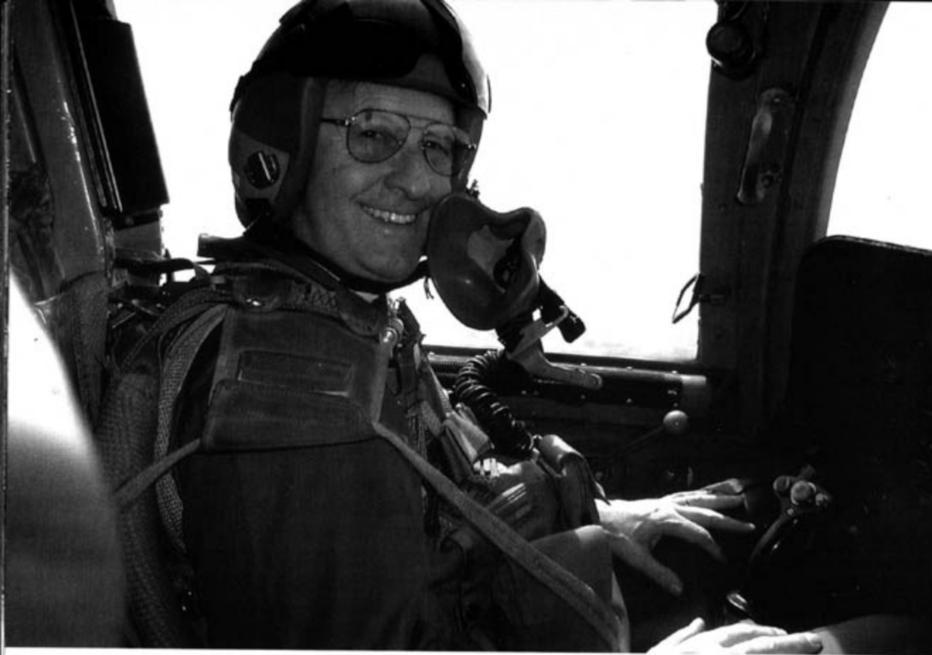
The author sits in the port (Pilot's) seat...hands off the controls. The strap over the shoulder pulls the arms in on ejection, preventing flailing injuries. The ACES II seats fitted to the B-1B incorporate an added cushion on the seat back and bottom for a more comfortable ride on long flights. (Maj Scott Cameron)
