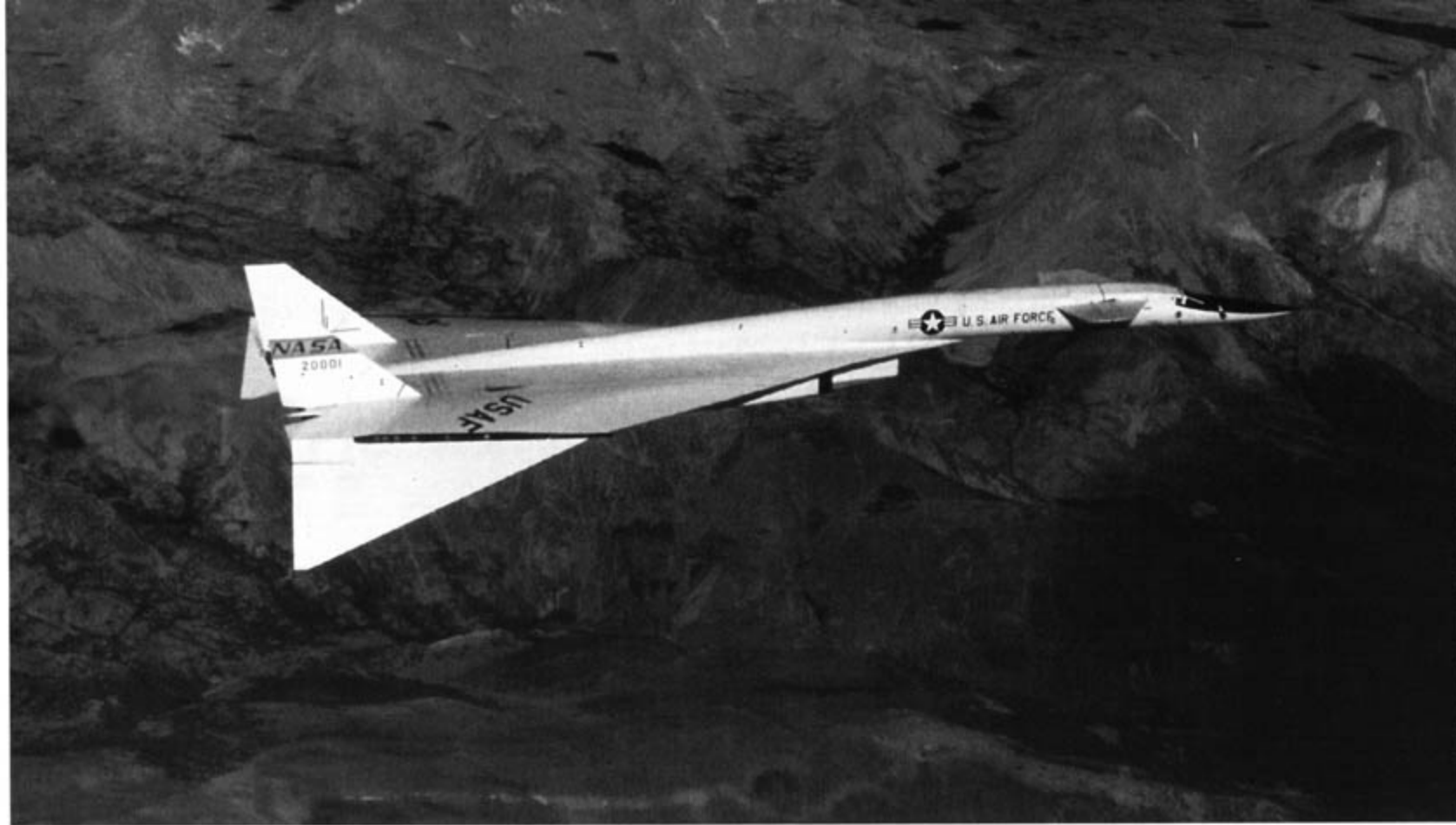
The first XB-70A Valkyrie (62-0001) flies above a canyon in the southwestern United States in 1968. Both wingtips are folded down to improve high-speed stability and increase lift. After the XB-70 was cancelled as a bomber in 1964, the two prototypes were used for high-speed flight research. The second XB-70A was lost in a mid-air collision in 1966. NASA used 62-0001 for research flights until it was retired to the US Air Force Museum in 1969. (NASA)
