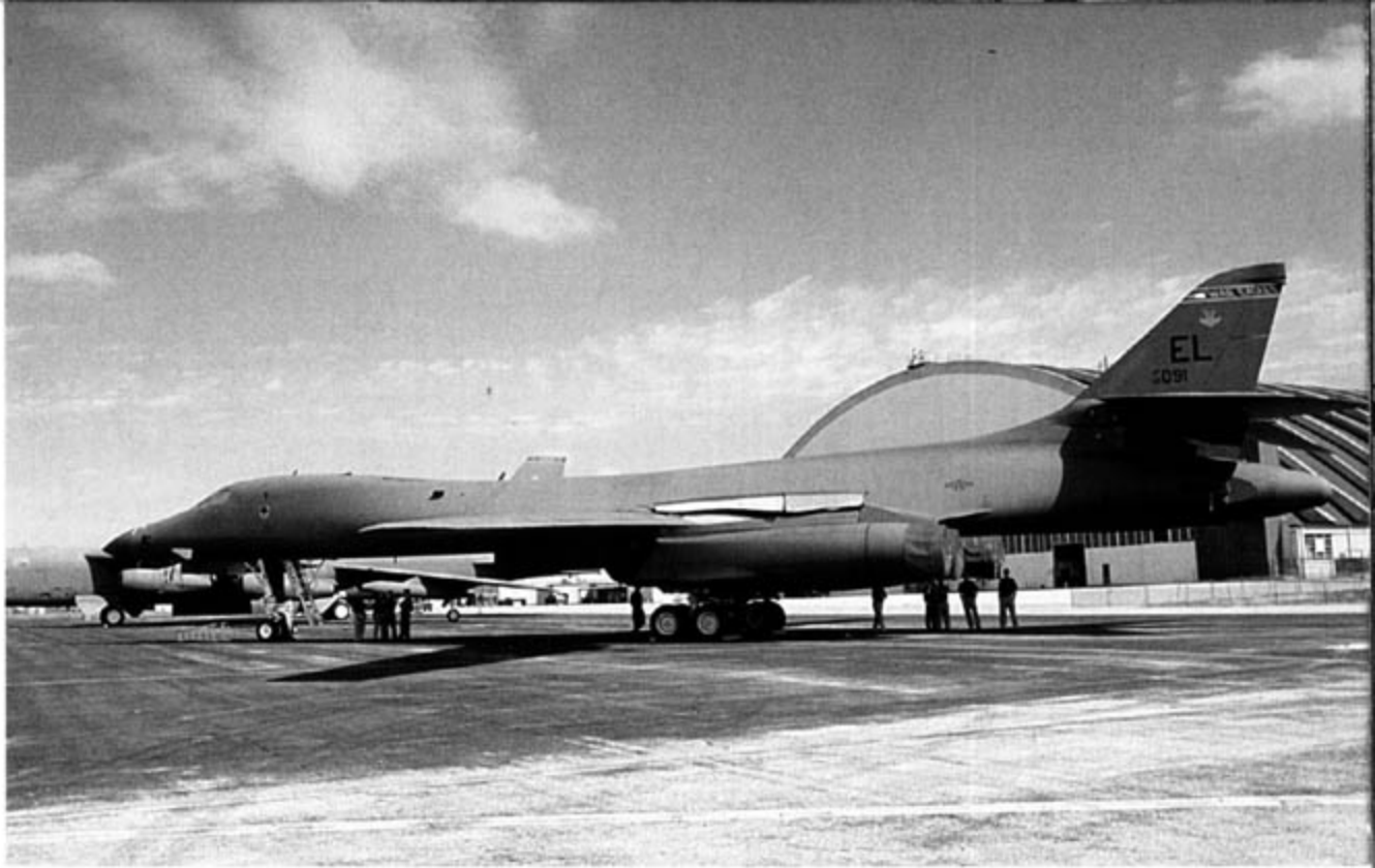
This 77th BS B-1B (85-0091) is parked at Ellsworth AFB in August of 1999, following combat over Yugoslavia. The 'Bones' flown during Operation ALLIED FORCE were the first Lancers equipped with the Towed Decoy System (TDS) on the tail cone sides. The TDS employs the ALE-50 radio frequency repeater jammer against enemy missiles aimed at the B-1. (Lou Drendel)
