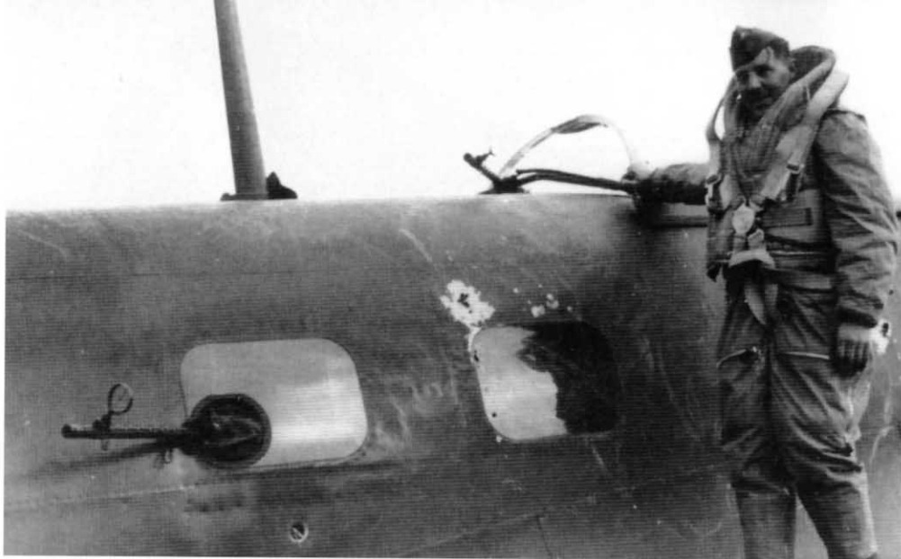
A gunner stands by the mid-fuselage of his He 111H, which landed at its home airfield despite battle damage. One 7.92mm MG 15 was mounted in the aft starboard window; another MG 15 was fitted to the opposite window. Shrapnel damage from anti-aircraft fire occurred above the next window on the starboard side. (Punka Archiv)
