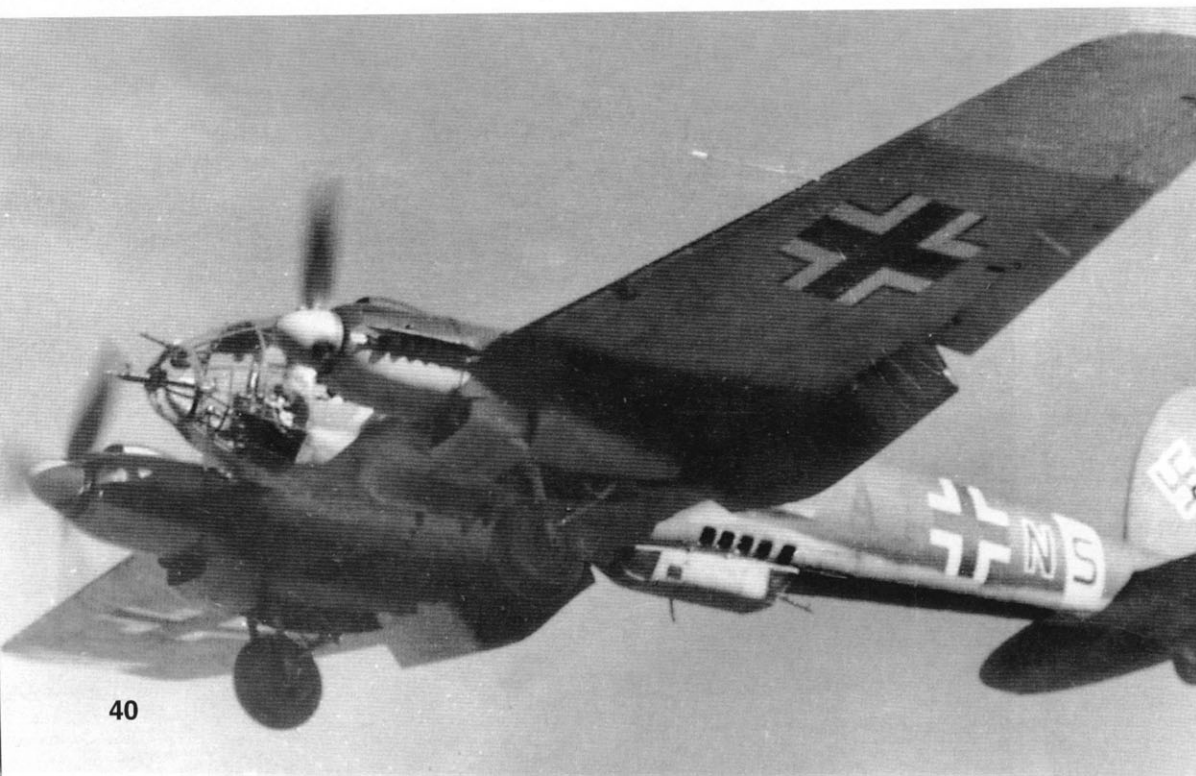
An He 111H bombardier/navigator practices aiming a 20mm MG FF cannon in the nose of his aircraft. The weapon was highly effective against trains and other surface targets when the bomber flew at low level. The MG FF was sighted using the L-FF/6 sight. This He 111H is also equipped with a Kuto-Nase (Nose Cutter) balloon cable cutter along the port side. (Schmidt)
