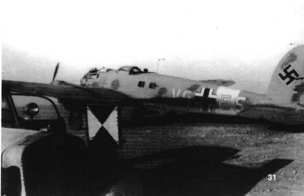
Field Marshal Erwin Rommel, commander of the Deutsche Afrika Korps , used this He 111H-4 (VG+ES, Werk Nr. 4085) as his transport. The aircraft's upper surfaces were painted RLM 79 Sand Yellow (FS30215) and RLM 80 Olive Green (FS34052), with RLM 78 Light Blue (FS35352) undersurfaces. The aft fuselage band and letters are white, while E and part of S are outlined in RLM 23 Red. (Schmidt)
