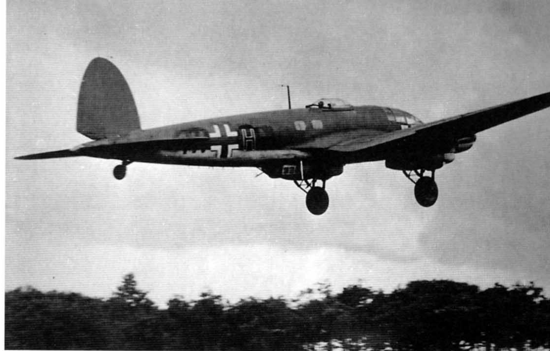
A 5/KG 26 'Löwengeschwader' He 111H-6 (1H+HN) departs its airfield in Norway bound for England during the Battle of Britain. The individual aircraft code letter H is RLM 23 Red (FS31140) outlined in White. This aircraft's tail swastika was overpainted in Black Green for an unknown reason. The Luftwaffe had 463 He 111s deployed in France, Belgium, and Norway when the Battle of Britain began on 13 August 1940. (Punka Archiv)
