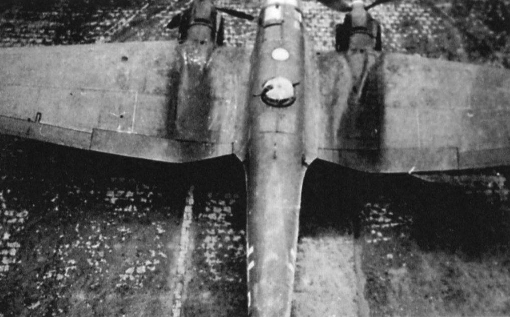
The He 111H-20's defensive armament included a 13MM MG 131 machine gun in a DL131 dorsal turret. This electrically-powered turret traversed 360° for improved protection against enemy fighters. A circular EZ-6 radio direction finder antenna is mounted to the upper fuselage forward of the turret. Flame dampers were fitted to the engine exhausts for night bombing missions. (Petrick)
