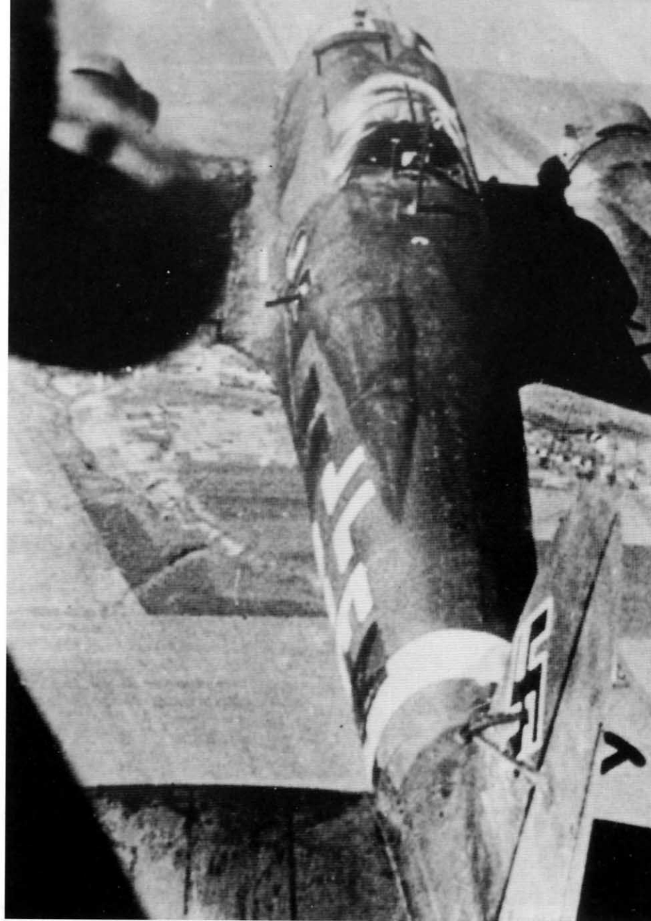
An MG 15 juts out of the port beam window on this He 111H-2 (T5+FU) of Wekusta Ob.d.L. The aircraft retained their defensive armament despite their weather reconnaissance tasking. The He 111's minimal defensive armament was slightly improved in effectiveness by close formation flights. This allowed the gunners to bring more weapons to bear against enemy fighters. (Punka Archiv)
