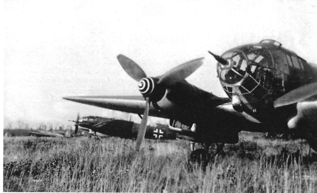
This He 111H-11 parked on a Hungarian airfield has a white Spiralschnauze (Spiral Snout) painted on the starboard propeller spinner. This marking was unusual for Luftwaffe bombers, although it was common for fighters during this period. The He 111H-10 parked in the background is armed with a 20mm MG FF cannon with flash hider in the nose for night bombing missions. The He 111H-11 is also equipped with this weapon, but without the flash hider. (Punka Archiv)
