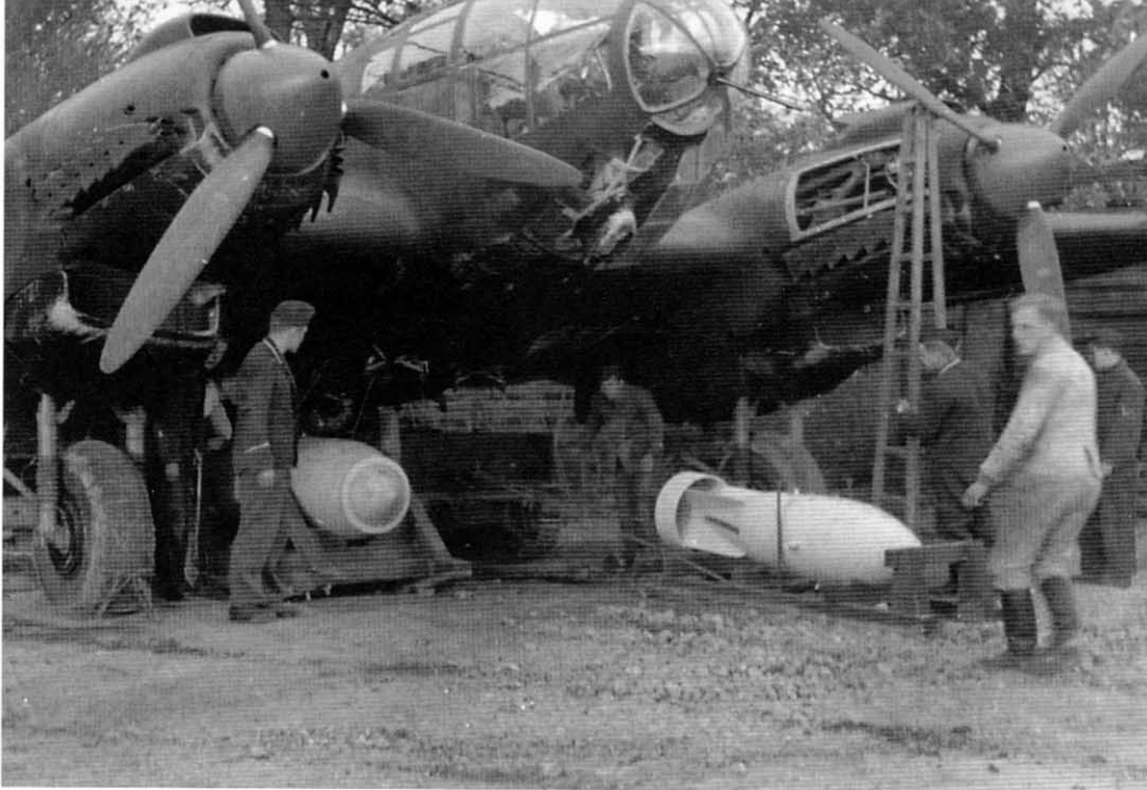
Luftwaffe armorers load two 1000 kg (2204.6 pound) SC 1000 bombs onto an He 111P prior to a mission over England in 1940. Each weapon was carried on ETC 2000 external bomb racks fitted to the fuselage undersurface. These racks covered the internal bomb cells, but allowed the He 111 to carry larger and heavier ordnance. (Bundesarchiv)
