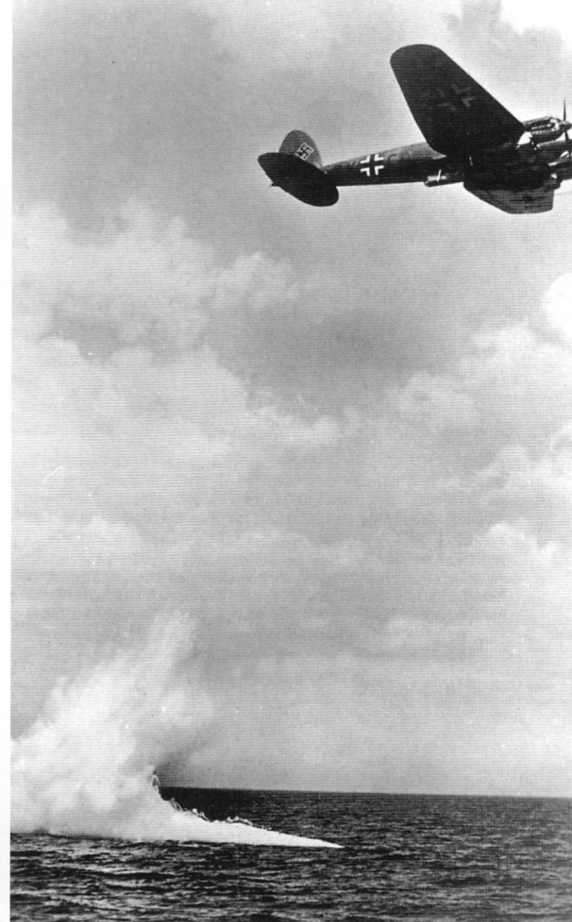
A 6/KG 51 'Edelweißgeschwader' He 111H-6 (9K+CP) pulls up after releasing two LT F5b torpedoes. The anti-ship weapons just entered the water and are bound for their target. The bomber retained its black undersurfaces from its earlier night bomber deployment against England. (Punka Archiv)
