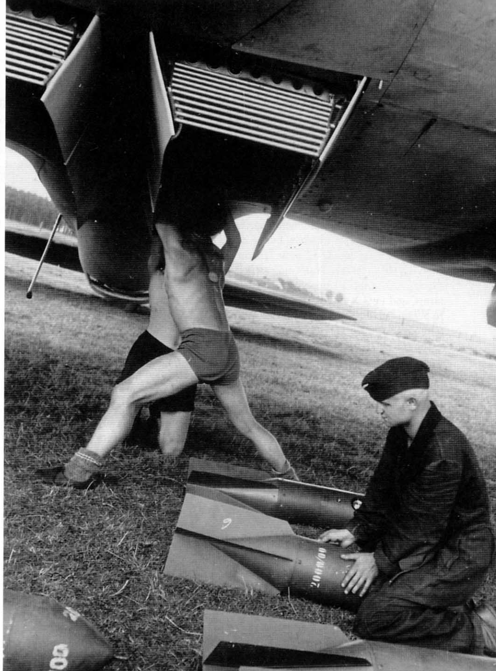
Armorers load 250 kg (551.1 pound) SC 250 bombs into an He 111P during the 1939 Polish Campaign. The bombs were loaded nose up into the eight ESAC bomb cells – two rows of four cells each. These cells allowed the He 111 to carry its bomb load internally; however, this restricted the weapons' size to 250 kg. A spoiler lowered between the two doors of the front cells to reduce airflow interference with weapons release. (Bundesarchiv)
