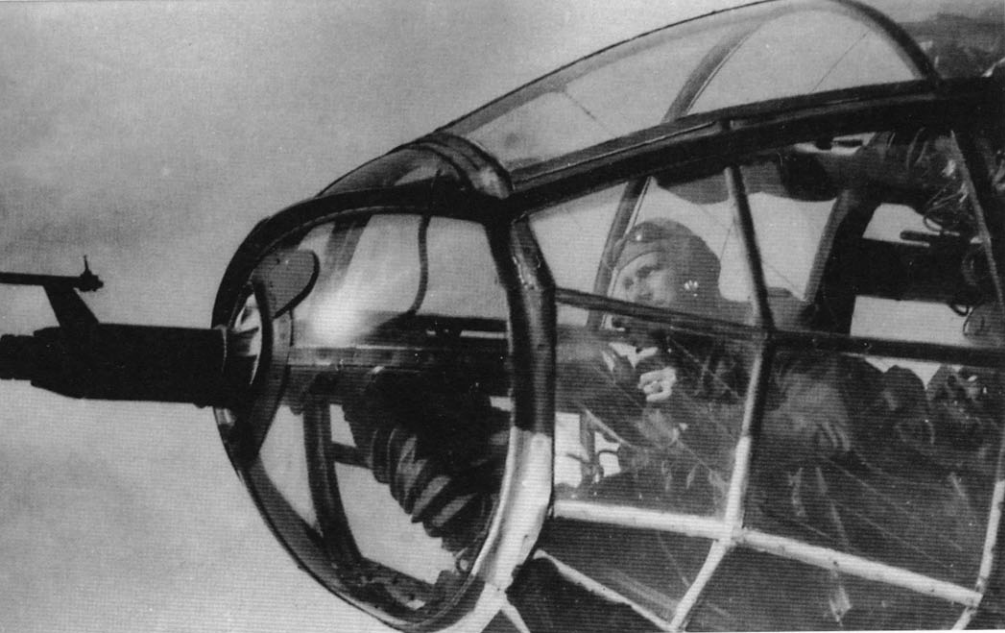
An He 111H bombardier/navigator practices aiming a 20mm MG FF cannon in the nose of his aircraft. The weapon was highly effective against trains and other surface targets when the bomber flew at low level. The MG FF was sighted using the L-FF/6 sight. This He 111H is also equipped with a Kuto-Nase (Nose Cutter) balloon cable cutter along the port side. (Schmidt)
