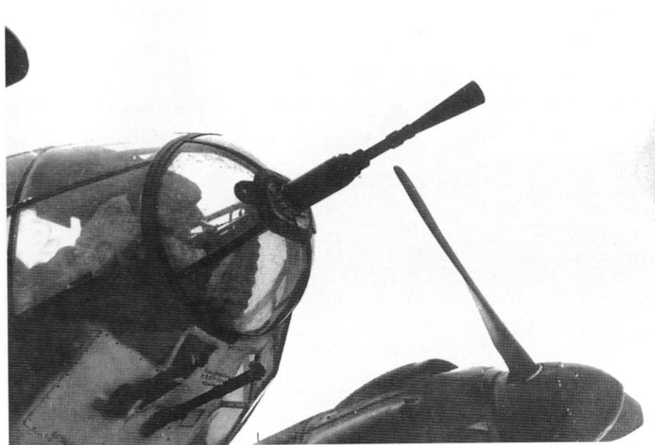
The nose-mounted MG FF is fitted with a conical muzzle flash suppressor, which reduced the blinding muzzle flash in the bombardier/navigator's and pilot's eyes at night. This He 111H was field modified with two 13mm Rheinmetall MG 131 machine guns below the nose cone for additional frontal firepower. The bomber operated in the Orscha and Smolensk areas of the Soviet Union in late 1942. (Schmidt)
