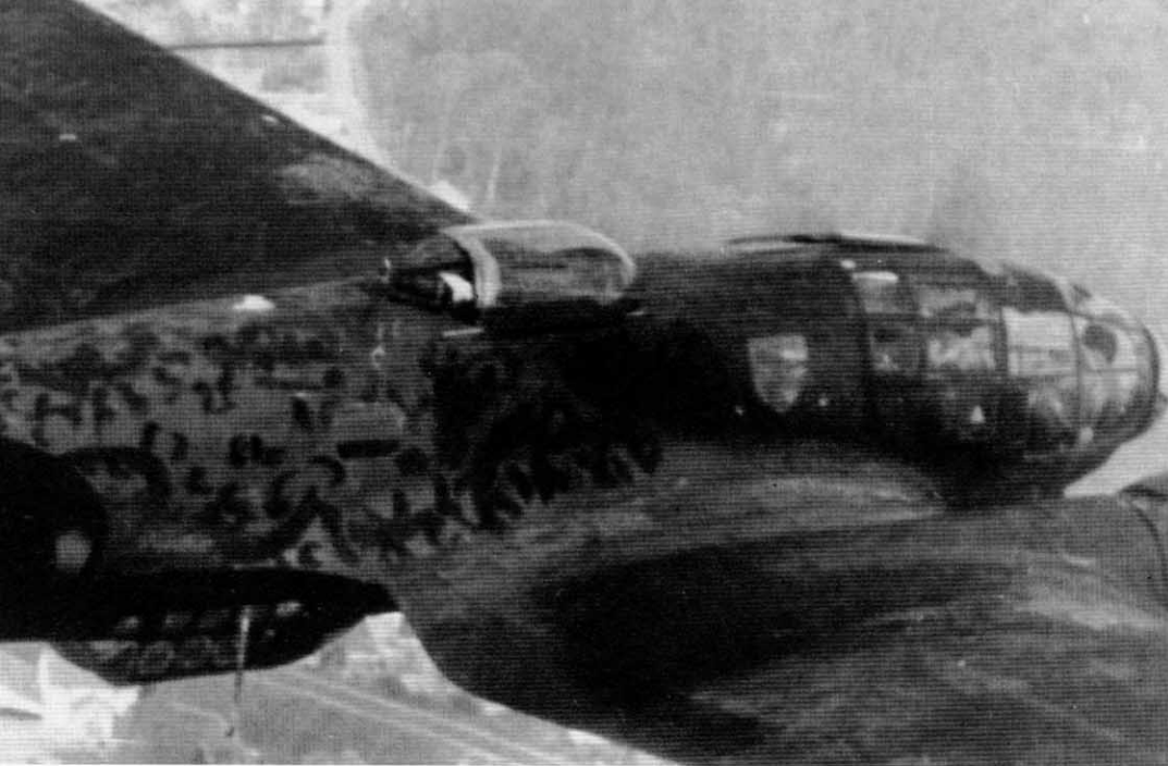
The dorsal gunner's canopy is mostly closed on this KG 55 He 111P-2, which operated from northern France during late 1940. The closed canopy greatly reduced the radio operator/gunner's exposure to the airstream. It opened to allow the gunner to escape in an emergency. One 7.92MM MG 15 was mounted in this position.
