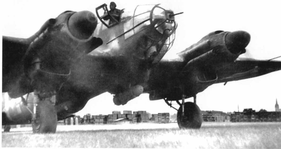
A KG 55 He 111H-20 prepares to taxi out on a night raid on London in early 1944. The bombardier/navigator leans out his open window to get final instructions from the ground crew. This bomber has exhaust flame dampers, a refined Kuto-Nase , and is armed with a 1000 KG (2204.6 pound) PC 1000RS bomb under the port fuselage. (Löhr)
