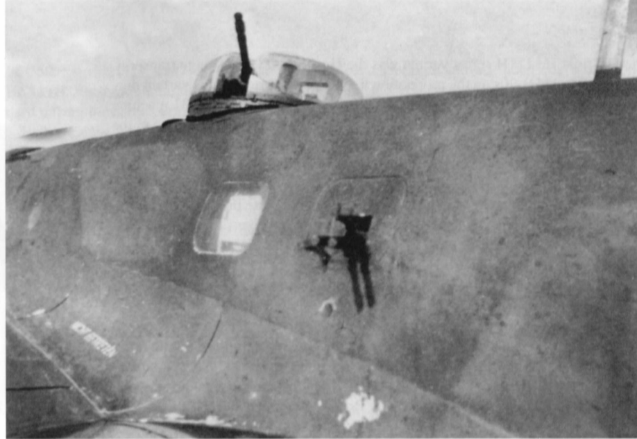
The He 111H-20's defensive armament included 7.92MM MG 81Z twin-barrel machine guns in the port and starboard beam positions. The weapons were fitted inside covered windows, which allowed the gunner to fire without exposure to the airstream. The radio antenna base is mounted aft of the 13MM machine gun turret. (Petrick)
