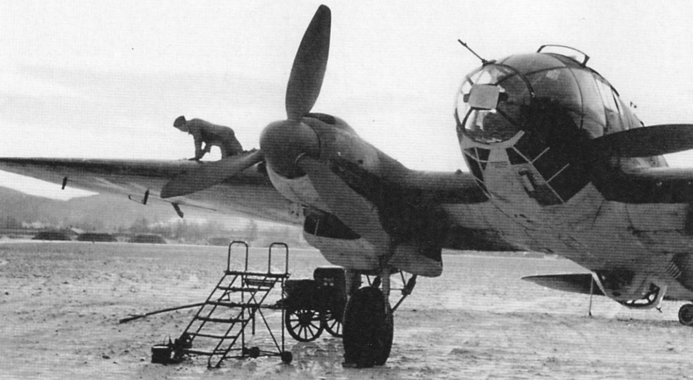
A crewman performs maintenance on the starboard wing of an He 111H-6, which is parked on a snow-covered airfield in Norway. This variant introduced the wide chord Junkers VS-11 wooden propeller, which replaced the narrow chord VDM metal propeller of earlier He 111s. The VS 11's increased width allowed it to better grab thin air at high altitude, while the wood construction conserved scarce metals. (Bundesarchiv)
