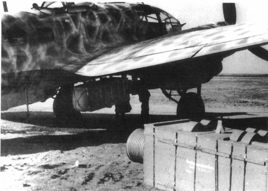
Ground crewmen install a 700 kg (1543.2 pound) supply container under the fuselage of this KG 4 He 111H-6 on the Eastern Front in 1943. A second container awaits installation near the starboard wing. A parachute fitted to one end of this container slowed its descent after release from the aircraft. RLM 76 Light Gray mottling was painted over the He 111H-6's upper surfaces. (Schmidt)
