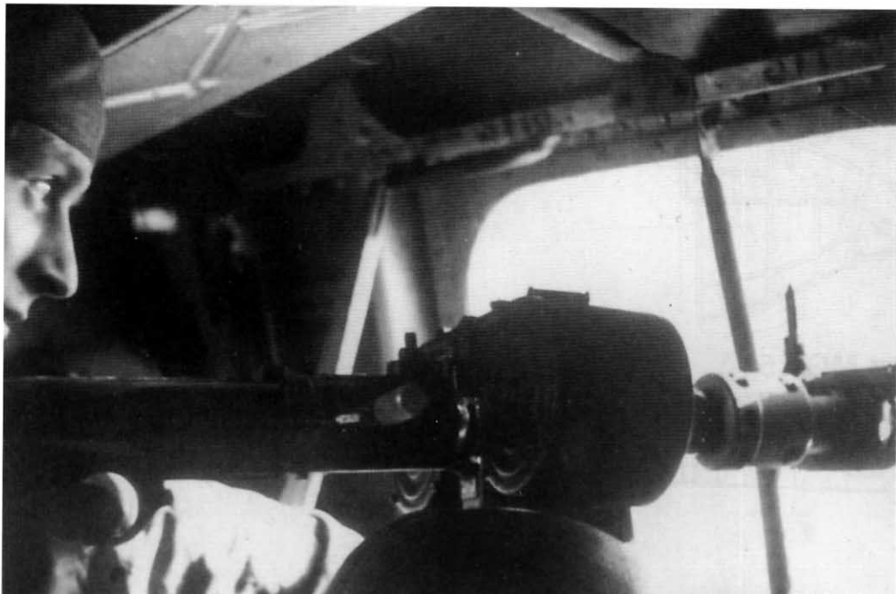
An MG 15 juts out of the port beam window on this He 111H-2 (T5+FU) of Wekusta Ob.d.L. The aircraft retained their defensive armament despite their weather reconnaissance tasking. The He 111's minimal defensive armament was slightly improved in effectiveness by close formation flights. This allowed the gunners to bring more weapons to bear against enemy fighters. (Punka Archiv)
