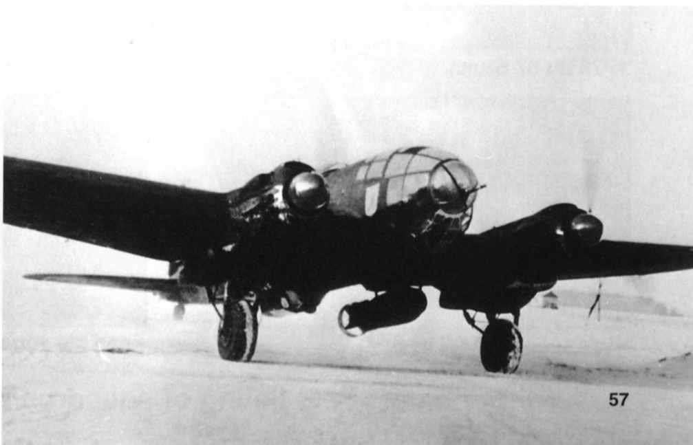
A KG 26 He 111H-6 begins its take off run on a snow-covered airfield in Russia. It is armed with a 1000 kg SC 1000 bomb on the port rack, which was the standard rack used when only one underfuselage external stores station was required. The He 111H-6 retains the black undersurfaces of its previous night bombing deployment over England. (Punka Archiv)
