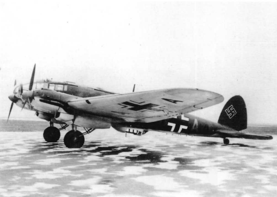
This He 111H-4 (1T+AA) was assigned to Stab/KG 28 during 1942. The ventral gondola access door was removed from this aircraft for an unknown reason. The Squadron identification letter A was RLM 24 Dark Blue (FS25053), while the other lettering was black. No war theater band was painted on this He 111. (Dr. Volker Koos)
