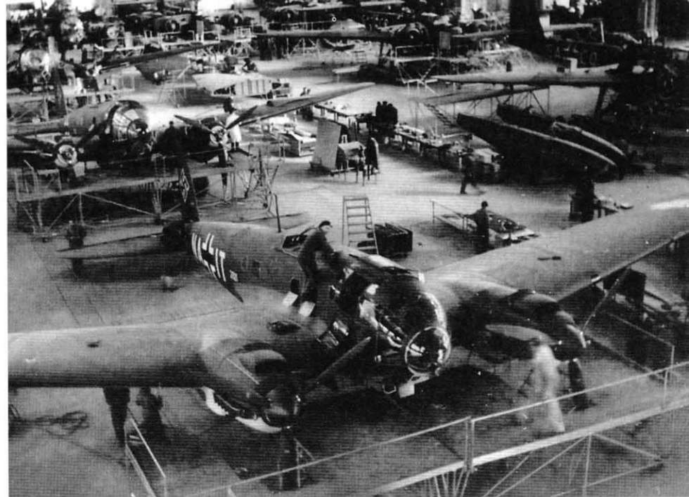
An He 111P (NA+IT, Werk Nr. 2921) undergoes final assembly at Heinkel's Rostock-Marienehe factory. White radio codes were painted at the factory, then were repainted in Staffel colors when delivered to their units. He 115 floatplanes are being assembled alongside the He 111 bombers. (Werkfoto via Petrick)
