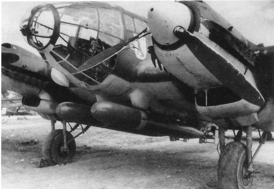
This He 111H-6 assigned to KG 26 is armed with two 765 kg (1686.5 pound) LT F5b torpedoes. The weapons were mounted on PVC 1006 racks fitted to the fuselage undersurface. Temporary wooden fins stabilized the torpedo's entry into the water, then broke away from the weapon. The torpedo was believed to have a dark gray nose and an aluminum body. In early 1941, KG 26 deployed from Norway to Grosseto, Italy for anti-shipping operations in the Mediterranean Sea theatre. (Punka Archiv)
