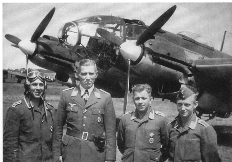
Early He 111s were equipped with VDM three bladed metal propellers. These propellers featured narrow blades and had variable pitch for various flight conditions. The VDM propeller was replaced by Junkers VS-11 wooden propellers on the He 111H-6. (Smithsonian Institution)
