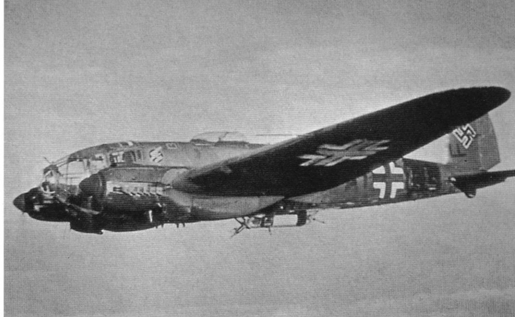
A forward-firing 20mm MG FF cannon is mounted in the ventral gondola of this He 111H-10 (A1+LL) of 3/KG 53 'Legion Condor.' This weapon was primarily used to attack surface targets on land and sea, although it was also employed against enemy aircraft. He 111 gunners nicknamed the gondola the 'Sterbebett' ('Deathbed'), due to their vulnerability to enemy fire. The aircraft's undersurfaces are overpainted black for night bombing missions. (Punka Archiv)
