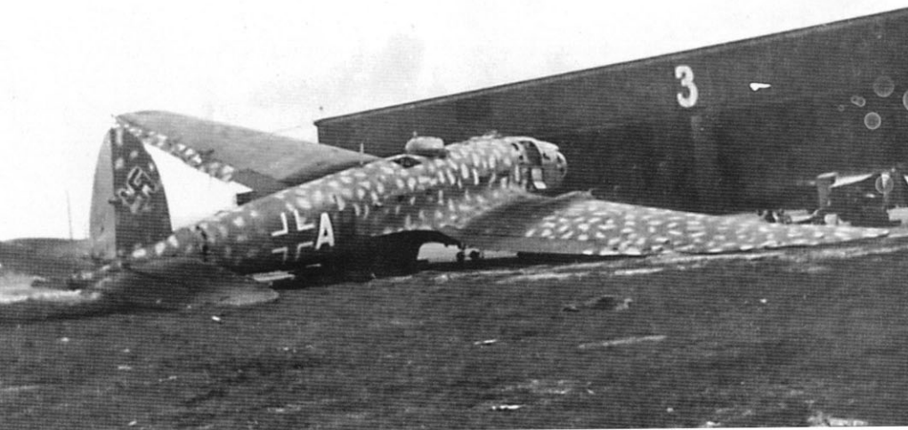
An He 111H-16/R1 (+AH) lies damaged at Hradec Králové airfield, Czechoslovakia in May of 1945. Retreating German troops damaged the aircraft to prevent its use by advancing Soviet forces. This variant featured a turret-mounted 13mm MG 131 machine gun in the dorsal position. RLM 76 Light Gray (FS36473) mottling was painted over the upper surface camouflage. (Zdenek)
