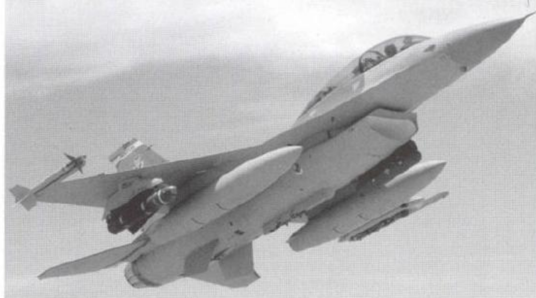
F-16D on a 1994 training mission out of Shaw AFB, S.C. It carries a LANTIRN (FLIR/TFR) navigation pod on the port intake, 5L stores adapter and an inert AGM-65 Maverick missile on the port intermediate wing station. (Lou Drendel)
