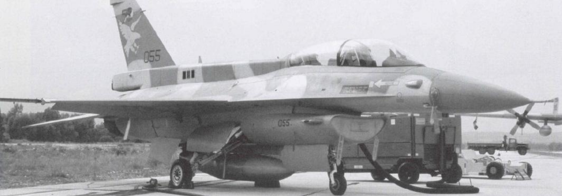
(Above) F-16D of the Valley Squadron of the Tsvah Haganah le Israel/Heyl Ha'Avir (Israel Defense Force/Air Force). All of the IDF/AF's F-16D two-seaters (both Block 30 and Block 40 aircraft) have been fitted with enlarged dorsal spines. Although the IDF/AF has not revealed exactly what is in these spines, they are believed to accommodate Wild Weasel electronic equipment which detects emissions from enemy radar sites and pinpoints their locations. Other speculation is that the "hump" on some of these aircraft is for a nuclear weapons delivery capability. Only the F-16D has the enlarged dorsal spine, the two-seat F-16B being similar to the USAF version. (Steven Drew via Andre Jans)
