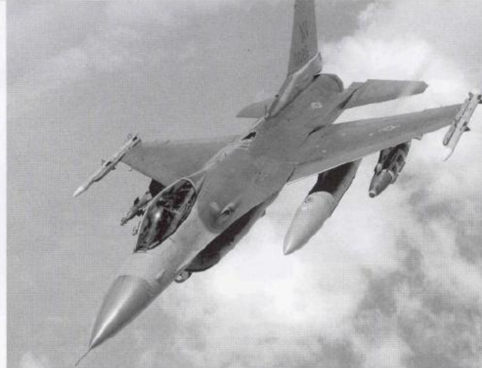
An F-16C of the 555th TFS, out of Aviano AB, Italy moves into refueling position during Operation Iraqi Freedom. During the second Gulf War, most munitions carried by the F-16 were precision-guided, either JDAM or LGB as on this Viper, which carries two 1,000 pound LGBs and one 2,000 pound JDAM. (USAF)
