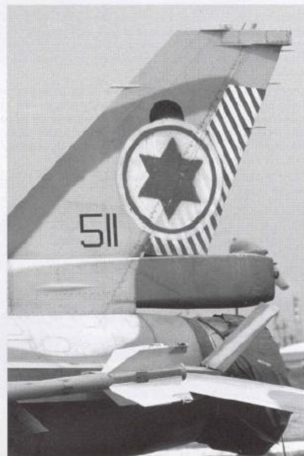
(Above) F-16D of the Valley Squadron of the Tsvah Haganah le Israel/Heyl Ha'Avir (Israel Defense Force/Air Force). All of the IDF/AF's F-16D two-seaters (both Block 30 and Block 40 aircraft) have been fitted with enlarged dorsal spines. Although the IDF/AF has not revealed exactly what is in these spines, they are believed to accommodate Wild Weasel electronic equipment which detects emissions from enemy radar sites and pinpoints their locations. Other speculation is that the "hump" on some of these aircraft is for a nuclear weapons delivery capability. Only the F-16D has the enlarged dorsal spine, the two-seat F-16B being similar to the USAF version. (Steven Drew via Andre Jans)
