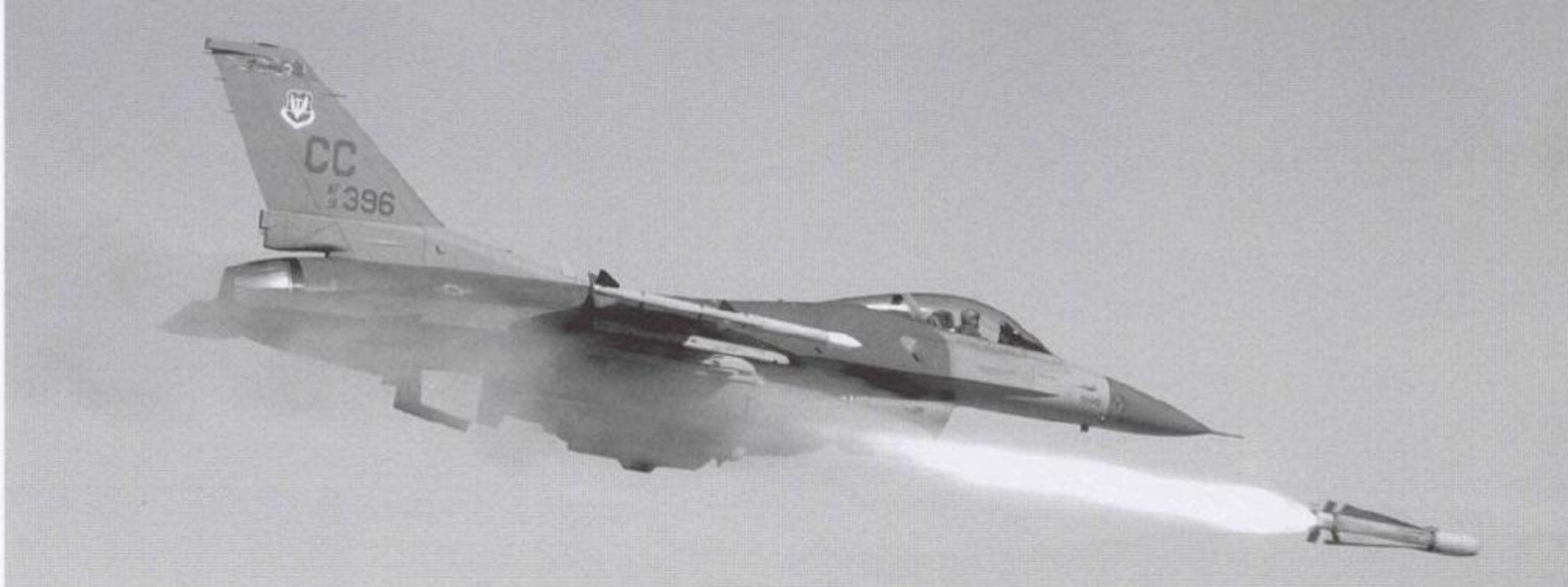
An F-16C Fighting Falcon assigned to the 522nd Fighter Squadron at Cannon Air Force Base, N.M., fires an AGM-65H Maverick air-to-ground missile at a target located over the Utah Test and Training Range. The mission was part of an air-to-ground weapons system evaluation program commonly referred to as Combat Hammer. The squadron is deployed to Hill AFB, Utah. The Maverick missile family provides day, night, and limited adverse weather capability and is currently USAF's primary discriminatory antitank weapon. Maverick is a primary weapon for LANTIRN equipped aircraft. (U.S. Air Force photo by Master Sgt. Michael Ammons)
