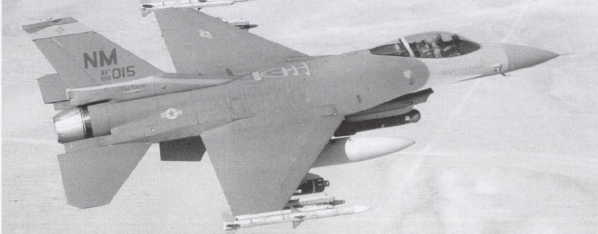
(Above) In 2002 the U.S. Air Force began using a software update developed by Lockheed Martin Aeronautics Co. that added new "smart" weapons capability to its 400-aircraft fleet of Block 40/42 F-16C/Ds. The weapons included the GBU-31 Joint Direct Attack Munition (JDAM) – INS/GPS (Inertial Navigation System/Global Positioning System [satellite]) guidance, the AGM-154 Joint Stand-Off Weapon (JSOW) – INS/GPS guidance, the CBU-103/104/105 Wind-Corrected Munitions Dispenser (WCMD) – INS guidance, EGBU-27 enhanced laser-guided bomb – laser seeker plus INS/GPS guidance. (Lockheed Martin)
