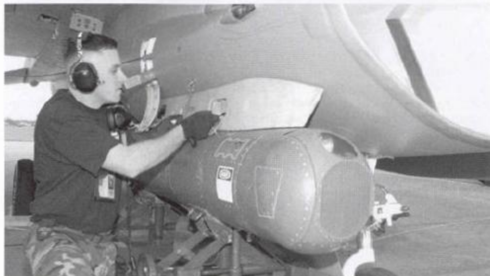
LACKLAND AIR FORCE BASE, Texas -- Tech. Sgt. Marcos Farias attaches a Low-Altitude Navigation and Targeting Infrared for Night targeting pod to a 149th Fighter Wing F-16 Fighting Falcon. The 149th FW was the first unit in the Air Force to graduate pilots from the F-16 basic course with targeting-pod training. (U.S. Air Force photo by Senior Master Sgt. Mike Arellano)
