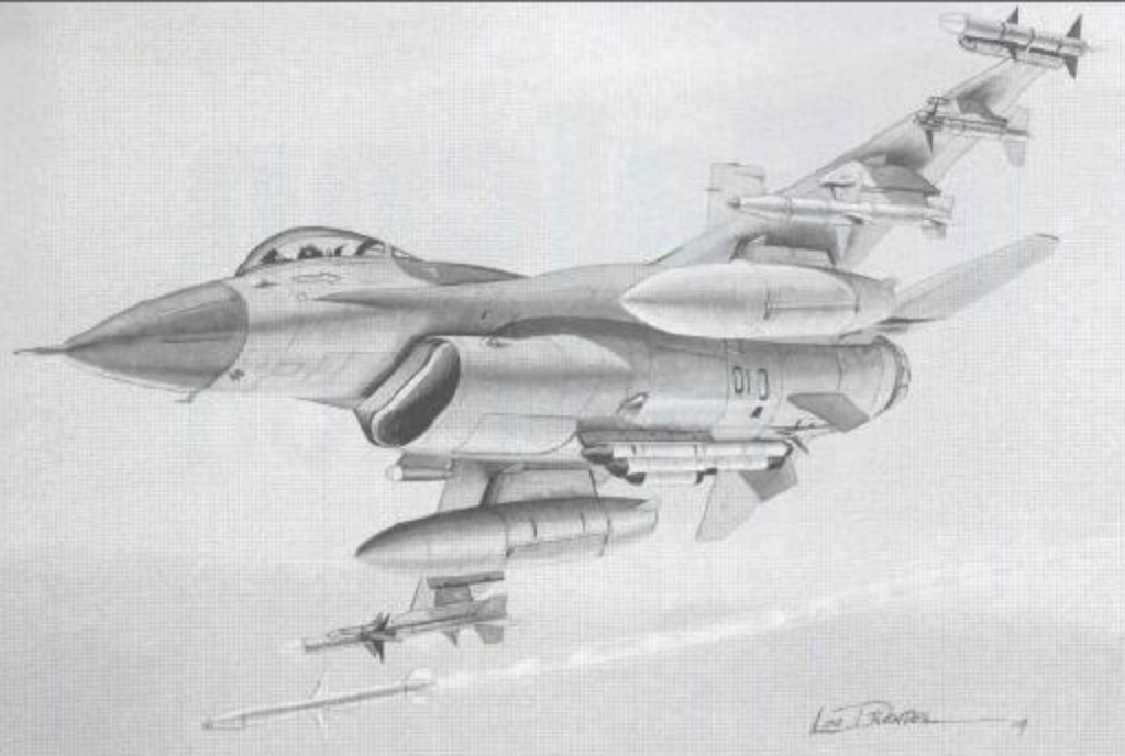
Cover: The Suppression of Enemy Air Defenses (SEAD) configured F-16C firing an AGM-88 High Speed Anti-Radiation (HARM) missile at an enemy radar site.
