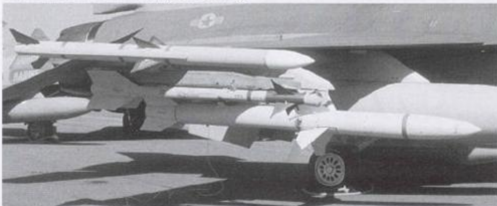
An F-16CJ with typical SEAD mission armament of AIM-120 and AIM-9 air-to-air missiles and AGM-88 HARM missiles. (John Gourley)
