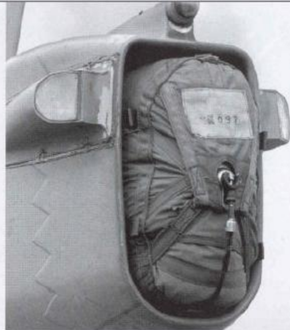
The parachute braking system was originally designed for use by the Royal Norwegian Air Force. It has since been used on several other foreign F-16s. RHAW antennas are installed on either side of the chute housing. (John Gourley)
