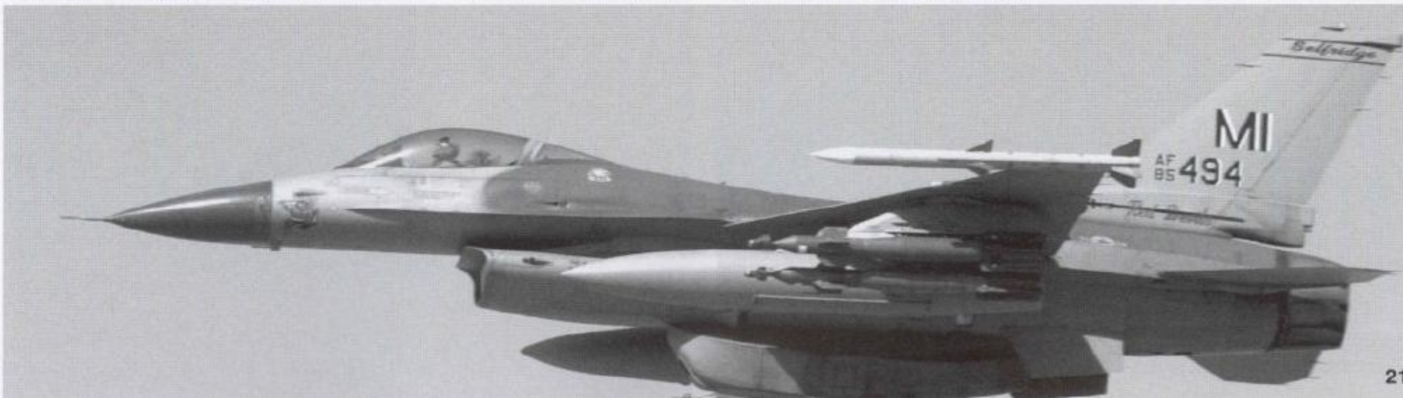
(Below) OVER IRAQ -- An F-16 Fighting Falcon on a 28 April 2003 mission in support of Operation Iraqi Freedom. The F-16 is assigned to the Michigan Air National Guard's 107th Fighter Squadron at Selfridge Air National Guard Base. It carries LGBs, but no target pod, and is also loaded with a tactical reconnaissance pod on the centerline. With the retirement of the RF-4 Phantom II, USAF no longer had a dedicated tactical reconnaissance aircraft, which necessitated development of the AN/ASD-11 Theatre Airborne
