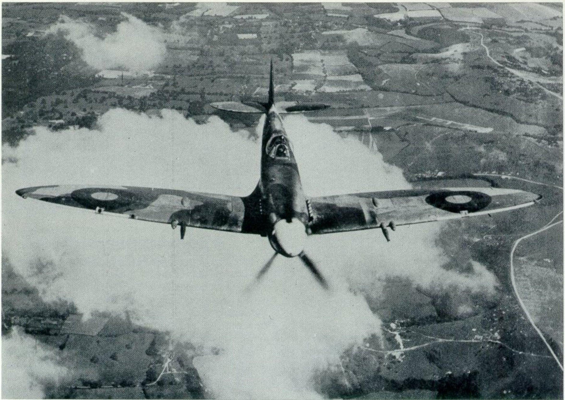
Frontal view of a Spitfire F.Mk.XIV C shows off the "tear-drop" hood/"bubble" canopy.
