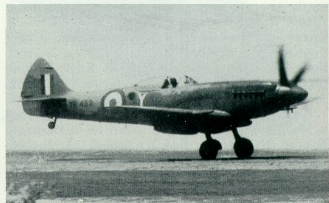
Destined for the Middle East and No. 208 Squadron, RAF, a Spitfire FR.Mk.XVIII (TP334) photographed while, presumably, still being held by No. 109 Maintenance Unit, RAF. The camera port is covered. (Photo: Air-Britain Photo Library)
