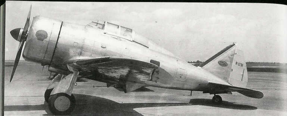
The SEV-DS (Doolittle Special) was flown by Major James Doolittle for the Shell Oil Company testing 100 octane aviation fuel. It differed from military P-35s in that it was powered by a Wright R-1820 engine, had a cut down canopy and a flat wing. (Vincent Berinati)
