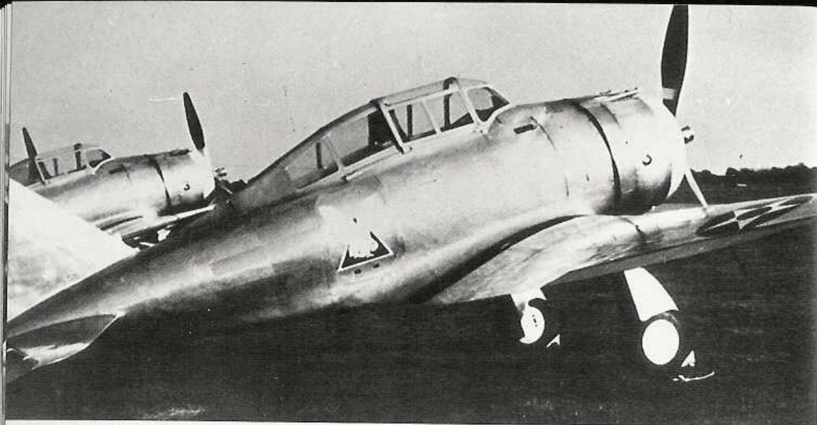
A pair of 17th PS P-35s at Nichols Field during 1941. It is generally assumed that no regular production P-35s went to the Philippines, but neither of these aircraft have the .50 caliber wing guns and their cowl guns are unfaired which are standard fittings on P-35As. (AFM)
