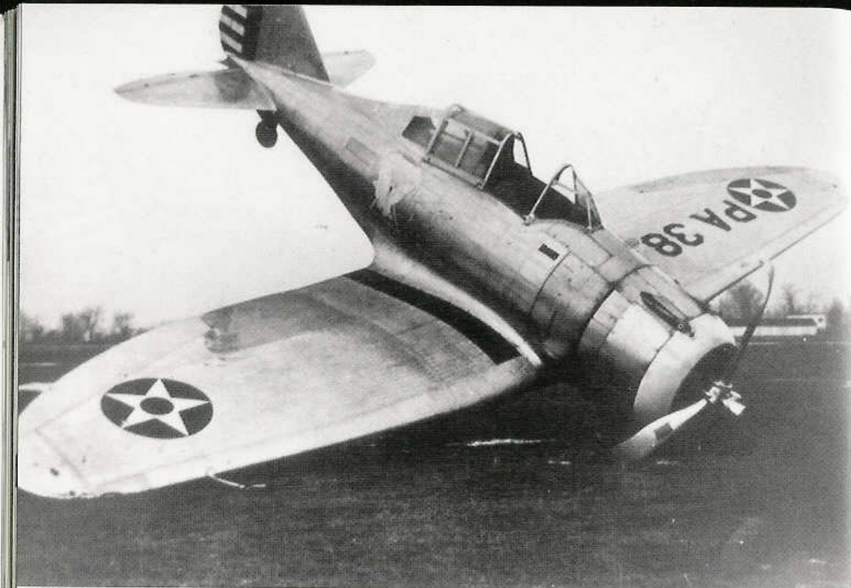
The narrow landing gear of the P-35 led to many ground accidents such as this nose over of a 17th Pursuit Squadron P-35. The aircraft was of sturdy construction and repairs were usually quickly made and the aircraft returned to flyable condition. (AFM)
