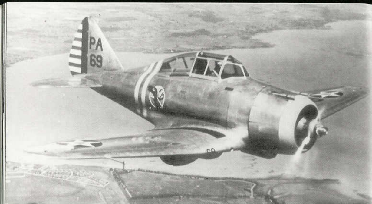
The first P-35s to enter squadron service went to the 1st Pursuit Group based at Selfridge Field, Michigan. This P-35 was assigned to the 27th Pursuit Squadron and was flown by the squadron commander. It carries a Yellow nose and command stripes on the rear fuselage. The aircraft also had the production semi-enclosed landing gear housings in place of the fully enclosed housing found on the first production aircraft. (AFM)
