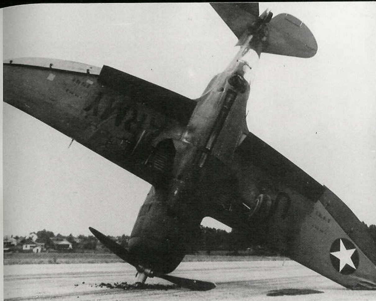
This P-43A (40-2939) of the 122nd Reconnaissance Squadron nosed over on landing at Winston Salem, North Carolina during maneuvers held in 1942. The white band around the rear fuselage was a special marking applied to the aircraft for the war games.
