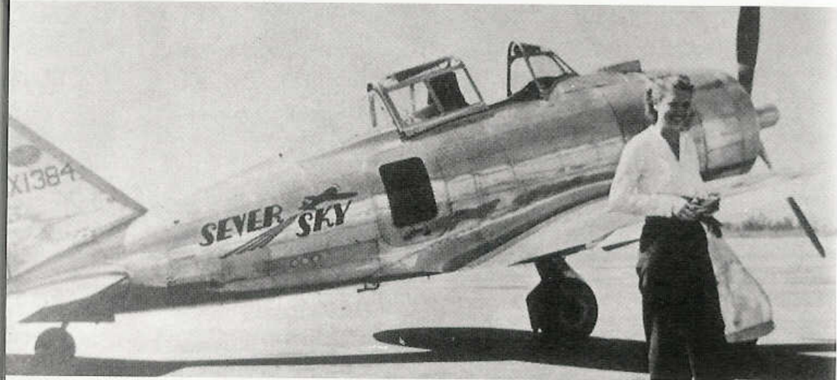
At one point the AP-1 demonstrator was fitted with a large spinner and tight cowling in an attempt to reduce drag.
