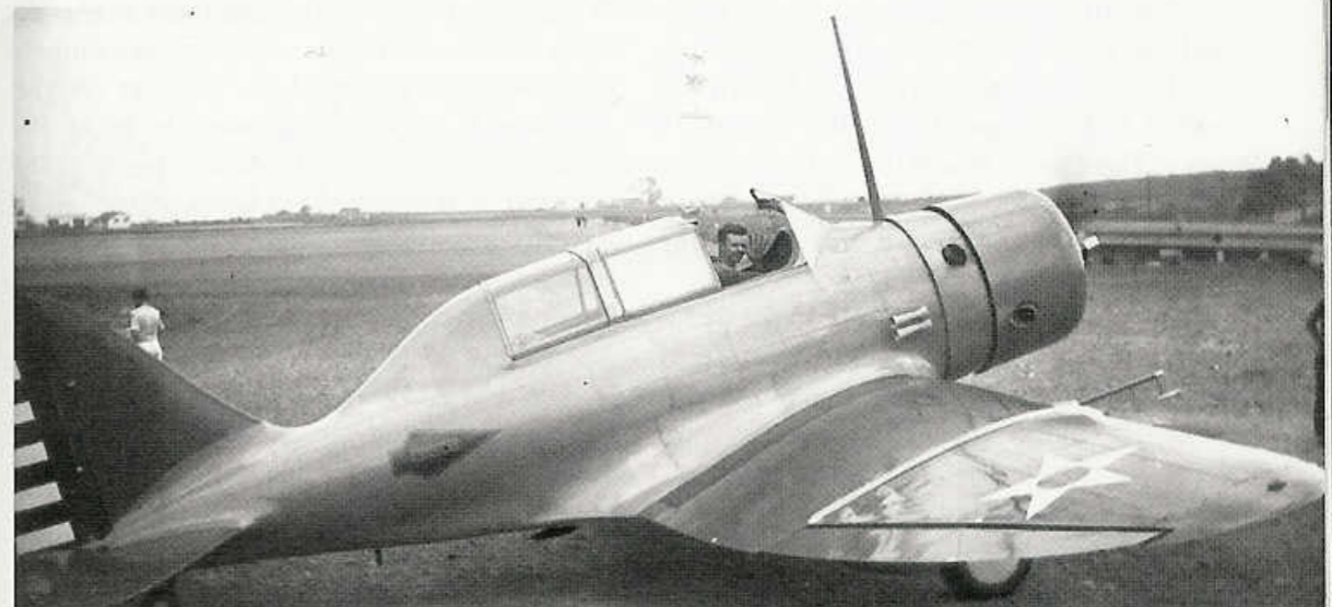
The SEV-1XP was the prototype P-35 aircraft. The SEV-1XP had rearward retracting main landing gear and was powered by a Wright R-1820 Cyclone engine driving a two-blade propeller. The prototype had a large engine cowling and rounded vertical tail/rudder assembly. (AFM)
