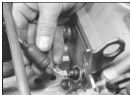
11.23c Oil pressure switch electrical connection
