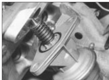
11.7a Fitting fuel pump
