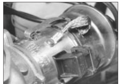
11.10 Fitting distributor cap and earth lead
