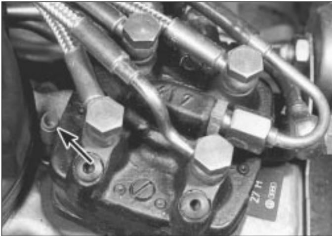
7.2 Idle CO adjustment screw location (arrowed)
