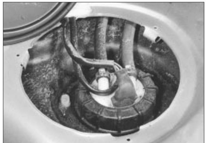
18.2 Fuel tank sender unit and connections
