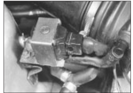
5.2 Increased idling speed valve (air conditioned models)
