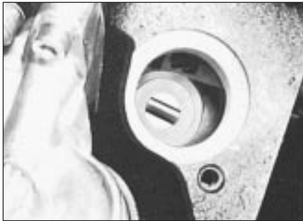
7.22 Oil pump drive spigot position prior to refitting distributor
