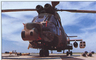
Mock up of the stabilised sighting system fitted to an Oryx (AFI)
