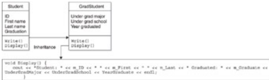
Figure 3-2: The GradStudent class has attributes and procedures that are the same and some that are different from the Student class.
