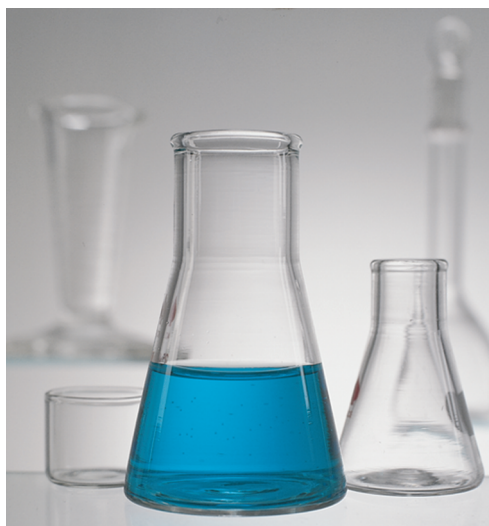
FIG. 17.6 The complex ion of \text{Cu}^{2+} and water. A solution containing copper sulfate has a blue color because it contains the complex ion \text{Cu}(\text{H}_2\text{O})_4^{2+} . (Andy Washnik.)
