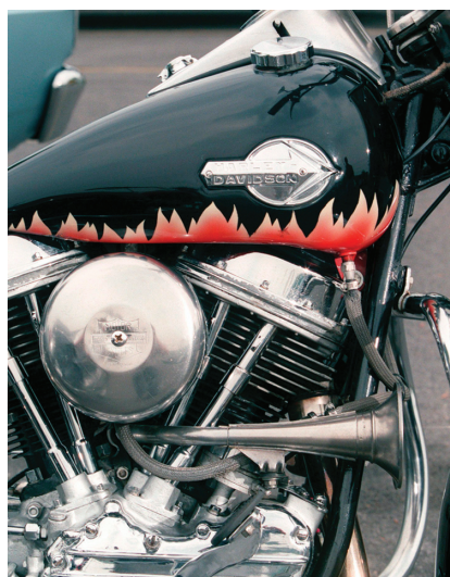
This motorcycle sparkles with chrome plating that was deposited by electrolysis. The shiny hard coating of chromium is both decorative and a barrier to corrosion. ( Syracuse Newspapers/The Image Works. )
