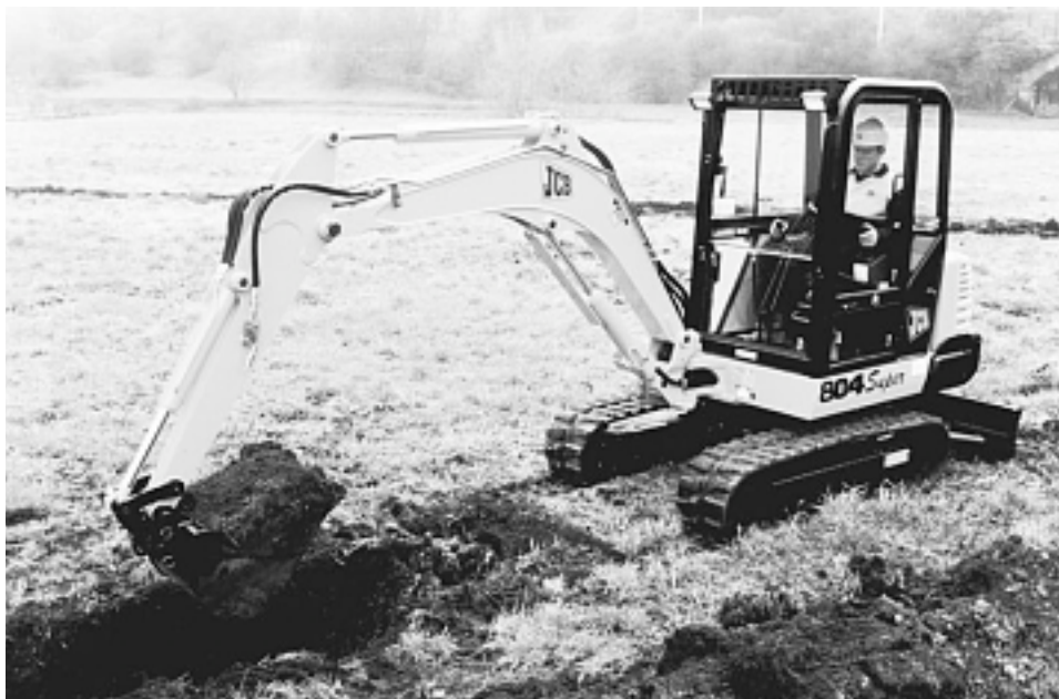
Figure 3-5 Mini-excavator. (Courtesy of JCB Inc.)
