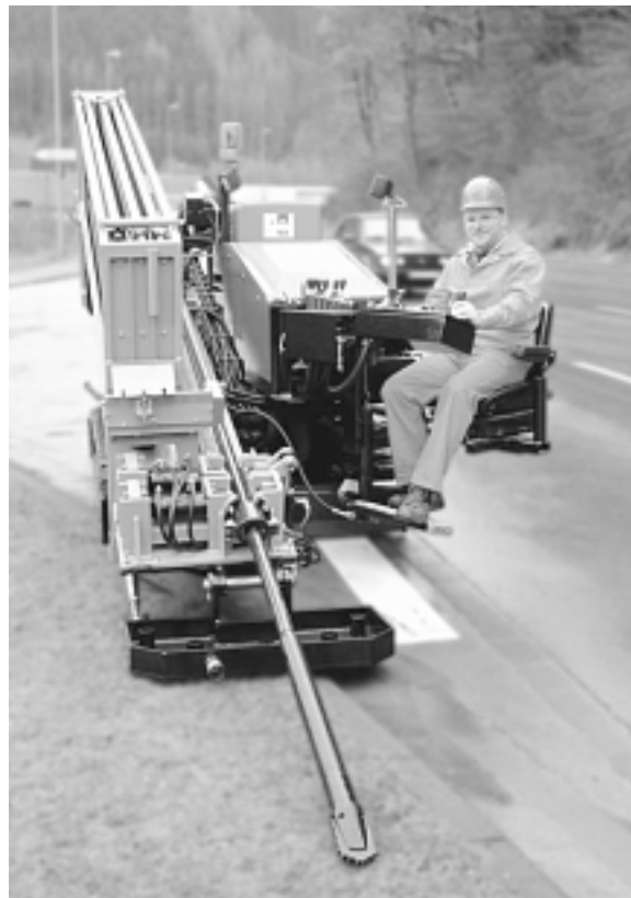
Figure 3-19 Grundodrill & Thrust boring machine with percussive action. (Courtesy of TT Technologies, Inc.)
