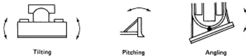
Figure 4-8 Dozer blade adjustment.
