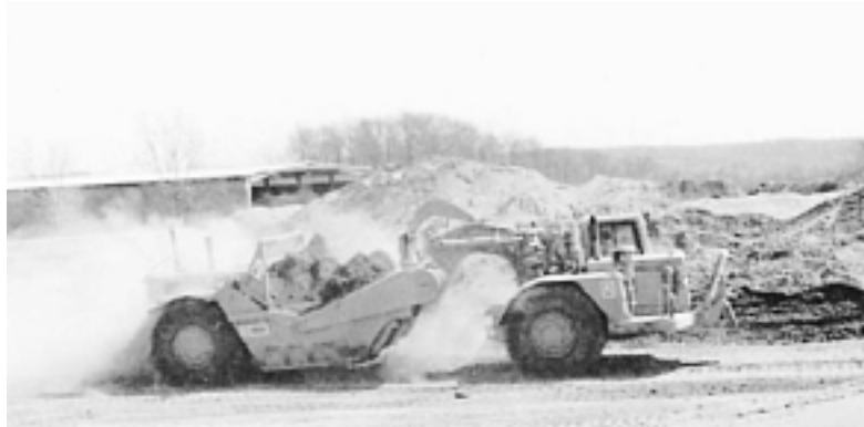
Figure 4-17 Twin-engine all-wheel drive scraper. (Courtesy of Caterpillar Inc.)
