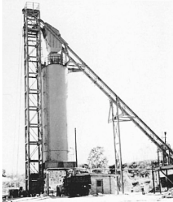
Figure 7-11 Insulated hot-mix asphalt storage bin with skip hoist. (Courtesy of Terex Road Building)
