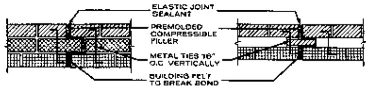
EXPANSION JOINTS IN STRAIGHT WALLS
