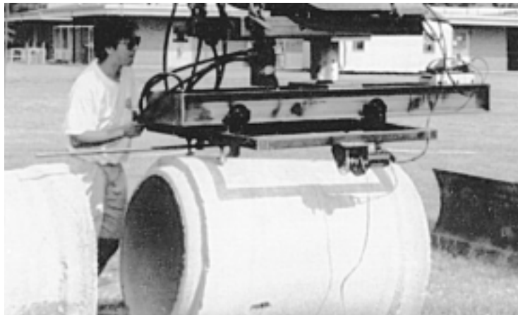
Figure 20-8 Remote-controlled pipe manipulator. (Courtesy of the Construction Automation and Robotics Laboratory, North Carolina State University)
