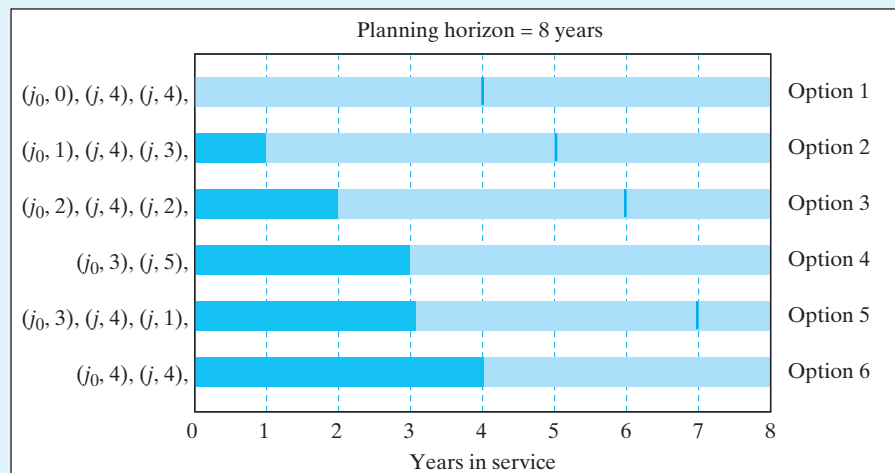
Figure 14.9 Some likely replacement patterns under a finite planning horizon of eight years (Example 14.5).
