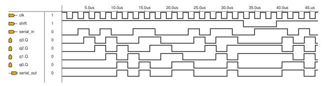
FIGURE 7-78 SISO register simulation.
