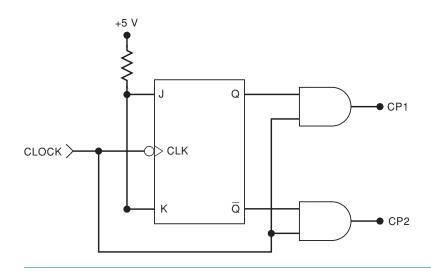
(b) This circuit would have a problem if the FF were changed to one that responds to a PGT at *CLK*. Draw the CP1 and CP2 waveforms for that situation. Pay particular attention to conditions that can produce glitches.
