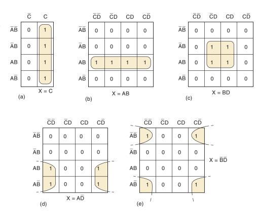
As another example, consider Figure 4-13(d), where the four squares containing 1s are  $AB\overline{C}\overline{D}$ ,  $A\overline{B}\overline{C}\overline{D}$ ,  $ABC\overline{D}$ , and  $A\overline{B}C\overline{D}$ . Examination of these terms indicates that only the variables A and  $\overline{D}$  remain unchanged, so that the simplified expression for X is
