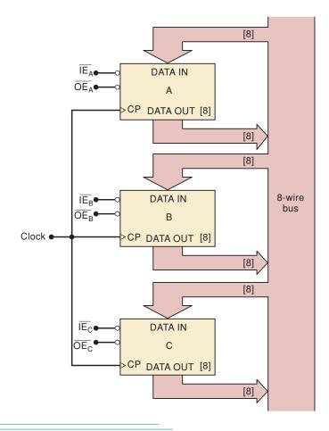
The connections to and from the data bus are represented by wide arrows. The numbers in brackets indicate the number of bits that each register contains, as well as the number of lines connecting the register inputs and outputs to the bus.
