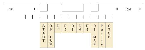
FIGURE 2-5 Asynchronous serial data with even parity.
