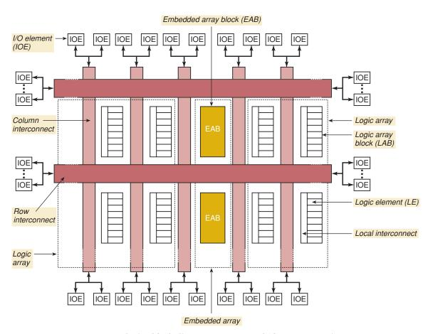
FIGURE 13-18 FLEX10K device block diagram. (Courtesy of Altera Corporation.)
