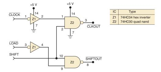
the gates on this chip are designated with the label Z2. By numbering each gate as Z1, Z2, Z3, and so on, we can keep track of which gate is part of which chip. This is especially valuable in more complex circuits containing many ICs with several gates per chip.
