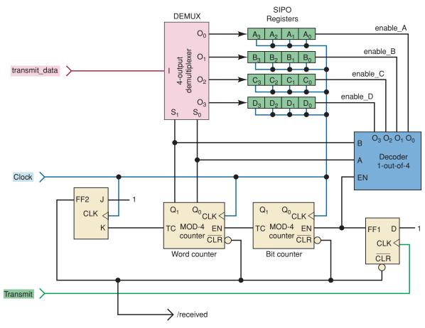
FIGURE 9-33 Receiver block in synchronous data transmission system.
