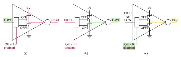
FIGURE 8-35 Three output conditions of tristate.
