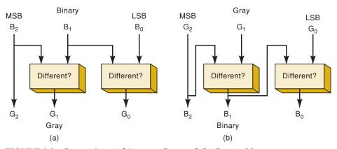
FIGURE 2-2 Converting (a) binary to Gray and (b) Gray to binary.
