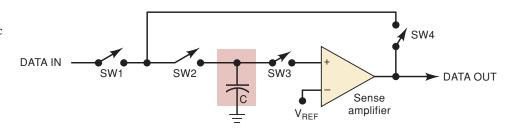
writing to and reading from a DRAM. The switches SW1 through SW4 are actually MOSFETs that are controlled by various address decoder outputs and the  $R/\overline{W}$  signal. The capacitor, of course, is the actual storage cell. One sense amplifier would serve an entire column of memory cells, but operate only on the bit in the selected row.
