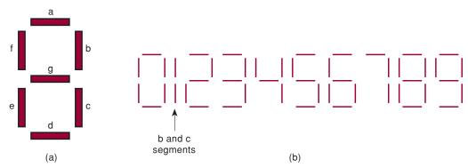
FIGURE 9-7 (a) 7-segment arrangement; (b) active segments for each digit.
