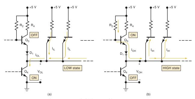
FIGURE 8-13 Currents when a TTL output is driving several inputs.
