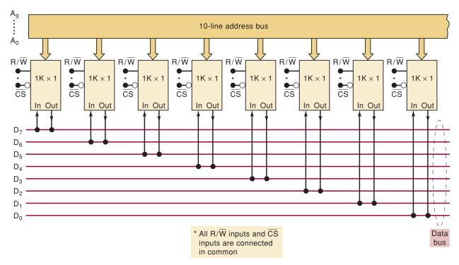
**FIGURE 12-35** Eight 2125A 1K  $\times$  1 chips arranged as a 1K  $\times$  8 memory.
