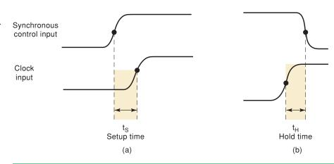
minimum acceptable value of hold time  $t_H(min)$ . If this requirement is not met, the FF will not trigger reliably.
