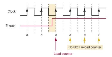
In order to know what the *trigger* was on the last active clock edge, the system must remember the last value that *the trigger had at that point*. This is done by storing the value of the trigger bit in a flip-flop. Recall that we discussed a similar concept in Chapter 5 when we talked about using a flip-flop to detect a sequence. The code for a one-shot is written so that the counter is loaded only after a rising edge is detected on the *trigger* input.
