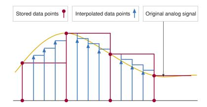
with simpler analog circuitry. DSP performs this role in your CD player to provide an excellent audio reproduction. The round dots represent the digitally recorded data on your CD. The triangles represent the interpolated data points that the digital filter in your CD player inserts before the final analog output filter.
