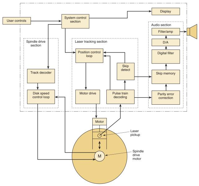
FIGURE 4-45 Block diagram of a CD player.
