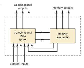
to produce various outputs, some of which are used to determine the binary values to be stored in the memory elements. The outputs of some of the memory elements, in turn, go to the inputs of logic gates in the combinational circuits. This process indicates that the external outputs of a digital system are functions of both its external inputs and the information stored in its memory elements.
