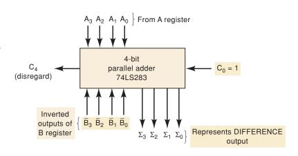
4. The parallel-adder circuitry adds [A] = 0100 to  $[\overline{B}] = 1001$  along with a carry,  $C_0 = 1$ , into the LSB. The operation is shown below.
