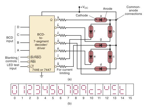
Seven-segment decoder/drivers such as the 7446/47 are exceptions to the rule that decoder circuits activate only one output for each combination of inputs. Rather, they activate a unique pattern of outputs for each combination of inputs.
