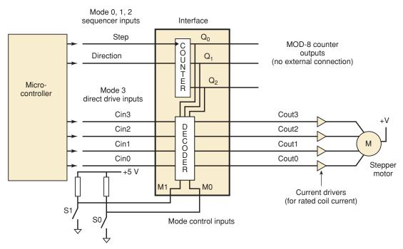
FIGURE 10-1 A universal stepper motor interface circuit.
