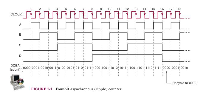
counter is in the 0000 state. In other words, the counter has gone through one complete cycle (0000 through 1111) and has *recycled* back to 0000. From this point, it will begin a new counting cycle as subsequent clock pulses are applied.
