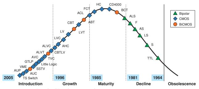
FIGURE 8-27 Logic product life cycle. (Courtesy of Texas Instruments)
