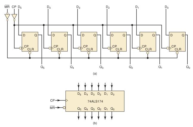
FIGURE 7-62 (a) Circuit diagram of the 74ALS174; (b) logic symbol.
