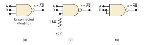
input B is not going to have its fan-out exceeded. This technique can be used for *any* type of gate. For OR gates and NOR gates, the unused inputs cannot be left disconnected or tied to +5 V because this would produce a constant-output logic level (1 for OR, 0 for NOR) regardless of the other inputs. Instead, for these gates, the unused inputs must either be connected to ground (0 V) for a logic 0 or be tied to a used input, as in Figure 8-15(c).
