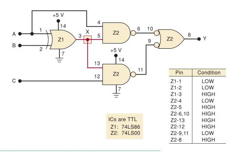
When the circuit is tested, the technician observes that output Y goes HIGH whenever A is HIGH or C is HIGH, regardless of the level at B. She takes logic probe measurements for the condition where A = B = 0, C = 1 and comes up with the indications recorded in Figure 4-41.
