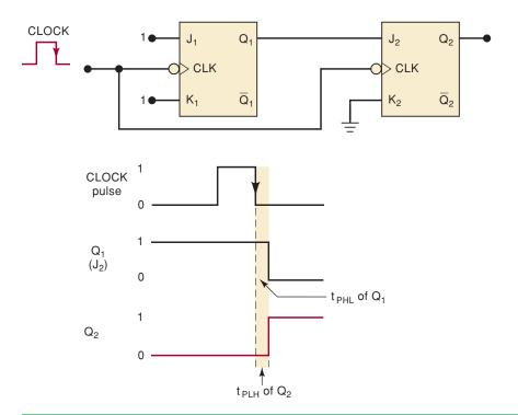
The potential timing problem is this: because  $Q_1$  will change on the NGT of the clock pulse, the  $J_2$  input of  $Q_2$  will be changing as it receives the same NGT. This could lead to an unpredictable response at  $Q_2$ .
