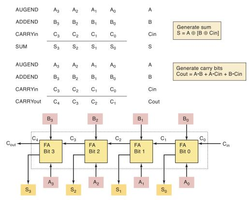
FIGURE 6-19 Four-bit parallel adder.
