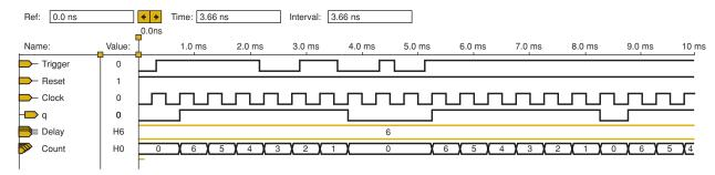
FIGURE 7-90 Simulation of the nonretriggerable one-shots.
