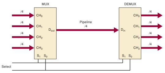
FIGURE 9-61 Four channels of data sharing a common data path.
