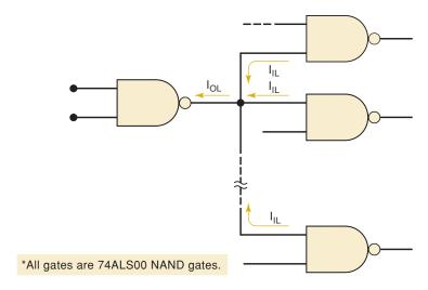
(*Note:* The entry for  $I_{\rm IL}$  is actually -0.1 mA. The negative sign is used to indicate that this current flows *out of* the input terminal; we can ignore this sign for our purposes here.) The HIGH state is analyzed in the same manner. Refer to the data sheet to find values for  $I_{\rm OH}$  and  $I_{\rm IH}$ , ignoring any negative signs.
