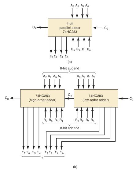
8-bit numbers.  $C_8$  is the carry out of the MSB position. It can be used as the carry input to a third adder stage if larger binary numbers are to be added.
