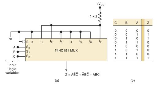
connected LOW. Likewise, Z is supposed to be LOW for CBA = 011, 100, 101, and 110, so that inputs  $I_3$ ,  $I_4$ ,  $I_5$ , and  $I_6$  should also be connected LOW. The other sets of CBA conditions must produce Z = 1, and so multiplexer inputs  $I_1$ ,  $I_2$ , and  $I_7$  are connected permanently HIGH.
