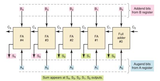
FIGURE 6-6 Block diagram of a five-bit parallel adder circuit using full adders.
