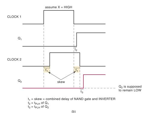
clock skew. The NGT of *CLOCK1* will cause  $Q_1$  to go HIGH after a time  $t_2$  that is equal to  $Q_1$ 's  $t_{\rm PLH}$  propagation delay. If  $t_2$  is less than the skew  $t_1$ ,  $Q_1$  will be HIGH when the NGT of *CLOCK2* occurs, and this may incorrectly set  $Q_2 = 1$  if its setup time requirement,  $t_{\rm S}$ , is met.
