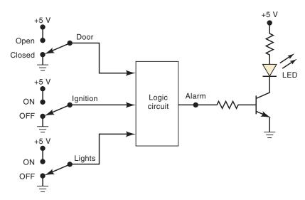
indicate the status of the door by the driver's seat, the ignition, and the headlights, respectively. Design the logic circuit with these three switches as inputs so that the alarm will be activated whenever either of the following conditions exists:
