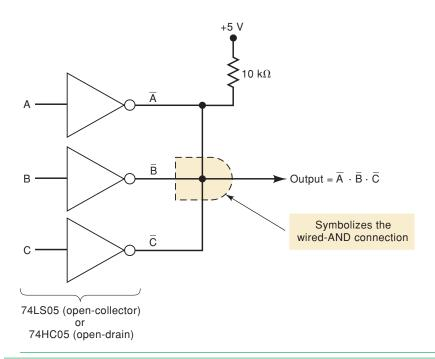
state. Because the common output is HIGH only when all the outputs are in the HIGH state, connecting the outputs in this way essentially implements the logic AND function. This is called a **wired-AND** connection. This is shown symbolically by the dotted AND gate symbol. There is no actual AND gate there. A wired-AND can be implemented only with open-collector TTL and open-drain CMOS logic devices.
