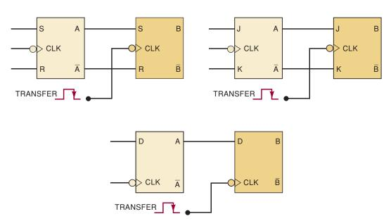
**FIGURE 5-42** Synchronous data transfer operation performed by various types of clocked FFs.
