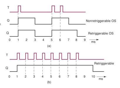
Both types of OS respond to the first trigger pulse at t=1 ms by going HIGH for 2 ms and then returning LOW. The second trigger pulse at t=5 ms triggers both one-shots to the HIGH state. The third trigger pulse at t=6 ms has no effect on the nonretriggerable OS because it is already in its quasistable state. However, this trigger pulse will *retrigger* the retriggerable OS to begin a new  $t_p=2$  ms interval. Thus, it will stay HIGH for 2 ms *after* this third trigger pulse.
