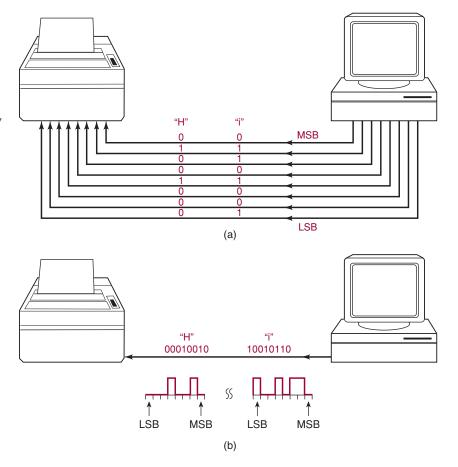
Figure 1-10(a) demonstrates parallel transmission of data from a computer to a printer using the parallel printer port (LPT1) of the computer. In this scenario, assume we are trying to print the word "Hi" on the printer. The
