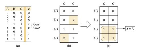
Here the output z is not specified as either 0 or 1 for the conditions A, B, C = 1, 0, 0 and A, B, C = 0, 1, 1. Instead, an x is shown for these conditions. The x represents the **don't-care condition**. A don't-care condition can come about for several reasons, the most common being that in some situations certain input combinations can never occur, and so there is no specified output for these conditions.
