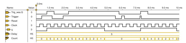
FIGURE 7-94 Simulation of the edge-triggered retriggerable one-shot.
