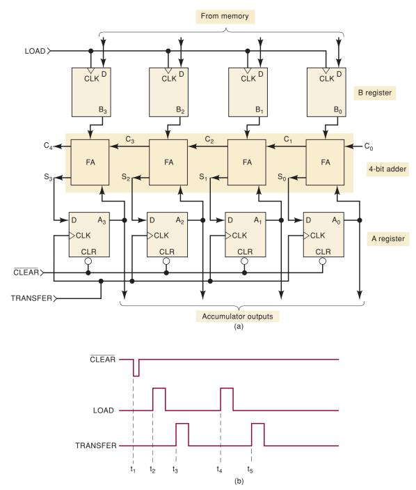
**FIGURE 6-10** (a) Complete four-bit parallel adder with registers; (b) signals used to add binary numbers from memory and store their sum in the accumulator.
