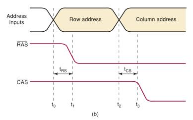
**FIGURE 12-27** (a) Simplified architecture of the TMS44100 4M  $\times$  1 DRAM; (b)  $\overline{RAS}/\overline{CAS}$  timing. (Reprinted by permission of Texas Instruments)
