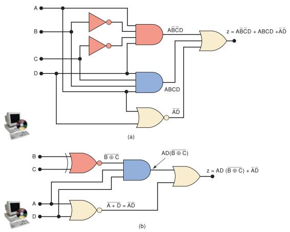
**FIGURE 4-24** Example 4-18, showing how an XNOR gate may be used to simplify circuit implementation.
