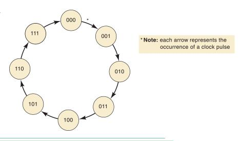
Each circle represents one possible state, as indicated by the binary number inside the circle. For example, the circle containing the number 100 represents the 100 state (i.e.,  $Q_2 = 1$ ,  $Q_1 = Q_0 = 0$ ).
