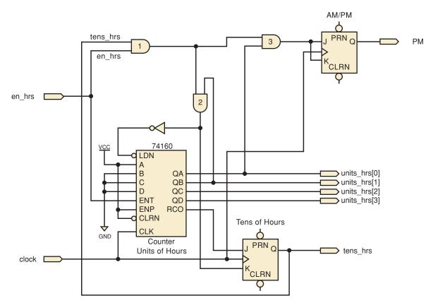
FIGURE 10-18 Detailed circuitry for the HOURS section.
