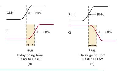
Modern IC flip-flops have propagation delays that range from a few nanoseconds to around 100 ns. The values of  $t_{\rm PLH}$  and  $t_{\rm PHL}$  are generally not the same, and they increase in direct proportion to the number of loads being driven by the Q output. FF propagation delays play an important part in certain situations that we will encounter later.
