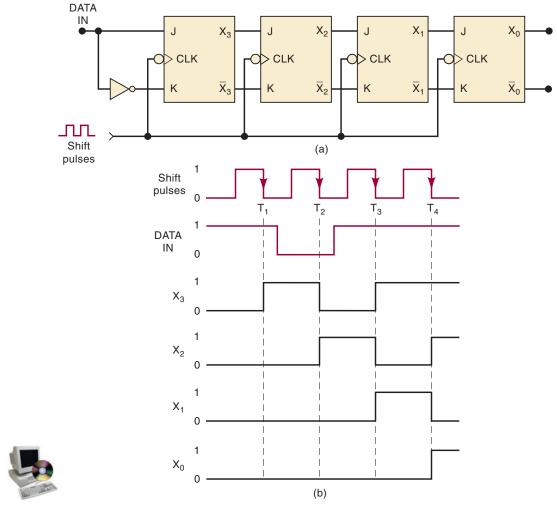
FIGURE 5-45 Four-bit shift register.
