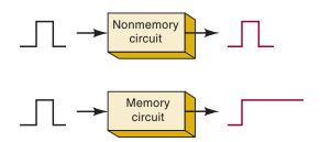
Memory devices and circuits play an important role in digital systems because they provide a means for storing binary numbers either temporarily or permanently, with the ability to change the stored information at any time. As we shall see, the various memory elements include magnetic and optical types and those that utilize electronic latching circuits (called *latches* and *flip-flops*).
