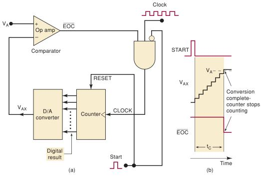
FIGURE 11-13 Digital-ramp ADC.
