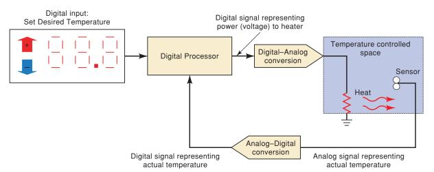
FIGURE 1-1 Block diagram of a precision digital temperature control system.
