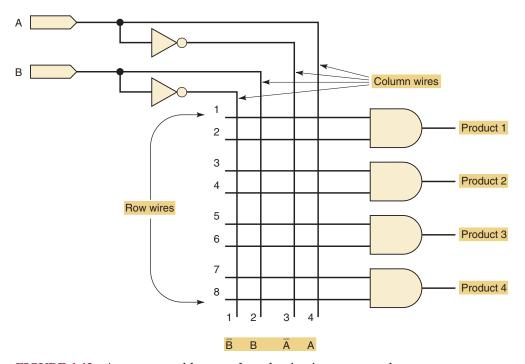
FIGURE 4-42 A programmable array for selecting inputs as product terms.
