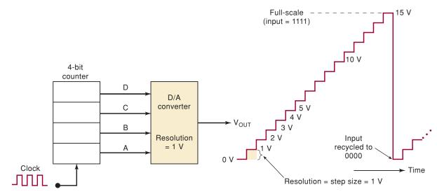
**FIGURE 11-3** Output waveforms of a DAC as inputs are provided by a binary counter.
