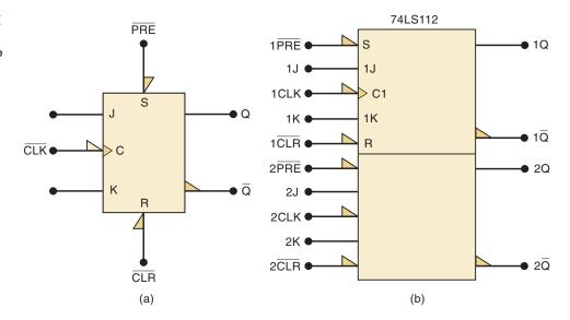
like the one symbolized in Figure 5-33(a). Note how the inputs and outputs are numbered. Also note that the input labels inside the rectangles are shown only for the top FF. It is understood that the inputs to the bottom FF are in the same arrangement as the top one. This same IC symbol applies to the CMOS 74HC112.
