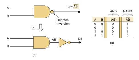
The truth table in Figure 3-22(c) shows that the NAND gate output is the exact inverse of the AND gate for all possible input conditions. The AND output goes HIGH only when all inputs are HIGH, while the NAND output goes LOW only when all inputs are HIGH. This same characteristic is true of NAND gates having more than two inputs.
