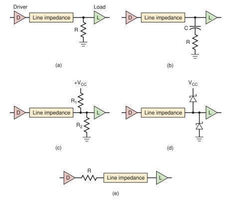
diode termination shown in Figure 8-40(d) simply clips off or clamps the overshoot/undershoot of the ringing caused by the reactive LC nature of the line. Series termination at the source, as shown in Figure 8-40(e), slows down the switching speed, which reduces the frequency limits of the bus but substantially improves the reliability of the bus signals.
