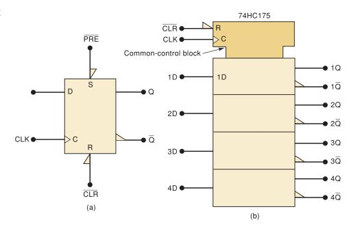
Figure 5-34(b) is the IEEE/ANSI symbol for a 74HC175 IC, which contains four D flip-flops that share a common CLK input and a common  $\overline{CLR}$  input. The FFs do not have a  $\overline{PRE}$  input. This symbol contains a separate rectangle to represent each FF, and a special **common-control block**, which is the notched rectangle on top. The common-control block is used whenever an
