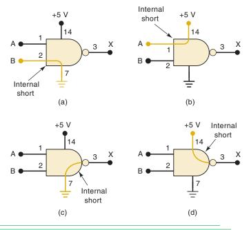
Similarly, an IC input pin could be internally shorted to +5 V, as in Figure 4-35(b). This would keep that pin stuck in the HIGH state. If this input pin is being driven by a logic signal A, it will effectively short A to +5 V.
