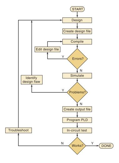
After each circuit in a subsection has been tested, all can be combined and the subsection can be tested following the same process that was used for the small circuits. Then the subsections are combined and the system is tested. This approach lends itself very well to a typical project environment, where a team of people are working together, each responsible for his or her own circuits and sections that will ultimately come together to make up the system.
