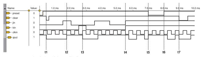
**FIGURE 5-69** Simulation of the JK flip-flop.
