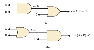
the circuit in Figure 3-13(a). This circuit has three inputs, A, B, and C, and a single output, x. Utilizing the Boolean expression for each gate, we can easily determine the expression for the output.
