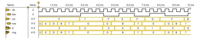
FIGURE 10-16 Simulation of the scanning keypad encoder.
