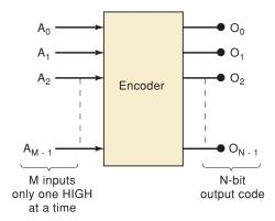
We saw that a *binary-to-octal decoder* (3-line-to-8-line decoder) accepts a three-bit input code and activates one of eight output lines corresponding to that code. An *octal-to-binary encoder* (8-line-to-3-line encoder) performs the opposite function: it accepts eight input lines and produces a three-bit output code corresponding to the activated input. Figure 9-13 shows the logic circuit and the truth table for an octal-to-binary encoder with active-LOW inputs.
