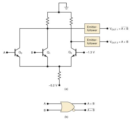
FIGURE 8-42 (a) ECL NOR/OR circuit; (b) logic symbol.
