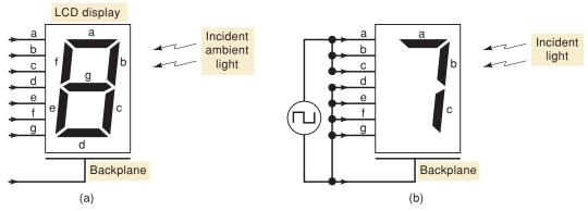
**FIGURE 9-9** Liquid-crystal display: (a) basic arrangement; (b) applying a voltage between the segment and the backplane turns ON the segment. Zero voltage turns the segment OFF.
