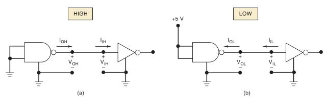
FIGURE 8-1 Currents and voltages in the two logic states.
