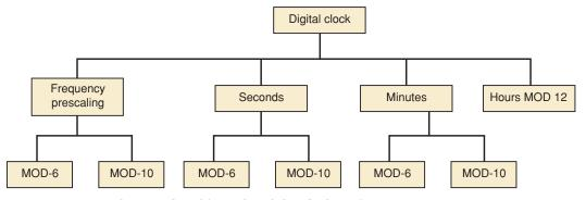
**FIGURE 10-22** The complete hierarchy of the clock project.
