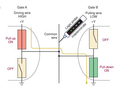
**FIGURE 8-29** Totem-pole outputs tied together can produce harmful current through  $Q_4$ .
