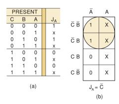
levels at  $J_A$  for each PRESENT state. Of course, for some of the cases,  $J_A$  is a don't-care. To develop the logic circuit for  $J_A$ , we must first determine its expression in terms of C, B, and A. We will do this by transferring the truthtable information to a three-variable Karnaugh map and performing the K-map simplification, as in Figure 7-27(b).
