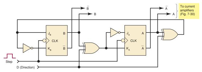
**FIGURE 7-32** Synchronous counter implemented from the *J*, *K* equations.
