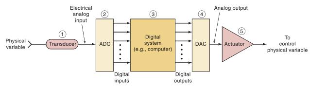
**FIGURE 11-1** Analog-to-digital converter (ADC) and digital-to-analog converter (DAC) are used to interface a computer to the analog world so that the computer can monitor and control a physical variable.
