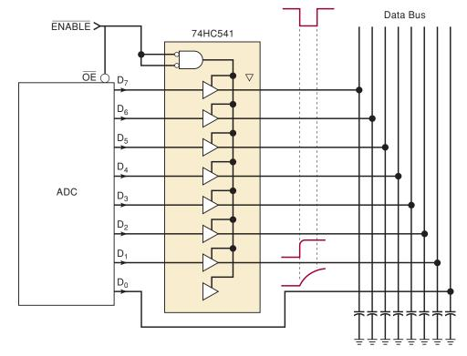
**FIGURE 9-48** Simplified representation of bus arrangement.
