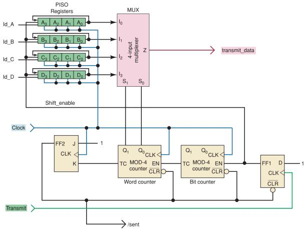
FIGURE 9-32 Transmitter block in synchronous data transmission system.
