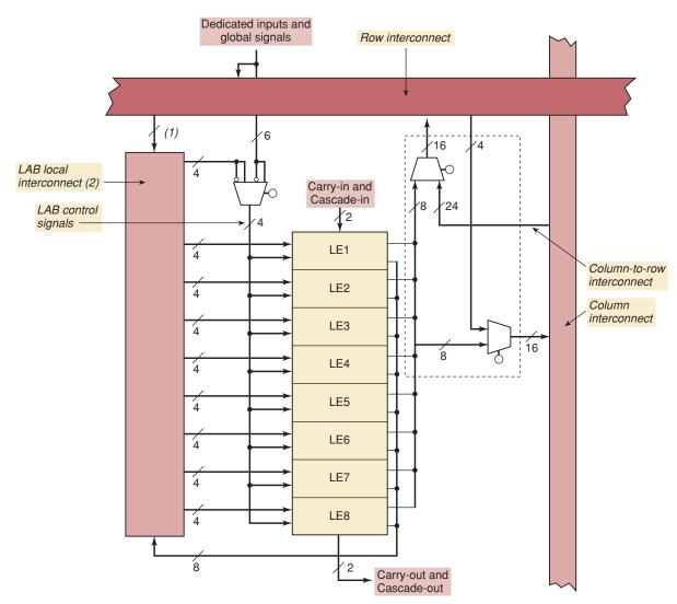
FIGURE 13-17 FLEX10K logic array block. (Courtesy of Altera Corporation.)
