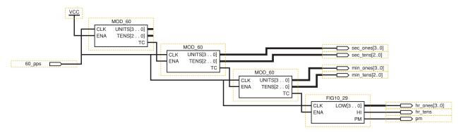
FIGURE 10-34 The complete clock project connected using block symbols.
