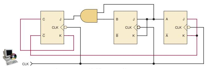
FIGURE 7-23 Synchronous counter with different control inputs.
