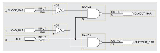
FIGURE 4-33 Logic diagram using schematic capture.
