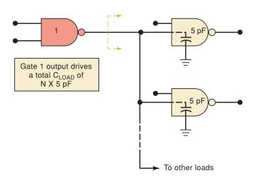
time will be increased in proportion to the number of loads being driven. Typically, each CMOS load increases the driving circuit's propagation delay by 3 ns. For example, NAND gate 1 in Figure 8-26 might have a  $t_{\rm PLH}$  of 25 ns if it were driving no loads; this would increase to 25 ns + 20(3 ns) = 85 ns if it were driving *twenty* loads.
