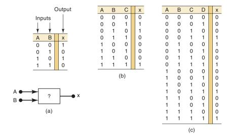
combinations of logic levels present at inputs A and B, along with the corresponding output level x. The first entry in the table shows that when A and B are both at the 0 level, the output x is at the 1 level or, equivalently, in the 1 state. The second entry shows that when input B is changed to the 1 state, so that A = 0 and B = 1, the output x becomes a 0. In a similar way, the table shows what happens to the output state for any set of input conditions.
