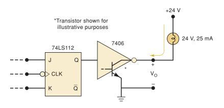
Q=0, the 7406 output transistor turns off; there is no path for current, and the lamp turns off. In this state, the full 24 V will appear across the OFF output transistor so that  $V_{\rm OH}=24$  V, which is lower than the 7406 maximum  $V_{\rm OH}$  rating.
