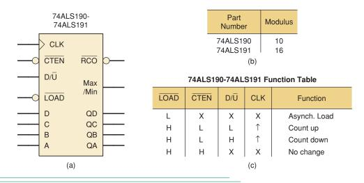
means that as soon as  $\overline{LOAD}$  goes LOW, the counter will be preset to the parallel data on the D, C, B, A (A is LSB and D is MSB) input pins. If the load function is inactive, it does not matter what is applied to the data input pins. The load input has priority over the counting function.
