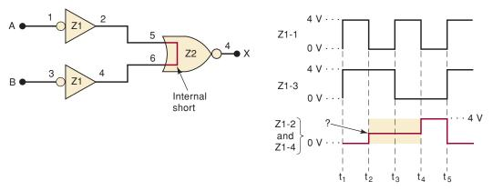
**FIGURE 4-39** When two input pins are internally shorted, the signals driving these pins are forced to be identical, and usually a signal with three distinct levels results.
