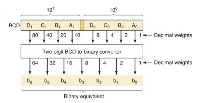
$D_0C_0B_0A_0$ , representing the  $10^0$  or units digit, and  $D_1C_1B_1A_1$ , representing the  $10^1$  or tens digit of the decimal value. The outputs from the converter are  $b_6b_5b_4b_3b_2b_1b_0$ , the seven bits of the binary equivalent of the same decimal value. Note the difference in the weights of the BCD bits and those of the binary bits.
