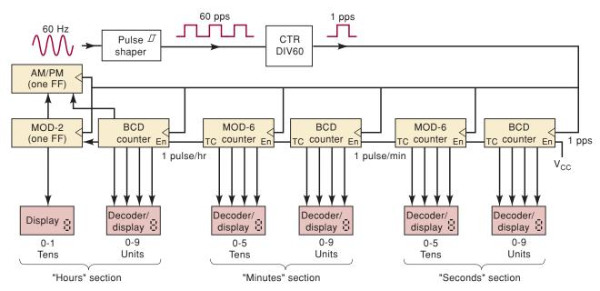
FIGURE 10-17 Block diagram for a digital clock.
