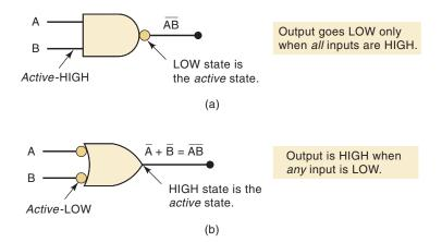
The alternate symbol for a NAND gate shown in Figure 3-34(b) has an active-HIGH output and active-LOW inputs, and so its operation can be stated as follows:
