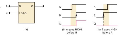
In order for this circuit to work properly, *A* must go HIGH prior to *B* by at least an amount of time equal to the setup time requirement of the FF.
