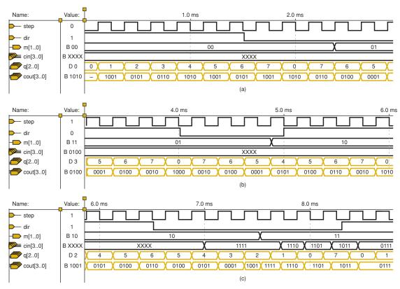
FIGURE 10-10 Simulation testing of the complete stepper driver.
