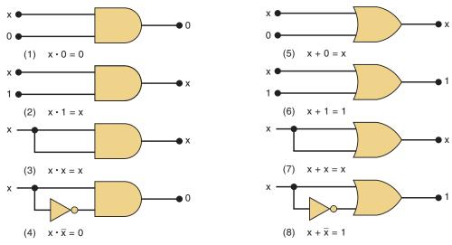
FIGURE 3-25 Single-variable theorems.
