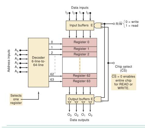
ranging from 0 to  $63_{10}$ . In order to select one of the 64 address locations for reading or writing, a binary address code is applied to a decoder circuit. Because  $64 = 2^6$ , the decoder requires a six-bit input code. Each address code activates one particular decoder output, which in turn enables its corresponding register. For example, assume an applied address code of
