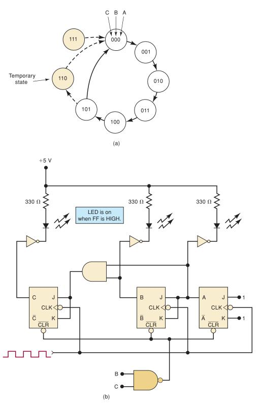
**FIGURE 7-7** (a) State transition diagram for the MOD-6 counter of Figure 7-6. (b) LEDs are often used to display the states of a counter.
