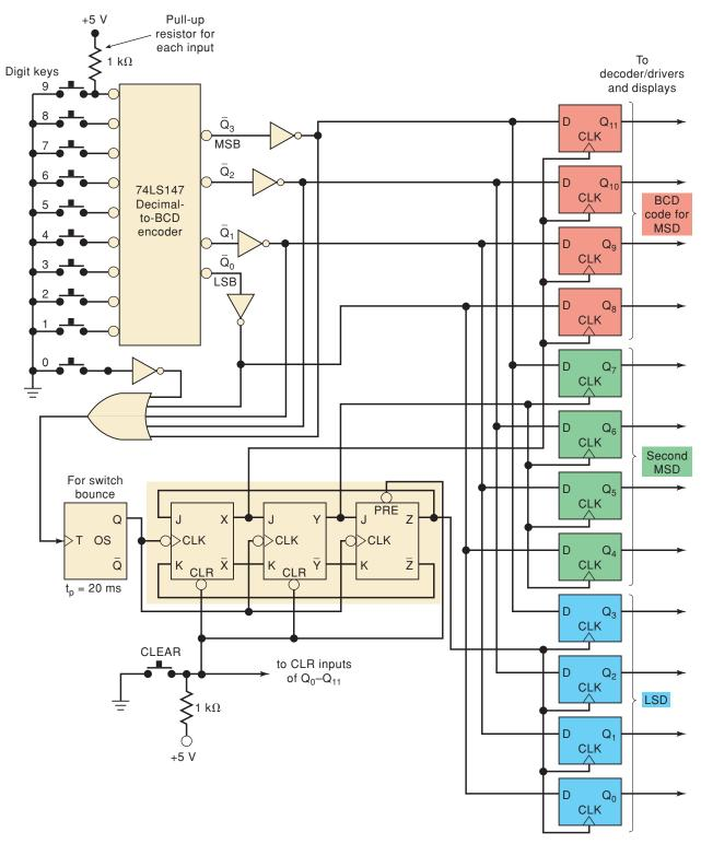
FIGURE 9-16 Circuit for keyboard entry of three-digit number into storage registers.
