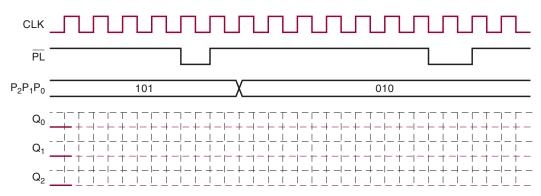
FIGURE 7-95 Problem 7-16 timing diagram.
