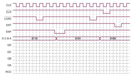
FIGURE 7-97 Problem 7-18 timing diagram.
