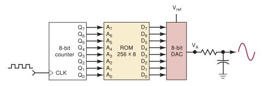
FIGURE 12-18 The ML2035 programmable sine-wave generator. (Courtesy of MicroLinear Corp.)
