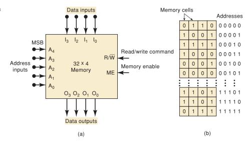
of the memory locations for a read or a write operation, the five-bit address code for that particular location is applied to the address inputs. In general, N address inputs are required for a memory that has a capacity of  $2^N$  words.
