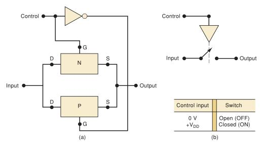
FIGURE 8-43 CMOS bilateral switch (transmission gate).
