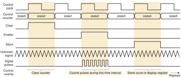
FIGURE 10-40 Frequency counter timing diagram.
