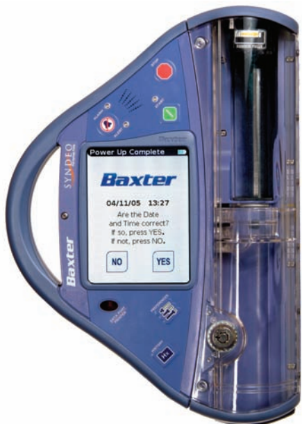
FIGURE 14-15 Syndeo PCA (patient-controlled analgesia) syringe pump (Photo courtesy of Baxter Medication Delivery)
