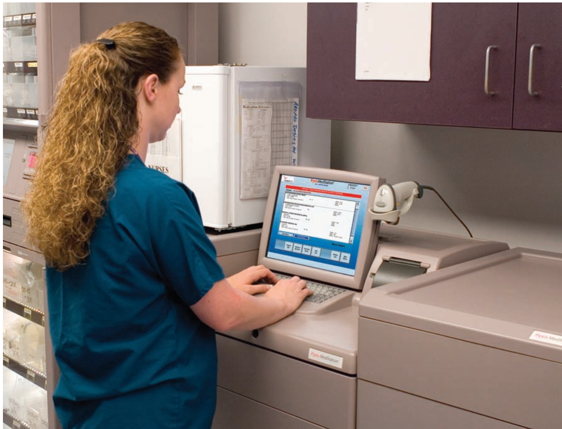
FIGURE 9-7 The Pyxis MedStation® is an example of an Automatic Medication Dispensing Machine (Photo Courtesy of Cardinal Health)
