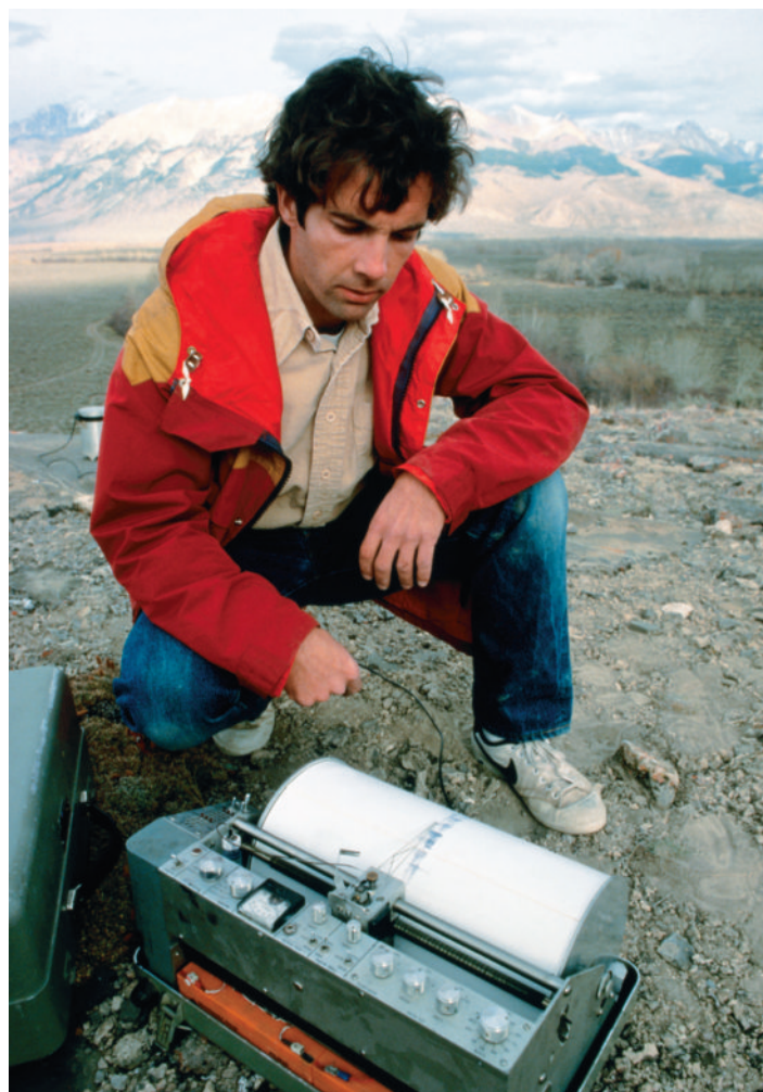
FIGURE 1.9 This field geologist is checking a seismograph. (Photo by Andrew Rafkind/Getty Images Inc.—Stone Allstock)
