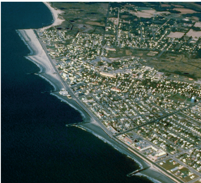
FIGURE 20.18 Groins along the New Jersey shore at Cape May. (Photo by John S. Shelton)
