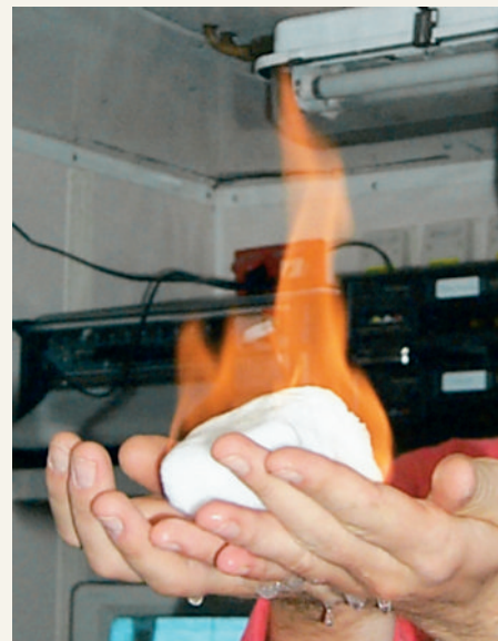
FIGURE 23.B Gas hydrates evaporate when exposed to surface conditions and release natural gas, which can be ignited. (Photo courtesy of GEOMAR Research Center, Kiel, Germany)
