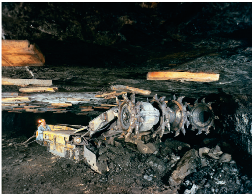
FIGURE 23.6 A. Modern underground coal mining is highly mechanized and relatively safe. (Photo by Melvin Grubb/Grubb Photo Services, Inc.) B. Strip mining of coal at Black Mesa, Arizona. Surface mining is common when coal seams are near the surface. (Photo by Richard W. Brooks/Photo Researchers, Inc.)
