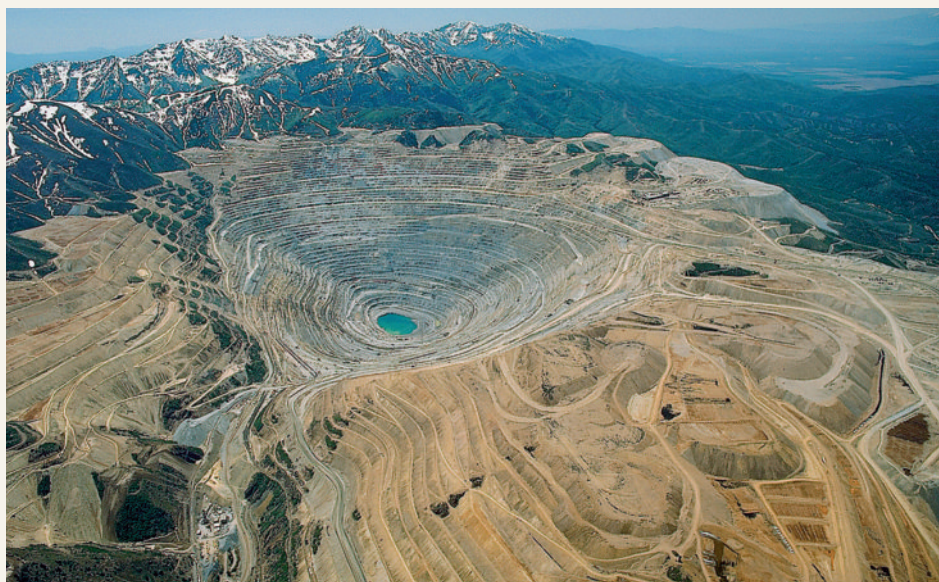
FIGURE 23.C Aerial view of Bingham Canyon copper mine near Salt Lake City, Utah. This huge open-pit mine is about 4 kilometers across and 900 meters deep. Although the amount of copper in the rock is less than 1 percent, the huge volumes of material removed and processed each day (about 200,000 tons) yield significant quantities of metal. (Photo by Michael Collier)
