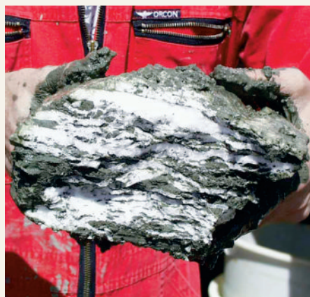
FIGURE 23.A This sample retrieved from the ocean floor shows layers of white icelike gas hydrate mixed with mud. (Photo courtesy of GEOMAR Research Center, Kiel, Germany)
