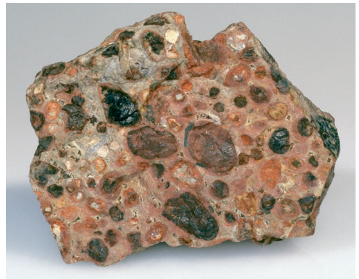
FIGURE 23.25 Bauxite is the ore of aluminum and forms as a result of weathering processes under tropical conditions. Its color varies from red or brown to nearly white. (Photo by E. J. Tarbuck)
