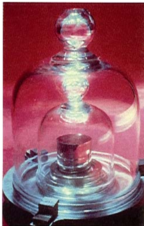
Figure 1.6 The standard kilogram mass.
