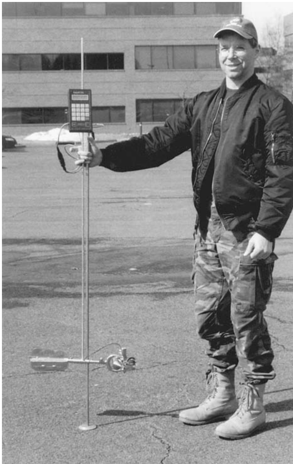
FIGURE 4-11 Price Type AA current meter mounted on a wading rod for use in shallow conditions up to 4 feet deep.
