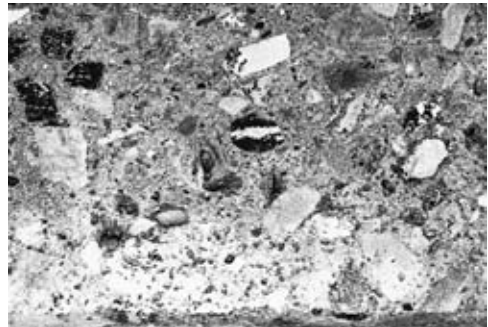
FIGURE 11.11 Cross section of portland cement concrete showing cement paste and aggregate particles.
