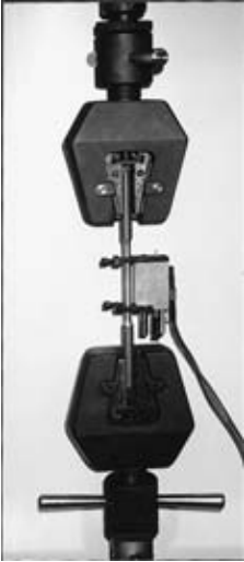
FIGURE 3.12 Tension test on a round steel specimen showing grips and an extensometer with an LVDT.
