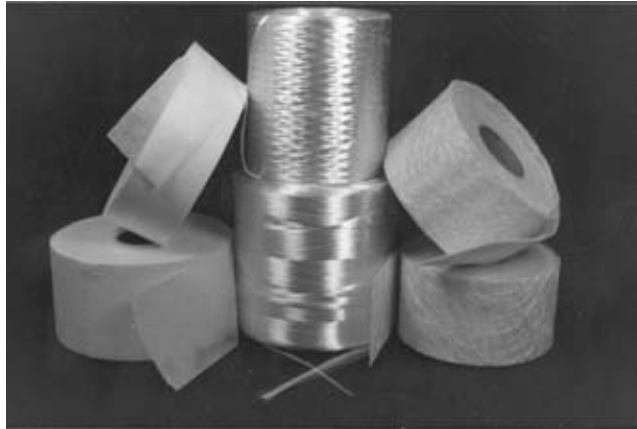
FIGURE 11.3 Common glass fibers (veil, roving, and mat). Photo courtesy of Creative Pultrusions, Inc.
