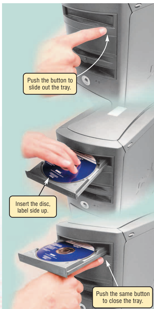
FIGURE 19 On optical disc drives, you push a button to slide out a tray, insert the disc, and then push the same button to close the tray.
