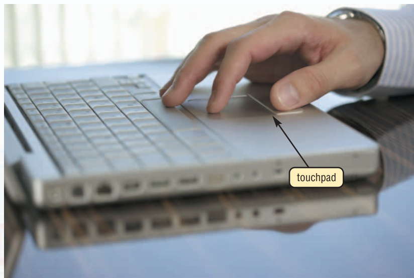
FIGURE 8 Most notebook computers have a touchpad that allows a user to control the movement of the pointer.
