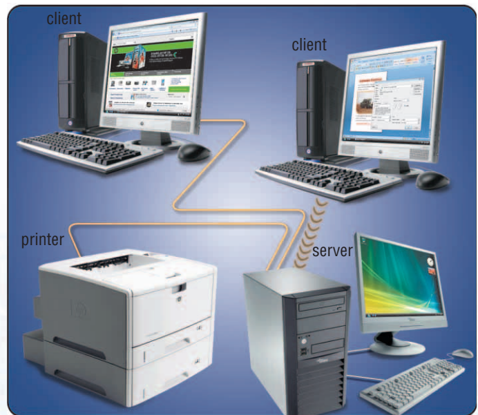
FIGURE 33 The local area network (LAN) enables two or more separate computers to share the same printer.
