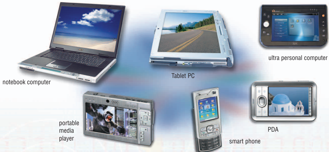
FIGURE 14 Notebook computers, Tablet PCs, ultra personal computers, portable media players, and most PDAs and smart phones have color LCD screens.
