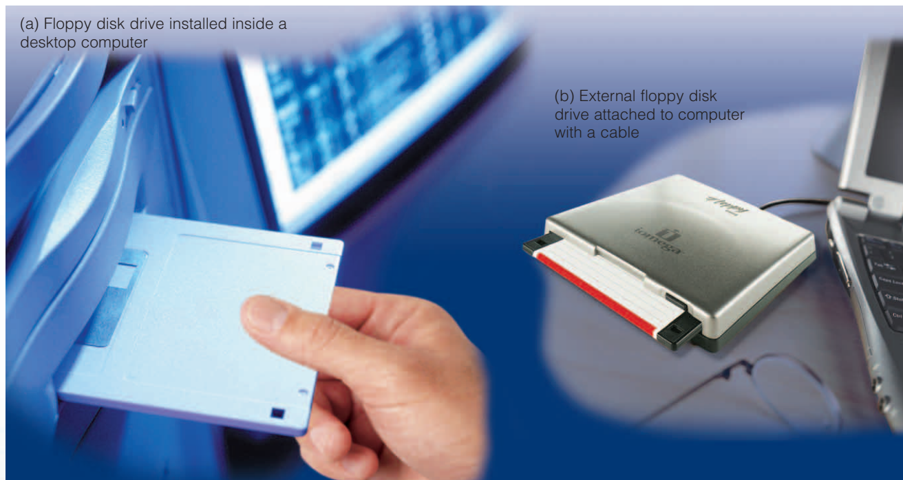
FIGURE 18 On a personal computer, you insert and remove a floppy disk from a floppy disk drive.
