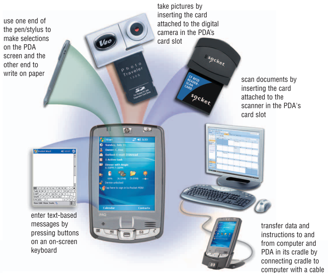
FIGURE 5 Users enter data and instructions into a PDA using a variety of techniques.
