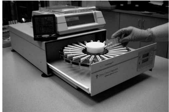
■ FIGURE 14-12 A gel card is loaded into a centrifuge. The gel test employs the principle of controlled centrifugation of RBCs through a dextran-acrylamide gel/reagent matrix contained in a specially designed microtube.
