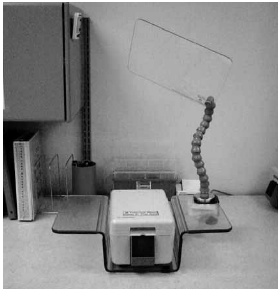
■ FIGURE 14-5 This sterile docking device allows for entry into donor units without affecting the expiration date of the product.
