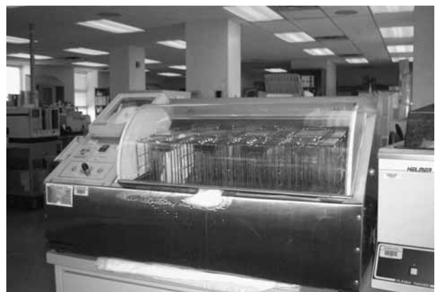
■ FIGURE 14-6 Platelet rotators prevent the formation of platelet aggregates and optimize the exchange of gases required for platelet survival.
