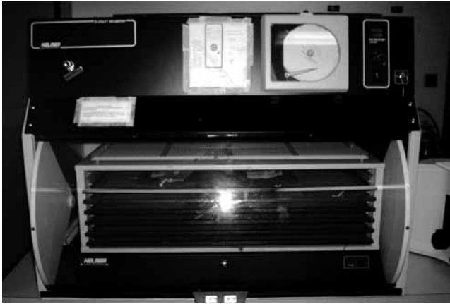
■ FIGURE 14-7 Flatbed agitators like this one provide optimal environmental conditions for platelet viability during storage.
