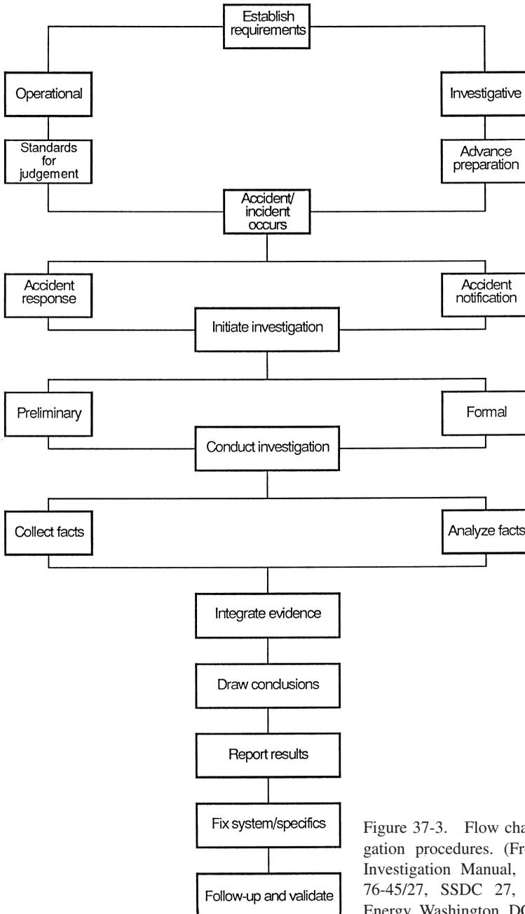
Figure 37-3. Flow chart of accident investigation procedures. (From Accident/ Incident Investigation Manual, 2nd ed., DOE/SSDC 76-45/27, SSDC 27, U.S. Department of Energy, Washington, DC, November, 1985.)
