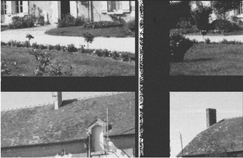
**Figure 3.17** *Embedded digital audio as viewed on pulse-cross monitor*
