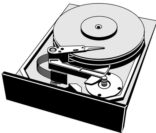
**Figure 8.29** *Hard disk-drive construction*
