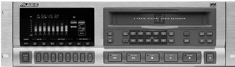
**Figure 7.8** ADAT rotary digital multi-track machines
