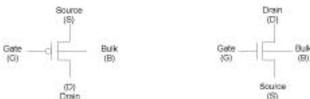
**Figure 2.1** PMOS and NMOS transistors.
