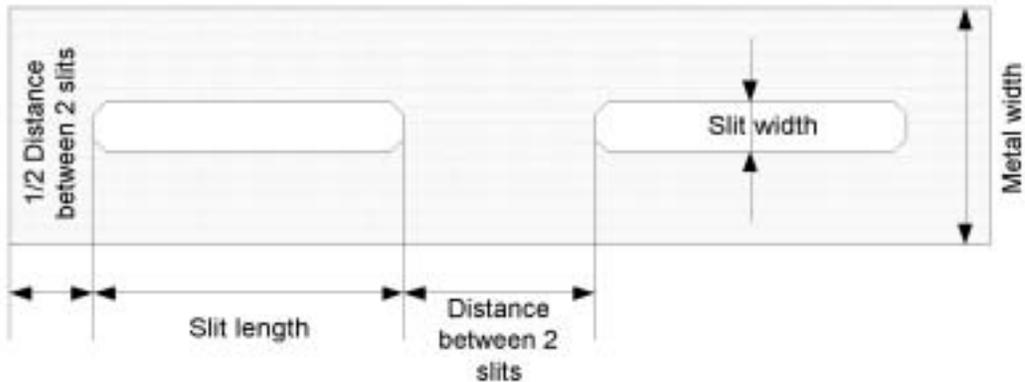
**Figure 8.2** Metal slit example and design rules.
