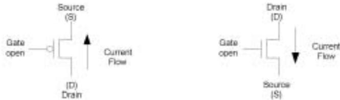
**Figure 2.2** PMOS gate open and NMOS gate open.
