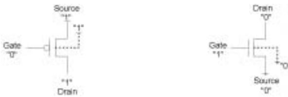
**Figure 2.5** MOS transistors showing implied bulk connections.
