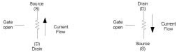
**Figure 2.3** PMOS resistor model and NMOS resistor model.
