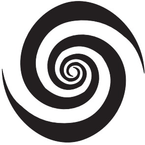
Figure 13.9 A spiral antenna where the metal areas are identical to the spaces between
