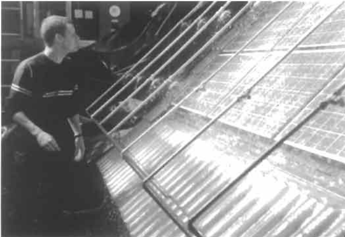
Figure 7 Shell PV roof undergoing 'Prescript' test in Solar Simulator at Cardiff, UK.
