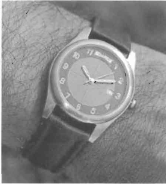
Figure 2 Solar watch incorporating a round array of four amorphous silicon solar cells.
