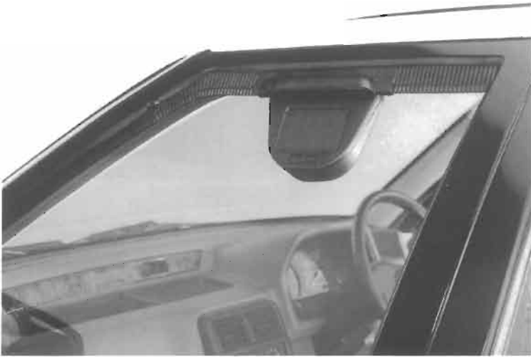
Figure 8 An AutoVent Turbo fitted in the front window of a parked car. The thin film solar cell array inside the window powers a fan, which exhausts stale air out over the top of the window glass.
