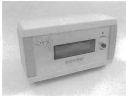
Figure 2 A domestic PV output display receiving radio-linked data from a sensor next to the inverter. (Photo EETS.)
