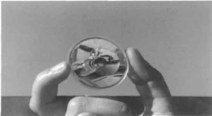
Figure 14 XRI concentrator allowing 1000+x geometric concentration with \pm 1.5^\circ acceptance angle. It is envisaged that such compact mini-concentrators will provide adequate optics for high-efficiency third generation micro-cells (IES, 1994).
