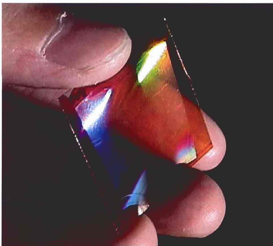
FIGURE 14.31 Photograph of two SRGs inscribed on an azopolymer film using a flexible plastic substrate.
