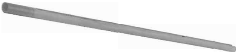
Figure 8.14 Photograph of a single tubular SOFC. (Courtesy of Siemens Westinghouse Power Corporation.)
