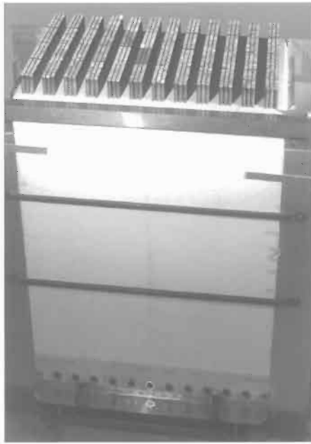
Figure 8.19 Photograph of a 100 kW tubular cell stack, showing 48 bundles of 24 cells each. (Courtesy of Siemens Westinghouse.)
