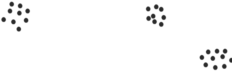
FIGURE 12.1: Three clusters are formed by the feature vectors. When q is constrained to a value less than 3, the BSAS algorithm will not be able to reveal them.
